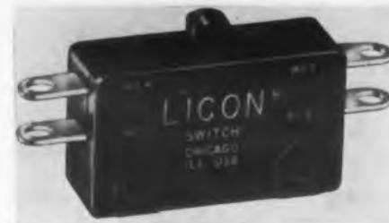
This switch is 1/4 in. thick and 25/32 in. long and gives a life cycle consistently over 5 million. It is rated 10 amps, 30 v dc inductive at a time constant of 0.026 sec which is four times greater than other switches can handle. Movement differential is 0.010 to 0.020 in. A wide range of forces is available, with a nominal of 6 oz.
