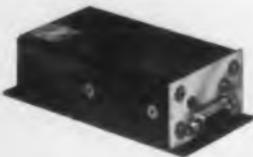
REL-103 GALVANOMETER AMPLIFIER... performs the functions of amplifying and impedance transforming low level signals from Barium Titanate transducers to a level and impedance suitable to drive fluid damped optical galvanometers and similar devices.
