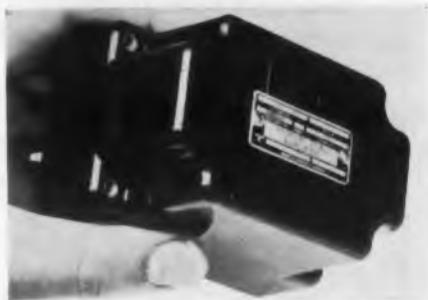
The type PA3C-1 magnetic amplifier is designed specifically to provide proportional temperature control of a heating element in response to a change in resistance of a temperature sensor. Power output is proportional from 0 to 100 w, 400 cps, as the temperature sensing element resistance changes by approximately 1 ohm. Nominal output load is 130 ohms.
