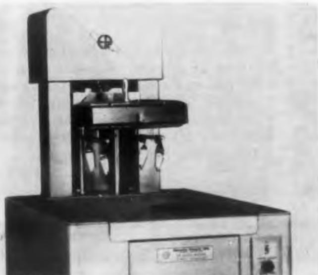
This EPC dip soldering machine, is a production and laboratory tool to facilitate semi-automatic production of electrical and electronic assemblies and circuit boards utilizing printed and etched circuit techniques. The machine has a capacity of 120 units per hr. and requires only one operator.
