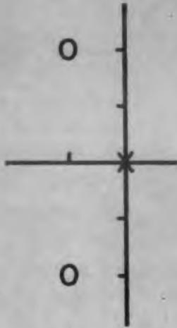
Fig. 3. Pole-zero pattern of the transfer ratio  $E_o/E_1$  of Fig. 1.
