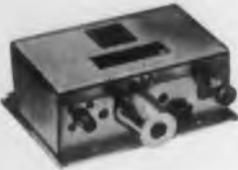
REL-09 R-F POWER AMPLIFIER... provides power amplification over the 215-235 mc telemetering band. With 1.4 watts input drive, will deliver an 11 watt output to a 52-ohm load.
