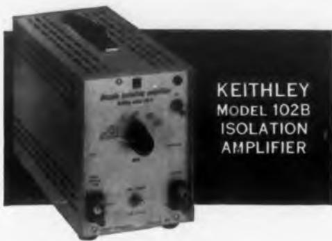
**TYPICAL** applications are: vibration and noise studies, work with accelerometers and hearing aids, and pulse amplification. A 5-volt 50-ohm output is provided for driving oscilloscopes, sound level meters, and pen recorder power amplifiers.
