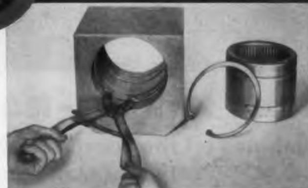
Assembly is simple, even with giant 7" diameter Truarc ring. Special Truarc ratchet pliers grasp the ring securely, ease it into the groove, snap it securely into position. Smaller pliers and various high-speed assembly jigs are available for other rings, permit assembly-disassembly to be performed rapidly even by unskilled labor.
