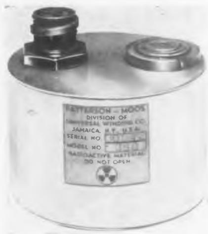
**T**IME delays from milliseconds to forty hours with an accuracy of  $\pm 3$  per cent from  $-65$  to  $165$  F are obtained by combining a nuclear battery (25 year shelf and use life) with gas diode circuitry in one miniature unit. The timer weighs about six oz and is able to withstand extremes in pressure, vibration, jolt, jumble and brutal acceleration.
