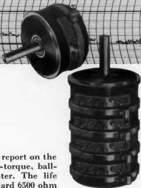
Take for instance a recent test report on the TIC Type ST20, a 2-inch, low-torque, ball-bearing precision potentiometer. The life test was conducted on a standard 6500 ohm unit. At 30RPM the ST20 was subjected to 700,000 cycles, reversing direction every 30 minutes. The linearity graphs shown above show the before and after of the ST20's independent linearity. *As can be seen, the linearity change is imperceptible.*
