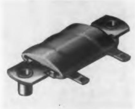
Vitrohm stack mounting type resistors in characteristic V for styles RW20 to 24 are recommended for electronic and other applications where space for components is limited. Stack mounting power resistors feature strong oval-shaped ceramic cores, low mounting brackets and Vitrohm (R) construction. Power ratings in Characteristic V range is from 21 to 91 w, while resistance values are available from 0.8 to 71,000 ohms.
