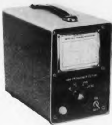
Fig. 2. Preamplifier increases microphone output level to a value easily measured with a VTVM. Low frequency cutoffs are provided at 50, 250, and 1250 cps, to improve signal to noise ratio.
