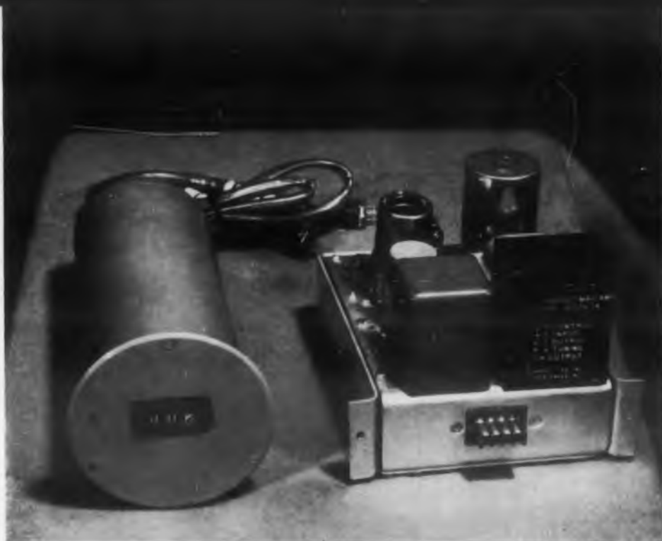
Fig. 1. Unusual flexibility and compactness are provided in this digital voltmeter.
