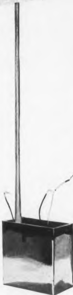
These miniature electronic components potted in Epon resin will withstand solder bath temperatures and retain excellent dimensional stability.
