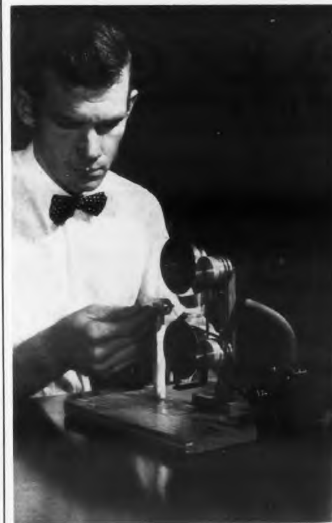
"Pinhole" Coil Winder developed by Stanford Research Institute's Computer Development Group. Core is held in clamp immediately to left of operator's hand.
