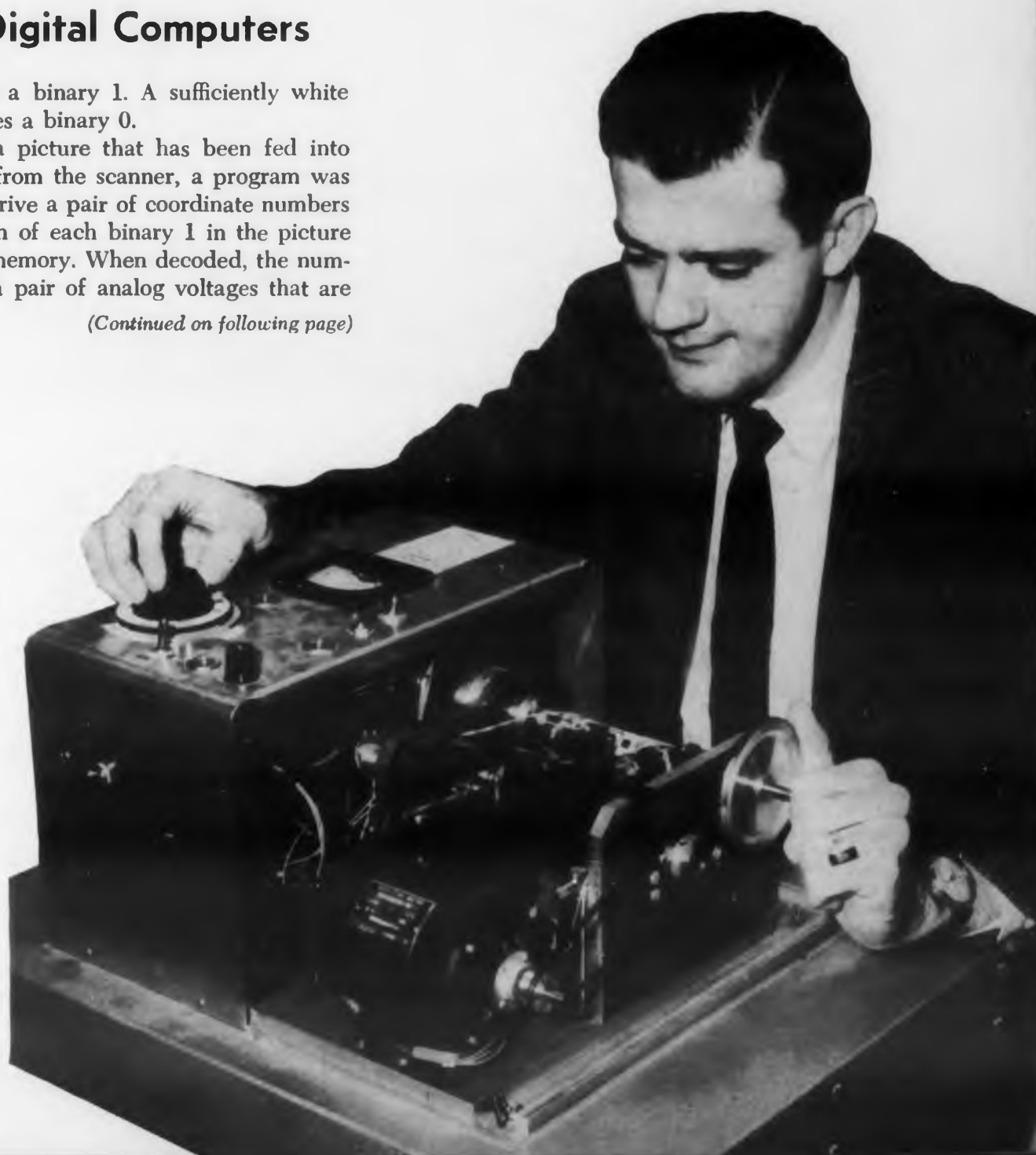
Fig. 1. Photograph to be scanned is mounted on a drum 2/3 in. in diam. As the drum rotates a photomultiplier and a source of illumination mounted on a lead screw move parallel to the axis of the drum. A mask in the optical system illuminates a 0.25 mm square and a strobe disc produces optical pulses for each 0.25 mm of drum rotation. The photo-multiplier can examine the relative reflectance of each 0.25 mm square.
