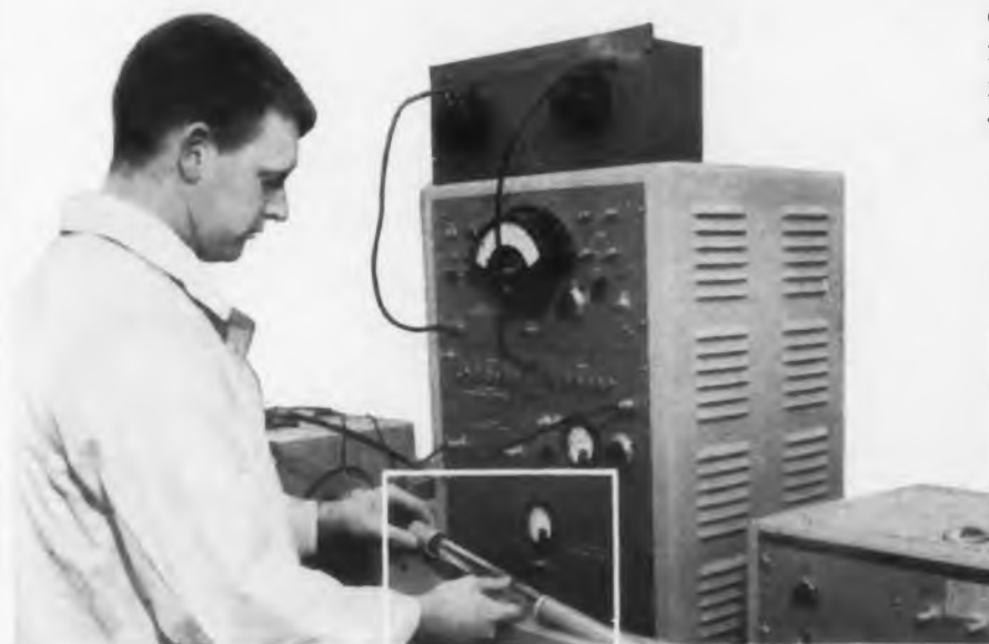
Microwave test equipment used in calibrating all Bendix noise source tubes.
