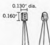
These new Raytheon Submin Transistors have one-fourteenth the volume of the JETEC-30 package.
