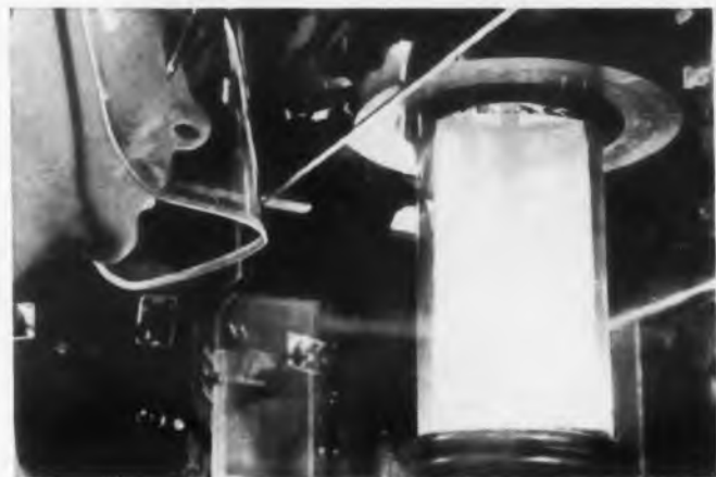
Molten Ladle of silicon is watched during first step in the precise manufacture of Hughes semiconductors. Constant innovations in Research, Development and Manufacture have positioned Hughes Products as a commercial electronics leader.
