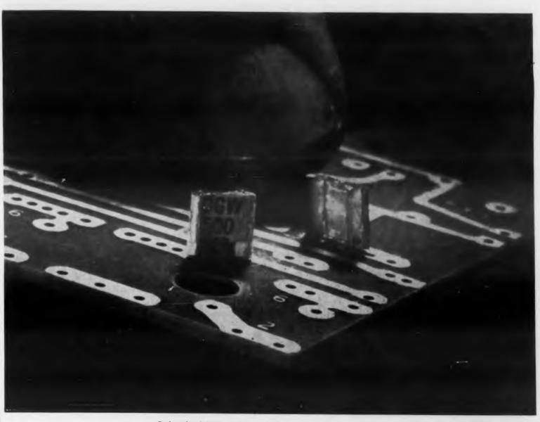
Truly sub-miniature, these capacitors were devised especially for printed circuits and automatic assembly. Since they retain all the properties of larger, pig-tail capacitors, they are well sulted to general circuitry as well.
