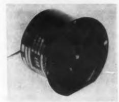
Weighing less than four ounces, this axial lower measures 1-1/2 in. length, 2 in. diam., it a 2-1/2 in. mounting flange. It is single capsula have, operating on 27.5 v 400 cps or on 115 v tion ps, and delivers 10 cfm at 0.11 in. static resure with 5 w input.
