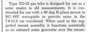
Typical applications for the tube are: radio receiver calibration; radiometer; micro-wave radio relay; radio telescope reference; and as a noise measurement standard.
