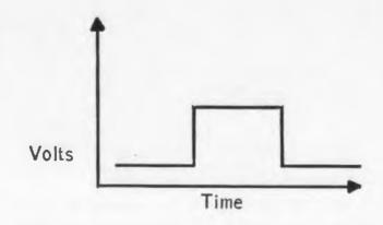
Figs. 6. and 7. When rectangular pulse (Fig. 6 above) is impressed on circuit (Fig. 7 below),  $R_{\rm k}$  is effectively zero for the transient rise and fall but not for the flat top. In effect, the circuit differentiates the pulse.
