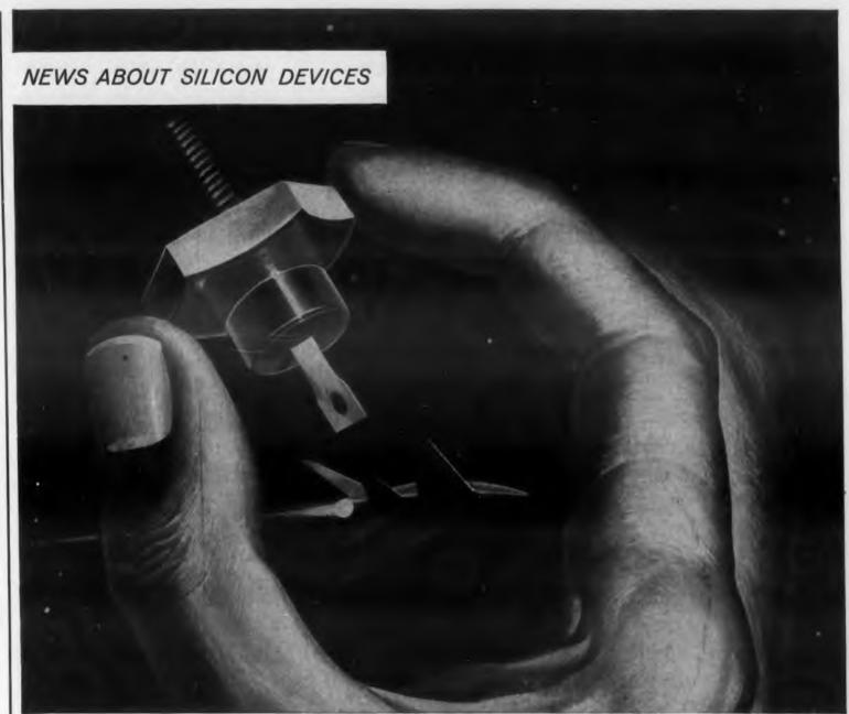
SILICON RECTIFIERS are finding increasing use at elevated temperatures in aircraft and missile applications by providing more power per pound.
