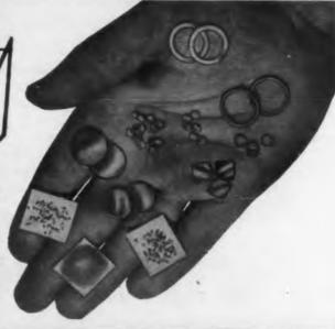
. . FIRST to pioneer the development of solder metals & alloys for the semi-conductor field. Made from indium, indium-gallium, indium-gold, indium-tin, indiumlead, gold-antimony, gold-gallium, tin, tin-antimony, tinlead, tin-arsenic, lead-antimony, lead-arsenic, aluminum, aluminum-tin, platinum, and others. From "stock" or to your specification.
