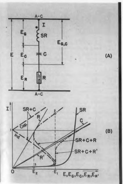
Fig. 6-1. Ferro-resonance. (A) Series, non-linear resonant circuit. (B) Voltage and current relations. (Voltages are rms).
