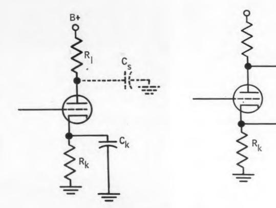
Fig. 5. For voltage-gain stabilization, this circuit can be used with unbypassed cathode; or, to extend the bandwidth,  $C_k$  can be chosen to bypass during roll-off caused by  $C_s$ .
