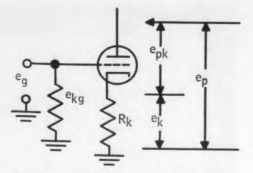
**Fig. 4.** Basic cathode follower circuit. If load (cathode) resistance is not too small, large positive low-duty-cycle pulses can be passed with low distortion because of inherent self-biasing feature.
