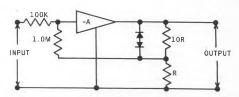
A double-anode "zener" diode in the amplifier feedback loop changes the gain whenever the output exceeds the breakdown voltage of the diode.
