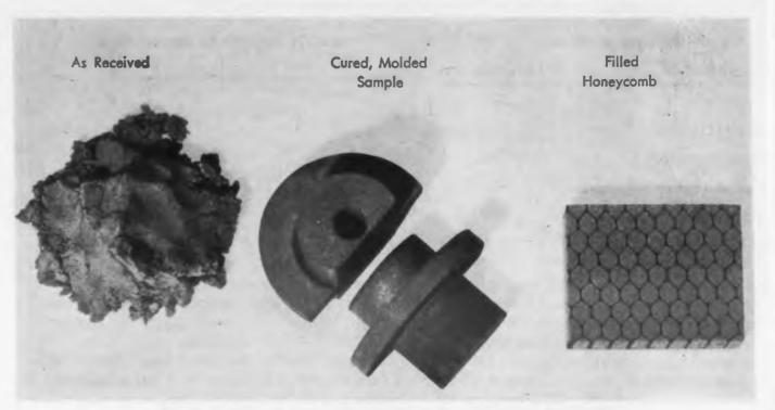
Fig. 3. Artificial dielectric "Pack-in-place" foam Eccofoam HI K 625D.
