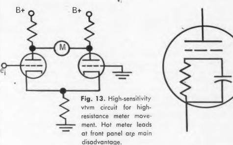
Fig. 14. Tube symbol showing cathode-interface effect, resulting from leaving heaters on standby with plate voltage removed. A "drooping" pulse output results.
