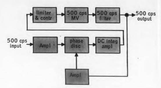
Fig. 1. Electronic filter servo.
