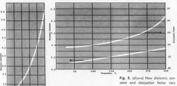
Fig. 4. (left) Dielectric Constant VS Dissipation Factor at Room Temperature for a typical epoxide Artificial Dielectric Foam at 8600 Mc.
