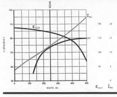
Fig. 3. Empirical performance curves of a typical static inverter. At 250w rated output efficiency is about 74 per cent.
