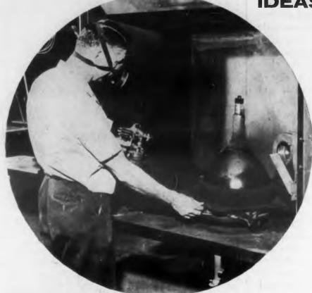
Television tube being sprayed with "dag" colloidal graphite. For exterior use the graphite is dispersed in lacquer, providing a smooth, black, adherent, conductive coating on any type of glass.
