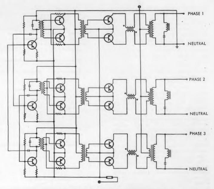
Fig. 1. Basic schematic of a static inverter. Inversion system used is switching (class D): transistors are driven from saturation to cutoff; resultant square waves are filtered at the output. Theoretical efficiency and power levels are very high.
