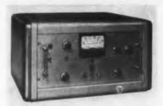
Model C-2910, spectrometer is designed to count only those pulses lying within a selected channel defined by front panel controls, and can provide from 750 to 2000 volts with a regulation of 0.01 per cent of the ac line voltage. Maximum counting rate is 10,000 counts per sec. Five different ranges are provided for both count rate and integral methods of operation.
