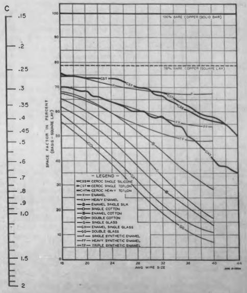
Fig. 2. Typical comparative wire space factors, on the basis of each turn being placed directly on top of the one below it (i.e. square lay), with no allowance for interleaving layers of insulation. The winding space factor (S<sub>10</sub>) as used in this article is less than the wire space factor, since it represents the fraction of the window area filled with pure conductor. (Source-Sprague Electric Company Engineering Bulletin No. 400 A.)
