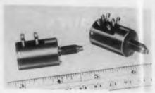
Type 75-M28 sealed trimining potentiometer is particularly suited for moisture or shock and vibration conditions. The aluminum housing makes possible a dissipation of 2 w when the trimmer is panel mounted. Resistance values per section of up to 50,000 ohms can be provided in a standard 1-1/8 in. housing length, with higher resistance values available with a slight increase in housing length.
