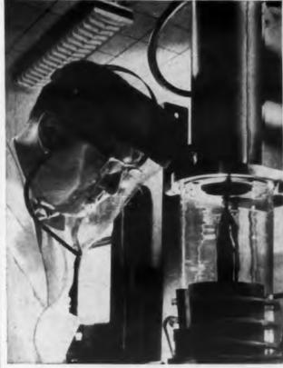
In the center of the quartz housing, a germanium crystal is being grown. A "perfect crystal lattice," it will be cut into wafers 3/10ths of an inch square and less than 1/100th of an inch thick to become the heart of Delco High Power transistors.
