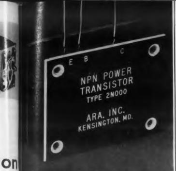
omposite high-gain, high power transistor can be sed as switching device or small signal parameter mplifier. Maximum power is 10 w; undistorted class-A
