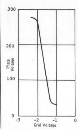
Fig. 5. (left) Gain characteristics of the DC amplifier.
