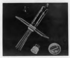
This Teflon miniature tube socket requires no mounting hardware thus saving space and assembly time. The socket is pressed into a single chassis hole, slightly smaller than the Teflon body of the socket.
