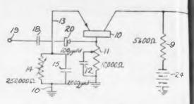
The patent points out that the tin interval for the trigger pulses must be greater than the time interval of the sat tooth wave of the emitter circuit at must be less than twice this time interval. With the values shown on the figure the delayed pulse may be varied betwee 160 and 320 microseconds.
