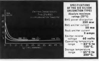
The unijunction features open-circuit-stable negative resistance characteristics. In switching and oscillator applications, one unijunction not only does the work of two transistors with less circuitry, but the circuit is also more stable over a wide temperature range.
