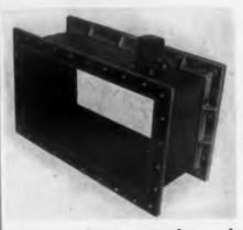
Operating by means of a probe otating in the plane of circular olarization of a wave-guide, this otary standing wave indicator proides a non ambiguous read-out of he sign of reactive components. Measurement of vswr, reflection oefficient angle, hence impedance, the low frequency range, is simlified. The unit is available in vaveguide sizes from WR-650 to VR-4200. If desired, the rotating robe can be motor driven for renote operation and to provide an c) general scilloscopic presentation of vswr.
