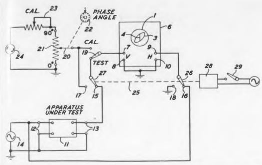
the same frequency is measured by pidly switching the cathode ray tube display sequentially the elliptical Lisjous figure and a vertical line which st reaches the intercept points of the lipse on the vertical axis. The vertical ne is generated by an ac voltage from source which is calibrated in terms of hase angle. A mercury relay may be sed to switch the signals to a high perstence oscilloscope.
