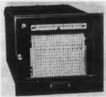
This 5-in. strip chart recorder is available with a variety of ranges by means of plug-in resistors, for thermocouple, resistance bulb and linear millivolt spans. Chart speeds are from 1 in. per hr to 2 in per sec. Total panel space required is 9-5/8 in. wide by 8-1/2 in. high.
