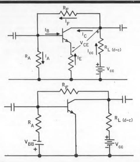
**Fig. 3.** Voltage and current feedback.
