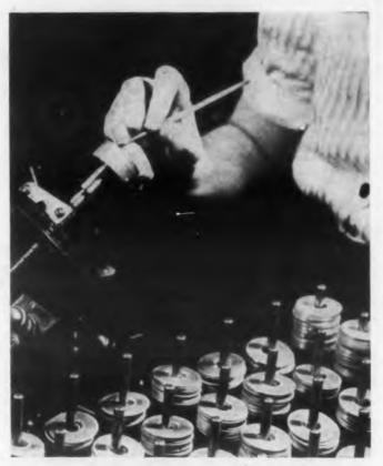
Copper oxide rectifier discs being painted with "Aquadag," a colloidal graphite. The dispersion fills the cavities in the relatively rough, crystalline surface, producing a smooth surface with large contact area.
