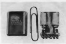
This dual-coil relay, model SL, operates on a 1-w, 3-msec pulse to either coil. A magnetic latch and high contact pressures hold the contacts closed under 100 g shock and 30 g vibrations to 2000 cps. The relay will switch loads up to 2 amp at 30 v dc resistive or 1 amp at 115 v ac resistive, and operates in ambient temperatures from -65 to +125 C.
