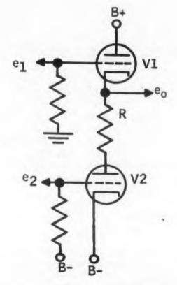
Fig. 9. Summer circuit which can be designed for any predetermined dc component in output.
