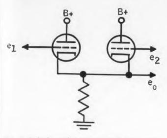
**Fig. 8.** Cathode-coupled summer circuit used in computers.
