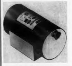
Model 24614 ac accelerometer provides a very low threshold on the order of 0.0017 g for a 10 mv output. Available in low natural frequencies, and in ranges from ±1 g to ±20 g, the instrument provides an ac output proportional to linear acceleration parallel to its mounting base. Full scale output is 6 v, with a maximum null of 0.015 v. The output can be fed directly into a relatively low impedance with little or no phase shift.
