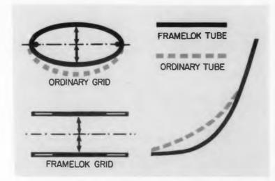
Uniform transfer characteristics of the Framelok Grid tube result largely from greater control of both major and minor dimensions of the grid. Above is a graphic representation of variations in characteristics which result from distortion of the minor dimensions in wound grids. Since both major and minor are fixed in the rigid frame grid, these variations are virtually eliminated.
