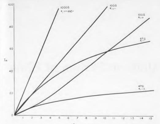
Fig. 12. Meter current in vtvm circuit versus input voltage. For lower values of cathode resistor, positive swing of meter current is limited as shown, giving protection to meter on overloads.
