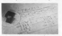
Model CTR-250 magnetic core shift register elements can operate up to 250,000 shifts per sec
