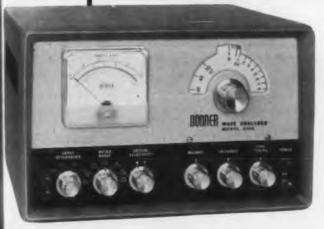
Donner's new Model 2102 Wave Analyzer accurately measures implitude and frequency for each component of a complex input waveform, whether or not the components are harmonically related. Selectivity, controlled by a front panel switch, provides narrow or wide band pass. Narrow selectivity permits easy eparation of input signal components. Broad selectivity permits A phote rapid scanning of the spectrum.
