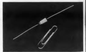
Model CX7A1H copper oxide diode is for a in low voltage, low current applications. The air is insulated by nylon tube housing, 3/8-in. low by 3/16-in. od, through which the leads are serted. Specifications for instrument use are: or rent rating of 2 ma continuous duty, ac implementary of 8 max, peak inverse of 8-1/2 v max. In other applications, the current value can be creased 5 times and voltage value doubled. Max mum temperature rating is 85 C.
