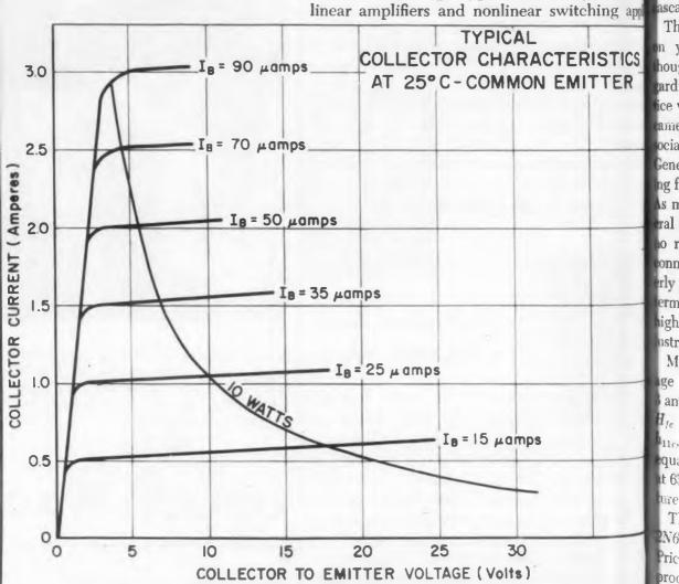
Characteristic curve of the germanium-silicon npn power transistor.
