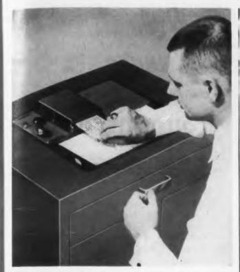
**Sliding punched card** into the slot actuates the switch. Knob on the left releases it.
