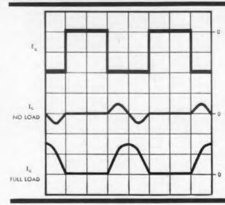
Fig. 2. Voltage and current wave forms for one transistor of a push-pull pair, no load and full load.
