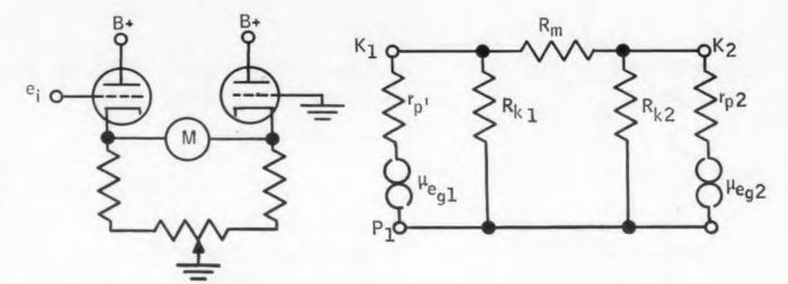
Fig. 11. Cathode-coupled vtvm circuit and equivalent.
