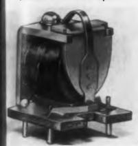
The LR-1301 relay, for printed rcuit mounting, has palladium incontacts to assure good contact dry circuit switching. Coil retances up to 10 K can be had in ther treated or un-treated coils. ne terminal mounting block can furnished in either glass epoxy, ass silicone, or phenolic. Overall mensions are 3/4 in. square by 8 in. high; weight, 13 grams. American Monarch Corp., Amer-
