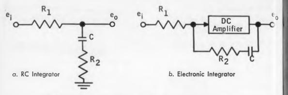
Fig. 3. Comparison of an RC Integrator with an Electronic Integrator.
