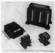
Coil construction and high temperature insula tion permits miniaturization in these trans formers. The units have a 10,000 hr life in 125 ambients, with temperatures to 175 C available shorter life applications. Units have been a proved to Mil-T-27A Grade 5 Class T Life specifications. The construction includes a mois ture barrier which prevents moisture penetration without using bulky encapsulation. Encapsulation tion techniques permit complete saturation
