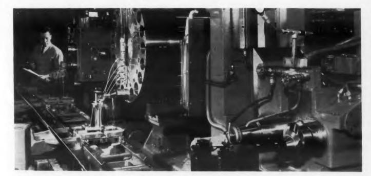
**Completely operated** by Digitape electronic controls, the milling, drilling, and boring machines (above, I. to r.) pass parts along automatically. Transistorized digital computers convert information contained on tapes (at right) into operational instructions.
