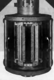
The new 512A Bryant general purpose magnetic storage drum meets the exacting demands of all permanent storage problems, yet is versatile enough to be used as a laboratory instrument. These 5" dia. x 12" long drums are stocked for immediate shipment at a price that is far below the cost of customer-designed drums.
