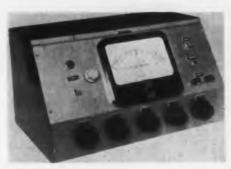
Intended to indicate the percentage deviation of a sample resistor from a standard resistor, type 957 bridge offers very high accuracy over a resistance range from 1 ohm to 10 meg through the use of a chopper-stabilized feedback amplifier. Accuracy as a limit bridge is better than 0.05 per cent for resistances greater than 10 ohms.
