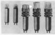
These units provide three degrees of side visibility in models designated 1 DH 6, 1 DH 7, and DH 8, respectively. The replaceable-lamp indicators were designed expressly for the T-2 lamp which provides longer operation in 6, 12, 24, and 8 v incandescent lamp ratings and extra visibility in neon types. Lenses are butyrate; cases are luminum, either black or aluminum-anodized.
