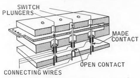
**Top portion** of switch assembly down showing how plungers are pushed to close contacts.
