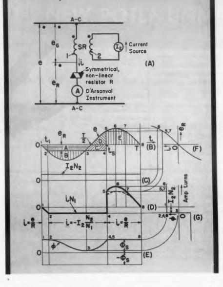
Fig. 5-1. DC without rectifiers. (A) Circuit diagram, (B) Voltage inventory, (C) Ampereturns in winding 2, (D) Ampere-turns in winding 1, (E) Core flux, (F) Voltage-current characteristic of non-linear, symmetrical resistor R, (G) Flux-current relationship.
