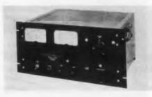
Supplying up to 36 v dc and 15 amp at any voltage, model H3615 transistorized power supply has a combined line and load regulation of less than 0.5 per cent for changes of load from 0-15 amp and for line changes from 105-125 v. Output ripple is 3 mv over most of the range. The instrument measures 8-3/4 x 19 x 14 in. and weighs approximately 50 lb.
