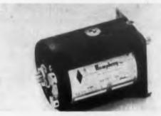
Since this rate switch is externally adjustable, it is possible to stock units and set them for the desired rate as projects require them. Typical ranges supplied are 1 to 10 deg per sec, 5 to 50 deg per sec, and 10 to 500 deg per sec. Model no. RSO3-0101-1, now in production, has a rate range from 10 to 200 deg per sec, and a natural frequency greater than 30 cps.
