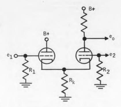
Fig. 10. Cathode-coupled subtracting circuit—a variation of Fig. 8.
