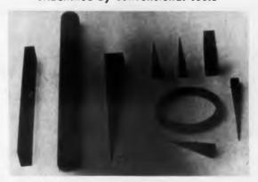
Called Radite 75, this microwave absorbent material is obtainable in standard rod form or to specially molded shapes. Intended primarily for use is microwave circuitry, the material is rigid, moisture repellent and is worked with conventional machine tools. Applications include waveguide and coaxial matched terminations, spurious mode absorbers, microwave attenuators, and others.
