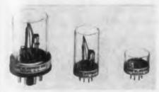
Due to its low mass, the thermaline thermal time delay relay offers delays as low as 250 msec. The 1/8 in. diam silver contacts can carry 3 amp at 115 v 60 cps noninducting current, for a minimum of 250,000 operations. Operating voltages range from 6-115 v. Timing ranges, normally open or normally closed as 250 msec to 3 min. Contact recovery time is 2 sec max, timing tolerance for any range is ±10 per cent of total time. Available in glass or metal enclosures.
