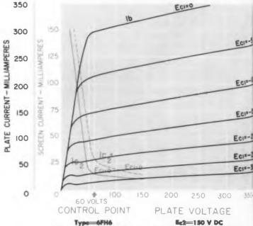
Avg. Plate Characteristics Ef—Rated Voltage Ec2=150 V DC
