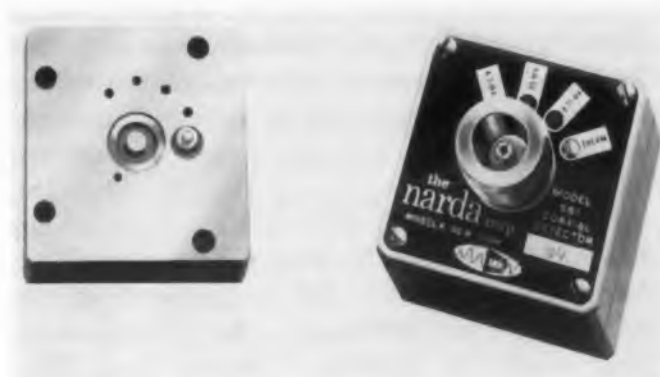
Fig. 7. Photograph of coaxial mount opened to replace the element. It can be used with disc bolometer elements.
