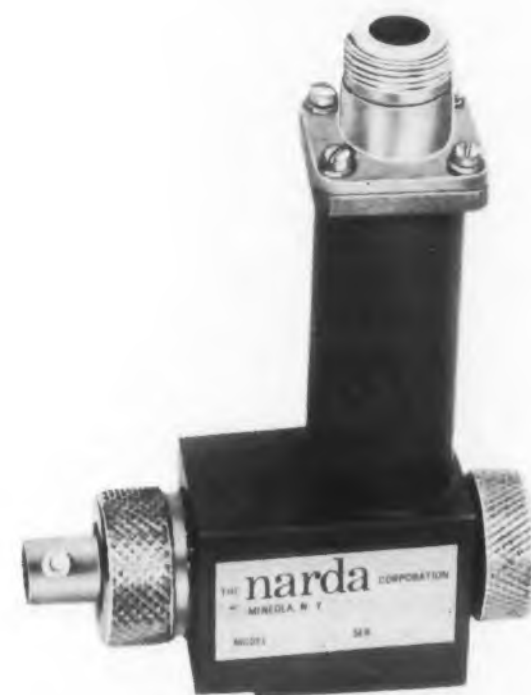
Fig. 8. Coaxial thermistor mount using two replaceable cartridge thermistor elements. Blocking capacitors are built into the mount.
