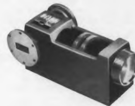
1. FREQUENCY METER. Frequency range 8.2 to 12.4 kmc. Reaction type. Waveguide size 1 x 1/2". Accuracy ±0.08%. Seven models covering the frequency range from 3.95 to 40 KMC. (Model 535 is illustrated.)
