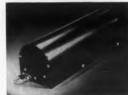
Type 39803 solenoid was designed to produce a flux of 600 gauss for focusing traveling wave tubes. The solenoid proper is 7-1/2 in. long and has a circular opening of 1-1/2 in. Weighing 13 lbs, it produces full flux field with an input power of 100 to 125 w. A small built-in blower keeps the temperature rise to 65 C.
