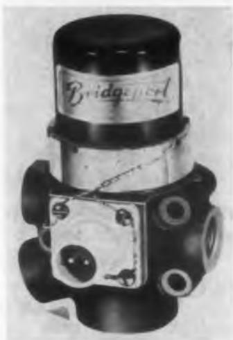
Containing a captive seal, this three-way solenoid-operated valve weighs 0.77 lb. It can handle pressures of over 3000 psi and withstands more than 350 F.
