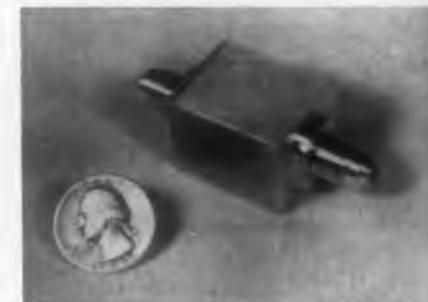
Series 1000 pressure transducers occupy one cubic in. of space and are available with an output signal which varies linearly or non-linearly with pressures over ranges of from 0-10 to 0-50 psi. The units use a precision carbon film resistance element requiring minimum brush pressure. Resistance values range up to 10,000 ohm. Best linearity is 0.4 per cent.
