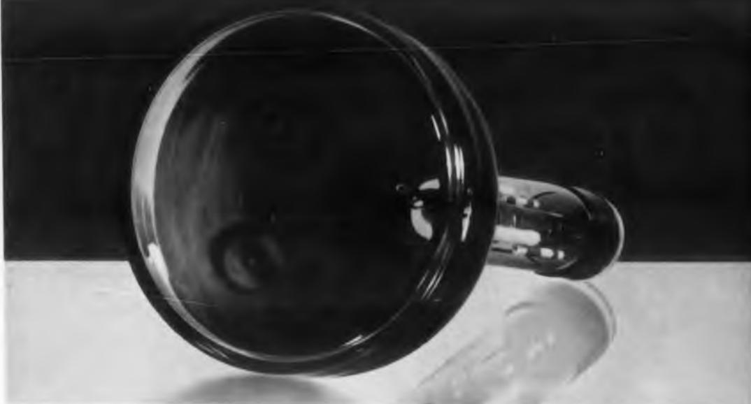
New five-inch experimental evaporated phosphor CRT
