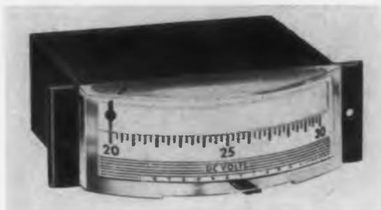
Expanded scale dc voltmeters can be supplied in the model 1135 and 1145 side indicator panel meters. The 1135 has a scale length of 2.1 in. and a panel area of 2 sq in. Scale length of the 1145 is 2.7 in., and panel area is 5.5 sq in. Voltage ranges lie between 4 and 265 v dc, and accuracy is  $\pm 2$  per cent of full scale.
