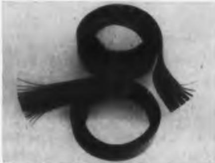
Insulated with Teflon resin applied in thicknesses of 0.003 to over 0.030 in., Multi-Tet cable ribbons come in wire sizes from AWG 12 to 34. A single ribbon can have up to 100 conductors.
