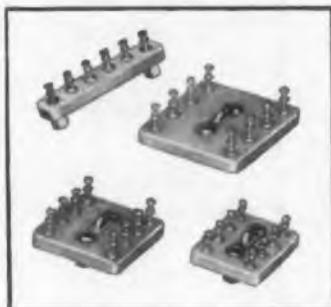
Cambion<sup>®</sup> grade L-5 silicone-impregnated ceramic terminal boards are completely unaffected by moisture, heat, and humidity. The brass terminals are silver-plated, the brass internally-threaded mounting studs are cadmium-plated — making for 100 percent protection. These
