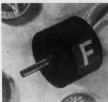
The Type 11 potentiometer has a starting torque of 0.5 gm cm. As part of the manufacturer's range of precision potentiometers, it is designed to provide analog conversion from mechanical rotation to an electrical signal. Linear and sine/cosine laws are available and other non-linear functions can be manufactured. Potentiometer has good resolution and linearity. They are capable of reliable operation under severe shock.
