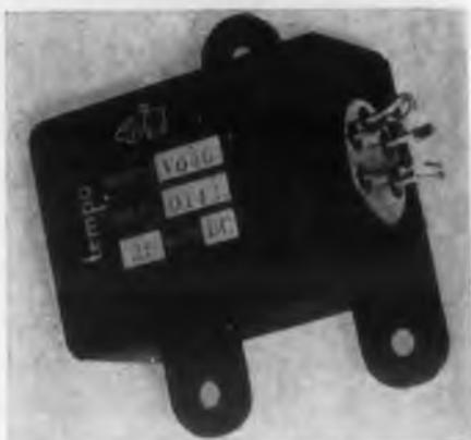
Design and performance details of these transistorized time delay relays include: time delay periods from 0.01 to 60 sec; timing accuracy of  $\pm 10$  per cent of nominal delay period; and contact arrangements and ratings of either 1-pole, double throw, 10 amp resistive or 3-pole, double throw, 10 amp resistive.
