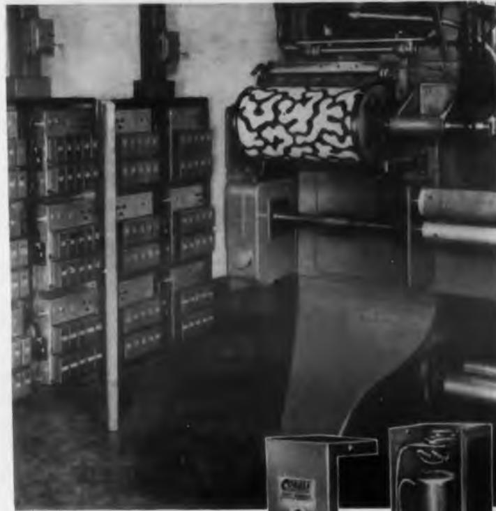
Electrical contact fingers transmit impulses to 120 CLARE RELAYS each housed in a modular type unit.
