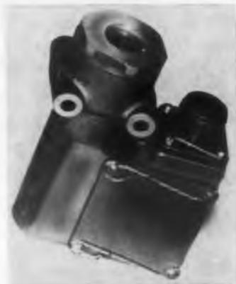
An intermediate mechanical snap action in the 90000 series pressure switch insures trigger switching of the electrical switch element and prevents welding of contacts. For use with hydraulic fluids or compressed air, the unit comes in pressure settings from 5 to 4000 psi.
