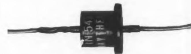
Fig. 5. Diodes like this one have piv's to 1000 v.
