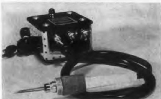
Designed for production soldering, this dual metal tip soldering tool incorporates the advantages of resistance soldering without requiring a grounding circuit. The tool is especially designed for soldering miniature connectors.
