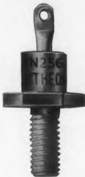
Fig. 6. Stud mounted diodes can carry more than 5 amperes.
