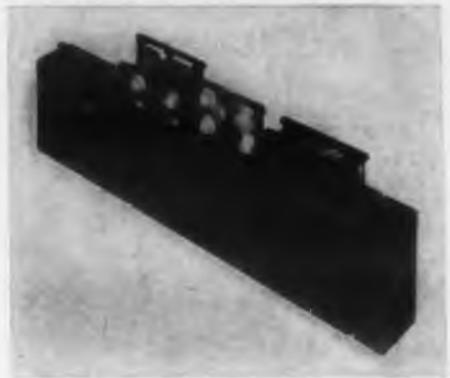
Designed for use in airborne data acquisition systems, the Minidrive provides for 14 channels of pulse data recording on magnetic tape. The unit will present the parallel output code of the company's Minidatrac to tape heads, and will also provide odd-even parity checking and gates which will allow the recording of additional information, such as block counter pulses and other auxiliary inputs.
