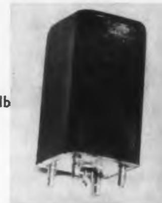
In these encapsulated, hermetically sealed twin-T filters, precision resistors and temperature compensating capacitors maintain attenuation over a wide temperature range. Null attenuation is 60 db or better. A range of null frequencies and impedance levels are available.
