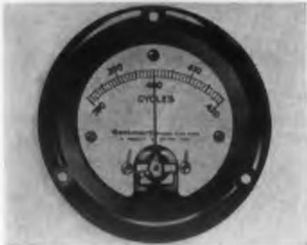
A self-contained, needle-indicator type unit for panel mounting, this 400 cps expanded scale frequency meter has a standard 380 to 420 cps scale readable to accuracies of 0.25 per cent over its full range. Between 380 and 420 cps the bridge used in the meter provides an output linearly proportional to input frequency.
