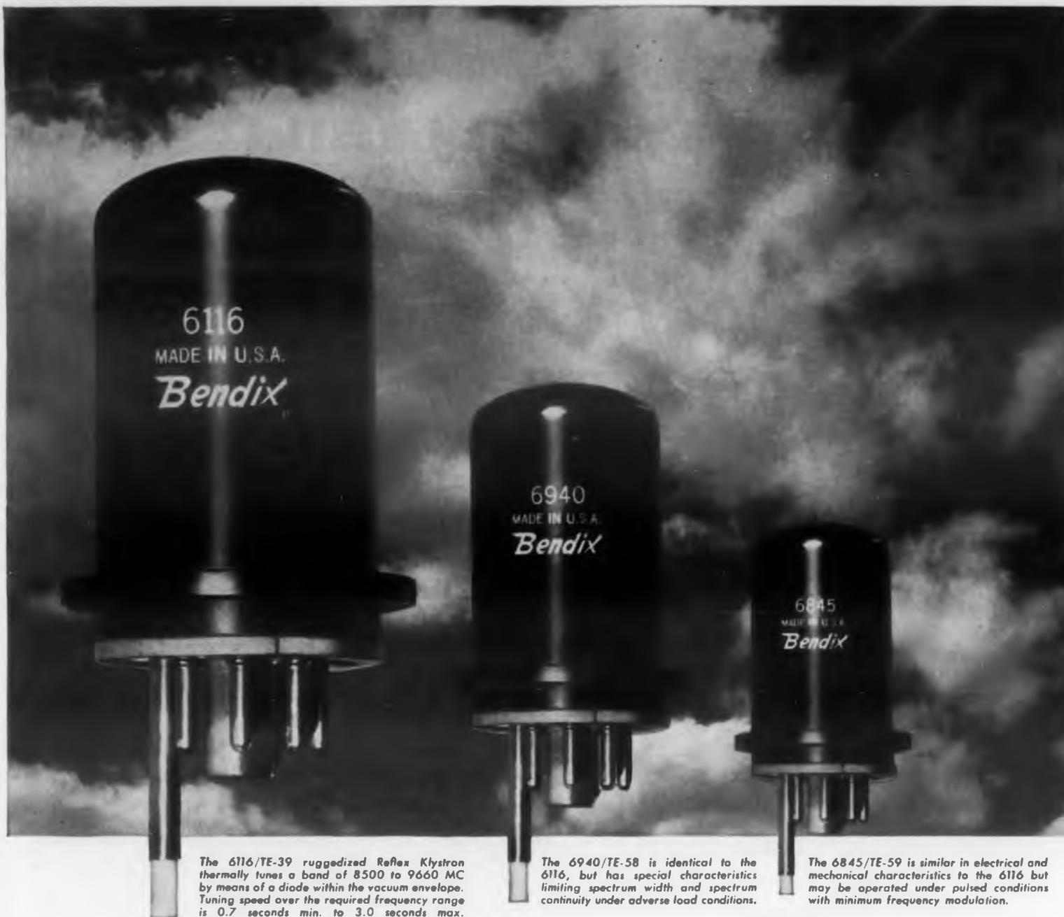
The 6116/TE-39 ruggedized Reflex Klystron thermally tunes a band of 8500 to 9660 MC by means of a diode within the vacuum envelope. Tuning speed over the required frequency range is 0.7 seconds min. to 3.0 seconds max.
