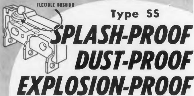
A flexible bushing compressed around the pin actuator combines with bonding of the case halves to provide a splash-proof, dust-proof, explosion-proof (MIL-E-5272) switch with improved reliability. Ideal for use in miniaturized electronic and electrical apparatus.
