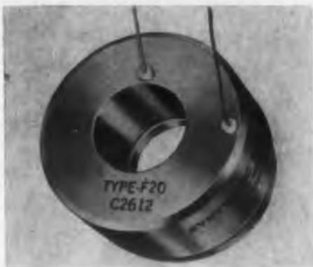
Type F20 electromagnetic focus coil is designed for photographic, flying spot, military and other special purpose tubes requiring short focal lengths at up to 25 kv accelerating potential without overheating. Minimum spot distortion is achieved by machining coil case to close dimensional tolerances. Sharp focus for high beam currents is assured by a large id to focus gap ratio.
