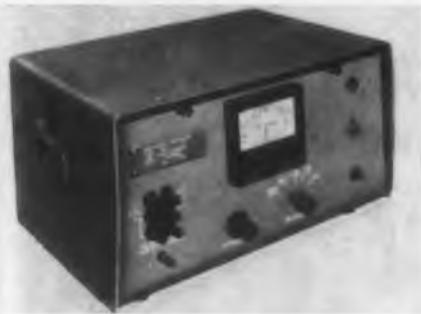
Model 343 impedance comparator features high stability. The equipment gives accuracy of 0.05 per cent over wide range of impedances from 10 ohm to 15 meg without adjustment.
