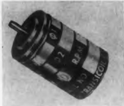
Weighing 0.9 oz, this size 6 servo motor will develop a stall torque of 0.125 oz-in., and has a free speed of 6200 rpm. The unit is available for 400 cps operation with 26, 33, or 52 v control phase windings. The control phase is center-tapped for operation directly with transistor amplifiers. Operating temperature range is from  $-55$  to  $+120$  C.
