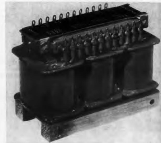
**High-temperature transformer** announced by Gresham Ltd. for airborne applications operates at 130 to 150 C.
