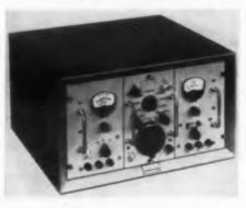
Model 82 signal generator series have power supply and five plug-in rf oscillators with frequency ranges between 20 to 80 mc and 2700 to 3000 mc. Units have 1000 to 2000 v dc continuously variable power supply.
