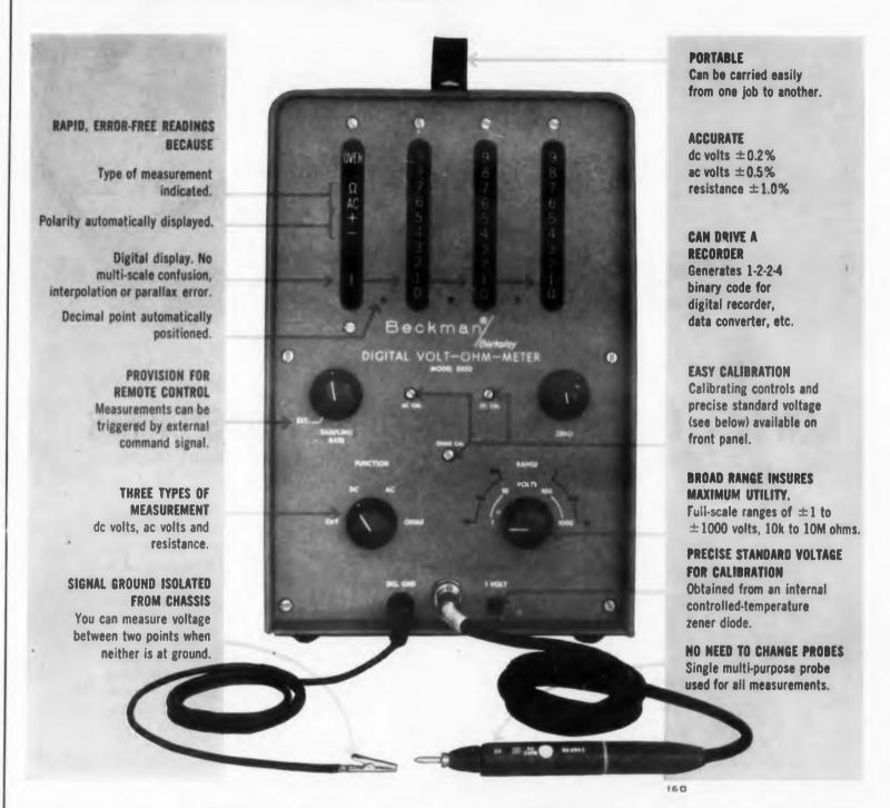
As the picture reveals, BECKMAN/Berkeley's Model 5350 is the most useful, most versatile digital instrument of its kind. It offers operating flexibility and features not found in digital voltmeters costing three times as much. The Model 5350 makes it feasible to replace multipurpose analog equipment with a more accurate, rapid and foolproof means of making the vast majority of everyday voltage and resistance readings.
