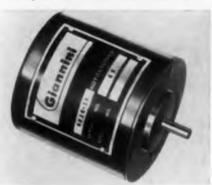
The model 8915 stepping motor provides controlled CW or CCW shaft rotations in 2 deg increments. Stepping output is as rapid as 60 steps per sec, unlimited in either direction, and torque is provided as high as 14 oz-in. The input power requirement of 1 amp at 28 v can be applied for as little as 10 msec per step of output.
