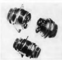
This push-pull, quick disconnect environmental connector utilizes six coaxial contacts. Pins or sockets are available in either the plug or the receptacle, and coax contacts will accept RG-196/U cable.
