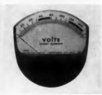
An anti-parallax scale for use with model MM-3 3-1/2 in. meters places dial markings in the same plane as the pointer. The pointer swings under the raised scale.
