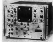
Model LA 260 provides plug-in single or dual trace vertical preamplifier design. Frequency response is flat from dc up to 15 mc, and useable beyond 30 mc.
