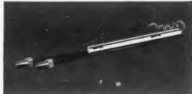
THE TRAVELING-WAVE AMPLIFIER TUBE, also available from Bendix Red Bank, is designed for operation in the 4.0 to 8.0 kmc frequency range with approximately 40 db gain and 200 milliwatts output power. The tube utilizes a helical slow-wave structure with coupled helix attenuator section. The mechanical design minimizes the effects of vibration upon the tube operation.
