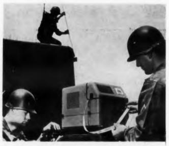
Super-speed printing reperforator which prints out messages at 750 words per minute will play a part in tomorrow's tactical communication system.
