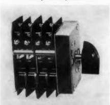
Millions of operating sequences are available with series 20AS rotary selector switches. The assemblies are available with 4, 6, 8, 10, 12, 14, 16, 18, or 20 spdt basic switching units. Electrical rating is 10 amp, 125, 250, or 460 v ac; 0.5 amp, 125 v de: 0.25 amp, 250 v de.
