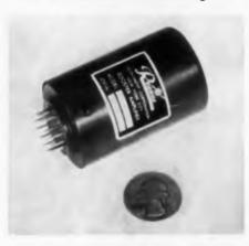
For resolver systems, this dual transistorized booster amplifier has an input impedance of over 5 megohms and a feedback gain of 60 db minimum. It maintains zero phase shift and a constant transformation ratio of unity from -65 to +85 C. Each amplifier section is individually encapsulated.
