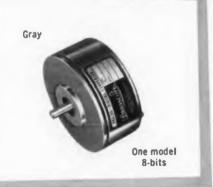
Features of Librascope Shaft Position-to-Digital Converters include serial/parallel time sharing, double brush pick-offs, no dead time, variety of codes, digital-analog and analog-digital conversions. They are designed for the transfer of data from a shaft position to a form suitable for digital computers or data logging systems. Special converters are designed to meet customer requirements (including Sine Cosine). Please submit desired characteristics. Features of Librascope Shaft Posi-
