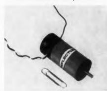
This line of dc permanent magnet motors features reduction in length and bulk, ceramic magnetics, and efficiencies as high as 45 per cent. The Index I field structure is enclosed within a steel shell, providing complete self-shielding. The assembly can be mounted or dismounted without affecting its magnetic characteristics. Stock models can be obtained varying from a 4 to 30 v dc input range.
