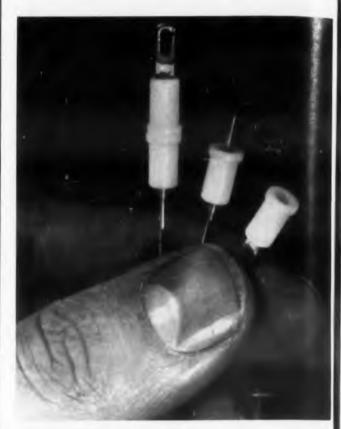
Tetrafluorethylene fluorocarbon resin, duPont's Teflon, has application in miniature electrical connectors. Made by Sealectro Corp., these units will withstand temperatures up to 550 F.
