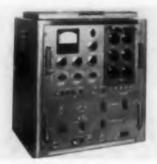
Model 5002AB diode test set automatically compares the dc forward and reverse characters of semiconductor diodes against preset limits and gives the results in go-no-go form.
