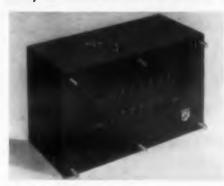
The 145 to 1 delay to rise time ratio of these extended bandwidth lumped-constant delay lines permits the design of delay line memories with 72 bit storage capacity. Temperature coefficient of delay is less than 65 ppm per deg C.
