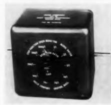
This series of in-line shaft speed reductors is available with exactly repeatable ratios up to 1000 to 1. They are remommended for continuous duty up to 1500 rpm, intermittent to 3000 rpm, with output torque capacity to 50 oz-in.
