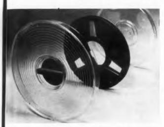
High heat styrene gives color, finish, and excellent imensional stability to these IBM magnetic tape reels. Container material is clear styrene; knob is topolymer styrene. Great cost reductions were rehieved using this material over the former metal parts.
