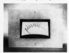
These meters meet American Standard C16.5-1954, but occupy at least 15 per cent less panel space than comparable units. They have a response time for a step change of  $0.3 \, \text{sec}$ ,  $\pm 10 \, \text{per cent}$ . Overshoot is 1 to 1.5 per cent.
