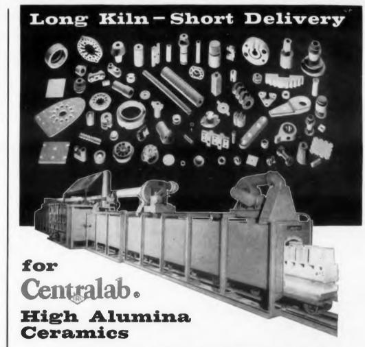
Fast delivery of 95% and 85% High Alumina, to your most critical specifications, is assured by Centralab's new 80 foot continuous kiln. First of its design in the United States, this new kiln is capable of producing 21 tons of exceptional quality High Alumina every month. Consistent reproduction of electrical and physical properties from batch to batch is guaranteed.
