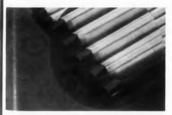
Polyethylene resin extruded, is used in the tubes of this Exide battery. Using duPont's Alathon, Exide engineers expect a 20 per cent increase in life over former batteries using rubber tubes. Alathon doesn't corrode and maintains its strength and flexibility under low temperatures.
