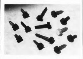
Nylon head self-tapping screws are used in portable TV receivers to avoid having a metal contact on the outside of the case. Made by Gries Reproducer Corp., the self-insulating fasteners can be used in high-voltage equipment. Dielectric strength (short time) is 385 volts per mil.
