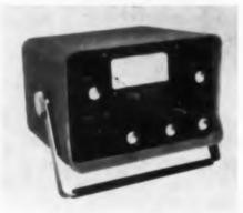
The SIE Model R-3 voltmeter measures ac voltages from 1 mv to 1000 v full scale, positive and negative dc voltages from 1 v to 1000 v full scale, and half-scale resistance readings from 10 6hms to 10 meg at an over-all 3 per cent accuracy on all readings. It also has an electrometer input for measuring 0 to 1 v dc at an impedance greater than 10,000 meg.
