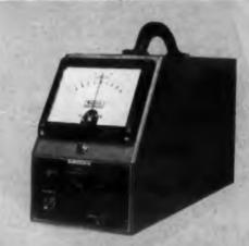
ELECTRONIK null indicator is completely electronic with chapper input. Highly sensitive, fast reading, vibration resistant. No damping resistance is required. Large, clearly legible dial. Ruggedly built. Price: \$175. Write for Data Sheet 10.0-12a
