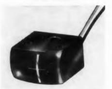
The dc erase head provides 50 db erasure with 5.5 ma of current through the coil. This head is currently manufactured in a 20-mil track width configuration.
