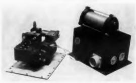
Model E/AP-150, type 205, provides pressurization and circulation of dehydrated air to the waveguide radar system for missile control. Weighing 8 lb, it has a delivery of 160 cu in. per min. An operating switch maintains a pressure of 17 psig.
