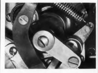
Phenolic, nylon filled, was found by IBM to possess the high strength and dimensional stability necessary for service as a high-speed cam. About 1 in. in diameter, the cam is subject to extremely high pressure. It is molded, not machined, for use in IBM's 24 and 56 punched-card accounting machines.
