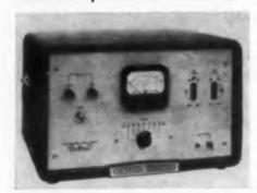
The model 434A calorimetric power meter measures power from 10 mw to 10 w, full scale, and at any frequency from dc to 10 kmc. Power is read directly in watts and DBW. The unit has a response time of less than 5 sec on all ranges, and its accuracy is  $\pm 5$  per cent or better.
