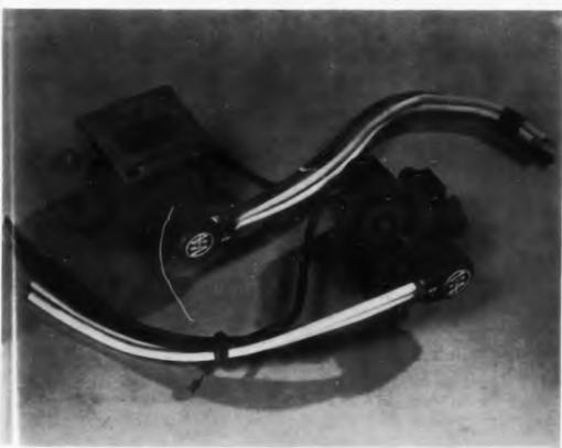
Fig. 4. Klystrons operate better at high altitudes when equipped with Silastic insulated high voltage terminals and leads.
