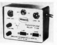
Model T-681 transistorized relay for use with thermoregulators and other units requiring microampere operation. Using 110 to 120 v ac power, it provides a 5 µa activating current through the thermostat or other sensing element and controls a load up to 1500 w.
