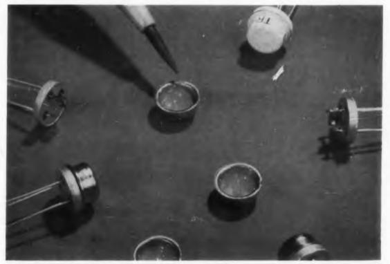
Fig. 1. High dissipation ratings are obtained by filling transistors with electrical grade silicone compounds.
