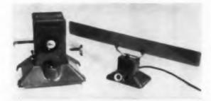
X band microwave wattmeter Type U-182 is intended to replace the water calorimeter. Makes possible rapid production checks on magnetrons, klystrons; has in-line wattmeter for radar. Measurements can be made in 10 to 200 w power range with 2 per cent accuracy.
