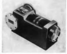
These direct-reading, TE<sub>111</sub> mode frequency meters cover a full waveguide band in the frequency range from 3.95 to 40 kmc. Designated types 532 through 538F1, the meters have a direct-reading accuracy of 0.08 per cent for most
