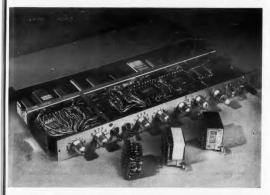
Fig. 3. Protection of electronic subassemblies from shock and extreme moisture is assured by potting with room temperature vulcanizing silicone rubber.
