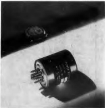
Power supply which occupies 5 cu. in. and supplies 60 ma at 300 v dc from a 115 v, 400 cps ac input source. Ripple is less than 5 per cent at full output rating. Qualified per MIL-T-5422C.
