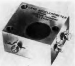
Three mutually perpendicular sensing elements are mounted in these small accelerometers. The units have 25 kc frequencies and 5 to 9 mv per g sensitivities. Model 2230 operates to 200 F; model 2243 to 500 F.
