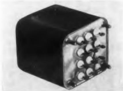
These 400 cps transformers are hermetically sealed and meet MIL-T-27A, Grade 4, Class S specifications. They operate at 85 C ambient, 45 C rise. Maximum operating altitude is 70,000 ft and life expectancy is 10,000 hr. Included in the line are 10 power transformers with high voltage secondaries ranging from 40 to 300 dc ma and multiple filament secondaries ranging from 3 to 20 amp. All units have 2500 v rms insulation.
