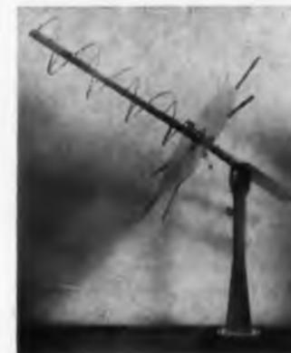
Model MAM-1000 telemetry antenna is for use where the antenna can be manually oriented. It also comes with a remote controlled motor-driven mount. Unit pictured is a 4-turn helical beam antenna with a 50 deg acceptance angle and a 10 db gain over an isotropic source.
