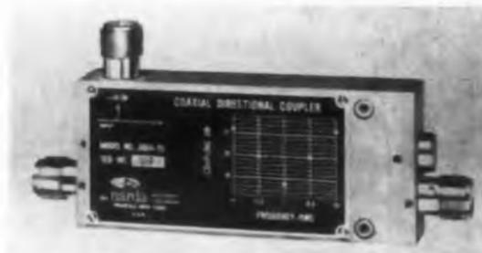
The couplers cover a 2-1/2 to 1 freq. range with flat coupling and high directivity from 4000 to 10,000 mc. Units include chart providing calibration to 0.2 db accuracy at 5 freq.
