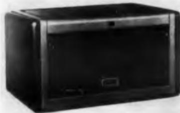
Providing a static nulling error of 0.02 per cent, the DLI-101 servo multiplier has two channels, each of which multiply three variables by a fourth. Its automatic gain control feature maintains constant loop gain for reference voltage variation in the 2 to 100 v range. The unit is composed of Digitrol plug-in building blocks.
