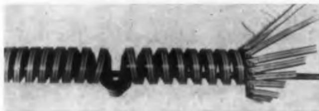
The winding direction is reversed in the middle of this multiconductor retractable cable. When the cable is extended, the twisting forces are transmitted to the reverse point, and there is no strain on the wires where they terminate. A few ounces will extend a cable of 100 wires.
