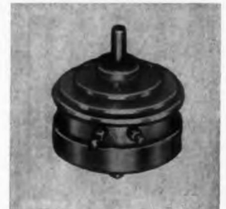
Half as long as its mounting diameter, the model PC-8 precision clutch has encapsulated coils, fixed terminals, 1,000 servo mounting diameter, and guaranteed torque of 16 oz in.
