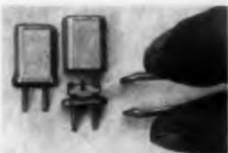
For operation from 300 kc to 125 mc, this miniature crystal is packaged in an HC 18/u case. The crystal wafer is suspended between the two terminals.
