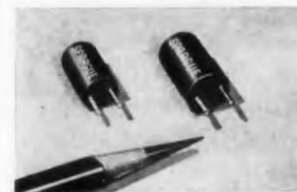
Type 89D Verti-lytic capacitors are plastic-encased electrolytics for stand-up mounting on printed wiring boards. Terminals are easily identified by the larger size of the negative terminal. Standard ratings range from 1 to 290  $\mu$ f at 3 v dc to 1 to 25  $\mu$ f at 50 v dc.
