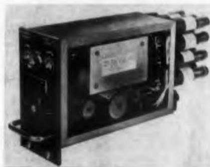
The Model 605C start-stop regenerative repeater is designed for use on telecommunication circuits where it reshapes and retimes distorted incoming signals. All components are packaged as plug-in subassemblies. A plug-in speed tuning network is furnished for 60, 75, or 100 wpm operation.
