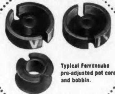
Typical Ferroxcube pre-adjusted pot core and bobbin.
