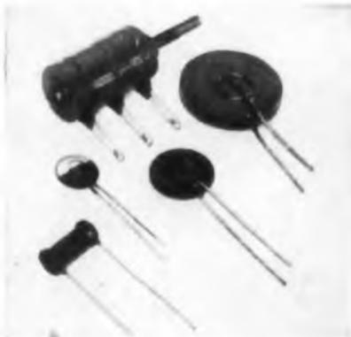
GLOBAL Type BNR varistors are non-linear (voltage-sensitive) resistors for voltage control and stabilization applications. They are made from the highest electrical grade silicon carbide, ceramically bonded into disc, rod and cylindrical shapes. Flexible production facilities make possible a wide range of physical sizes, watt ratings and changes of resistance with applied voltage. For details, write for Bulletin GR-2.
