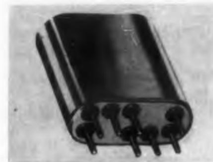
This relay utilizes a novel contact configuration for maximum over travel and a large degree of wipe. Type BR8 exceeds applicable military specifications for miniature relays: 30 g, 10-2000 cps. operate and release less than 5 msec, with pull-in power 200 mw for dpdt and 80 mw for spdt relays.
