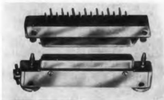
The UPCC-ML series printed circuit connectors have straight-through terminals on the male member. Terminals are solder dip for 1/16, 1/8, or 1/4 in. boards, or solder eyelet or turret type. Insulation resistance is over 5000 meg, with voltage breakdown over 2500 v ac rms, and current rating 7.5 amp. With 7, 11, 15, 19, and 23 terminals.
