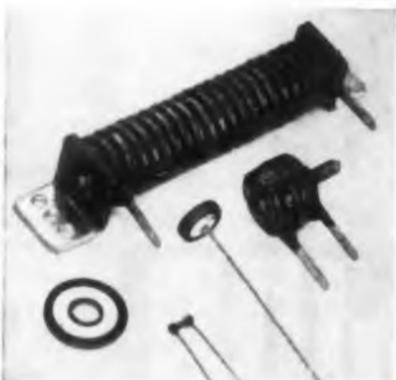
GLOBAL Types B, F and H thermistors are non-linear, negative temperature coefficient resistors, available with coefficients from approximately .3% to 5.1% at 25°C. Disc and rod shape bodies may be manufactured in a wide range of sizes to provide desired resistance values, thermal time and dissipation constants and temperature coefficients for a variety of electronic circuits. For details, ask for Bulletin GR-3.
