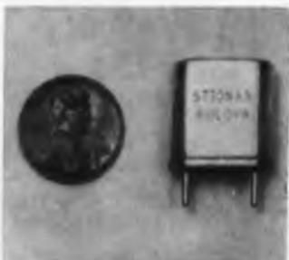
Series ST-70NXS low frequency crystals cover a frequency range of 100 to 250 kc with a frequency tolerance of  $\pm 0.015$  per cent from  $-55$  to  $+90$  C. They stand 100 g initial shocks and 20 g vibration up to 2000 cps.
