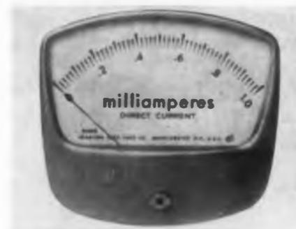
Panel meter MM-5 occupies panel space of conventional 4-5/8 in. meters and mounting space of ASA/MIL 3-1/2 in. units, yet provides greater scale length and readability. Tracking can be held to 0.5 per cent of full scale, when plotted linearly or with a protractor reference for deflection angles up to 100 deg.
