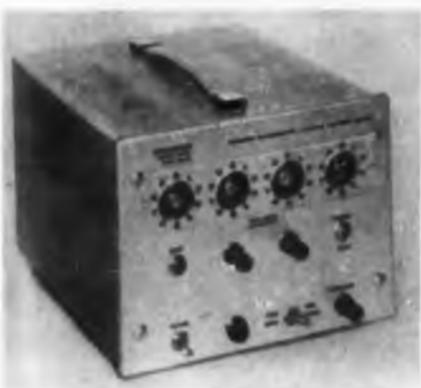
For measuring time intervals between opening and closing of contacts on almost any instrument or control, the Dynatimer electronic stopwatch has  $\pm 1$  msec accuracy. Contact time intervals range from 2 msec to 10 sec. The unit comes with glow counter tube or Nixie readout.
