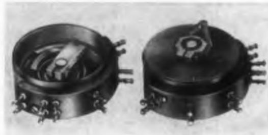
Model 200-CEUS 2 in. precision potentiometer may have up to 13 preset taps or it can be tapped in the field by the user. Spacing of terminals facilitates direct attachment of padding resistors to produce nonlinear functions; nonlinear units can be wound to any specified function. All nonferrous parts are anodized or plated. Up to 15 units can be stacked without loss of accuracy.
