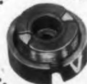
Bobbin, wound with specified number of turns of wire for desired inductance, placed in pot core.
