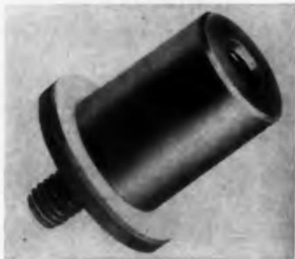
Insulator mounts, rated up to 4000 v, are designed for high altitude operation and efficient heat transfer to chassis or ground. In over-all thermal drop, the mounts are rated better than 1 deg C per watt.
