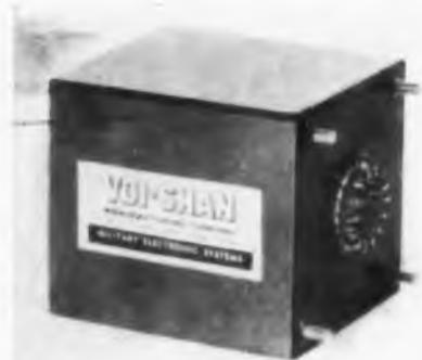
This time delay relay is a 6pdt, 5 amp type with delays from 60 msec to 600 sec. Either delay-on-make or delay-on-break configurations are available. Accuracy from  $-62$  to  $+72$  C at constant 28 v dc is  $\pm 4$  per cent. Shock, acceleration, and vibration meet MIL-E-4970.
