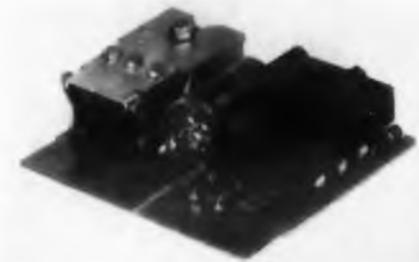
A self-contained unit with power relay, thyatron amplifier, and power supply, this sensitive miniature relay control requires 1/4 μw for switching. The unit contains printed circuitry and has an edge-type plug-in arrangement. It mounts vertically or horizontally. Output, one to three poles, is 5 amp each at 250 v ac.
