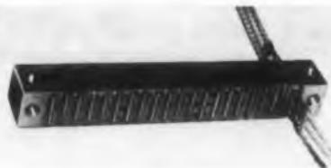
In 1, 2, and 3, row units, these solderless terminal blocks accept standard AMP 53 taper pins. With internal buss connections to eliminate external wiring, units come in any combination of feed-through individual or shorting terminals.
