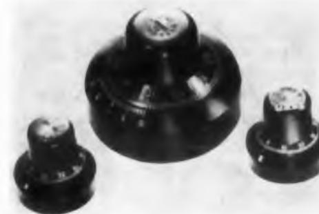
Used with ten turn potentiometers, these Migit-Mite counting dials have sealed unit construction. Numerals are held in place until completion of the next full rotation of the dial. The dials provide continuous operation in either direction, and come in sizes up to 2 in. OD.
