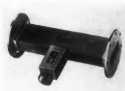
Frequency ranges of these direct reading microwave attenuators are from 2.6 to 3.95 kmc to 12.4 to 18 kmc. Units in each range have 20 or 40 db maximum attenuation. They have a maximum vswr of 1.15 and feature accurate attenuation settings.
