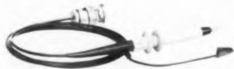
**-hp- AC-21C Voltage Divider Probe.** 50:1 divider with 10 megohm input impedance and 2.5  $\mu$ mf capacitance. For *-hp-* 150A but usable with most scopes, VTVM's, preamps. \$25.
