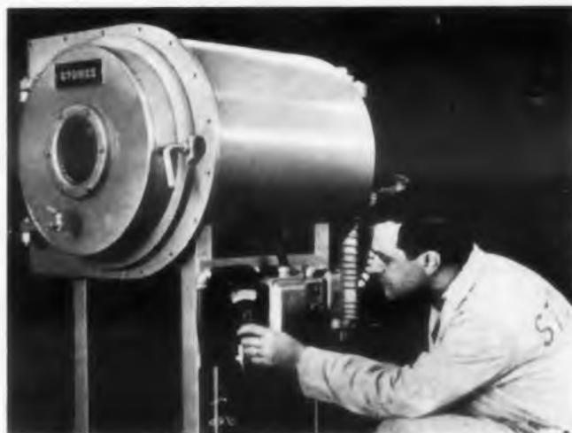
Semiconductor components can be outgassed and brazed or fused under closely controlled vacuum conditions in this oven. The vacuum baking oven has its own vacuum pumping system, heating equipment, and temperature regulating and indicating instrumentation. The vacuum chamber can be evacuated to a pressure of  $10^{-6}$  mm and heated to approximately 450 C. Upon completion of the bake, vacuum is broken to the inert-gas atmosphere of the dry-box.
