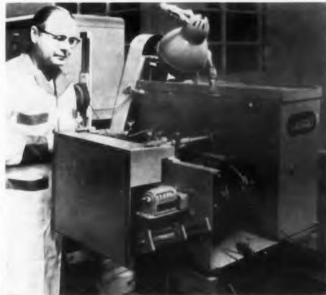
All automatic, from unreeling insulated wire to stacking pieces in a trough, the Acme wire cutter and stripper processes over 9000 pieces an hour in 1 to 40 in. wire lengths. Rate for 80 to 120 in. lengths is 3000 pieces per hour. The machine handles stranded wires up to 10 gauge and solid wires to 12 gauge.
