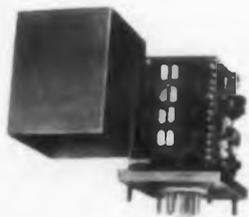
Frequency stability of the TCO 300-OC transistorized crystal oscillator is  $\pm 0.002$  per cent from  $-55$  to  $+85$  C. The unit has oven control and square-wave type output. It stands 100 g shock and 10 g vibration to 2000 cps.
