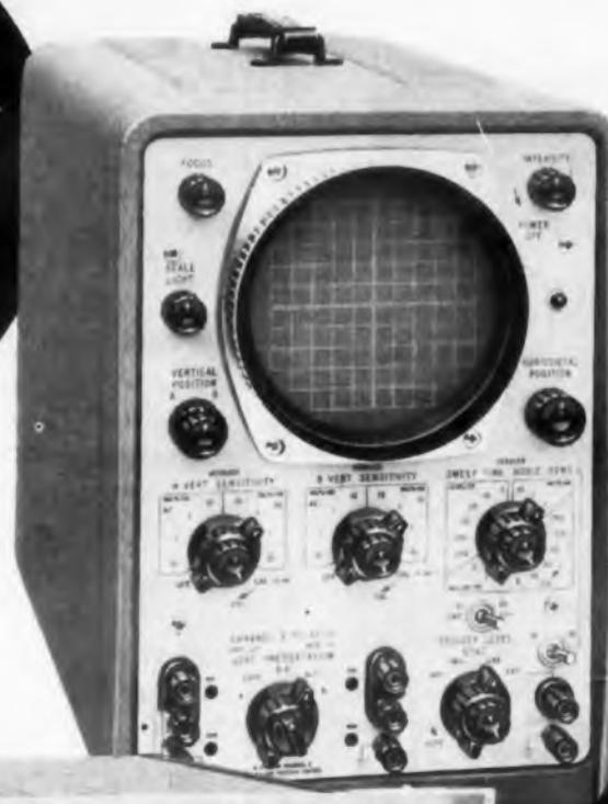
New 122A uses alternate sweep or 40 KC chopper for dual trace display
