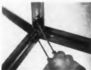
Locking connector and extrusions
