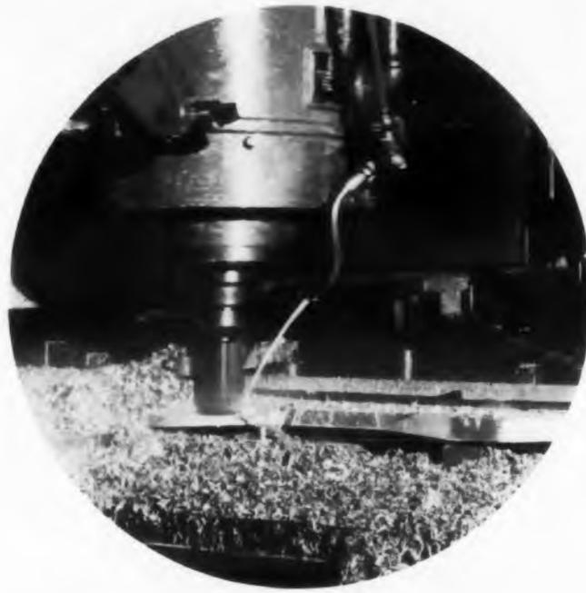
**The business end** of a giant tracer-controlled profile milling machine. Electronic controls are by GE's Specialty Control Dept.
