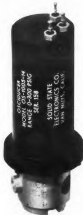
Pressure-to-frequency converter OS-1000 can be used in missile, aircraft, and industrial telemetry. The unit combines a variable inductance diaphragm type transducer and a temperature stabilized transistor oscillator. It needs three connections: 28 v dc at 2 ma, ground, and output. For all IRIG channels, units are diaphragm and flush-type with ranges from 5 to 5000 psi differential, absolute, or gage.
