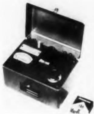
The MV-1 potentiometer section has two voltage ranges: 0 to 60 mv and also 95 to 105 mv. Its ammeters are scaled from 0 up to 5.0 ma dc.
