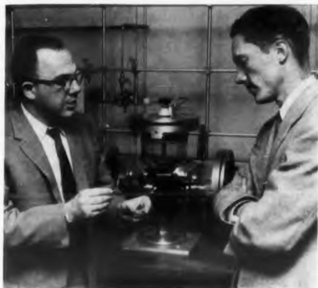
Experimental sputtering apparatus which laid down resistor film under inspection.
