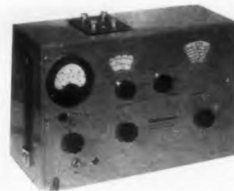
For use at frequencies between 100 kc and 100 mc. Oscillator is modulated at 60 cps 50 per cent, so that dc amplifiers need not be used in the voltmeter.
