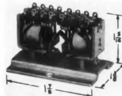
A 1.5 w pulse for 10 msec transfers the contacts in the KE series miniature relay. The 6pdt dc unit operates under 30 g shocks and 10 g vibration at 55 cps. Contact rating is 2 amp, 115 v, 60 cps for resistive loads.
