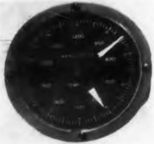
To obtain high readability and accuracy, this miniature null-balance potentiometer indicator utilizes an accumulative reading. Supplied with a remotely mounted servo amplifier, the unit has 0.25 per cent accuracy and 0.1 per cent sensitivity.
