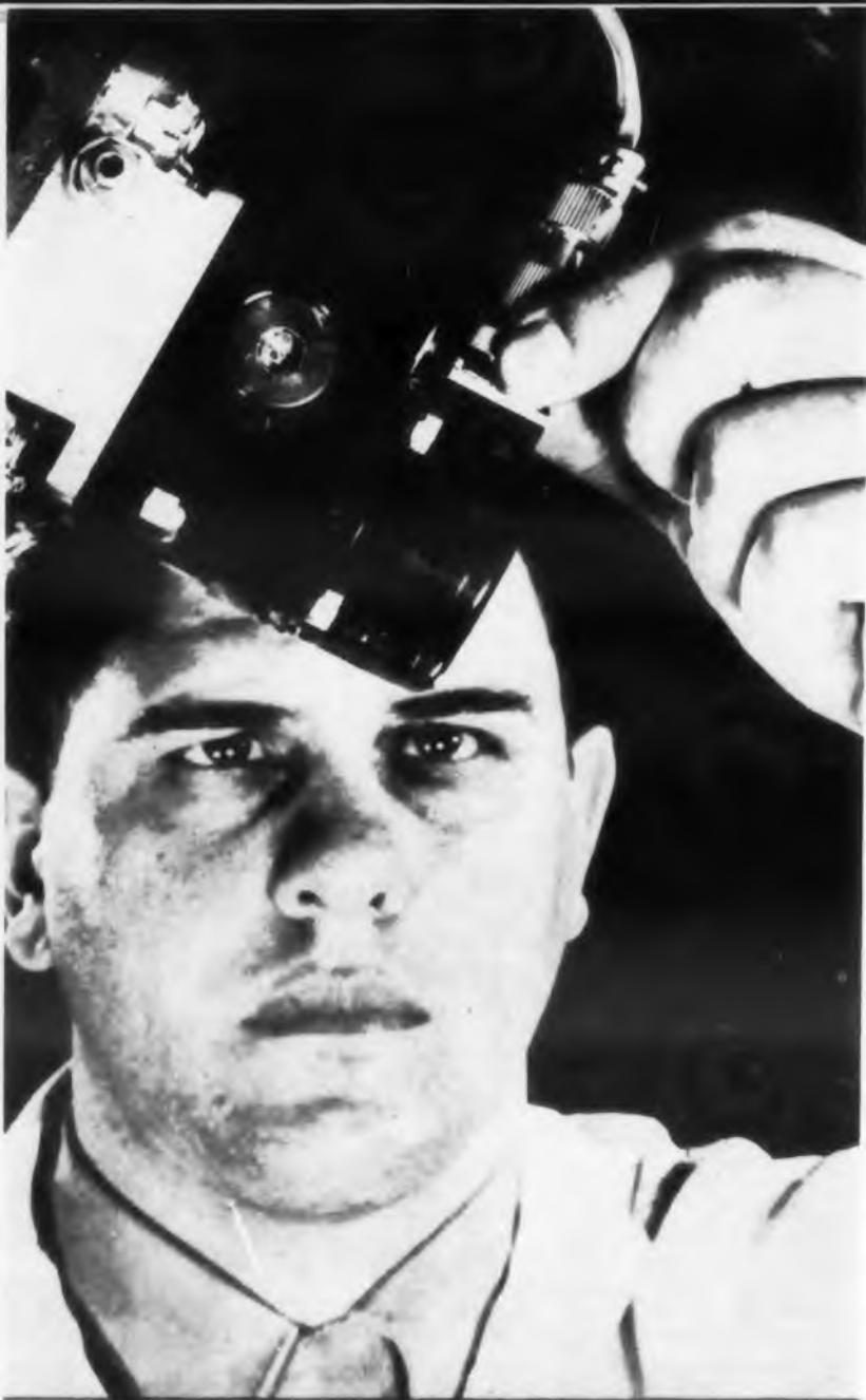
Hydraulic servo on Bendix punched tape controlled milling machine.
