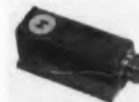
Effects of humidity and rf radiation are eliminated in these self amplifying accelerometer systems Designated 2806-2807 and 2808-2809, the systems combine two units, one for vertical, one for horizontal vibration measurement. Sensitivity up to 300 mv per g is preset to user specifications. First accelerometer resonances are above 35 kc with frequency range  $\pm 5$  per cent from 10 cps to 2 kc.
