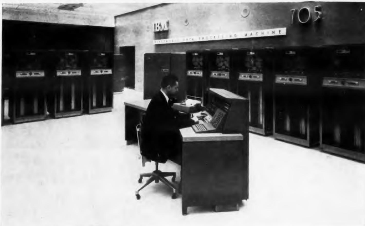
**KEEPING "ELECTRONIC BRAINS" FROM LOSS OF MEMORY.** One of science's greater marvels is IBM's 705 Electronic Data Processing Machine—which makes intricate calculations and logical decisions in millionths of a second. Heart of this electronic "wizard" is its main magnetic core memory. Designed for use with the machine's high-speed printer is the IBM 760 Control and
