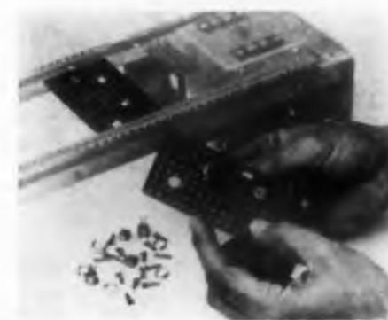
Model BP-31TR transistor mounting kit contains twenty push-in type lugs for component wiring, four no. 3304 round sockets and rings for mounting, four no. 799BC rectangular sockets and four clamps for mounting in flat position.
