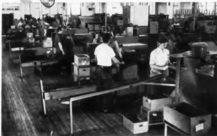
**AUTOMATIC COLOR CODING MACHINES** apply color bands and oven-bake the enamel at high temperatures to assure that the color coding will withstand the maximum operating temperatures of 150°C and all types of cleaning solvents.
