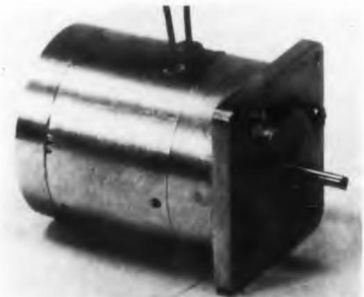
This stepper motor has a life that exceeds 24,000,000 steps. It will meet MIL specifications on vibration, temperature, shock and acceleration. The unit steps 9 times per revolution and weighs 4.5 oz. At 17.5 w input it will produce 2.5 oz in. of torque and follow a 25 cps pulse with a low torque, low inertia load. Higher pulse rates are possible if torque requirements are reduced.
