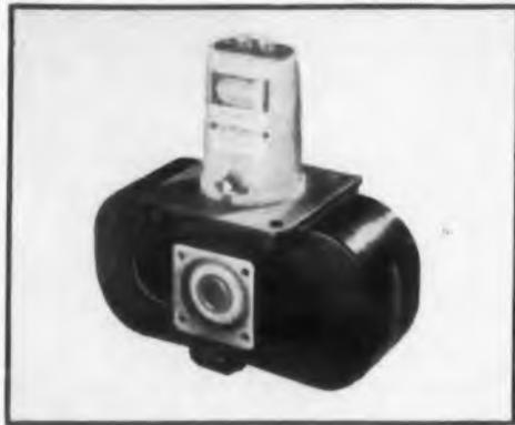
power output is 100 kw at typical pulse conditions of 0.5 μ sec. (.001 duty cycle). The tube operates at a peak anode voltage and current of 15 kv and 13.5 amp. respectively.
