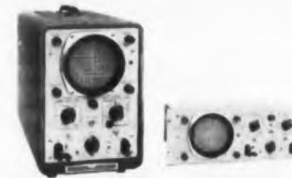
**-hp- 120A/AR, DC to 200 KC.** 15 sweep times, 1  $\mu$ sec/cm to 0.5 sec/cm. Times-5 magnifier, automatic trigger. Simple to use, rugged, outstanding value. \$435.
