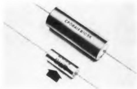
Type P1232NNG metallized-paper capacitors are rated at 50 v dc and were designed for transistor applications. The units, sealed in a metal tubular case, operate from -65 to +85 C at full voltage rating.
