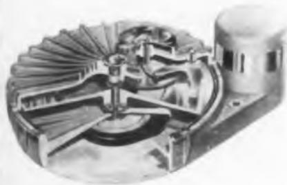
An 8-in. diameter hermetically sealed disc, this memory processor has two recording modes. One uses fixed channels for digital computation and control; the other uses a scanning head channel for data processing and correlative control.
