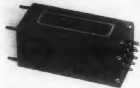
For missile and other military and industrial uses, this magnetic amplifier relay series includes three types: 15 amp RL-101 with 0.5 sec response time and 140 μw sensitivity; 2 amp RL-102 with 0.4 sec response and 40 μw sensitivity; and 2 amp RL-103 with 0.6 sec response and 80 μw sensitivity. All units are dpdt.
