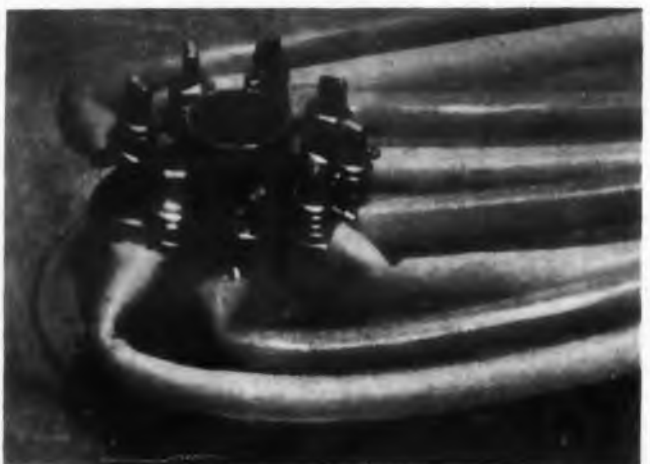
Fig. 3. Connections to subminiature button-base tube socket.
