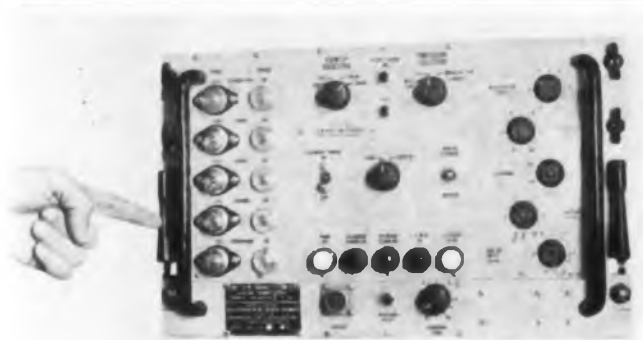
Fig. 4. Handle latch, needed on developmental models, was eliminated on production models when closer tolerances were held.
