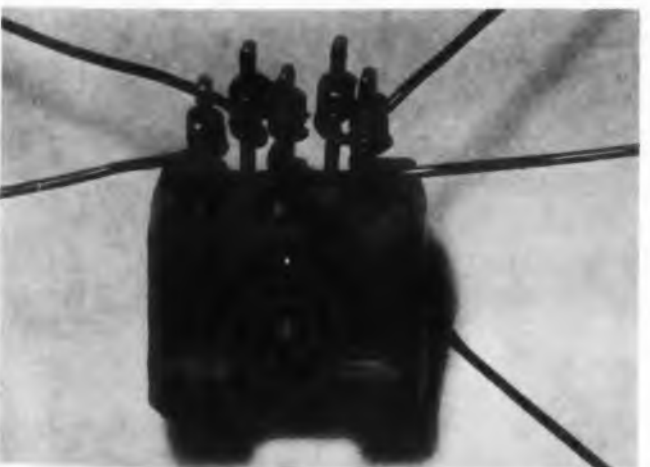
Fig. 4. Connections to subminiature flat-press tube socket.
