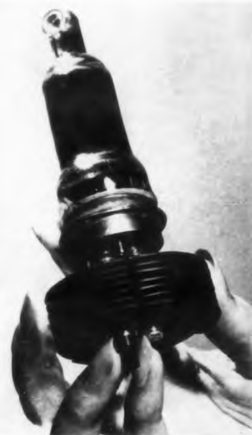
Infrared seeker —lead sulfide—and two Peltier devices in cascade are contained in this tube, made by Nortronics. The PbS sees infrared radiation through the sapphire window (shown at the top).
