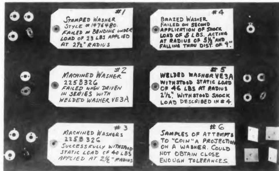
Fig. 10. (right) Results of tests on various stop washers to determine the one least expensive which would meet tolerance limits.
