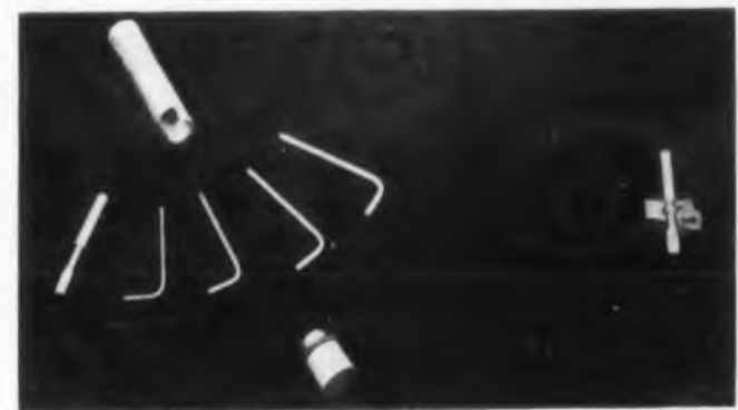
Fig. 6. Tool kit was simplified by substituting set of wrenches (left) with special tool (right).
