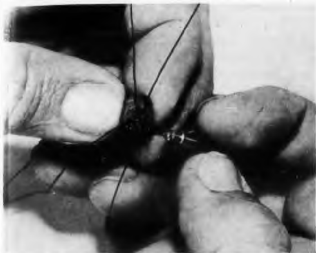
Fig. 1. Using the subminiature wire wrapping tool to connect 28 awg wire to a transistor socket.
