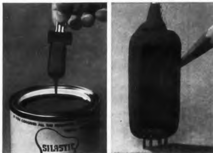
Electronic tube encapsulated with Silastic.
