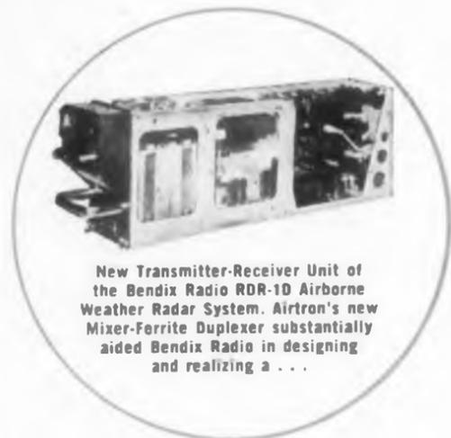
New Transmitter-Receiver Unit of the Bendix Radio RDR-1D Airborne Weather Radar System. Airtron's new Mixer-Ferrite Duplexer substantially aided Bendix Radio in designing and realizing a . . .
