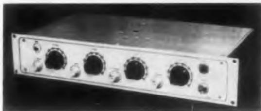
Any delay from 10 to 10,000  $\mu$ sec may be switch selected on the 1104 crystal controlled delay generator. Input pulses may be positive or negative from 5 to 40 v, and output is a 10 v standardized pulse of both polarities. A 1 mc crystal controlled oscillator keeps jitter to  $\pm 0.5$   $\mu$ sec at the maximum range.
