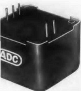
Miniature transformers, designed for printed circuit applications, come in 5 standard case sizes at range from 0.56 in. sq by 0.56 in. height up to 1.27 in. by 1.27 in. height. Audio, power and signal transformers and inductors in these sizes are available in resistor or vacuum tube type. They meet Mil-T-27A Class R or S Life X. Terminal inserts are on standard grid multiples. Special design can meet 500 and 2000 cps.
