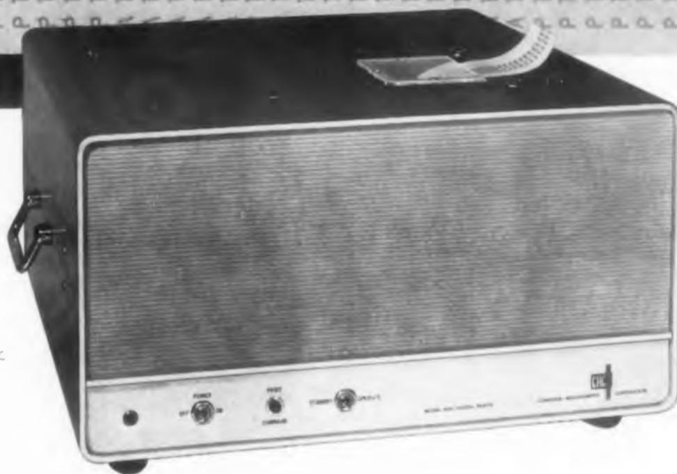
**ALL NEW**, the CMC Model 400C is a reliable, economical instrument for permanently recording digital data from counting, timing, frequency measuring, and data handling systems.
