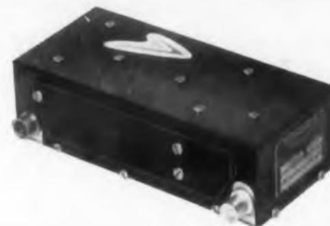
NEW Type 1004 Crystal-Stabilized FM Transmitter—5-watt output from 22 ounce package. True frequency modulation for first time in telemetry attained by diode capacitance variation (circuit patent applied for). 215-260 mc in one unit. Crystal stabilization holds center frequency to 0.01% accuracy through -55 to +100° C, 15g-2000 cps, 80g shock, 8 tuning adjustments. Has built-in output filter. Meets MIL-I-6181B. Available with 6.3 and 28 v filaments.
