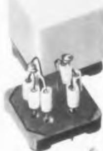
A silicon diode circuit embedded in Stycast 2850 GT — almost indestructible.
