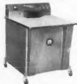
MODEL 942 will saturate Alnico magnets weighing up to 34 lbs. and high flux ceramic magnets of any shape or pole configuration. Operates on condenser discharge principle from regular 115-volt, 60-cycle line. Produces charging outputs (depending on number of 100  $\mu$ f condensers employed) from 100,000 to 200,000 ampere-turns through plug-in transformers, up to 3600 watt-seconds using wire-wound fixtures. Adapters for
