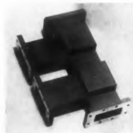
Model FD-TC-501 is a four-port ferrite T circulator for the 5.925 to 6.425 kmc frequency range. The device handles an average power of 20 w and provides 22 db of isolation with 0.5 db of insertion loss. Other three- and four-port ferrite circulators are available to cover the frequency range from 5 to 26 kmc with bandwidths up to 10%.
