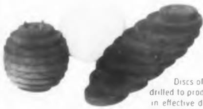
Discs of Eccof foam Hi K 625 D drilled to produce a radial variation in effective dielectric constant and assembled to produce a microwave lens. Lens is encapsulated in Eccof foam FPH. Unit made for Melpar, Inc.
