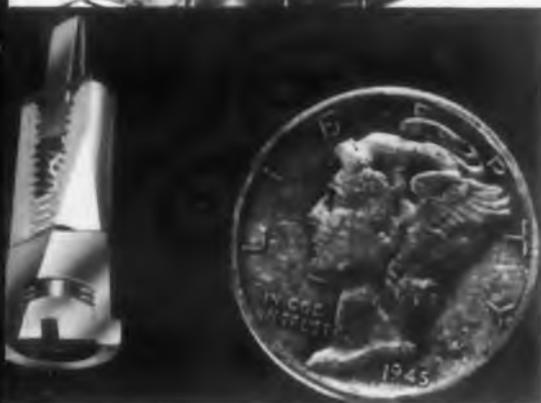
Silicon diode sealed against moisture with Stycast 3020 passes all Mil Spec humidity cycling. This new technique paves the way for a more ruggedized production unit.
