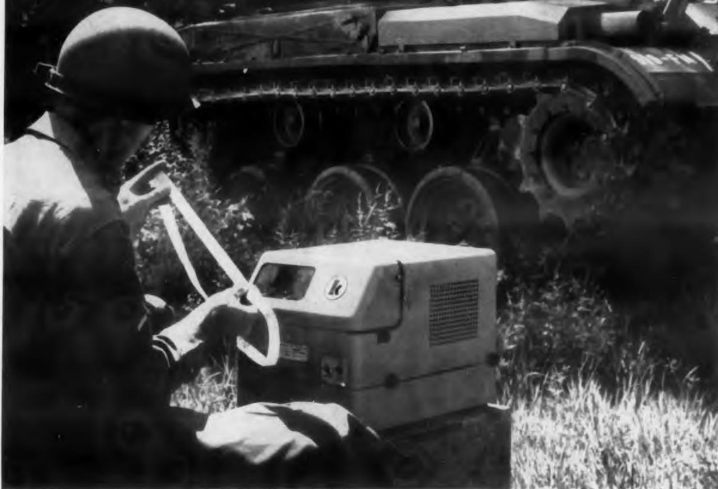
**Capable of reception at speeds of 750 words a minute, new Kleinschmidt unit is world's fastest message printer and code puncher**
