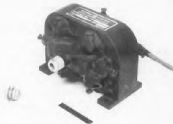
**Fig. 4.** Z5299 voltage-tunable magnetron and experimental 5283 package (General Electric Co.)
