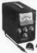
MODEL 1295 is a stable, all transistorized Gaussmeter which provides a conservative accuracy of 3% over nine full-scale ranges: 0-100, 200, 500, 1 K, 2 K, 5 K, 10 K, 20 K and 20 K + gaussses, using a single probe. Two standard reference magnets having 1/4% accuracy are supplied. Weight is 12 lbs. Operates from battery or 115-volt, 50-400 cycle line. Price \$420.
