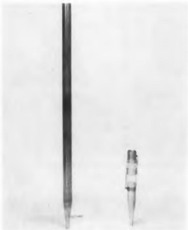
Fig. 1. Standard monopole (left) and 0.072 wavelength test monopole.
