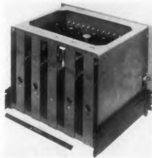
**Delay line driver** produces pulses delayed some 1.5  $\mu$ sec fifteen times. Pulses remain sharp and square, regardless of condition of input pulses.
