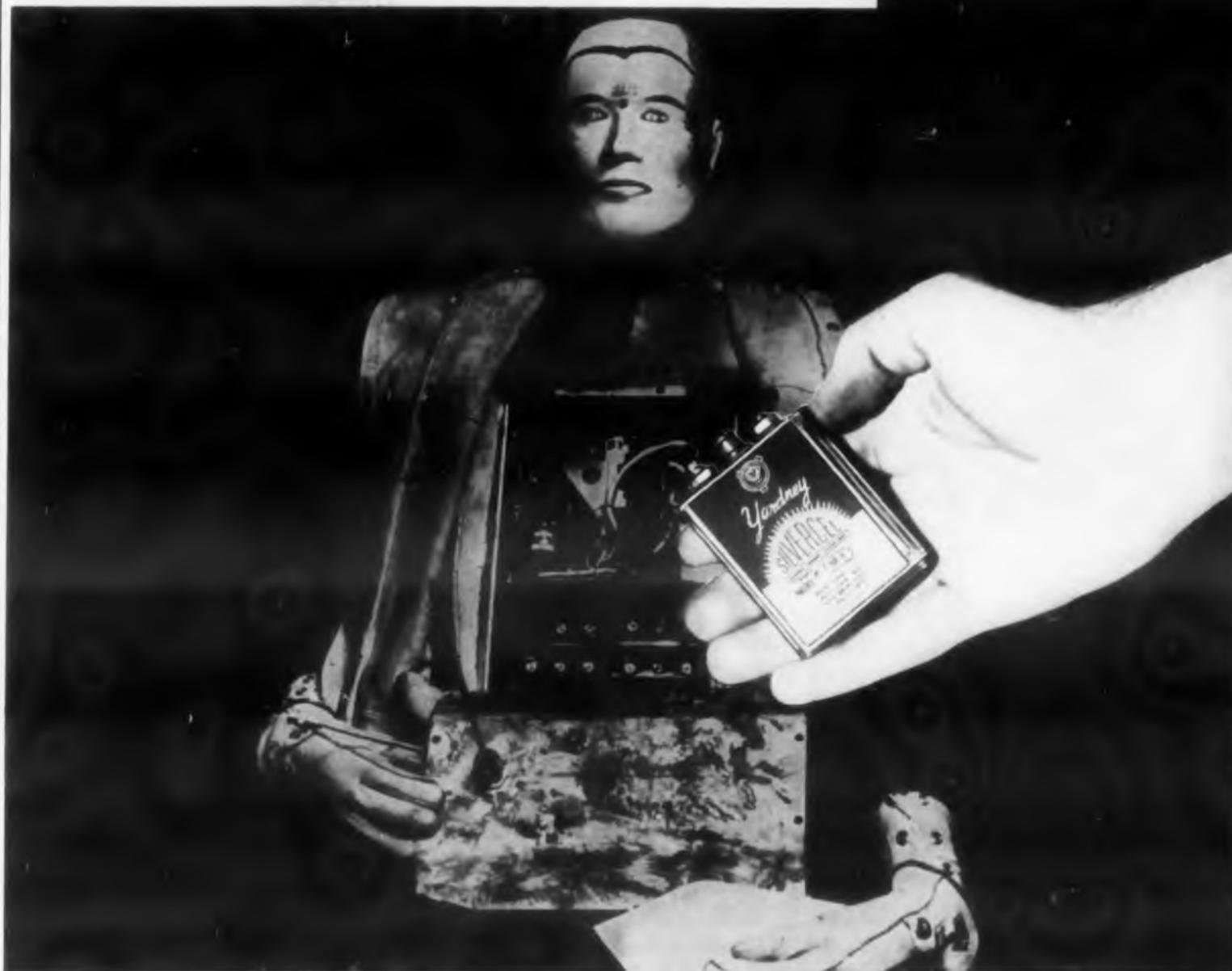
To perfect escape from supersonic aircraft, Coleman Engineering Company, Inc., has created Hurricane Sam, an amazingly real 6-ft., 180-lb. "man". Internally, a YARDNEY SILVERCEL® Battery—a power pack smaller than a human heart—runs strain gauges, accelerometers and a telemetering transmitter, that measure and transmit his almost-human reactions when ejected from a sled traveling at 1,500 m. p. h.
