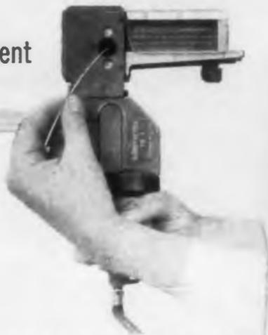
Precision hand, pneumatic, or automatic tooling guarantees uniform and complete crimp for each connection—a measurable quality control—at a high speed production rate.
