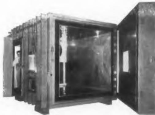
PLANTS, UNION, N. J. AND BALTIMORE, MD. • THERE IS A TENNEY CHAMBER TO SIMULATE ALTITUDE, HEAT, COLD, HUMIDITY, VACUUM, EXPLOSION, SAND, DUST, FOG, AND MOST OTHER ENVIRONMENTAL CONDITIONS.
