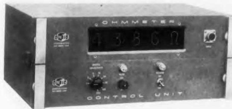
DIGITAL OHMMETER — for rapid, precise resistance measurement
