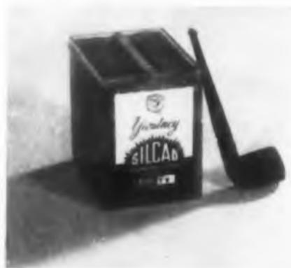
Maintenance free, the Silcad battery is designed to power a completely portable television set. It is also applicable to civilian and military communications systems, to remotely controlled equipment, and to space satellites, where it is recharged by solar cells. A 12 v, 5 amp hr power package, this silver cadmium battery weighs 3-1/2 lb. It combines the high power output of silver with the long life of cadmium and can be recycled as many as 200 times.
