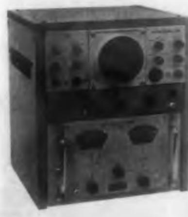
Model MPG-2 multipulse gating unit, for use with the company's microwave spectrum analyzers, provides a means for analyzing the individual pulses in the rf multipulse trains used in complex missile guidance radar systems. Gating circuitry follows the microwave rf head, gat-
