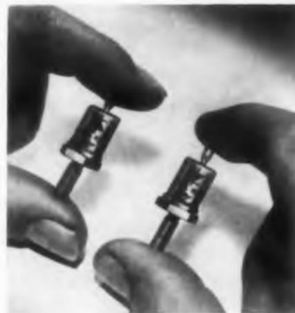
These stable silicon rectifiers are rated at 1500 piv, 300 ma and offer reverse leakages as low as 100  $\mu\text{a}$  at  $75^{\circ}\text{C}$ . Maximum forward voltage drop at  $25^{\circ}\text{C}$  and 150 ma is 4.5 v. Designed primarily for high temperature operation, these units are
