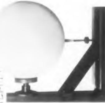
18" Ecco Luneberg Lens under test. Frequency 9 Kmc. Feed 1 1/2" x 1 1/2" horn (12 db). Both E & H plane antenna patterns are shown. Overall gain is about 32 db.
