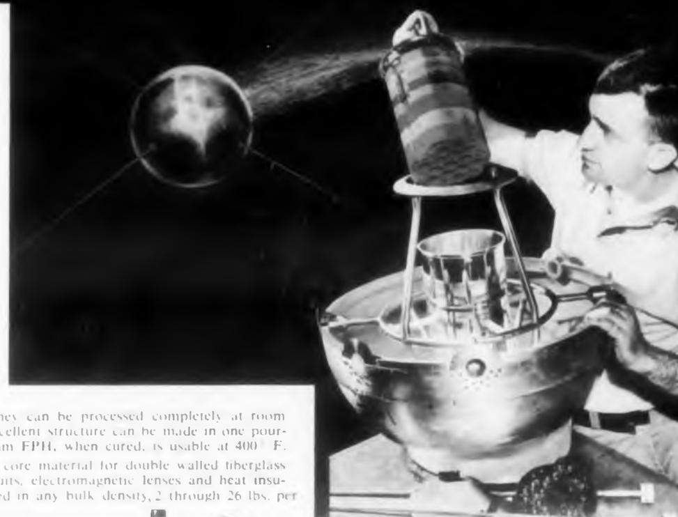
Eccof foam FP, an isocyanate foam in place resin, is used to embed electronic circuitry in the Navy Vanguard satellite. Circuit modules are embedded in blocks of foam and stacked together in the unit just above the containing canister. Similar foam embedment techniques are used in the Army Jupiter C satellite.
