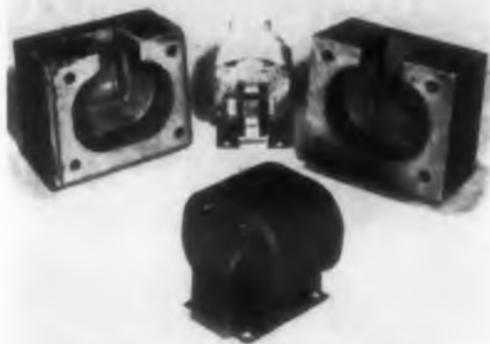
Hysol series 6700 single component epoxy compounds are ready to use without the addition of hardening agents. Stable at room temperature, the compounds meet MIL-T-27B requirements. Filled and unfilled systems are available with several degrees of flexibility and heat resistance to 150 C. The filled compounds are for encapsulation of transformers, toroidal coils, capacitors, and complete circuits. The unfilled are for impregnating transformers and coils.
