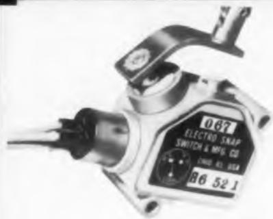
Terminal leads of an Electro-Snap Switch potted in Stycast 2850 GT. The only resin found to completely resist jet aircraft vibration in this landing gear switch application.
