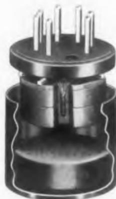
After the component is soldered to the epoxy header, a premeasured pellet is dropped into the cured epoxy shell. The cover and component are then inserted into the shell.
