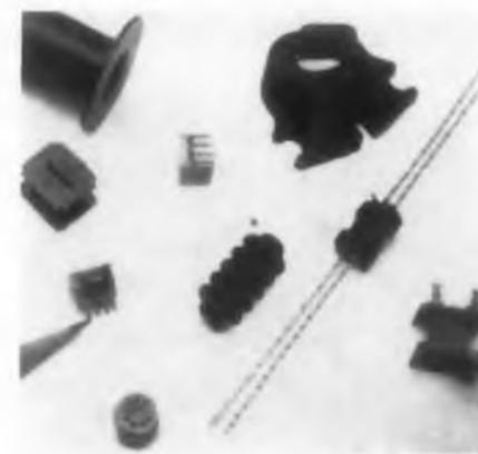
A one component epoxy molding powder, Hysol 8610 offers long storage stability, low shrinkage on cure, good electrical characteristics at high temperatures, and good dimensional stability. It cures quickly at moderate temperatures and has a heat distortion point exceeding 150 C. It can be used for coil and resistor bobbins, electrical component shells, relay assemblies, connector plugs, and switch gear.
