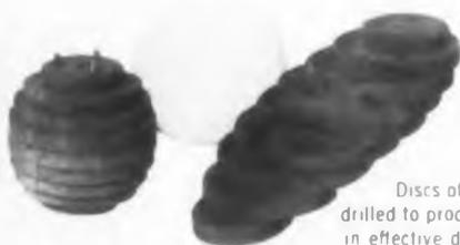
Discs of Eccof foam Hi K 625 D drilled to produce a radial variation in effective dielectric constant and assembled to produce a microwave lens. Lens is encapsulated in Eccof foam FPH. Unit made for Melpar, Inc.
