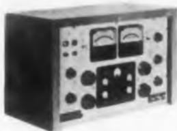
MODEL 829 checks AC and DC meters of all types and ranges. Compact cabinet contains power supply, special Weston standard meters, Wheatstone Bridge and all circuits for quick, convenient instrument calibration to 0.5% accuracy by non-technical personnel. Automatic protection for both operator and instrument under test is provided by interlocks and high voltage discharge circuits. Net price \$2650.
