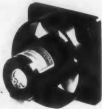
For spot cooling electronic equipment in restricted areas, model S2223-3 tubeaxial fan delivers 40 cfm at 16,500 rpm and 0 in. SP. It has a 1-in. diameter motor and operates from a 200 v, 3 phase, 400 cps source. Built to all MIL-E-5272 specifications, it can withstand ambient temperatures of up to 125 C with a minimum life of 2000 hr. The unit is 2 in. long and has a 2-1/4 in. square mounting flange.
