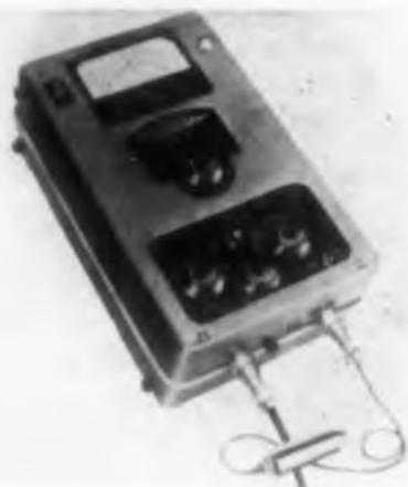
With the plugging in of appropriate transducers or strain gages, the model 1650 Poly-Gauge provides direct measurements of pressure, load, force, displacement, and strain. It indicates displacement in thousandths of an inch, strain in pounds per square inch, or load in pounds, dependent on the transducer in use. The range factors of 100, 25, 10, 2.5, 1, or 0.25 are selected by the range control. An output which can be used for recording or control
