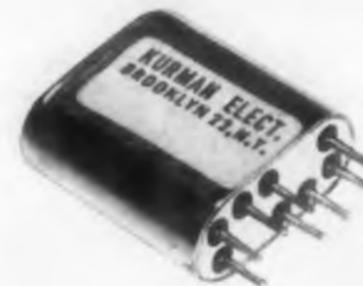
Model KX relays are 0.4 in. wide, 0.8 in. long, and 0.875 in. high. They operate from  $-65$  to  $-125$  C with 200 to 250 mw sensitivity, and are built to withstand shocks of 50 g and vibration frequencies of 20 to 2000 cps at 20 g. Maximum coil resistance is 10 K; maximum contact resistance, 0.02 ohms. The units are available with three different header combinations.
