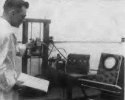
**LEAK DETECTION TEST** subjects components to minute inspection of hermetic sealing with a mass spectrometer type leak detector.
