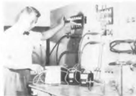
Preliminary testing of foil-wound transformer.
