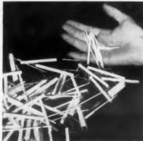
Insulation of thermocouple wires, used in such equipment as gas turbines and nuclear reactors, involves stringing them through a tube of sintered magnesium oxide, inserting in a stainless steel sheath and then swaging.
