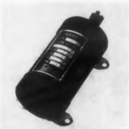
Designed for use with the company's continuous cable aircraft fire detection system, the model 297-115-3 magnetic amplifier control assembly is 1-3/4 in. in diameter and 3-5/32 in. long. It weighs 0.8 lb. Ruggedly constructed, it does not require a shock mounting and can be placed almost anywhere in the aircraft. The unit consumes 1 w for either standby or alarm and will carry a load of 170 ma at 28 v dc. Controls capable of carrying larger loads are also available.
