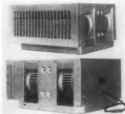
A recessed, two-speed, packaged blower, model ZEB610ESZ has a side exhaust and can be used to divert air into a duct system. It operates quietly and delivers 800 cfm at high speed and 600 cfm at low. Normally used for bottom-rack mounting, the unit is 8-3/4 in. deep and fits standard 19 in. racks. It is equipped with a permanent filter and meets MIL-E-4158A requirements.
