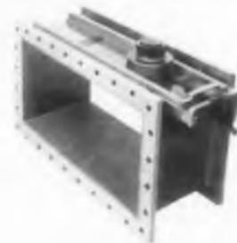
Type 223-LW Waveguide Rotary Standing Wave Indicator for standing wave and reflectivity measurements in WR-2100 waveguide systems over the frequency range from 350 to 530 mc/s. Residual VSWR less than 1.03.
