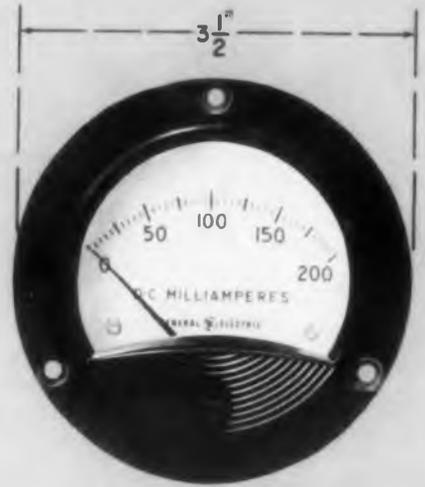
Old round design with 3 1/2-inch diameter has relatively small scale and numbers.
