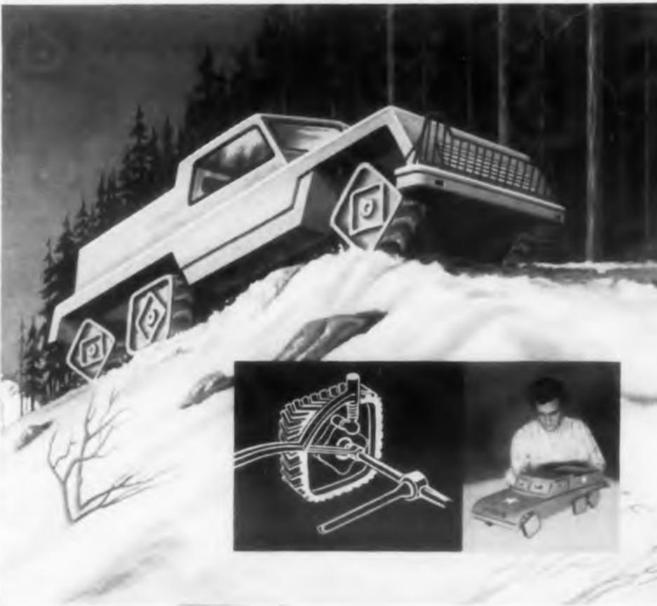
**SQUARE WHEELS?** Yes ... square wheels. Operating by means of a floating axle and cam gear, they take the bumps out of rough terrain and provide more traction. U.S. Patent No. 2736540 has been granted to designer Albert Sfredda of Bethlehem, Pa., for his invention.
