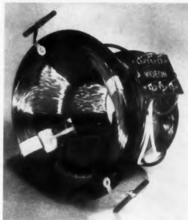
Standard horizontal deflection coils and toroidal vertical deflection coils are wound on a ferrite wedge-shaped ring in this TV yoke made by the Videon Company in France.
