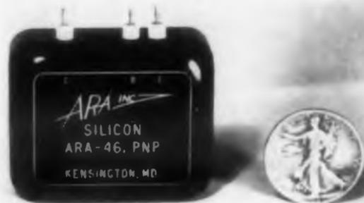
The ARA-46P silicon composite pnp transistor is thermally compensated to operate at temperatures up to 200 C. It has the general characteristics of a small signal transistor at the input and that of a power transistor at the output. Operating specifications are: collector voltage, 40 v; collector current, 3 amp; power dissipation at 25 C, 35 to 50 w; power dissipation at 150 C, 2 to 5 w; current gain, 10,000; input impedance, 2000 ohms; output impedance, 500 ohms.
