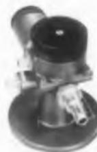
Type 219 Rotary Standing Wave Indicator for use in coaxial systems for standing wave and reflectivity measurements over the frequency range from 100 to 1,000 mc/s. Residual VSWR less than 1.03.
