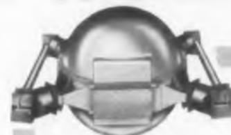
High-performance mounting system protects 180-lb. guidance platform against ICBM environment. Highly original design weighs only 18 lbs., uses Lord BTR elastomer for broad temperature operation.
