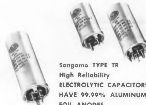
The use of 99.99% high purity aluminum anodes in Sangamo Type TR Twist-Tab Electrolytics, surgically clean papers, and a highly effective end seal gives these capacitors excellent operating life and superior electrical characteristics. They are designed to operate in a temperature range from -20°C to 85°C and are available in ratings from 3 to 450 volts D.C.
