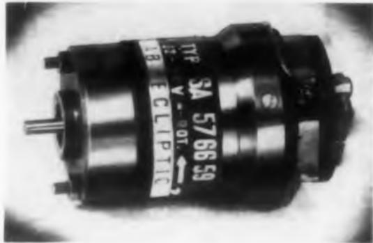
Rated at 1/100 hp at 4500 to 9000 rpm, this dc motor is equipped with a governor that controls shaft speed variation within 1%. Rotor torque is rated at 3.5 oz in. for intermittent duty. Overall dimensions are approximately 1-1/2 x 3 in., including the shaft which protrudes about 1/2 in. beyond the frame. Weight of the unit is about 7 oz. Body of the M-120 unit is solid aluminum with anodized finishes available in 6 colors.
