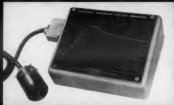
Since different types of pilot balloons have different rates of rise, and wind effects vary with each type of missile, signal inputs to the computer must be easily and quickly adjusted. That's one reason why USASRD engineers chose two Vernistat Adjustable Function Generators. Only seconds are required to change from one function to another.
