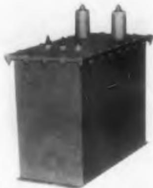
Designated Model PS-30T, this 30 kv, full-wave voltage-doubler power supply operates on 117 v, 60 or 400 cps. The unit delivers 1 ma continuous and 1.75 ma peak current. Ripple is 1.5% at 1 ma and regulation is approximately 7% from no load to full load. It has replaceable 1B3 rectifier tubes and plastic dielectric capacitors. Dimensions of the case are 5-1/4 x 11-3/8 x 9-1/2 in., and the unit has oil-tight solder-seal terminals.
