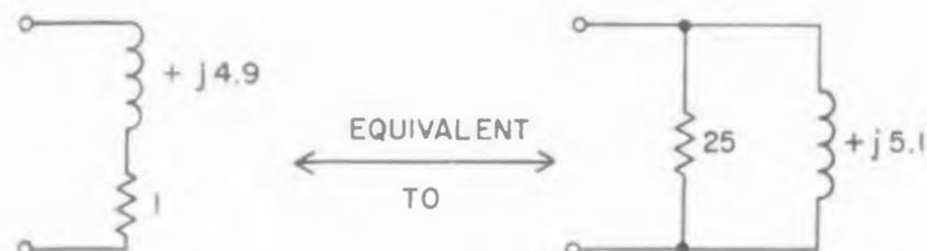
Fig. 8. Series and shunt representation of a load impedance,  $1 + j4.9$ .
