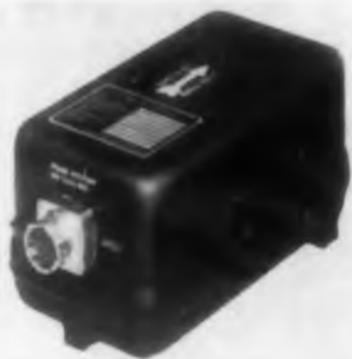
Flexible design of the series 1080 gyros allows the unit to be made into a directional gyro or a free gyro as well as a vertical gyro. Weighing a maximum of 4.75 lb, the unit's maximum dimensions are 3-7/8 x 3-7/8 x 6 in. Standard excitation of the gyro motor is 115 v, 400 cps, 3 phase. Optional excitation: 26 v, 400 cps, 3 phase; 115 v or 208 v, 400 cps, 3 phase, 4 wire. Standard pickoff is 115 v, 400 cps, 1 phase, with optional rated at 26 v, 400 cps, 1 phase.
