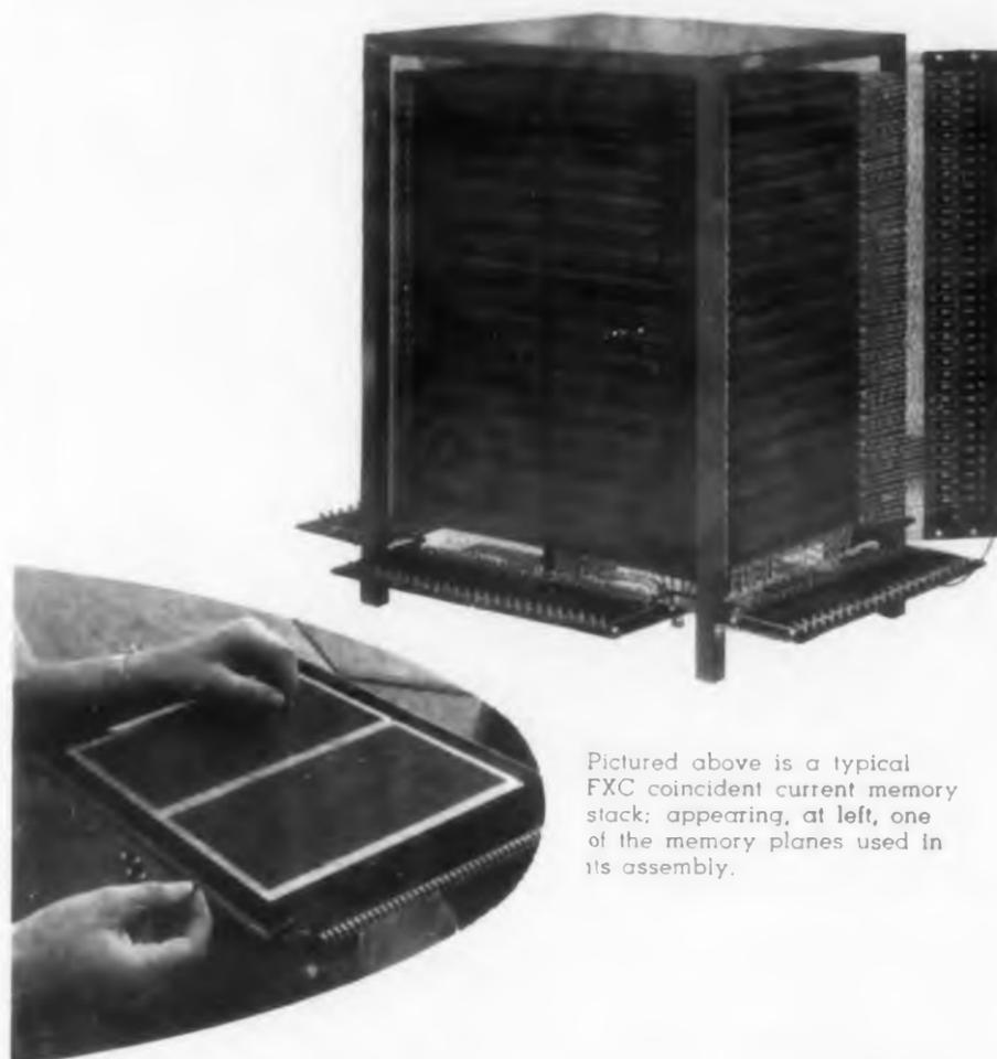
Pictured above is a typical FXC coincident current memory stack; appearing, at left, one of the memory planes used in its assembly.
