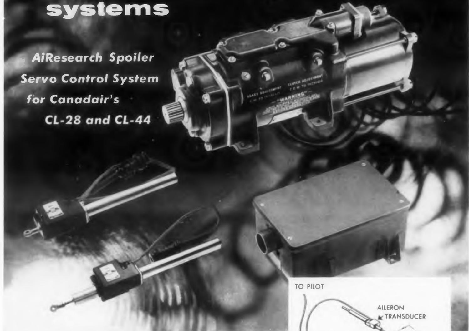
A substantial increase in aileron effectiveness is achieved by the AiResearch Spoiler Servo Control System which augments the function of the aileron by increasing the rate of roll of the aircraft. Full spoiler surface travel is achieved in 0.5 seconds by electromagnetic clutching of the 4 H.P. power servo.
