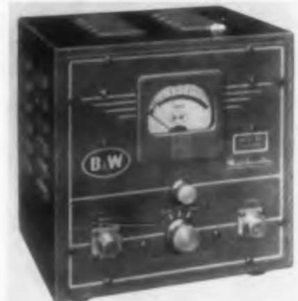
The Matchmaster is an instrument which tests transmitters without signals on the air. It consists of a dummy load with a direct reading rf wattmeter and a standing wave ratio bridge. It is useful for measuring the swr in antenna feed lines, the adjustment of radio transmitter power output before going on the air, and many other applications. All components are contained in a cabinet 6 x 8 x 8 in.
