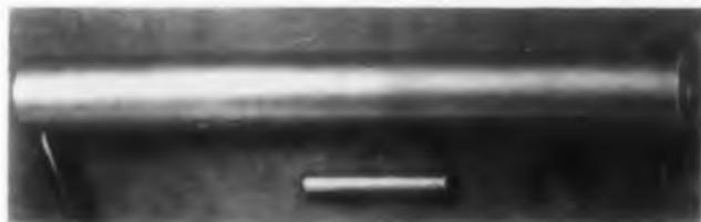
These differential transformers have a linear stroke of 70% of coil length, and high output and low impedance secondary windings. Linear displacement is from  $\pm 0.5$  to  $\pm 8$  in. Ratio of output voltage, at range limit, to null voltage is 1000:1. Linearity of  $\pm 0.5\%$  over a temperature range of  $-60$  to  $250$  F is attainable. The units are magnetically shielded, potted and furnished with Teflon insulated leads.
