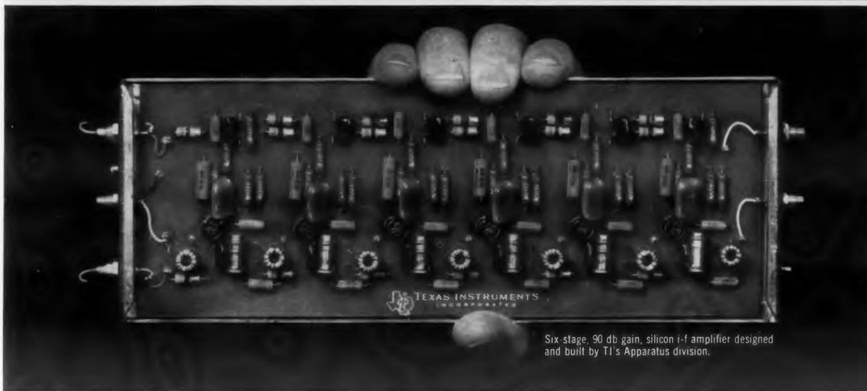
Six-stage, 90 db gain, silicon i-f amplifier designed and built by TI's Apparatus division.
