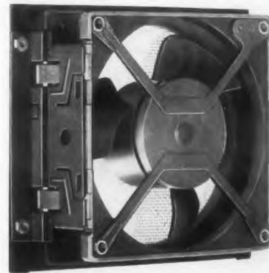
Three pieces of fan assemble without screws or bolts. Bezel with grill clamps onto molded venturi block.
