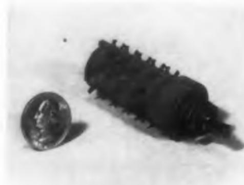
Series 1900 Rotary selector switch is totally enclosed and built to exceed MIL-S-6807A requirements. It will carry 10 amp continuously and 5 amp, 115 v ac or 3 amp 28 v dc intermittently. Dielectric strength is 1800 v. The unit is available with a single wafer or up to 16 wafers and with continuous rotation or 2 to 10 positions with stops.
