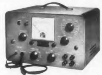
MEGPOT MODEL 573 provides all the efficiency, convenience and speed for high potential testing of components or complete assemblies, but without the megohm-meter, resulting in even more compactness and economy. Both models are self-contained, attractively housed and easily portable.
