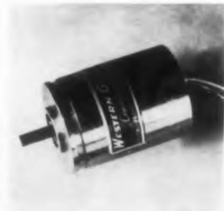
These size 10 and 11 servo motors are available for 26, 55, or 115 v ac, 400 cps operation. They are 6 pole units with a stall torque of 0.6 oz-in. minimum and a no load speed of 6500 rpm. Rotor inertia is  $1 \text{ g cm}^2$ , and acceleration at stall is  $42,000 \text{ radians per sec}^2$ . The units are 1-11/32 in. long and designed to operate in ambient temperatures from  $-65$  to  $+125 \text{ C}$ . Special voltage requirements are available on order.
