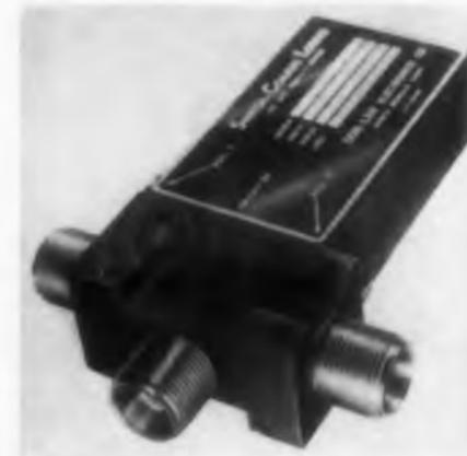
Type SP2T is a 0.7 lb rf coaxial lobing switch with a range of 100 to 10,000 mc, a maximum vswr of 1.2 to 1, and an isolation rating of 50 db down. Make before break or break before make switching is available. The unit is hermetically sealed, glass to metal, and has a minimum life of 1000 hr. Several models are available with a choice of type N, HN, or SC rf connectors.
