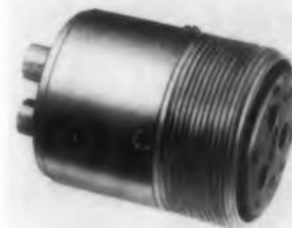
MS-E pin or socket types, Seal-E electrical connectors are supplied in sizes through O. Constructed with partitive hermetic glass seals they also have interfacial seals for internal moisture-proofing.
