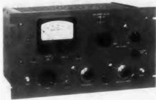
Designed primarily for telemetering instrumentation, this instrument measures: the dropout characteristics in a magnetic tape recording over a range of operating frequencies from 7.5 to 80 kc; a dropout amplitude range from 15 to 85%; and a dropout width range from 38 to 360 usec. For each dropout detected with respect to a predetermined amplitude and width, a 70 v positive going, rectangular pulse is emitted. It measures dropouts in accordance with Mil-T-21029 (Ships).
