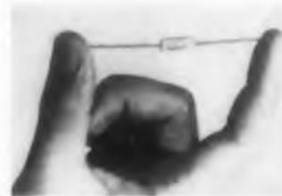
Hermetically sealed type RSH-2B precision wirewound resistors have resistances from 1 to 4200 ohms and stability levels of 1, 0.5, 0.25, and 0.1%. Depending on the stability level, power ratings are 0.75 to 1.5 w at 25 C, derating to 0 between 100 and 130 C. Temperature coefficient is 0.00002 per deg C, and tolerances are between  $\pm 0.05$  and  $\pm 3\%$ .
