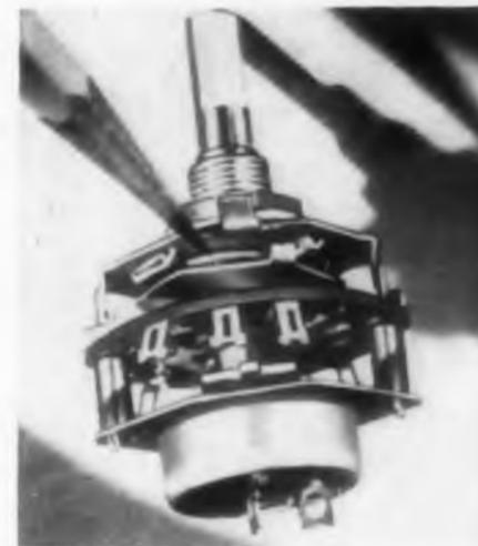
A steel alloy spring is built into the index mechanism of the PA-070 switch and it controls the spring return action. Switches with this feature can be supplied as single or double section units, or as single section units with line switch. Up to six positions per section, including the spring return position are available. Spring return can be placed in either the first or last position, and sections are laminated phenolic type PBE per Mil-P-3115, voltage breakdown 1000 v rms.
