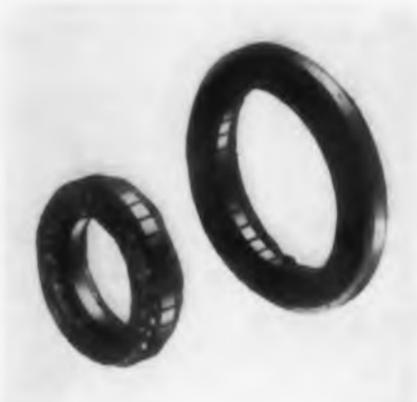
Available in size 20 and 27, these pancake synchros and resolvers feature accuracies down to 5 min and are made for instruments such as inertial guidance systems. Their electrical properties are designed to meet specific applications or to match standard components for accuracy, voltage gradient, and impedances. They may be obtained with integral flanges and hubs.
