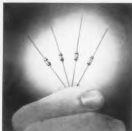
Major step in the trend to ever smaller radar and microwave equipment to meet today's military and commercial demands is represented by Sylvania's new line of subminiature microwave diodes. The new diodes meet the electrical performance of their larger counterparts and are equivalent in ruggedness and reliability. They combine in one unit Sylvania's unmatched experience in diode packaging and proven technical excellence in microwave diode design.
