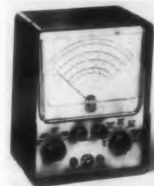
The VT-10 VTVM has an edge-lighted 6-in. meter for accurate reading. Sensitivity of the unit's movement is 400  $\mu$ a, with 2% accuracy. For measurement stability 1% precision resistors are throughout the range switch. The unit has 7 ac (rms) and dc ranges, 0 to 1500 v. Also 7 ac peak-to-peak ranges, 0 to 2000 v. Other ranges include resistance, 0 to 1000 megohms, and db.
