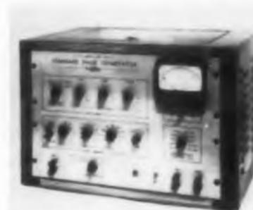
Phase generator model 410 is a combination phase shifter and phase difference generator that covers 5 cps to 200 kc. The addition of an external capacitor extends this range down to 0.1 cps. Accuracy is 0.1 deg over the audio frequency spectrum, decreasing above and below. The unit can be used for the calibration of phase measuring devices, or, with an external phase detector, as a precision phase measuring device.
