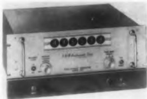
The 1300 series of electronic tachometers and frequency counters includes types for remote indication, for explosion-proof installation, and for dual readout requirements. Time bases available have fixed selectable times of 0.1, 0.5, and 1 sec. The units have an accuracy of  $\pm 1$  count, a display time that is adjustable from 0.1 to 10 sec, and a sensitivity of 50 mv rms. They have an input impedance of 1 meg and automatic or manual reset.
