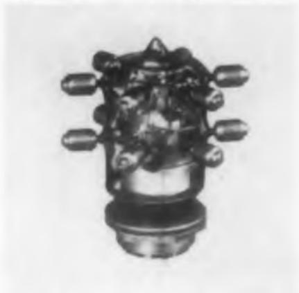
The model RB4 transfer relay is designed for high voltage applications involving antenna switching, pulse forming networks, and similar rf and dc circuits. The 4pdt unit has a vacuum dielectric, sapphire actuating rods, and removable actuating coils for 26.5 or 115 v dc operation. Peak test voltage is 25 kv dc or rf and rated operating voltage is 20 kv at 2.5 mc and 10 kv at 16 mc. Contact resistance is under 0.01 ohm and current rating is 13 amp rms at 60 cps and 8 amp at 16 mc.
