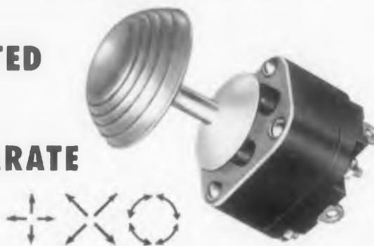
A familiar sight to helicopter pilots is this versatile Hetherington Type F441 Four-Way Switch. Here it is housed, along with other Hetherington Switches, in a hand-grip which fastens to the flight control stick. Moving the Switch's thumb-type knob up or down, right or left, operates control motors for hoists or lateral trim.
