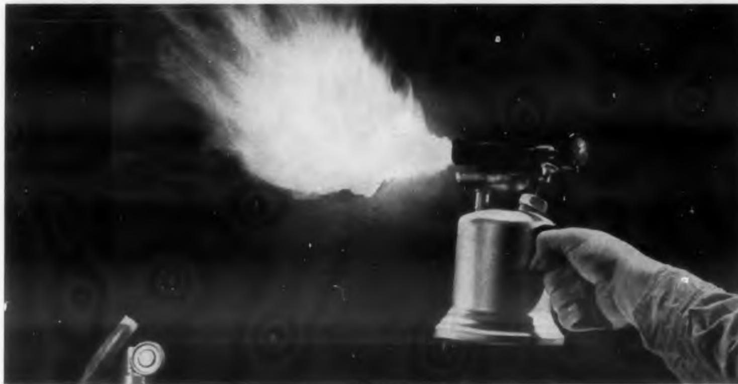
Sheet of Synthane to which blowtorch is being applied
