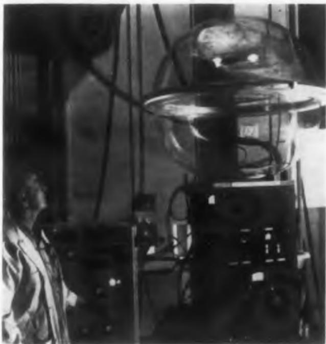
Note the antenna inside the globe and the corona discharge occurring in the thin air.
