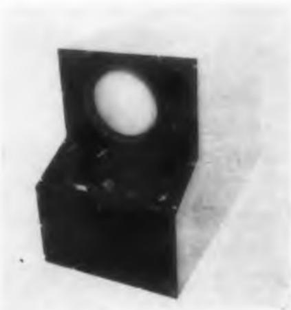
Designed as an attachment for the company's S-series winding machines, the IC-601 inductance comparator provides a means of winding toroidal coils to preset inductances on permalloy powdered or ferrite cores. The unit eliminates core grading and inductance adjustments and permits accuracies up to 0.5%. It has built-in decade inductances which allow a setup range and provides continuous monitoring of the winding process.
