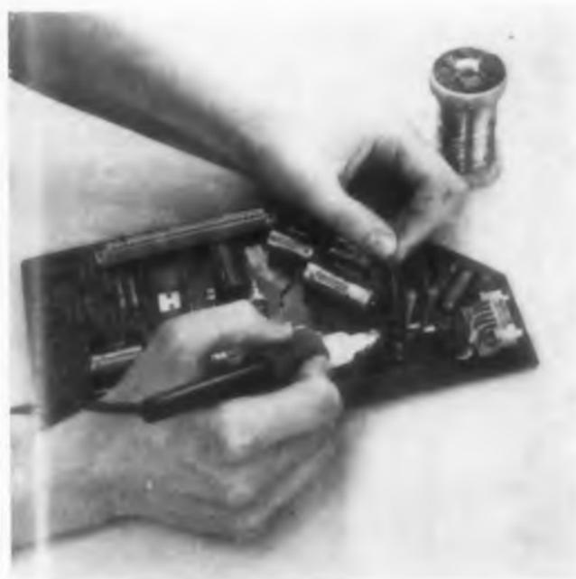
Fig. 2. The wet-felt heat sinks, to the right of the soldering iron, protect the diode from thermal damage during soldering.
