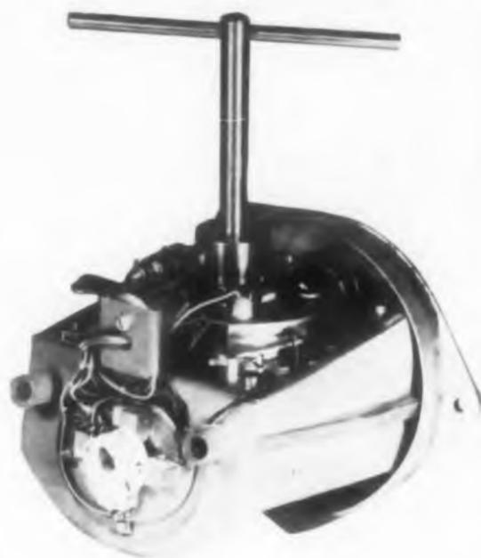
Fig. 1. Caging and winding of the gyro is done with a removable key at the factory. The unit is capable of being stored for an indefinite period in this condition.
