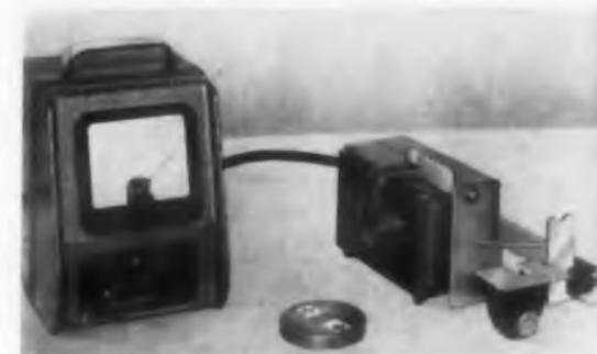
Model 100 Talysurf is a portable, semiautomatic instrument for production inspection and precision testing of surface finish. The assembly includes work table, pick-up, stylus, support, and motorized drive. It can carry small work in universal work-holding fixtures or be fitted with quick loading production tooling. The same unit, inverted, can be used to check large flat or cylindrical work.
