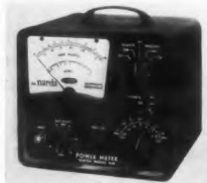
Self-balancing and transistorized, the model 410 microwave power meter provides automatic direct-reading measurements of cw or pulsed power. It may be used with all 100 or 200 ohm bolometers or thermistors, of positive or negative temperature coefficient, requiring any bias current up to 18 ma in any frequency range for which there are bolometer or thermistor mounts. It has 0.001 to 0.01 mw and 0.003 to 0.03 mw scales in addition to the five standard scales up to 10 mw.
