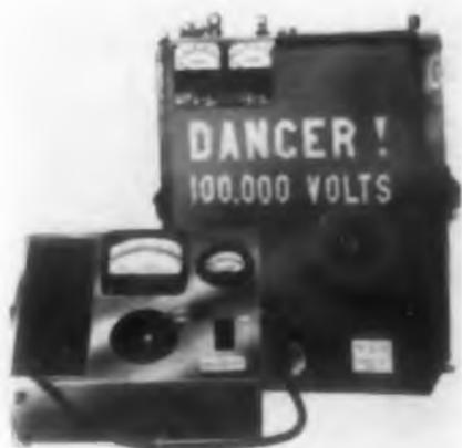
Series VON portable high voltage dc insulation test instruments and power supplies have ranges from 30 kv at 40 ma to 250 kv at 7 ma. All models are sectionalized to provide maximum portability and minimum weight, and supplemental stages may be added to the base power units to increase voltage ratings.
