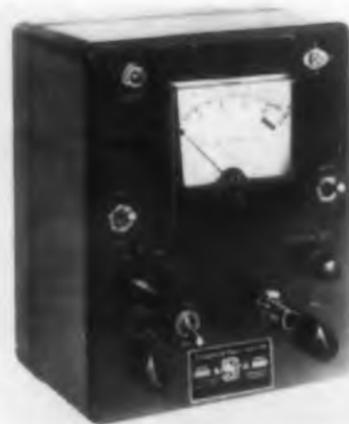
The model 219 A transistor tester permits the measurement of transistor beta parameters with transistors in the circuit. Beta and collector leakage current parameters may be measured with the transistors removed from the circuit. The unit is packaged in a compact carrying case and operates from either a self-contained battery supply or 110 v, 50 to 60 cps.
