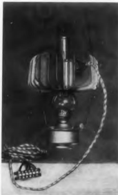
Fig. 1. Thermoelectric generator installed on a lamp, with the connecting plug to a radio receiver.
