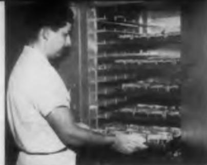
**SHOCK TEST** in each of three mutually perpendicular planes is available up to 150 G's—with concurrent electrical testing.
