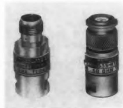
Model 535 50-ohm coaxial terminations are available with type TNC male or female connectors. They can also be supplied with types N, C, SC, and BNC connectors. The units have a dc to 10 kmc frequency range; 1 w average and 1 kw peak power handling capacity; and individual vswr calibrations of dc, 400, 1000, 2000, 4000, 7500, and 10,000 mc. The film resistors used are artificially aged for maximum stability.
