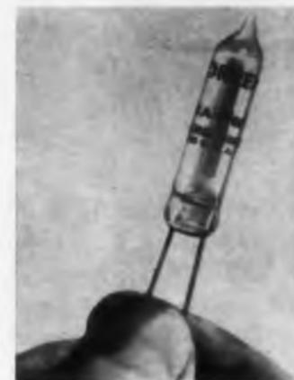
Type GV3A-700L corona type regulator tube is designed for operation at 700 v and for currents of 0.001  $\mu$ a or higher. Featuring economy of current drain from the primary power source, the unit can be used in nuclear battery regulation, solar cell regulation, and the regulation of transistorized power supplies.
