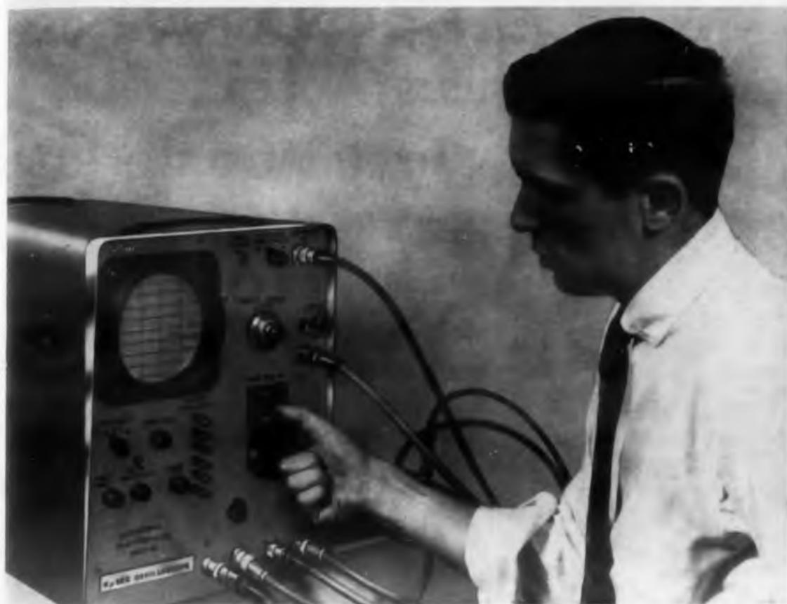
This scope features 400  $\mu\text{sec}$  rise time and 2.5 mv/cm sensitivity.
