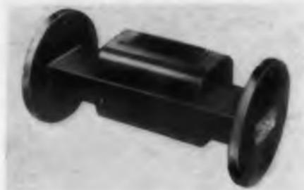
Covering the 3.95 to 12.4 kmc range in three models, these ferrite isolators have 1 db insertion loss and a 1.2 vswr. Rated at 5 w, they can handle up to 25 w with temporary electrical degradation. Model 1205 covers the entire 2 x 1 in. waveguide range with a minimum isolation of 16 db; model 1204 covers the 1.5 x 0.75 in. waveguide range with a minimum isolation of 20 db; and model 1203 covers the 1 x 0.5 in. waveguide range with a minimum isolation of 30 db.
