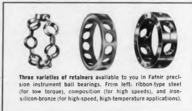
Three varieties of retainers available to you in Fafnir precision instrument ball bearings. From left: ribbon-type steel (for low torque), composition (for high speeds), and iron-silicon-bronze (for high-speed, high-temperature applications).
