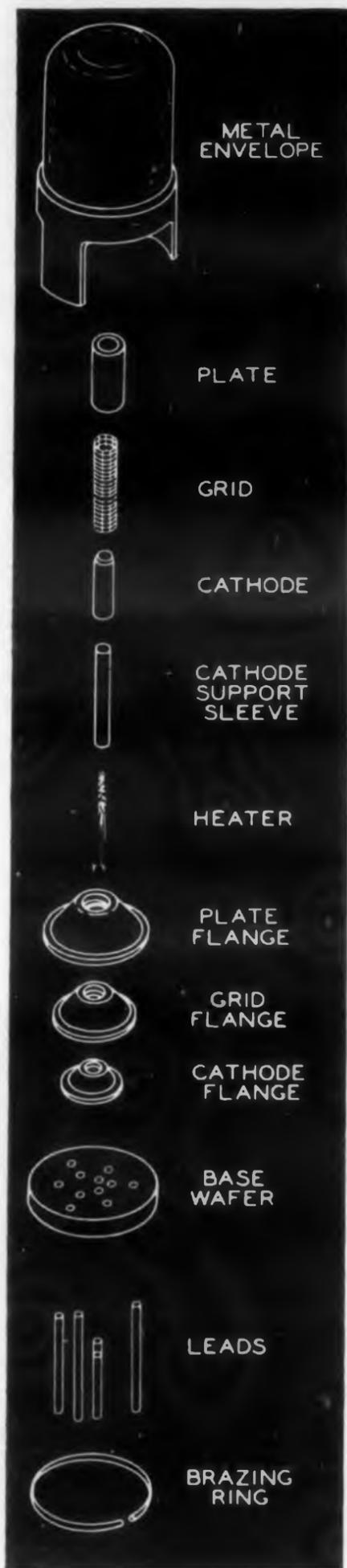
Fig. 1. Exploded view of development Nuvistor Triode.
