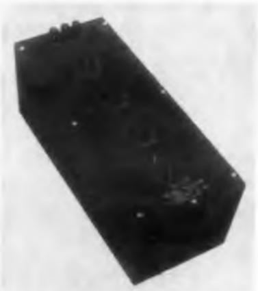
For substitution in the design of equalizers and filters at audio and ultrasonic frequencies, these decade inductors have moisture protected, low distributed capacity coils wound on temperature stabilized molybdenum permalloy cores. Types DIA1 through 4 have one decade and ranges from 0.001 to 10 h; types DIB2 through 4 have two decades and ranges from 0.001 to 11 h; types DIC3 and 4 have three decades and ranges from 0.001 to 11.1 h; and type DID4 has four decades and a 0.001 to 11.11 h range.
