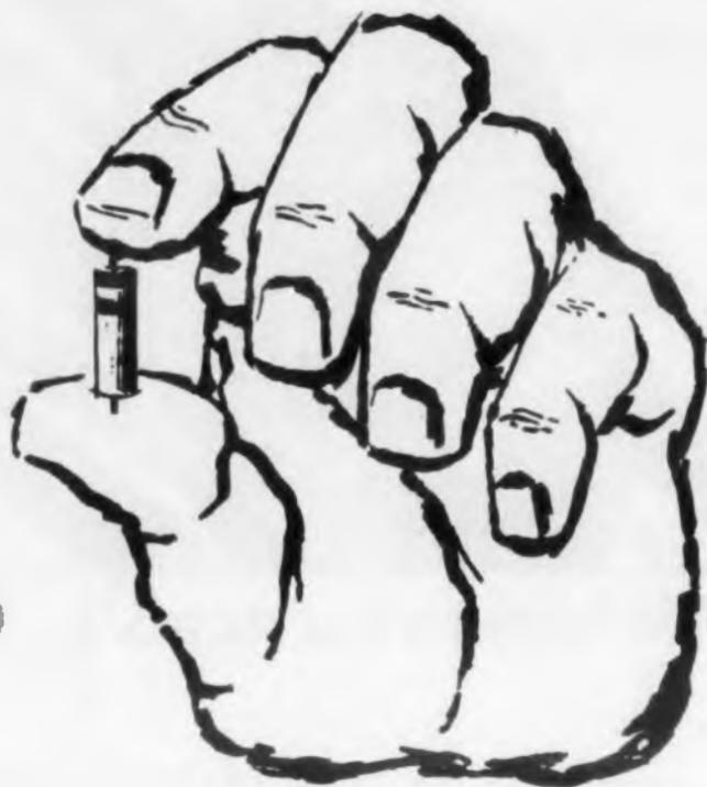
Take a 1-watt resistor. Place it across the programming terminals of a Regatron Programmable Power Supply. Instantly you've fixed the output voltage to 1/1000 of the resistance value. For example, a 22.5K resistor will fix the output at 22.5V. For a perfect repeat every time, use the same resistor. For other voltages use a different resistor. The output will always equal 1/1000 of the resistance value.
