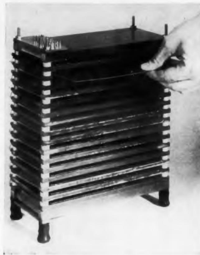
**Fig. 3.** Twistor matrix memory with 512 word, 26 bits per word capacity. Program or other semipermanent data is changed by removing plastic board with permanent magnets etched on it, substituting a new program. Size of module will soon be halved.
