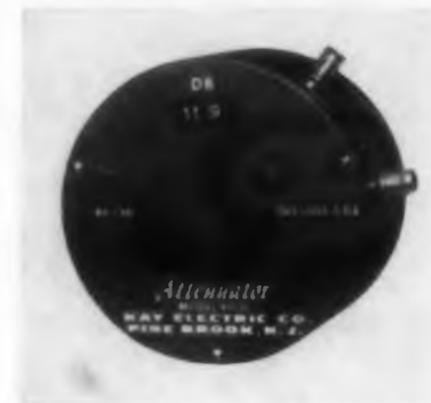
Rotary switched attenuator models 40-0, 41-0, and 42-0 have input and output impedance of 50, 75, and 90 ohms, respectively. They provide attenuation from 1 to 119 db in 1 db steps and operate from dc to 500 mc.
