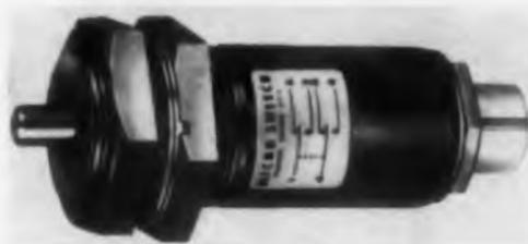
This switch, designated IEN75-R, meets the requirements of MIL-S-901B which call for a 2000 ft-lb shock test. The unit is designed for wide military applications. Its switching chamber is sealed and filled with an inert gas under pressure to insure operation regardless of changes in atmospheric conditions. Electrical rating at sea level or 100,000 ft: 28 v dc, 24 amp, inrush; 4 amp, resistive and 115 v ac, 5 amp, resistive.
