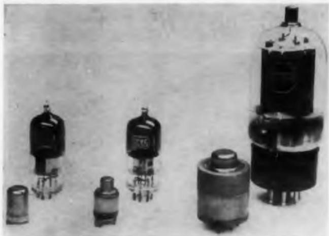
**Fig. 4.** Nuvistors compared with their present-day counterpart—triode (l), tetrode (c), beam power (r).
