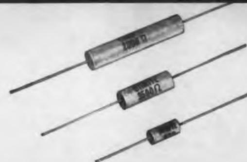
**MOLDED PRECISION WIRE-WOUND POWER RESISTORS** Insulated units with Silicone-Type molded covering. Available in 3-, 5-, and 10-watt sizes. Tolerances: 0.1%, 0.25%, 0.5%, 1%, and 3%. Maximum resistance: 3-watt, 10,000 ohms; 5-watt, 25,000 ohms; 10-watt, 50,000 ohms.
