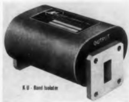
Model W-658-3A-2 transverse field isolator consists of rectangular waveguide with permanent magnetic transverse field and ferrite sections built into the unit. Frequency range of the unit is 12.5 to 18 kmc with isolation at 20 db min and insertion loss is 1 db max. Input vswr is 1.15 max throughout the range with peak power at 100 kw nominal. Ambient temperature operating range is -55 to 150 C. And size is 3 x 1.8 v 2.175 in.
