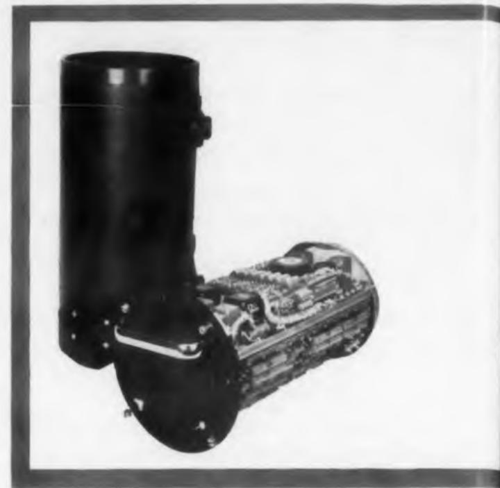
Excessive heating in electronic equipment may be detected and evaluated by building a thermal mockup of the proposed design. This article offers the designer a practical technique for solving the specific design problem of predicting the heating in an electronic package while the development work is still in the preliminary design stage. Evaluation of subsequent cooling methods may be made and the selection of a final design accomplished.
