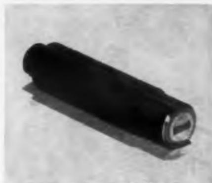
The model HD-9 is a single track, low inductance head that will read and record information on magnetic memory drum systems at high frequencies. It allows a 2-1/2 to 4 mil spacing between head and recording medium with negligible loss in definition. Using a locking four conductor polarized plug, the unit is 2.186 in. long and 0.5 in. in diameter.
