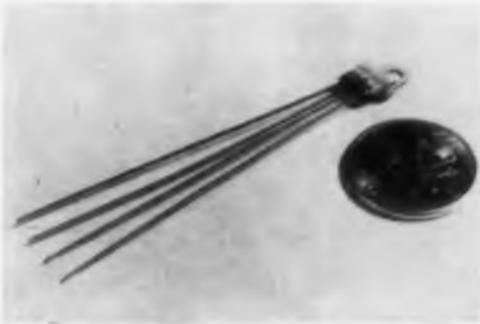
Series 80 rectifiers are designed for use with dc meters of 20 to 200  $\mu$ a full scale current. Active cell area is 0.0012 sq in. and dimensions are 0.125 x 0.27 x 0.4 in. exclusive of leads. The units are made for single hole mounting by a no. 2 screw and have nickel silver filiform leads that are easily soldered or formed to fit printed circuits.
