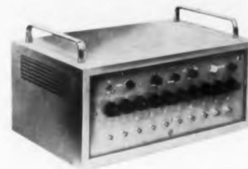
The Beamplexer is a ten position high speed electronic switch utilizing the Burroughs Beam Switching Tube. It provides a means of displaying up to ten separate channels of information on a conventional single-beam oscilloscope. Dual controls on each of the ten input channels allow both amplification and the vertical positioning of the signals, so that they may be superimposed on each other or placed in any desired relationship.
