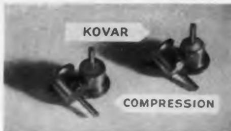
Two types are available. The first type is represented by KOVAR® matched seals in which the identical thermal expansion characteristics of KOVAR Alloy and borosilicate hard glasses result in a fused hermetic bond. Since KOVAR has about the same expansivity as silicon and germanium, stability in operation is assured. The second type is represented by the compression seal which relies on differences in contraction between glass and metals, like mild steel, to provide a tight joint.
