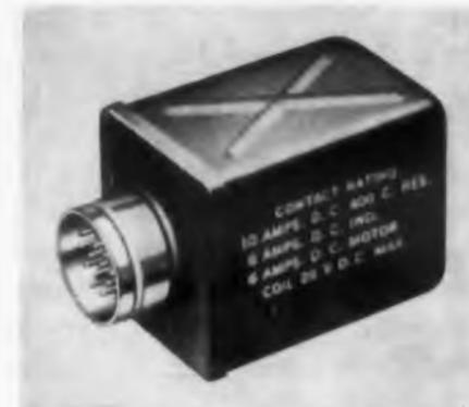
A 4pdt aircraft and missile relay, the series 3205 exceeds MIL-R-6106-B, Class B requirements. Contact rating is 10 amp for resistive ac and dc, normally open or closed, and 6 amp for inductive dc or motor dc, normally open or closed. The unit incorporates a Deutsch DM 5600 series miniature receptacle and measures 1-21/32 x 1-7/16 x 2.063 in.
