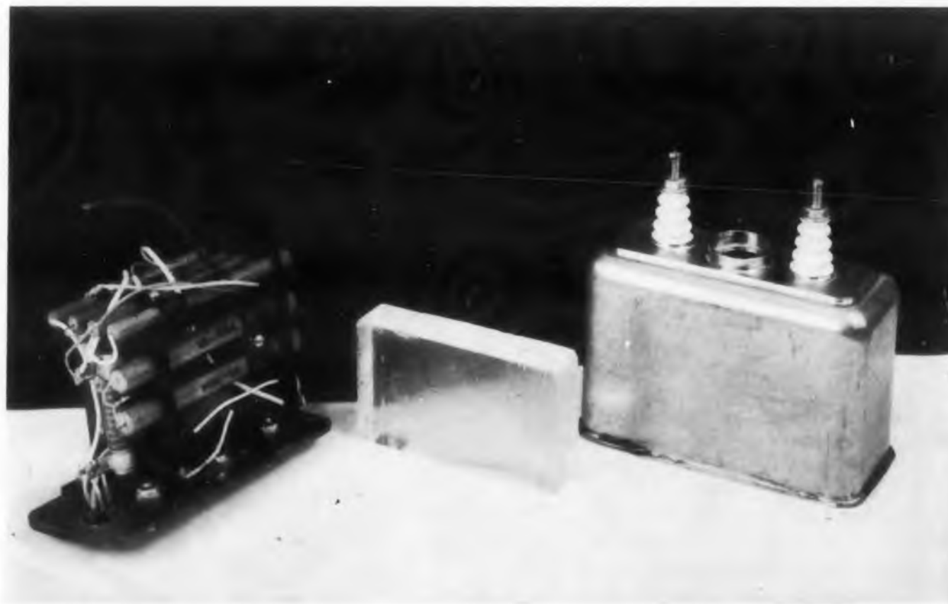
Fig. 1. Power supply (left) a block of polymerized vinyl silicone resin (center) and power supply cover can.
