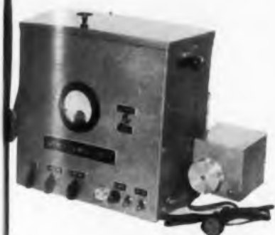
Instrument for fine wire measurements detects 0.000005 in. differences in diameters.
