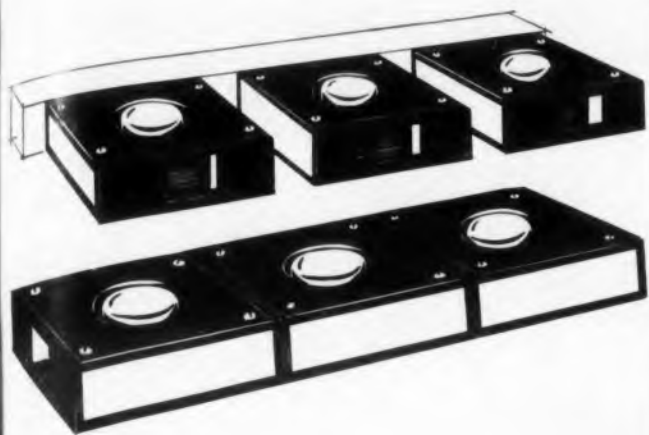
Fig. 3. Series (top) and parallel (bottom) mounting of exchangers. Calculation of air flow is the same as for current through resistors.
