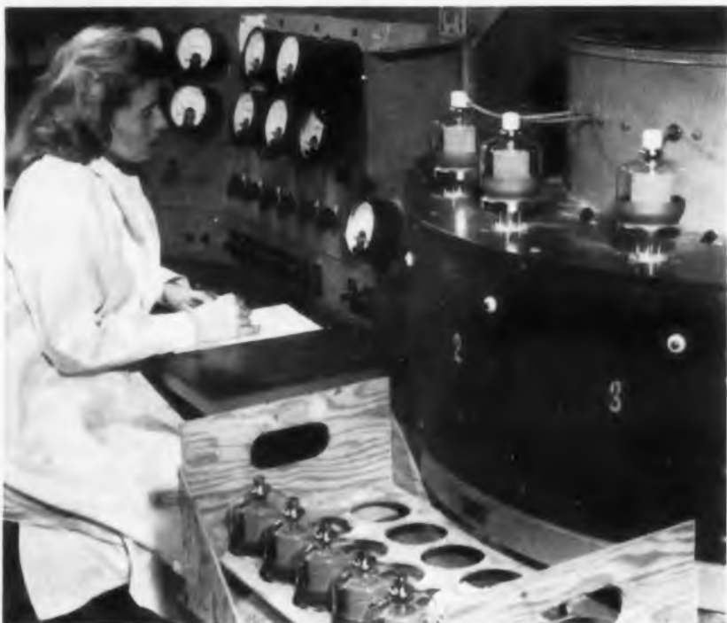
Every tube meets rigid Eimac specifications before shipment. On test consoles like this, dozens of electrical characteristics are patiently tested and recorded for each Eimac tube produced. Environmental testing equipment is also available for testing for severe applications.
