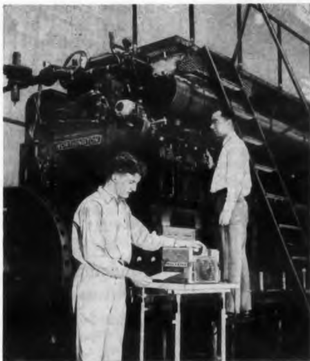
Ted Dupler (left) and John McAllister, Worthington Engine Research Engineers, measure intake manifold, cylinder, and exhaust manifold pressures and valve stroke on a Tri power with a Honeywell 906 Visicorder.
