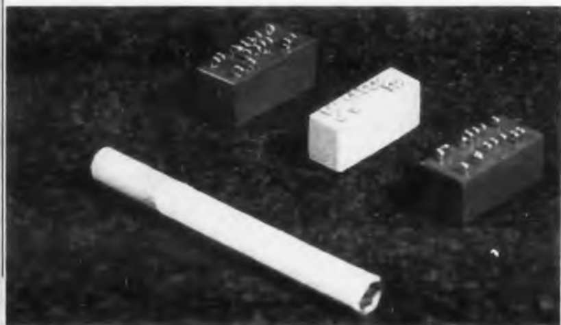
Fig. 1. These modular units will be part of the same assembly and should have the same dimensions. This results in more assembly flexibility.
