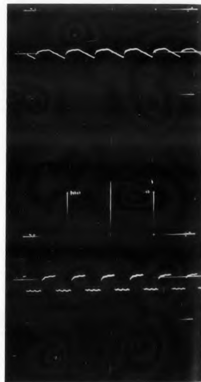
Fig. 2. Lower photo: power supply transient 10 cps squarewave. Upper photo: network output ripple to 200K load, capacitor 30 \mu f. (left)
