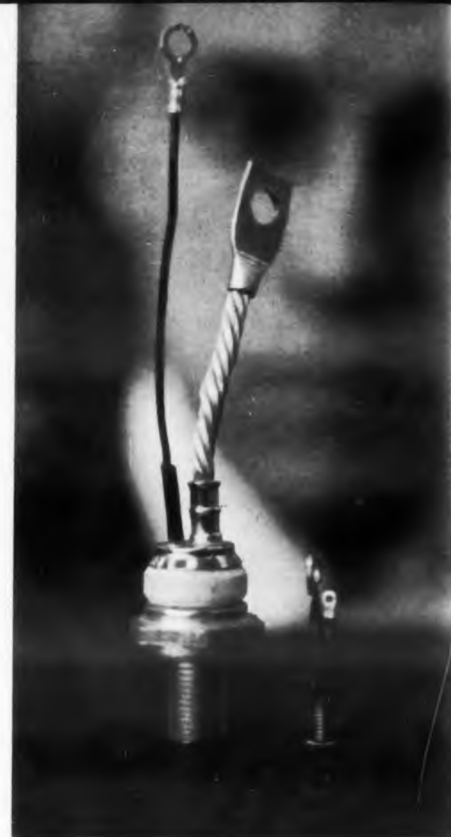
Currents as high as 50 amp can be controlled by as little as 15 ma with G. E.'s ZJ-50 silicon-controlled rectifier.
