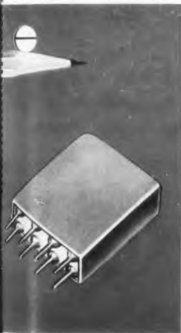
Epoxy's unique combination of dependable characteristics makes it suited to use in such equipment as totally enclosed motors, above; hermetically sealed relays, encapsulated dry-type transformers, below.
