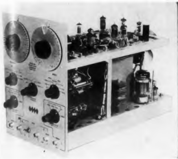
Compact pulse generator with the case removed.
