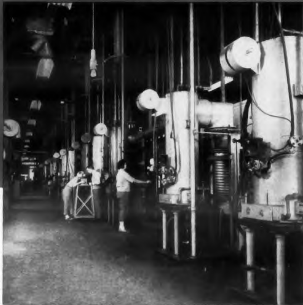
A battery of vacuum sintering furnaces, designed and built by Fansteel engineers, used in the production of Capacitor Grade Tantalum.
