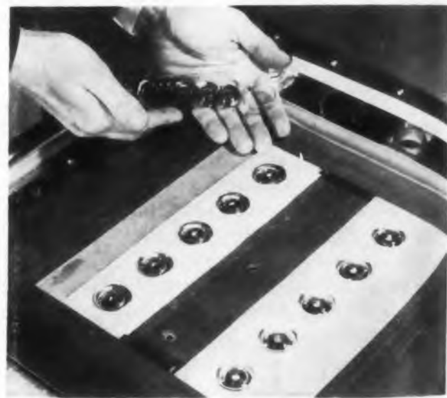
Packed in individual blisters, these bearings run far less risk of air contamination.
