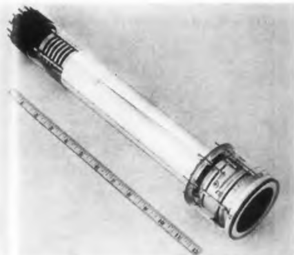
New orthicon is standard in configuration but gives better results in a specially adapted TV camera.
