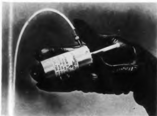
Cold end of compact cooler can chill infrared detector crystals to 195 C.
