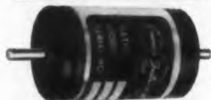
PRECISION MINIATURE SPEED REDUCER 1062. Standard ratios to 4000:1. Starting torque: .005 in.-oz.; Load torque: 25 in.-oz.; Backlash: 45 min. max.; Diameter: 1.062 in. Typical of many Bowmar designs currently being manufactured.
