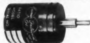
CONCENTRIC SHAFT SPEED REDUCER X-530. Single ended unit has optional internal slip clutch set to customer requirements. Most ratios available. Starting torque: .01 in.-oz.; Backlash: 30 min. max.; Diameter: 1.062 in. Typical of many Bowmar designs currently being manufactured.
