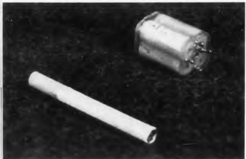
Fig. 2. Mounting of four capacitors as one unit saves assembly time and eliminates several solder connections.
