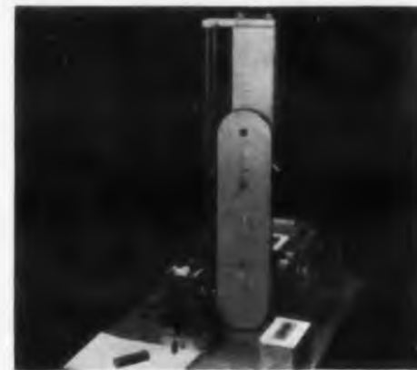
Synthane laboratory machine for measuring impact fatigue.
