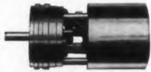
PRECISION SERVO MOTOR GEARHEAD 750-GH (with housing). Standard ratios to 2000:1; Starting torque: .005 in.-oz.; Load torque: 5 in.-oz.; Backlash: 30 min. max.; Diameter: .750 in. Typical of many Bowmar designs currently being manufactured.
