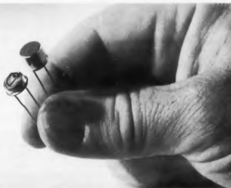
Up to 200 v can be switched on or off with Shockley Transistor Corp. four-layer diode, type AD.
