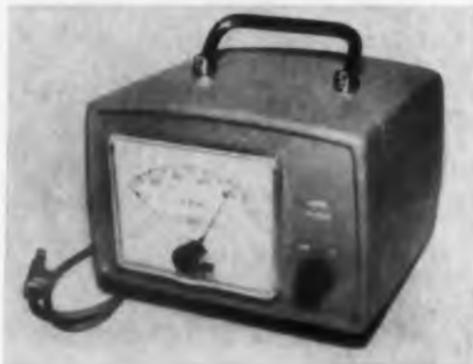
The series 7000 tachometer line has accuracies better than 1%. Types include multiple range, differential, expanded-range, control, and portable tachometers. Input signals may be supplied by electro-magnetic, photo-electric, and proximity pickups, tachometer generators, or turbine type flowmeters. Amplitude of the input signal may be as low as 0.005 v rms.
