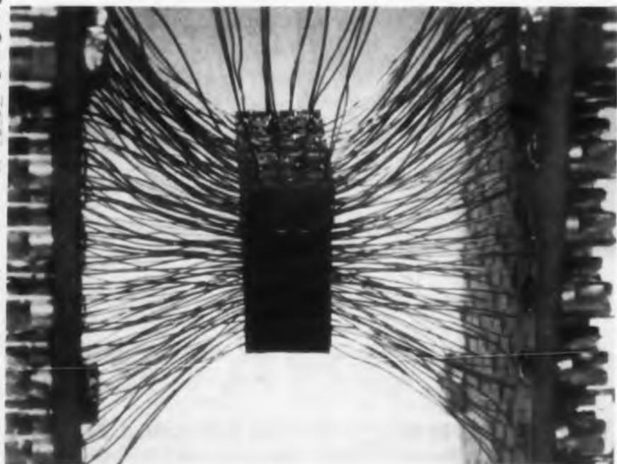
**A** COMPLETELY new memory element, the Biax was invented by Cravens L. Wanlass, Director of Research for Aeronutronic's Computer Operation. While the use of orthogonal magnetic fields for nondestructive readout has been explored by other people in the past—notably Thorenson and Arsenault of Magnavox Corp. during 1954-1957—Mr. Wanlass' application is the first practical device.
