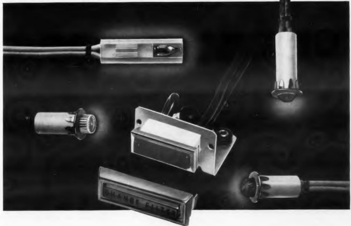
These are the smallest, low-cost complete assemblies on the market. The neon-filled lamps provide soft, steady illumination that is completely free from glare. With the bulb in series with a resistor for 115-230v. applications, neither transformers nor series hook-ups are necessary. Long, trouble-free operating life has been proved in thousands of the most demanding applications.
