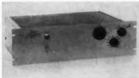
Power supply model 304 provides a continuously adjustable output of 500 to 2500 v at 25 ma. Load change is less than 0.002% for 0 to 25 ma output and regulation is 0.003% for line changes of 97 to 137. Ripple is less than 0.5 mv and stability is 0.01% per hr or 0.1% per day.
