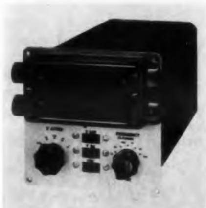
The model PIB2X10 general purpose Panelscope occupies 5-3/16 x 5-1/4 in. of panel and extends 10 in. behind. It features 100 mv rms sensitivity, a dc to 1 mc bandwidth, and a repetitive sweep continuously variable from 10 cps to 20 kc. Compensated attenuator steps of 1, 10, 100, and 1000 together with a 10 to 1 nonfrequency discriminating vernier provide a 10,000 to 1 continuously variable attenuation range. The unit contains its own
