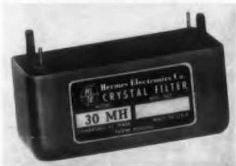
Models 30 MH, 30 MJ, 30 MK, and 30 MP crystal filters have center frequencies of 30 mc and 6 db bandwidths of 125, 40, 25, and 5 kc respectively. Maximum insertion loss is 3 db. Case sizes are 3-1/32 x 1-7/16 x 1 in. for model 30 MH and 2-3/8 x 1 x 1-1/32 in. for the remaining three.
