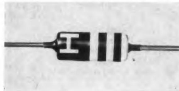
Designed for computer switching applications, these miniature silicon diodes have a maximum recovery time of 0.3 or 0.5  $\mu$ sec, depending upon the model. Minimum forward currents at 1 v and 25 C are from 6 to 200 ma. Hermetically sealed in glass envelopes with a maximum length of 0.265 in. and a maximum diameter of 0.107 in., the units have a -65 to +150 C operating range and a -65 to +200 C storage range.
