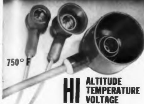
This is a new series of Tube Cap Connectors using special silicone components for high reliability applications. They provide the highest degree of resistance to temperature extremes and are virtually unaffected by ozone and corona. The excellent dielectric characteristics make them ideal for high voltage. Skirts and sealed-in leads guard against flashover at high altitudes. Additional features include anti-corona cup and long-life spring contacts.
