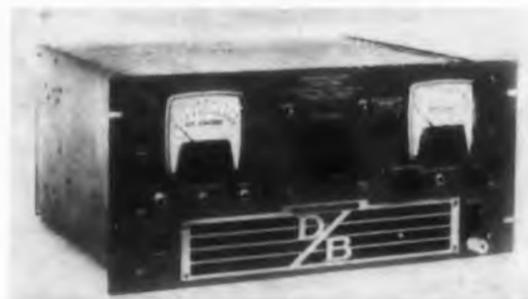
For laboratory use, these dc power supply models 62-141 and 62-142 provide 0.5 to 32 v dc at 0 to 5 and 0 to 10 amp, respectively. Line and load regulation are less than 18 mv, ripple is less than 1 mv, and load transients are less than 200 mv.
