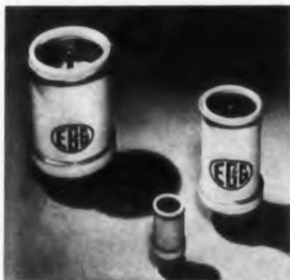
Miniature model HY-1 and 632 ceramic-metal hydrogen thyatron tubes have respective ratings of 5 megawatts, 20 kv, 500 amp peak and 67.5 kw, 3 kv, 45 amp peak.
