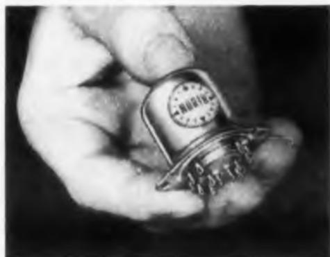
Available in a variety of contact ratings for ac, dc, and dry circuit operation, these miniature four and six pole relays exceed the requirements of MIL-R-5757A, B, and C and MIL-R-25018. They incorporate balanced rotary motors for shock and vibration resistance, stepped headers for easy wiring and inspection, and Teflon spatter shields to prevent contact shorting. The units are hermetically sealed in a 1.176 in. diam. corrosion resistant can that stands 1.272 in. above the mounting plane.
