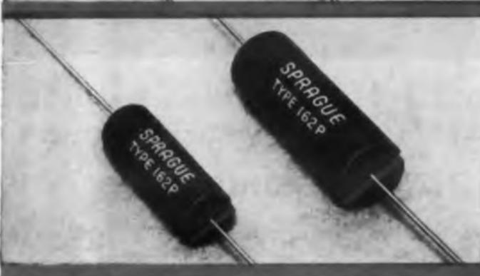
**NEW!**... DIFILM Type 162P slotted-base multi-purpose molded case capacitors for auto radios and other severe vibration applications. Slot prevents collection of moisture around leads when capacitor is end-mounted against chassis.
