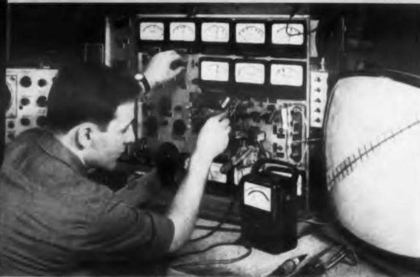
Photo courtesy of Admiral Corp. Engineer shown is using the Model 270 in evaluating operating characteristics of developmental type deflection tube.
