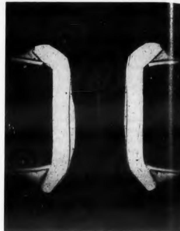
Fig. 5. This shows an experimental eyelet of insufficient length, which caused delamination of the conductor.
