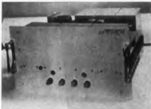
For precision test use, programmable power supply models PS-32, PS-33, and PS-34 operate from a programmed source such as a magnetic tape reader or punched card, or by manual selection from panel buttons. They furnish a voltage that is accurate within 0.1% and regulated within 0.1% from no load to full load. Voltage ranges are 6 to 36 v dc in 0.1 v steps at 30 amp for the PS-32, 1 to 500 v dc in 1 v steps at 1 amp for the PS-33, and 0 to 99.9 v dc in 0.1 v steps at 1.5 amp for the PS-34.
