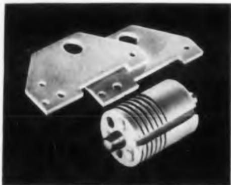
accuracy of ±.001 and the hole spacing is held to a tolerance of ±.002. The drum with its stainless steel bearing sleeves is a direct ceramic-to-metal assembly. The bearings must withstand a vertical load of 60 lbs. Three of the end holes are tapped. The slot, the pitch and the depth of the spiral winding groove are ground to tolerances of ±.001.
