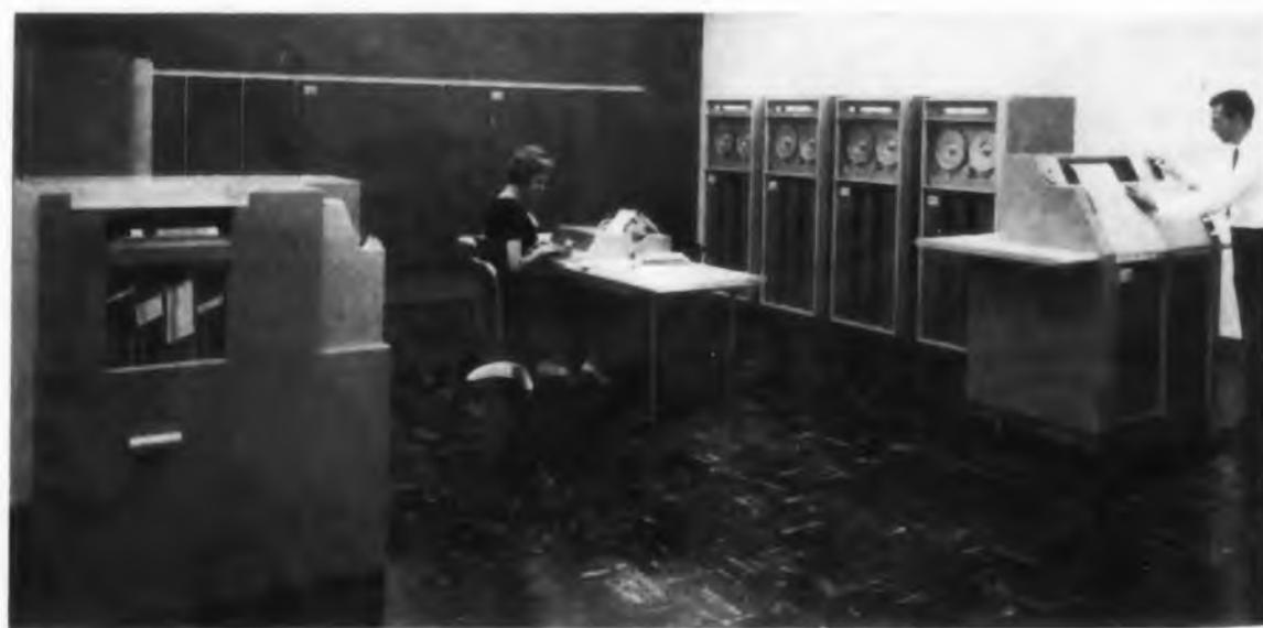
Henry Dreyfus-styled, all-transistorized computer is shown in medium-size configuration. Honeywell's Datamatic Div. expects to start delivering the highly touted unit in October, 1960. According to the company, the 800 can handle up to eight separate computations simultaneously.
