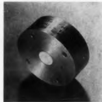
Designed to improve the performance of a klystron excited system, the model IKuL4 ferrite isolator provides a minimum of 25 db isolation from 16 to 17 kmc with a 0.45 db maximum insertion loss and a 1.12 maximum vswr. Rated at 5 w average power, the unit is 0.66 in. long and weighs 2.9 oz.
