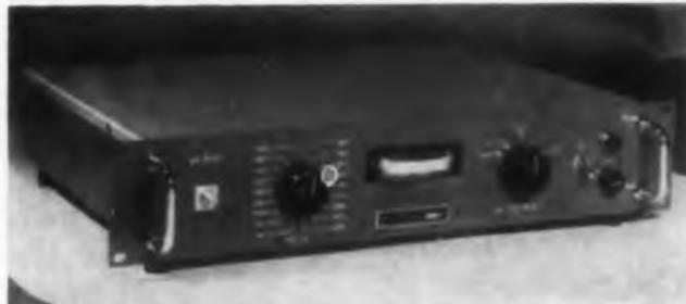
From a 117 v, 60 cps, single phase input, the model 409 nuclear power supply provides an output of 170 to 1530 v dc at 0 to 5 ma. It has a selective polarity, 0.02% stability, and less than 0.002% ripple. Regulation is within 0.01% for 10 v line changes, within 0.4% for 1 ma load changes. The unit is 19 x 3-1/2 x 12 in. and weighs 22 lb.
