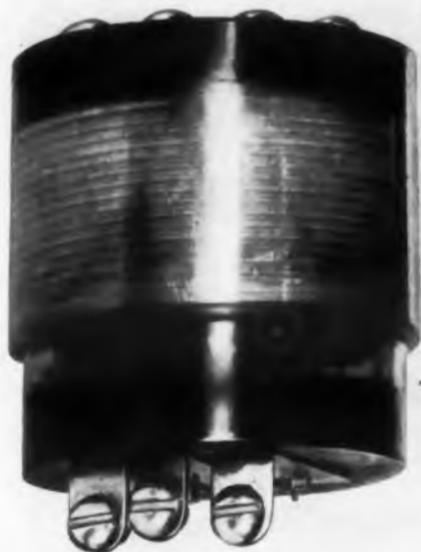
Chemical control unit for static switching is size of 1.5-inches cube, can handle from 3 to 70 v ac at 4 amp with no internal wear.
