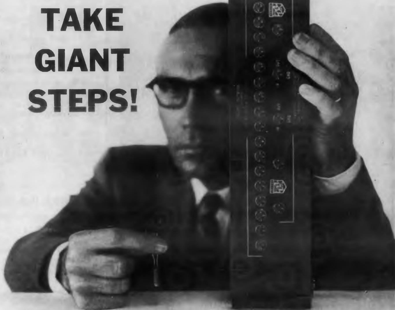
From the smallest to the largest—.005  $\mu$ sec. to 5,000  $\mu$ sec.—ESC's research staff has custom-designed delay lines for virtually every military and commercial application! And with every delay line prototype comes a comprehensive laboratory report, which includes submitted electrical requirements, photo-oscillograms (which indicate input and output pulse shape and output rise-time), the test equipment used, and an evalu-
