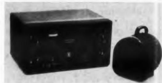
The model RS-8B OptiTherm infrared radiation source is designed to emit black body radiation over a 200 to 1000 C range. The source temperature, selected with a precisely calibrated single control dial, is maintained within  $\pm 0.3$  C despite ambient temperature changes, line voltage variations and transients, tube aging, and individual component replacements.
