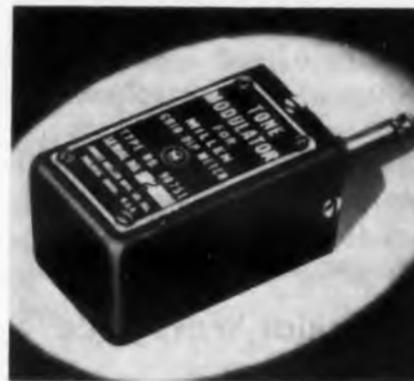
Containing a transistor oscillator with a mercury battery, the model 90751 transistor tone modulator plugs into the phone jack of a grid dip meter to modulate the signal at about 800 cps. The modulator is automatically turned on when it is plugged in.
