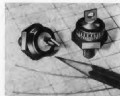
Rated 25 to 35 amp and 50 to 500 piv, these Quad-Sealed silicon power rectifiers have a four layer seal which makes them resistant to humidity, shock, vibration, temperature, and other environmental extremes. An oversized anode lug removes heat from the rectifier junction, allowing the unit to withstand high peak current surges. Full cycle average leakage current is 10 ma at 130 C base temperature. The anode lug has eyelets for easy wiring.
