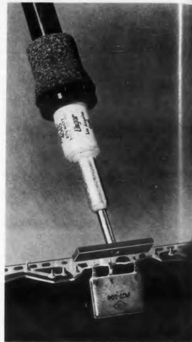
Bar tips remove straight line components.
