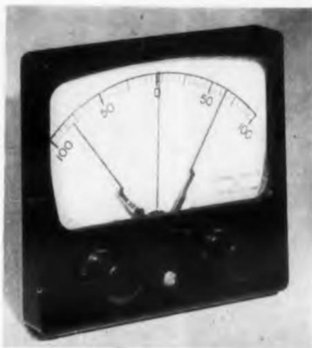
**Fig. 1.** Contacts in meter-relays can be either non-locking or locking. It is generally agreed that the locking type is the most reliable.
