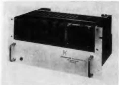
Core storage buffer models 144-BQ8A and 144-BA8A are designed for applications requiring an auxiliary memory to synchronize two data systems. They have a capacity of 144 8-bit characters and a 115 v 0.5 amp, 60 cps self-contained power supply that is unaffected by 100 to 130 v line variations. Loading and unloading occur at a rate of 100,000 characters per sec. Bits are loaded and unloaded in parallel, characters in sequence. The units operate best from 0 to 40 C and derate at 55 C.
