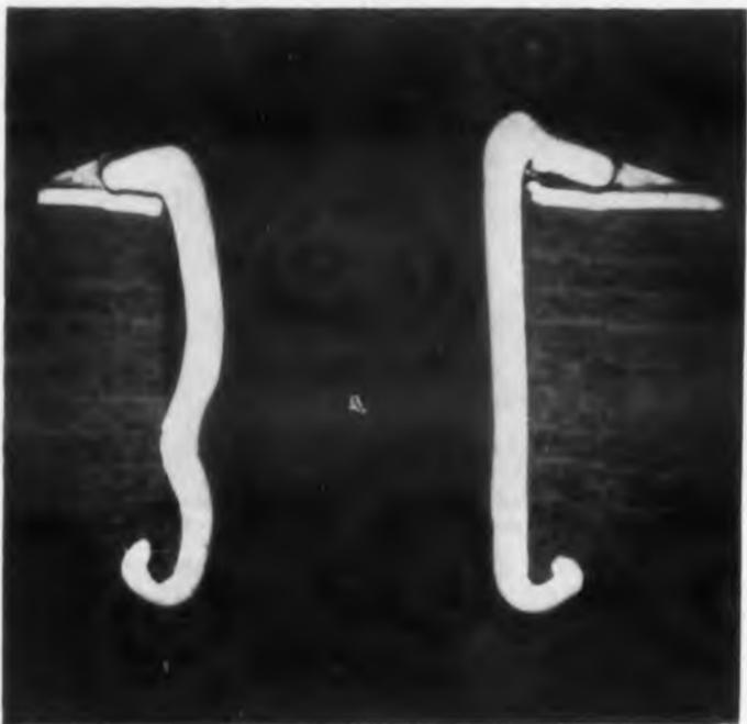
Fig. 3. Excessive pressures of normal riveting practices cause distortion of the eyelet (left).
