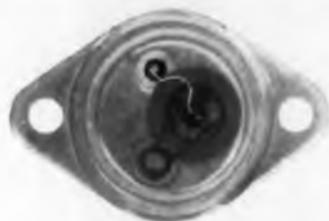
Low  $R_{CS}$  (0.05 $\Omega$ ) at high temperatures insured by large ring emitter-base area. Leakage currents minimized by all welded construction . . . no contaminating solders or fluxes used!
