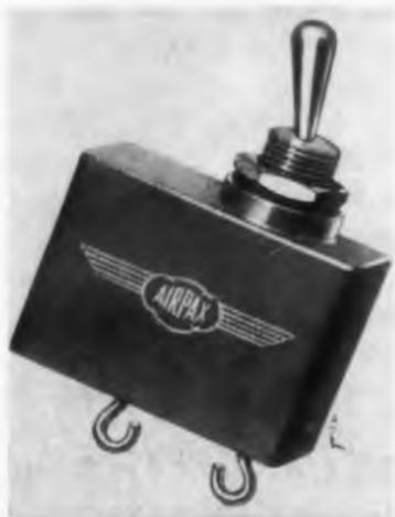
Miniature series 500 circuit breakers are electromagnetic, inverse time delay units that resist 100 g shock. Their trip level is 125% of rated current, independent of ambient or operating temperature. Units are available for interrupting 50 v dc at 0.05 to 10 amp or 120 v rms, 60 to 400 cps at 1 to 10 amp. They are provided with a short delay for protecting electronic equipment or a long one for protecting devices with
