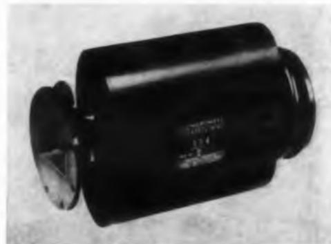
This liquid-cooled, high power ferrite load isolator, model MA-154, is used in radar systems operating in the 2700-2900 mc range. It operates at 5 megawatts peak and 400 w average power. Insertion loss is less than 0.4 db; isolation is 10 lb minimum. It weighs 50 lb and is 12 x 8 x 3-1/2 in. Ratings apply over an ambient temperature range of 0 to 65 C.
