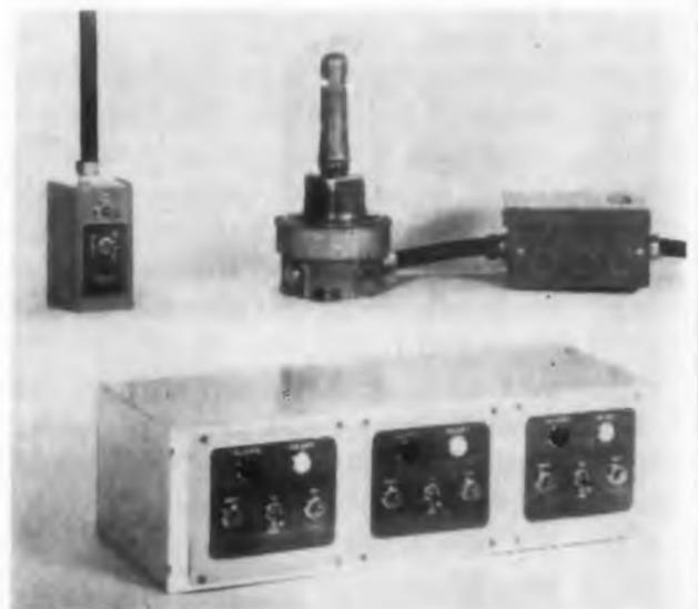
**SWAMI intrusion detector** (for Standing Wave Area Motion Indicator) consists of sensor (right, rear), Day-Night control box, (left, rear), and monitor unit. Uhf signals are used in radar-like fashion to keep an area under surveillance.
