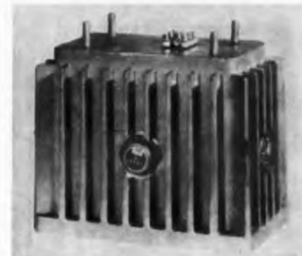
The SE series power supplies deliver 30 w with germanium transistors. Rated at 12 v from 0 to 3 amp continuous duty, the units have a voltage regulation of  $\pm 0.1\%$  for both line and load. Ripple is 2 mv peak to peak and the units can be operated for moderate periods without cooling at ambients of 105 F. Immersion-proof, the units weigh about 6 lb and measure 4-1/4 x 7 x 6 in.
