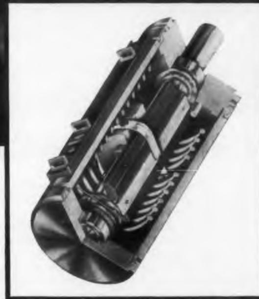
**THE PROBLEM:** A small, multi-turn potentiometer was required for the "black box" in the Thor missile which had to withstand severe environmental conditions, and have characteristics of low noise with no discontinuity under vibration, shock and acceleration.
