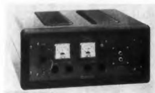
Permanent magnet focused twt amplifier model TA 36PM is a light compact unit for 0.5 to 1 kmc operation. It provides 0.1% regulation with a maximum ripple on the helix of less than 10 mv. Designed for relay rack or cabinet mounting, the unit has front panel metering for helix voltage, helix current, and beam current.
