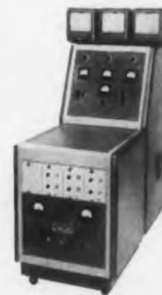
**DIFFERENTIAL WATTMETER** High precision test detection of extremely small power consumption differentials in gyro spin motors and other types of rotating components.
