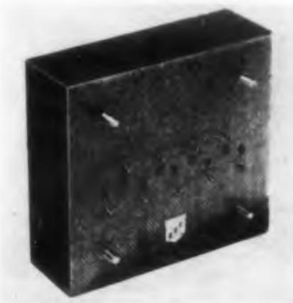
In a single  $3 \times 2\frac{7}{8} \times 1$  in. unit, the model 71-30 incorporates four separate delay lines, each with a 1  $\mu\text{sec}$  delay and a 1 K characteristic impedance. The device is cased in molded epoxy and has a glass melamine board with gold plated pins. Suitable for printed circuit applications, it is particularly adaptable to dip soldering techniques.
