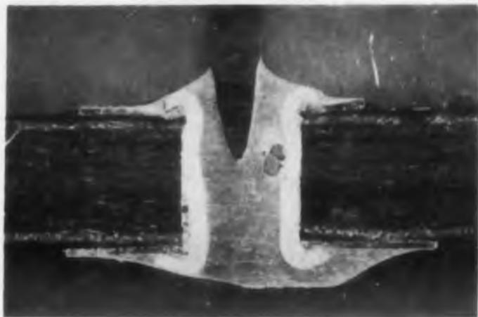
Fig. 1. Under the microscope an eyelet magnified at 20X shows no flaw.
