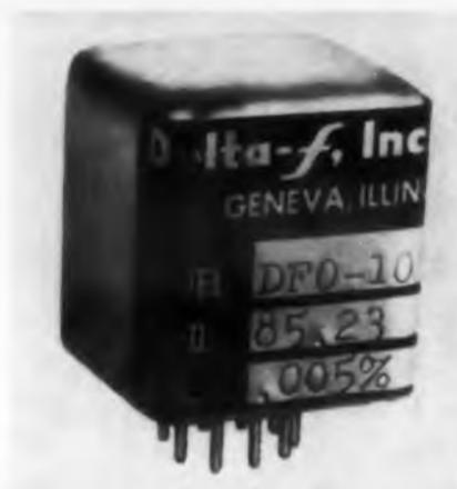
Available at any frequency from 3 to 100 mc, the DFO-10 transistorized crystal oscillator is  $1 \times 1 \times 1\frac{1}{8}$  in. and provides 0.0005% frequency stability from  $-55$  to  $+90$  C. The circuit is completely encapsulated with Silastic RTV 501 for operation under extreme vibration and shock. Output power is 0.1 mw minimum; load impedance is 50 ohms standard and up to 600 ohms on special order; and supply voltage is 20 to 30 v as specified.
