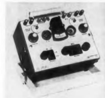
Impedance bridge model 502-A has ratio ranges that extend to 120 billion to 1 for resistance and 12 billion to 1 for capacitance and inductance. It measures 6 x 7 x 9 in., weighs 10 lb. and has direct reading controls.
