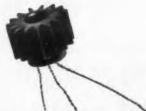
FOR MOST JETEC 30 TRANSISTORS (Jetec Outline TO-9)
