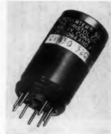
Miniature chopper model C1430 has a dry circuit to 100 v contact rating and less than  $1 \mu\text{v}$  thermal drift. The unit is resistant to shock and vibration and is available in plug-in models or in two-hole, four-hole, side, or clamp mounting types. Temperatures from  $-65$  to  $+125$  C have negligible effect on phase angle.
