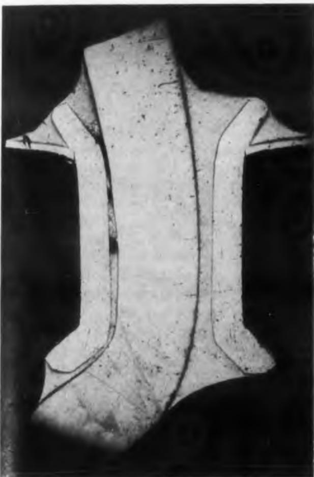
Fig. 7. This shows another sample of an experimental eyelet, showing large solder area and the component lead.
