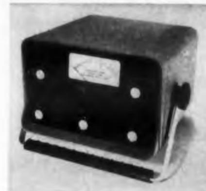
Portable, battery powered model T-1A vibration meter provides direct readings of the velocity, displacement amplitude, and acceleration components of vibration. Frequency can be determined by a simple computation. The unit can accept up to six simultaneous transducer outputs, three for velocity type pickups and three for crystal accelerometers. It provides readings of up to 1000 g acceleration, 0.01 to 100 ips velocity, and 0.001 to 10 in. displacement. Overall accuracy is better than 5%.
