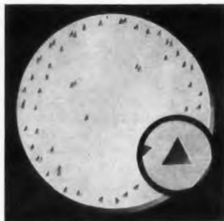
Dislocation density, Knapic silicon monocrystals. Crystal diameter 1/10" to 3/8"—None; 3/8" to 3/4"—less than 10 per sq. cm.; 3/4" to 1-1/4"—less than 100 per sq. cm.; 1-1/2" to 2" less than 1000 per sq. cm.
