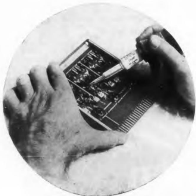
**Slotted de-soldering tip** is used to remove small components. It can also straighten folded or bent socket tabs.
