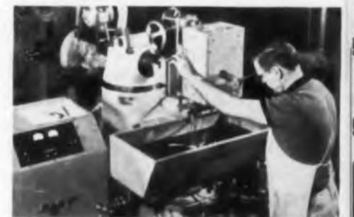
Metal disintegration, a fast, economical way Synthane uses to produce or revise dies.
