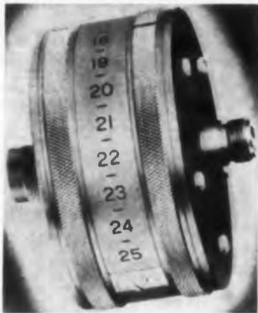
Model S-200 radial double-stub tuner covers 100 to 2000 mc range. The rotating tuning rings of the unit give calibration references from 0 to 25 and the double-stub provides adjustment of 12.6 in., with 1.9 in. spacing. Characteristic impedance is 50 ohms. The unit weighs 2 lb and measures 3-3/8 x 4 in.
