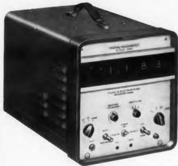
Model 520 . . . manual range switching AC, DC, OHMS . . . Rack or portable.
