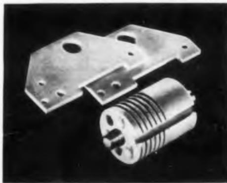
accuracy of  $\pm .001$  and the hole spacing is held to a tolerance of  $\pm .002$ . The drum with its stainless steel bearing sleeves is a direct ceramic-to-metal assembly. The bearings must withstand a vertical load of 60 lbs. Three of the end holes are tapped. The slot, the pitch and the depth of the spiral winding groove are ground to tolerances of  $\pm .001$ .
