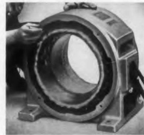
**Extended service life for motors** through RTV encapsulation of stator windings, introduced by General Electric motor departments. RTV's resistance to moisture and other contaminants enables these dripproof motors to meet certain applications formerly requiring totally enclosed units. RTV has low viscosity, rapid cure.
