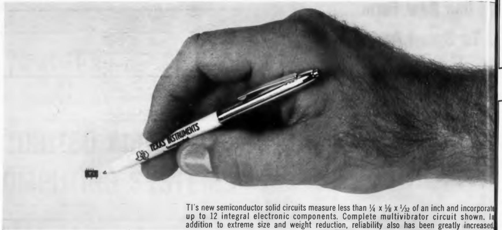
TI's new semiconductor solid circuits measure less than  $\frac{1}{4} \times \frac{1}{8} \times \frac{1}{32}$  of an inch and incorporate up to 12 integral electronic components. Complete multivibrator circuit shown. In addition to extreme size and weight reduction, reliability also has been greatly increased.
