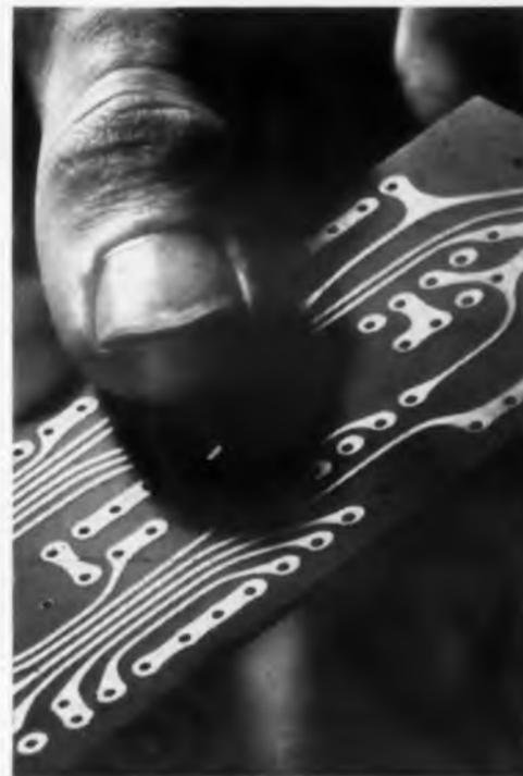
**FOTOCERAM,<sup>®</sup> an unusual new printed circuit board** We've resoldered more than fifty times on this board without damage to circuit runs or through-hole holes. No adhesives needed to bond copper to board. Bond strength between Fotoceram and metal is 15 to 20 lbs., when 1" strip is pulled perpendicular to board. Takes over 60 g vibration shock. All electrical properties equally outstanding.
