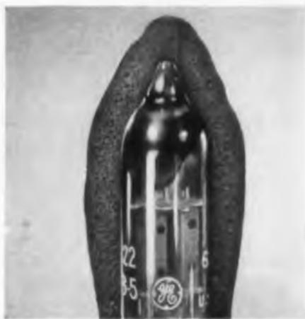
**New resilient, shock-absorbent RTV sponge** offers improved shock and vibration protection at elevated temperatures; permits easier fabrication than previous methods of cutting, inserting and sealing sponge in place. With RTV, just add sponging and curing agents to compound and mix.
