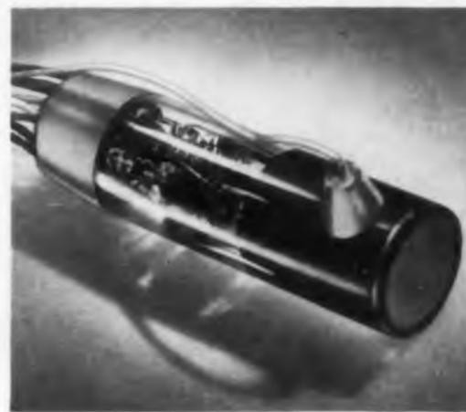
**Protection from high altitude arc-over and corona** is provided for this cathode ray tube by encapsulating all lead wires with RTV (room temperature vulcanizing) silicone rubber. Designed for airborne operation and installed in a non-pressurized section of the aircraft, tube is protected from arc-over and corona at altitudes up to 70,000 feet.
