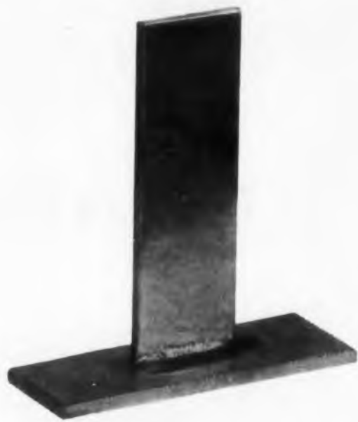
Fig. 1. Typical sample used in the tensile testing of the aluminum solder joints. Joint section is 1 \times \frac{1}{8} in.
