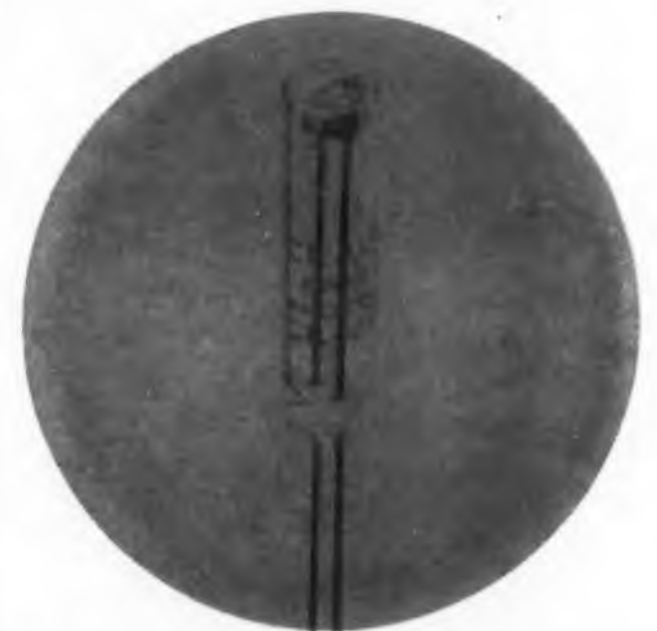
Fig. 2. Small size and weight is one advantage of photoconductive cells. This is one packaging method.
