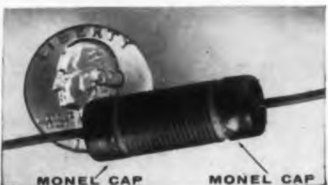
Close-up of Monel caps soundly brazed to wire winding and leads of semi-finished resistor. Made by Sage Electronics Corporation, 302 N. Goodman St., Rochester 7, N. Y.
