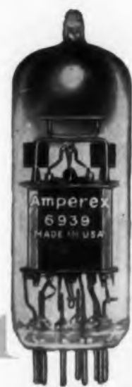
Amperex 6939 5 watts total anode dissipation
