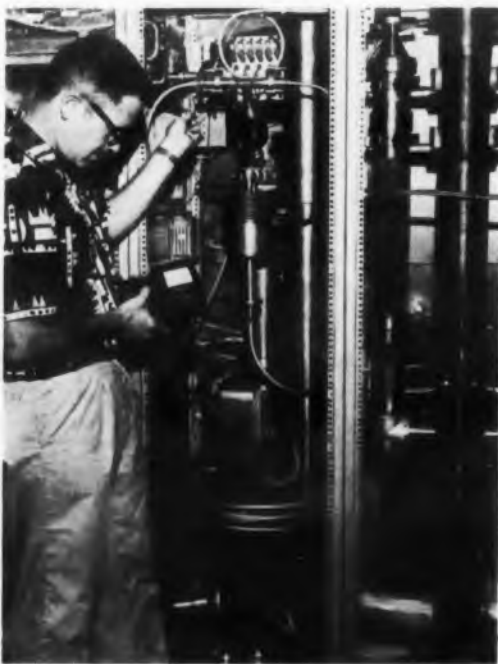
Fig. 2. David Russell adjusts the "magic T" input to the detector of the new NBS high-frequency piston attenuator developed by the Radio Standards Laboratory. The attenuator itself is in the Electronic Calibration Center. On the right is the large trombone phase shifter used in this dual-channel system.
