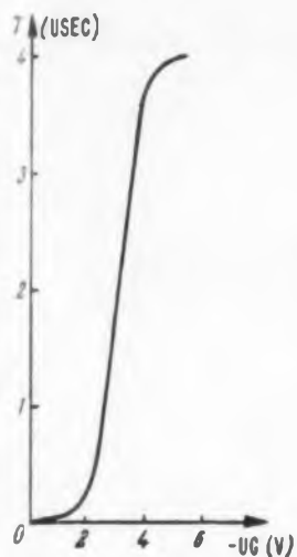
Fig. 2. Pulse duration of the multivibrator can be varied by changing the grid voltage on the control tube.
