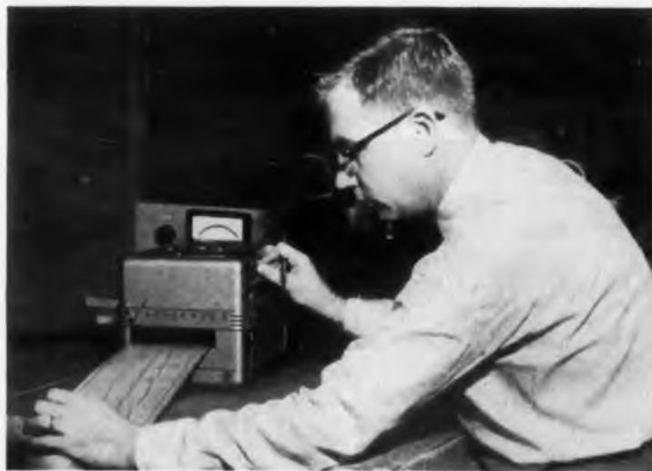
Byron Phillips, U. S. Weather Bureau Scientist, monitors thunderstorm data as it is recorded by the Honeywell Model 906 Visicorder.
