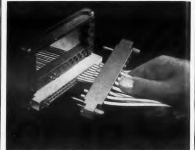
Both inner and outer contacts are crimped to the conductors, simplifying a previously complicated and difficult process. In addition this process eliminates many of the parts formerly used, and also eliminates any heat in the connection process. The result is a reliable coax connection, easily and quickly installed.
