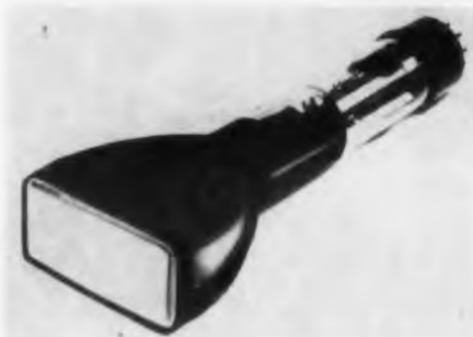
Having a 3-in. rectangular face-plate, type 3BDP cathode ray tube is for oscilloscope applications. An improved replacement for type 3SP, it has a pressed face-plate to minimize parallax errors and a gun structure which provides greater rigidity and improved electrical stability. Focus and deflection are electrostatic. Over-all length is 9 1/8 in.
