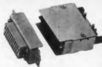
Four prong retention springs on pin and socket allow each contact to snap into insulator blocks easily, yet resist an axial pull of more than 20 lb. Inspection holes provide built-in quality control, permit visual checking of each wire for proper contact prior to assembly of connector.
