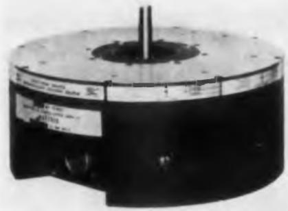
Type RD-17 photoelectric shaft-position encoder gives angular position data in 17-digit cyclic binary code with  $\pm 1$  digit accuracy. The 17-digit accuracy for 1 shaft revolution is obtained in unambiguous form without the use of gears. Designed to meet applicable portions of MIL-E-4158B, the 26-lb, 10-in. diam unit includes power supplies, amplifiers and control electronics. Solid or hollow shaft models are available.
