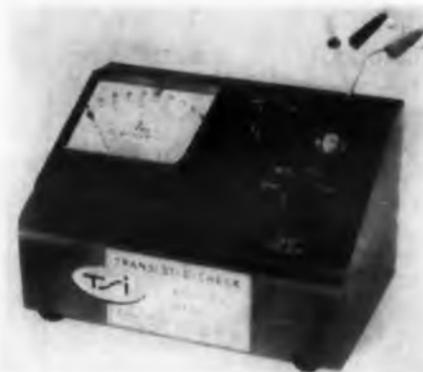
Model 902 transistor tester covers a beta range of 0 to 200;  $I_{CBO}$  is from 0 to 50  $\mu$ a, and  $I_{CEO}$  is from 0 to 5 ma. Battery operated, the instrument performs tests at a constant collector voltage of 6 v. Designed to meet laboratory as well as production requirements, it is completely self-contained and incorporates a 50- $\mu$ a meter for direct reading of current. All functions are controlled by two switches.
