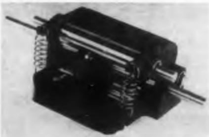
Model 031-2000 mechanical integrator has an output torque of 1 oz-in. max with a disc input torque (no load) of 0.33 oz-in. The unit weighs 6.5 oz and has a ball displacement of  $\pm 0.750$  in. It may be used as a breadboard item, or as a component in computing systems.
