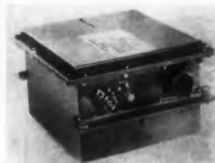
Suitable for telemetering use in missiles, model 6173 silver-zinc battery has 19 15-amp-hr cells for high voltage and 5 10-amp-hr cells for filament power. When discharged at the 7-min rate, the sections yield 90 and 60 amp, respectively. At 30 min, the sections offer 30 and 20 amp respectively. Normal discharge voltages are 28.5 and 7.5 v. Operating temperature range is 0 to 100 F, shelf life is 2 yr, and the battery can be recharged 20 times. It weighs 23 lb and measures 5.5 x 7.5 x 8 in.
