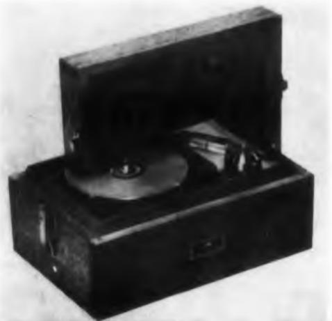
Model 4290 calibration exciter vibrates accelerometers or other small vibration pick-ups at a constant test level over the frequency range of 50 to 30,000 cps. A small accelerometer acts as a monitor for servo regulations of the driving signal generator to obtain the constant level of vibration. Used with model 3301 response recorder, it automatically measures and plots an accelerometer frequency response calibration from 200 to 20,000 cps and indicates mounted resonance up to 50,000 cps.
