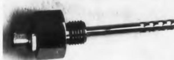
Able to stand an operating pressure of 5000 psi, type BA-9 temperature transducers have a resistance range of 50 to 5000 ohms at 77 F  $\pm 4\%$ . Response is 0.25 sec in fluid and repeatability is 0.5%. They can be supplied with a Balco element, or with platinum or tungsten.
