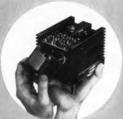
Designed primarily as a component power supply, units are widely used in computers, electronic instrumentation, production test equipment, and quality control check out systems. Best of all, the unique design makes these units available at the lowest possible cost to you.
