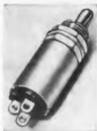
When it comes to making a *real* saving in space, this new SP-DT Hetherington Toggle Switch is the answer. It is only  $1\frac{1}{2}$ " in diameter by  $1\frac{1}{2}$ " long. It weighs less than  $\frac{1}{4}$  oz. Yet it breaks 5 amp. resistive loads at 28 volts dc ( $2\frac{1}{2}$  amps @ 115 v ac) for 50,000 operations.
