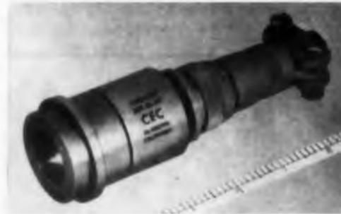
Available in pressure ranges from 0-100 to 5000 psi, gage and absolute, type 4-327 transducer has the pressure-sensitive diaphragm flush-mounted. Provision is made for adjustment of bridge balance, temperature compensation, and sensitivity external to the unbonded strain gage sensing element. It may be used in missile test stands, aircraft and missile engine test cells, and nuclear reactors.
