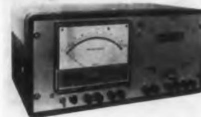
For measurements at sustained accuracy and resolution down to 0.01% of rated input, model 1483 electronic wattmeter provides a low impedance dc output. It can be used to actuate digital meters and to drive strip-chart recorders. Ranges are 250, 500 and 1000 w. Input is 5 amp normal and 10 amp max. The unit measures about 20 x 14 x 10 in., and approximate weight is 27 lb.
