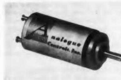
Designed to meet the environmental requirements of MIL-E-5272B and NAS 710, model 0610M multiturn potentiometer measures 1/2 in. in diam. It has a stop torque-limit of 25 oz-in. Operating temperature range is from  $-55$  to  $+125$  C. It is available with a linearity to 0.05%.
