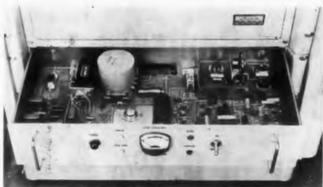
**Cyclelock tape** speed-control system holds timing accuracy to  $\pm 0.005$  per cent, according to designers, Mincom Div. of Minnesota Mining and Manufacturing Co.
