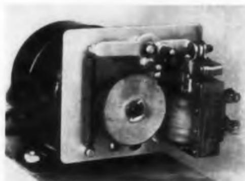
Designed for fhp motors, this precision brake is useful in computer mechanisms, tape transports, and other mechanisms where positive stop is necessary. Braking torque is 2 to 4 lb/in. for shafts to 3/8 in. All parts, including the brake band, are made with special dies to eliminate variations in braking power. A constant duty solenoid is furnished for connection in parallel with the motor. Without load the motor is stopped in less than 1/4 revolution.
