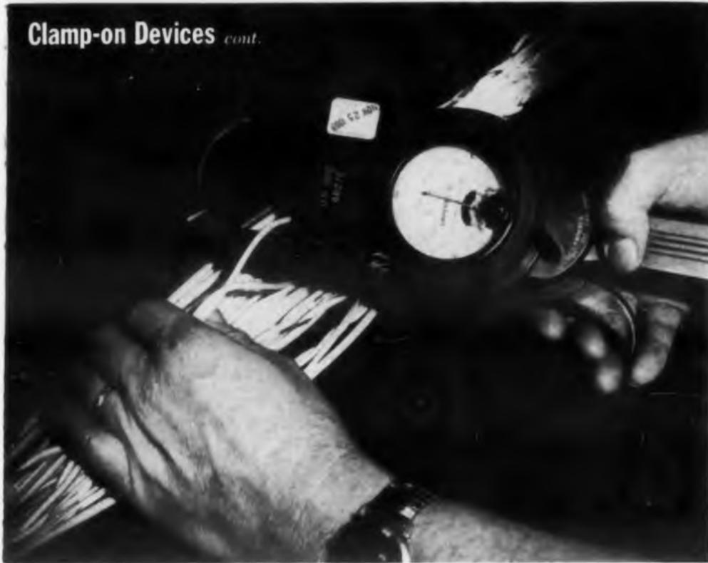
**Fig. 2.** Only a few minutes time is required to locate current carrying wires using a clamp-on ammeter.
