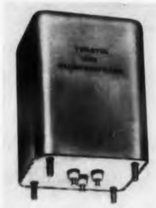
For use with multiplex systems, this line of standard-tone filters has 21 channels. The filters have high interchannel attenuation and flat pass band characteristics. They conform to Mil specs. Telemetering filters, from 400 to 70,000 cps, can also be furnished.
