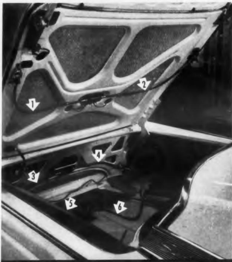
In the Ford Fairlane 500 Skyliner, the roof retracts into the trunk, and the trunk lid closes and locks. All this is done automatically, within 40 seconds. Powering this ingenious mechanism are six 3/16" high speed, remote control flexible shafts, driven by three reversible electric motors.
