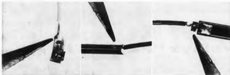
This beryllium-copper clip must exert a constant pressure against the potentiometer element. Too much heat in attaching the lead to it would destroy the spring temper, impair the accuracy of the instrument. Weldmatic's millisecond welding pulse solves the heat problem completely.
