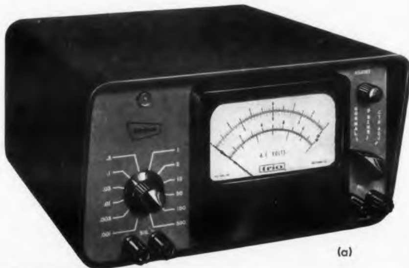
Fig. 2. Silk screening on small areas requiring much linework is impractical. For this type application, the use of an adhesive sticker is preferable.
