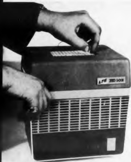
Compact disk memory fills only a 9-in. cube, weighs about 15 lb.
