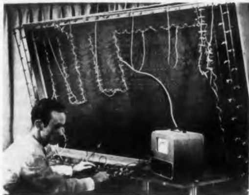
Fig. 8. The resistance network is mounted on the back of a large board of insulating material. The electrode configuration of Fig. 7 is outlined with lengths of copper wire attached to the appropriate contact points.
