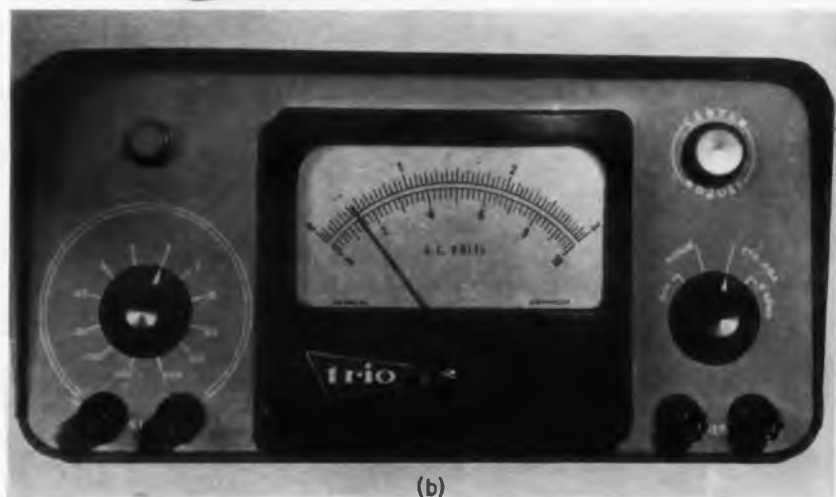
Fig. 4. By applying a circular pattern to unite lettering details to specific controls, as shown in (b), improved appearance together with a reduction of potential operator confusion are achieved.
