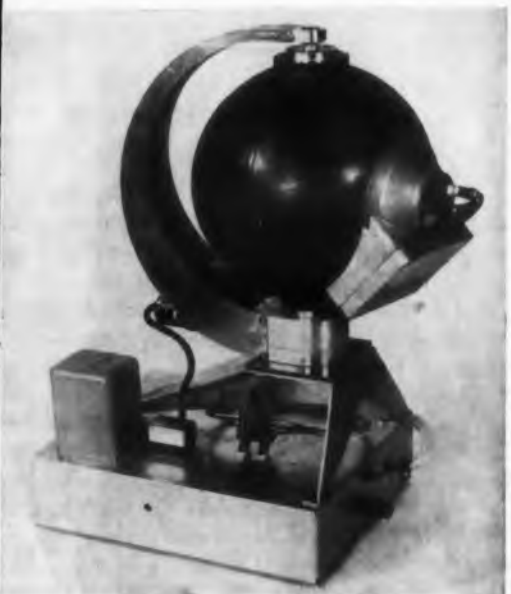
Passive reflector for drone radar augmentation combines the Luneberg and the Eaton-Lipman lenses. Bi-static and mono-static reflection are achieved in this Dalmo-Victor reflector.
