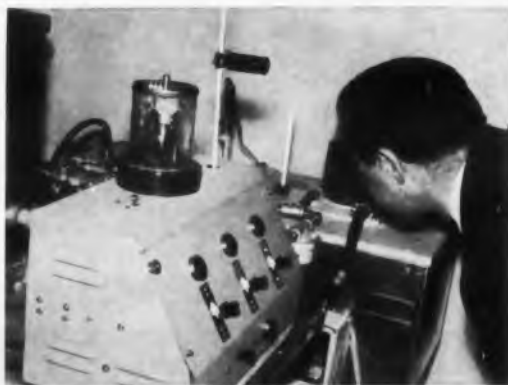
Staff engineer Reuben Wechsler, of E.I.A.'s Standards Lab, checks test setup for thermal resistance check of transistors. Other projects at the Standards Lab include test evaluations for slow- and high-speed diode reverse recovery tests.
