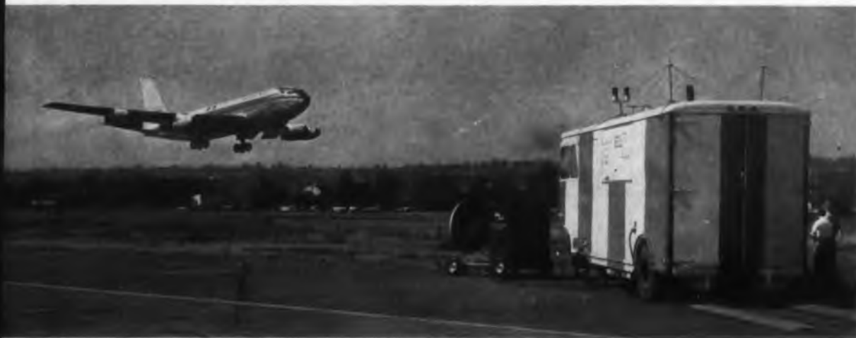
Sign of things to come? Boeing 707 is landed automatically with Bel Avionics' AN/GSN-5 landing system. The system, one of several being tested by the FAA, uses a computer to calculate flight paths. Computations are based on data input of precision tracking radar. Radio link carries corrective commands.
