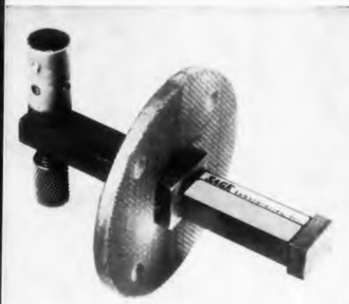
Fig. 2. Detector holder used as basis for receiver horn.
