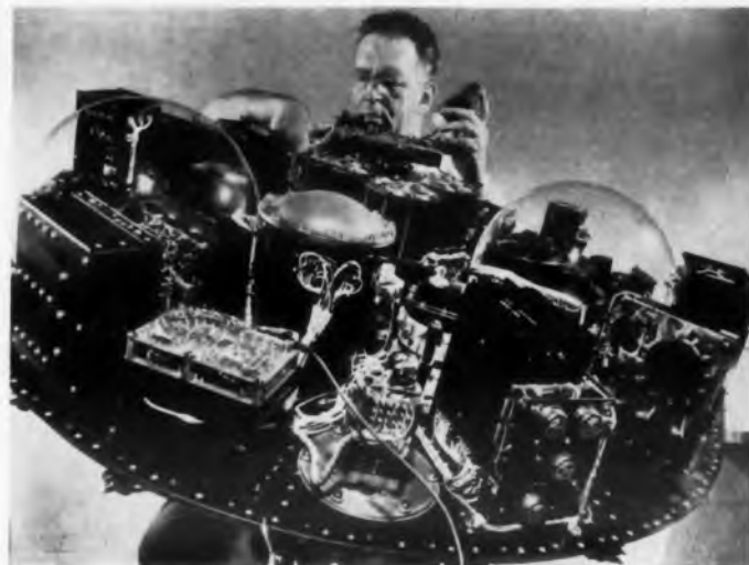
Opened Tiros shows camera front and center, tape recorders under plastic bubbles.
