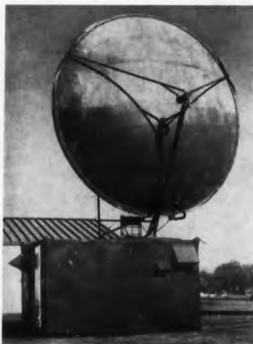
Air pressure maintains the shape for this air-transmittable 15-ft parabola. A dual-polarized horn eliminates the duplexer in the Collins scatter communications system.
