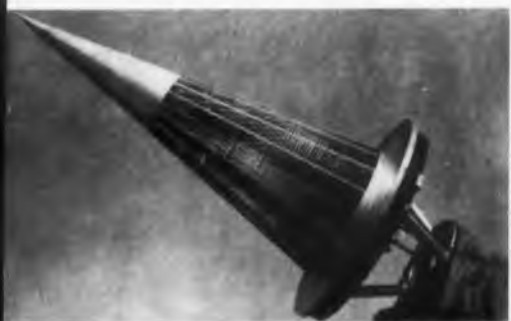
Nose-cone antenna is scanned over most of forward hemisphere. Hughes-developed, it replaces flush-mounted antennas.
