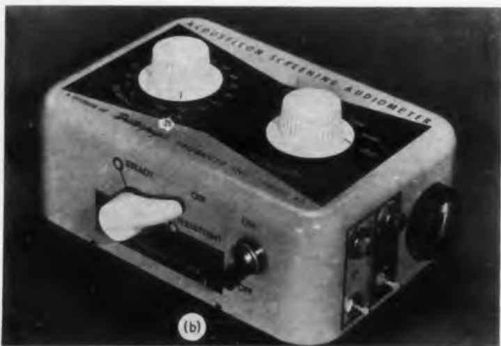
Fig. 3. Controls and switches should be identified and their functions specifically indicated. The interrupter switch in (a) does not disclose its three position settings; confusion is eliminated by appropriate marking applied as shown in (b).
