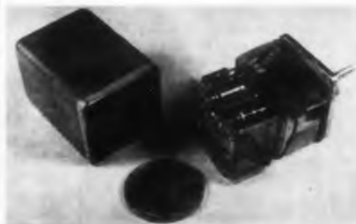
Fig. 1. Shrunken servo amplifier uses flexible printed-circuit board to increase component density. (Coin shows size—not price.)
