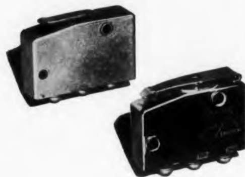
Fig. 2. Silk screening on small areas requiring much linework is impractical. For this type application, the use of an adhesive sticker is preferable.
