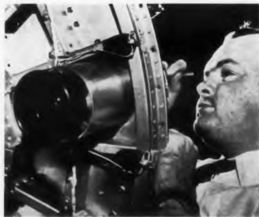
Wide-angle lens projects from cylindrical base plate of Tiros satellite. Vidicon camera behind lens is adjusted by technician.
