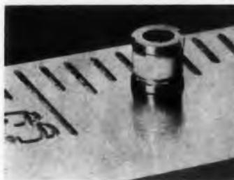
Having outside dimensions of 1/8 x 1/8 in., these microwave diodes offer cut-off frequencies up to 120 kmc. Applications are in traveling-wave, broadband parametric amplifiers. The diodes can be supplied to  $\pm 10\%$  capacitance tolerance. Other uses are as low-loss rf switches in resonant cavities at microwave frequencies and for doppler radar sideband modulators. Type 4253X has a cut-off frequency of 120 kmc and type 4254, 100 kmc. Capacitance at zero bias is 1.4 pf.
