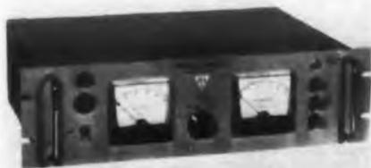
Type SCRT 32-15-1 transistorized power supply delivers an output of 10 to 32 v dc at 0 to 15 amp with both sides floating with respect to ground. Regulation is provided by silicon rectifiers. Dynamic response is less than 100 mv transient spike for 100  $\mu$ sec for a  $\pm 2\%$  step change in load current and less than  $\pm 1$  v transient spike for 0.1 msec for a step load change from 15 to 0 amp. Ripple is less than 1 mv rms.
