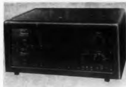
Consisting of the N-803 crystal-controlled timer and the N-276 scaler, this scaler-timer provides preset counts in 15 settings of 10 to 500,000 counts and preset time in 15 settings of 1 to 50,000 sec. Both the scaler and timer have staircase outputs for operation of a digital printer. A binary-coded decimal 1-2-2-4 output can also be provided. The scaler and timer can be used independently.
