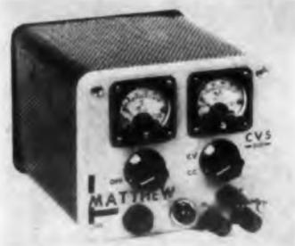
Designed for powering solid-state equipment, model CVS-300 power supply provides up to 400 ma at 30 v max on constant current operation and up to 500 ma at 4 to 36 v on constant voltage operation. A front panel switch sets the unit for constant current or constant voltage operation. Regulation is better than 1% against line and no load to full load variations. Ripple is less than 5 mv. For bench use or rack mounting, the unit measures 4.75 x 4.5 x 6.25 in.
