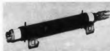
Model 206 10-kw traveling-wave tube, operating from an input of less than 500 mw, is for use over the frequency range of 8.4 to 9.4 kmc.
