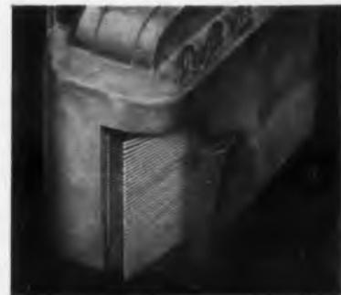
**RTV COIL IMPREGNATION** enables this Hughes Aircraft Co. transformer to provide top performance at  $250^\circ$ . Unlike other insulations tried, G-E RTV compounds proved successful both for coil impregnation and full encapsulation.
