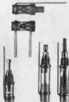
**ROTARY** in three models for high-frequency tuned circuits. Standard: to 12.0 mmfd; Split bushing: to 12.0 mmfd; Precision: to 4.0 mmfd; Full rating from -55 to +125°C., TC: +50  $\pm 50$ ppm/°C. Nonporous silver plating for corrosion resistance available on request.
