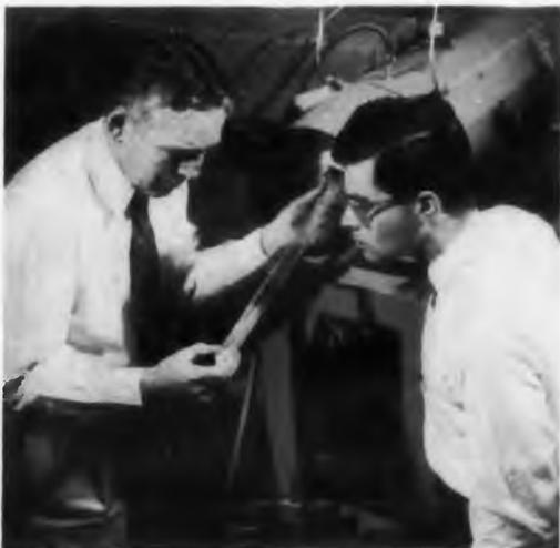
Scientists at Bell Telephone Laboratories, New York, inspect an ingot of gallium phosphide. Bell is developing methods of growing single crystals of a transparent semiconductor, gallium phosphide, and studying its properties. These studies will help in the basic understanding of high-energy-gap semiconductors. The material is transparent, making it possible to observe visually the differences which take place under varying conditions of doping and electron density.
