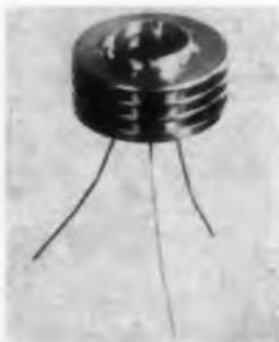
Types 2208 and 2209 heat sinks, designed especially for Mesa transistors, can be used for printed circuit board applications or can be mounted directly to the metal chassis. Heat generated in the transistor junction is conducted to the sink where it is removed to the surrounding air by means of fins.
