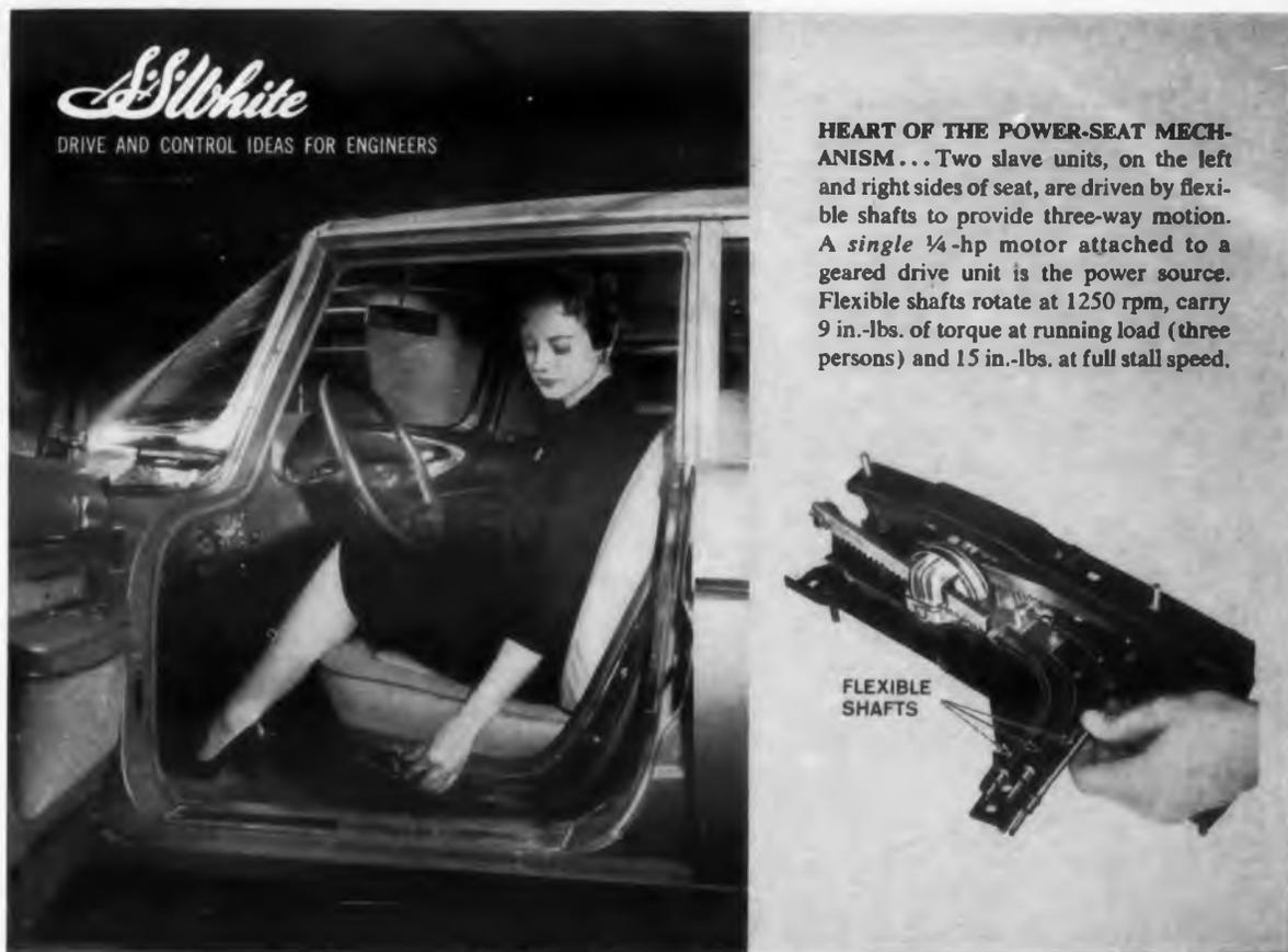
**HEART OF THE POWER-SEAT MECHANISM...** Two slave units, on the left and right sides of seat, are driven by flexible shafts to provide three-way motion. A single ¼-hp motor attached to a geared drive unit is the power source. Flexible shafts rotate at 1250 rpm, carry 9 in.-lbs. of torque at running load (three persons) and 15 in.-lbs. at full stall speed.
