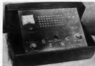
This automatic circuit tester is able to test 60 circuits per min. Designed for testing cable assemblies and components, the unit has applications in missile, instrument, and industrial fields. Three types are offered: a 50-circuit unit, a 100-circuit unit, and a 200-circuit unit. Continuity currents are 5 and 500 ma and 1 and 2 amp. The hi-pot voltage is variable up to 3000 v dc. The instrument measures 11.5 x 24 x 15 in.
