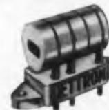
**CAT. 8718**—Ultra-High Temperature Socket for G.E. 7296 Triode can be soldered to printboard or mounted above or below a chassis. High Alumina insulating material; contacts gold plated Inconel-X. For continuous operation at 1000° F (538° C).
