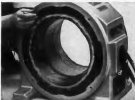
**ENCAPSULATION OF STATOR WINDINGS**, introduced by General Electric motor departments, extends service life of motors. RTV's resistance to moisture and other contaminants enables these dripproof motors to meet certain applications formerly requiring enclosed units.
