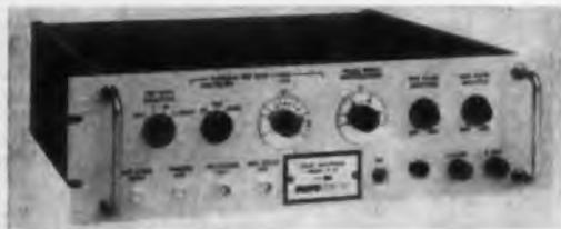
Model G-47 pulse generator produces positive and negative pulses with an output width of 2 to 20  $\mu$ sec and an output amplitude that is variable from 0 to 15 v into a 50-ohm load. The unit contains a variable repetition generator with a range of 1 to 1000 cps and two fixed-frequency sources of 1 and 10 cps. Containing both solid state and vacuum tube circuits, the unit is suitable for laboratory or ground support applications.
