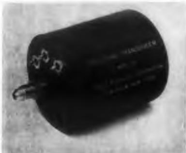
This series of pressure transducers, ranging from 0 to 25 up to 0 to 300 psi, is designed to stand 1,500 psi without shift or damage. The sensor design needs no auxiliary cut-off valving equipment. The units are for control, telemetry, and propulsion pressure measurement systems. Model 101, shown, measures 2.75 x 3 in. and is suited for differential pressure measurement applications involving the introduction of high pressures to the sensor and the instrument case.
