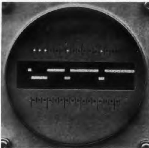
Placed over the oscilloscope tube face, the cardboard mask permits the display to be rapidly transformed to a digital form.
