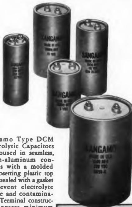
Sangamo Type DCM Electrolytic Capacitors are housed in seamless, drawn-aluminum containers with a molded thermosetting plastic top that is sealed with a gasket to prevent electrolyte leakage and contamination. Terminal construction insures minimum contact resistance in current-carrying members. Cover design provides an adequate safety vent in case of heavy overload.
