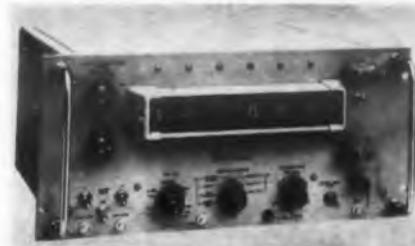
Types 523CR and 523DR electronic counters directly measure frequencies from 10 cps to 1.2 mc, time intervals from 1  $\mu$ sec to  $10^6$  sec, and periods from 0.00001 cps to 100 kc. Stability is 2 ppm per week. Sensitivity is 0.1 v. The 523CR has an in-line readout and the 523DR has a readout of six columnar neon indicators.
