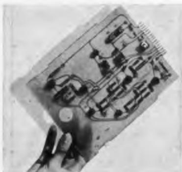
**Silicone Laminates.** Continuous-filament woven glass fabric impregnated with a silicone resin. These laminates combine high heat resistance (up to 500°F. continuous) with excellent electrical and mechanical properties. They are primarily used in high-temperature electrical applications and high-frequency radio equipment.
