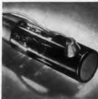
**POTTING OF AIRBORNE EQUIPMENT** provides protection from high altitude arc-over and corona as well as vibration and moisture. RTV silicone rubber protects this cathode ray tube up to 70,000 feet.
