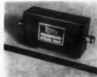
Model X-114 miniature isolator provides a minimum of 10 db isolation from 2700 to 3100 mc with less than 1 db insertion loss. Over the same bandwidth the vswr is 1.2:1. Suitable for airborne applications, the unit weighs 6 oz and measures 1 x 1-1/2 x 3-1/2 in. including TNC connectors.
