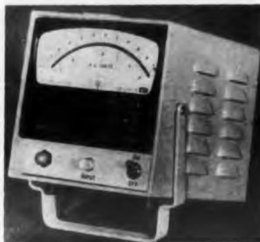
Model P-301 electronic millivoltmeter has 10 standard ranges from 0 to 10 mv up to 0 to 300 v. A dc meter, the instrument has an accuracy of  $\pm 2\%$  full scale on all ranges. Zero drive is  $\pm 1\%$  full scale for 8 hr. The input resistance is 10 meg.
