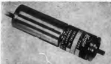
Type M840-001 servo motor-damping generator consists of a modified type of the R123 servomotor and type M863 generator. The low null voltage combined with the high generator output results in a 100:1 signal-to-noise ratio. This size 8 unit has a phase shift of 0 deg and a linearity of 0.2%. Output voltage for the generator is 1.1 v at 1000 rpm, the output impedance is 2100 ohms +j2500, and the rated load is 100,000 ohms. No load speed is 6500 rpm and stall torque is 0.25 oz-in.
