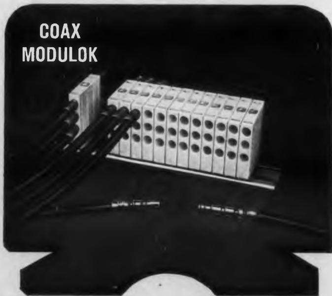
Same flexibility as regular MODULOK. Completely crimped contacts. Snap-in to insert. Press spring-loaded latch to release. Up to 30 modules (90 coax connections) per foot of track.
