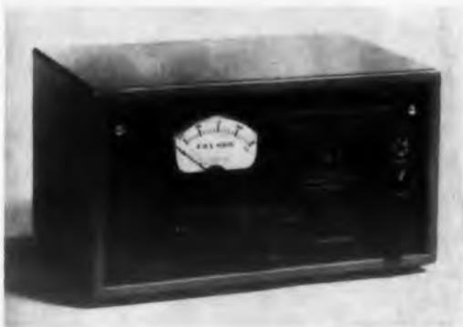
Model 811-B random noise generator has uniform output and a "pseudo-rms" metering circuit which reads identically on sine waves and white noise. It provides an output of at least 2.5 v rms on all ranges, and response is from 2 cps to 1.5 mc. A meter input jack enables its meter to be used for measuring other signals. It is available as a chassis unit, in a cabinet, or on a 19 x 5-1/4 in. rack panel.
