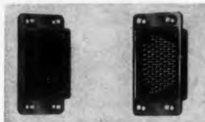
Series DTD rack and panel connectors are offered with single or double inserts mounted in a die-cast aluminum-alloy shell. Connectors with 50, 78, 100, and 156 contacts are possible. Either male or female inserts are interchangeable in the field as a sub-assembly. The insulating material is Melamine. Silver and gold plating are provided. Series DTD2 uses a screw fastener.
