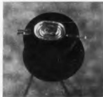
This microminiature transistor enclosure, a flat package measuring 0.125 x 0.18 x 0.06 in., permits greater component density than ordinarily possible. About 42 enclosures can be mounted on a 1-sq in. multi-element wafer, adding about 1/16 in. to the thickness. The cold-welded, metal-to-glass hermetically-sealed package provides a minimum seal length of 0.05 in. It houses any type of computer transistor.
