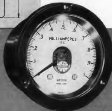
Mechanism: Permanent magnet moving coil. Available as: Rectifier-type AC voltmeter, milliammeter, microammeter, AC or DC tachometer Indicator. DC ranges: 200  $\mu$ a through 50 ma, 100 mv through 500 volts, self-contained.
