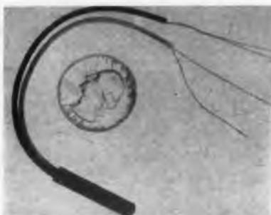
Model HP-315 axial field probe is for use as a gaussmeter probe and in other applications where the intensity of axial fields must be measured. Maximum diameter is 0.195 in. and length is 1 in. The device has a low ohmic residual error and a low temperature coefficient. The active element used is indium arsenide.
