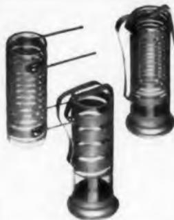
**DELIVERED OFF THE SHELF** 27 values ranging from 0.05 uh to 2.0 uh. High Q, 120 to 250. Frequency range from 10 MC to over 250 MC. High reliability under shock and vibration, since conductor is fired into glass, cannot shift. Low TC: 0 to +20 ppm/°C. Operation range from -55°C. to +125°C. No drift even under drastic dT. For panel or printed board mounting. Standard tolerance is  $\pm 10\%$ .  $\pm 5\%$  also available above 0.25 uh.
