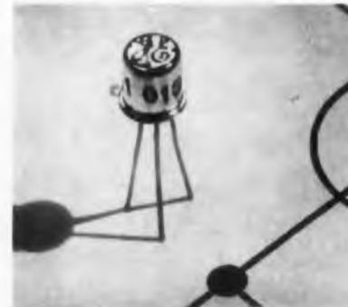
Types 1N2041 and 1N2969 germanium tunnel diodes, designed for use as circuit reference elements, have peak current ratings of 4.7 and 2.2 ma, respectively. These ratings are held to a variation of no more than 10%. Peak-to-valley ratio for both devices is 8:1. The 2N2941 has a total capacity of 30 pf and the 2N2969, 20 pf. The units have typical peak point voltages of 55 mv, typical valley point voltages of 350 mv, and typical forward peak point current voltages of 500 mv.
