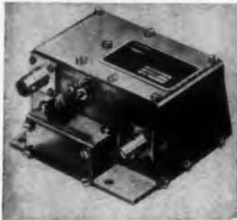
Model PA-11 10- to 25-w amplifier is for use with 1- to 5-w rf transmitters in the telemetering band of 215 to 260 mc. The frequency range is continuously tunable. The bandwidth is  $\pm 3$  mc. Input is 1.8 w and output is 10 w min into a 50-ohm resistive load with 1.8 w of driving power. The unit operates without forced-air cooling at rated temperatures and power. Heat transfer is sufficient for plate dissipations up to 15 w at 185 F. The unit stands shock and vibration.
