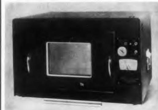
Model 7000A precision test chamber, which accommodates rack-mounted electronic equipment, has prolonged temperature runs with stability to within 0.5 F over the range of -100 F to +500 F. The unit has an internal test volume of 19-1/2 x 11 x 15 in. It can be preset for automatic hot-cold cycling at alternate temperature levels.
