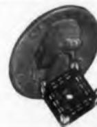
**CB-714B**—Printboard Application Socket for R.C.A. Micromodule. Measures only .400 maximum square by .094 high. Insulation resistance greater than 50,000 megohms. Employs silver plated beryllium copper contacts and DIALL FS-5 insulating material.
