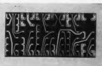
Low-Cost commercial circuits. Made from CDF's paper-based Di-Clad copper-clad laminate.
