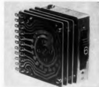
Series TMBD-P-10 multi-deck 8-, 10-, or 12-position thumbwheel switches are available with 2, 3, or 4 XXXP or epoxy printed-circuit modules. These consist of any combination of binary and digital rotary thumbwheel switches all annually operated by a single 1/4-in. thumbwheel. Contacts are precious metal alloy and mounting frames, corrosion-protected aluminum. One number at a time is exposed through bezel opening.
