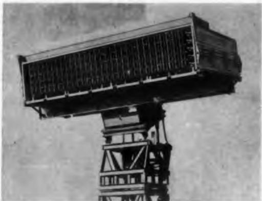
The corporate structure antenna is divided into a myriad of separate radiating elements, each of whose radiation can be carefully controlled.
