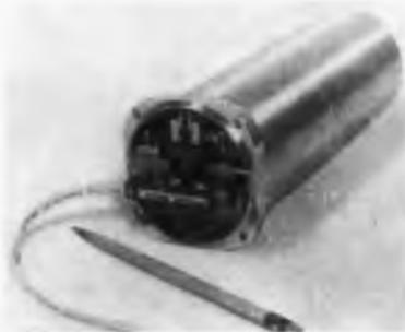
Able to print at speeds of better than 30 characters per sec on 5/16 in. tape, this printer measures 9-1/4 in. long, has a self-contained power supply, and fits a 3-in. instrument case. It is suitable as a printer for computer output and can also be used in check-out devices and in aircraft applications.
