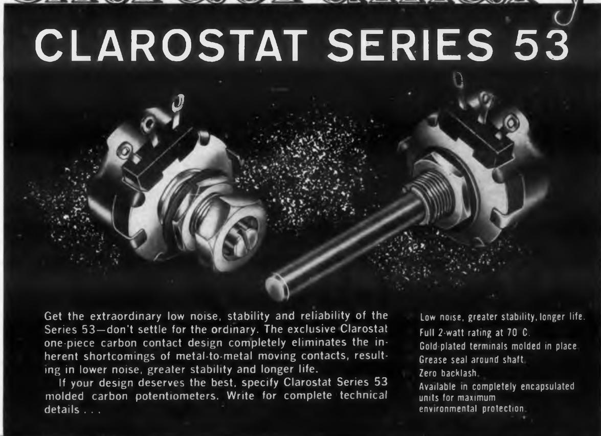
Get the extraordinary low noise, stability and reliability of the Series 53—don't settle for the ordinary. The exclusive Clarostat one-piece carbon contact design completely eliminates the inherent shortcomings of metal-to-metal moving contacts, resulting in lower noise, greater stability and longer life.
