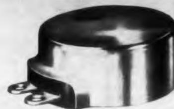
Designed for electronic heating or cooling applications, the Klixon 4286 low-differential, precision thermostat opens or closes on temperature rise. It is for use as a control device in guided missiles, aircraft control, computers, and crystal ovens. Continuous temperature exposure limits are  $-65$  to  $+270$  F; the temperature setting range is 0 to 250 F. Approximate weight is 3.5 g.
