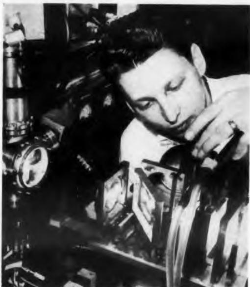
Technician inserts a filter in the path of a photon beam that is to interact with negative ions in the lighted chamber at left. This equipment has been designed by the National Bureau of Standards for the continuation of studies basic to plasma physics. It may be used in crossed ion-electron-beam experiments as well as in photodetachment work.
