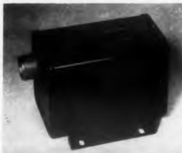
For instrumentation, telemetering, and recording systems, this 5-w power supply comes in three models having outputs of 5, 10, and 15 v dc. Input is standard airborne 115 v at 400 cps. Dual magnetic regulation consists of a flux oscillator and a magnetic amplifier regulator. Requirements of MIL-E-5272A are met.
