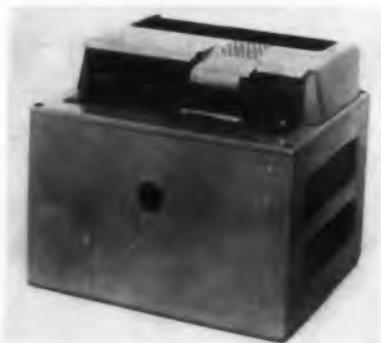
For reading out information stored on perforated paper, plastic, or metallic tapes, model 100 tape reader is for line-by-line reading at speeds to 60 lines per sec. A motor containing a printed-circuit armature can be started and stopped several hundred times a second. The tape reader has only one moving part. Its dimensions are 10-3/4 x 8-3/4 x 9 in.
