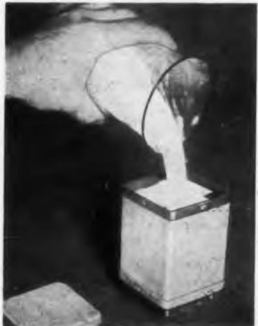
Research by Bell Telephone Laboratories suggests unusual possibilities in a special form of aluminum oxide developed by Carborundum's Refractories Division. The material is made by a process which converts alumina powder into microscopic, light-weight, free-flowing, non-abrasive bubbles. Ordinary granular alumina won't serve the purpose.
