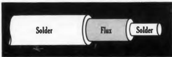
No other solder provides the performance advantages of ALPHA Cen-Tri-Core Energized® Rosin-filled Solder because no other solder is made this way.
