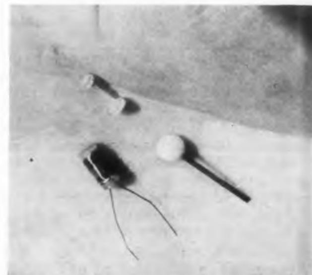
**Blood flow meter components** shown here are too large for animal or human use. The 6-mm ball was used in simulated flow experiments. Both the magnet coil and its plastic bobbin are illustrated. The ball is machined of Teflon or other physiologically inert material.
