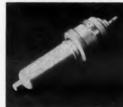
The type D-1008, a ceramic-metal power triode designed to withstand environmental extremes, is a water-cooled tube with a heavy-wall copper anode and mesh-type cathode. The tube is rated at 60 kw, full-power input to 50 mc and reduced input to 110 mc, with maximum anode dissipation of 20 kw. Applications include use as a class C amplifier, or as an oscillator in dielectric and induction heating service. The tube can switch 220 amp at 18 kv as a hard-tube radar modulator.
