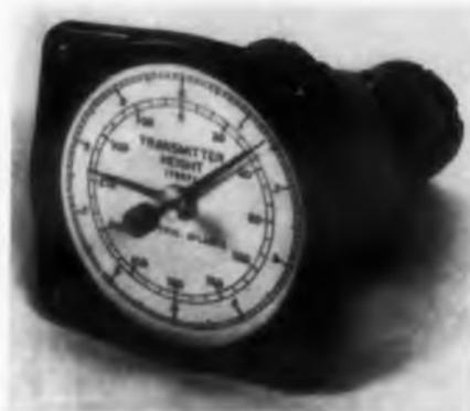
Series IU dual synchro position indicators are designed for accurate, non-ambiguous indication of linear or angular position of transmitter units. The indicators can be read accurately within  $\pm 0.03$  deg from a 5-1/4 in. panel mounting. A separate synchro receiver is geared to each pair of concentric dial pointers. Model IU-3 indicator can be reset to zero with respect to an arbitrary reference point; Model IU-6 indicator monitors mechanisms with fixed reference points.
