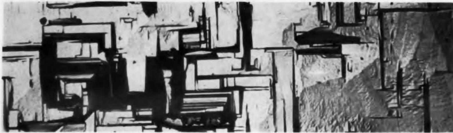
Exotic design at left is representative of the exotic circuits that may be possible using the epitaxial-growth process—position of vaporized silicon so that it continues the single crystal structure of the seed crystal. This is an example of silicon deposition on a crystal oriented along the 100 plane.
