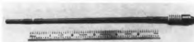
The Type M2101-B traveling wave tube is a broad band, periodically-focused low-noise device
