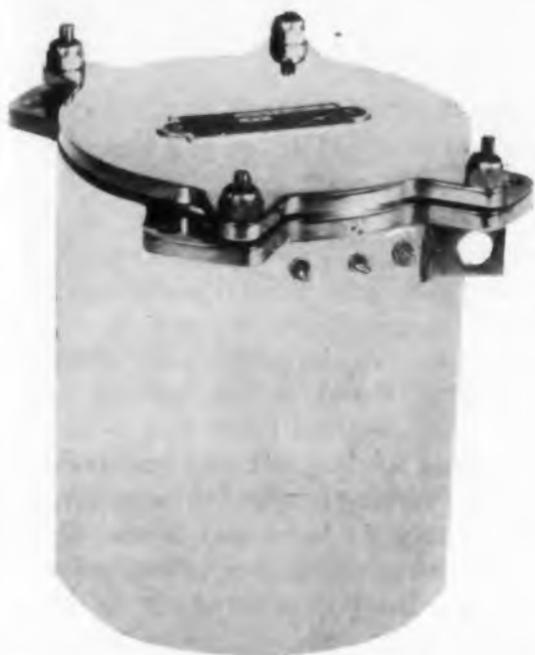
This Dewar flask is used to maintain a stable temperature for the stable oscillators in the Transit program. The quartz crystal is mounted in the flask, and the oscillator circuitry is mounted on a circular plastic board fitted inside the top of the flask.
