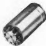
**Tiny Control Center.** Synchronous at 24,000 r.p.m. in less than five seconds — using overvoltage techniques — this 2 oz., subminiature floated rate gyro assures stable, precise flight control of missiles, special weapons and space vehicles. MPB bearings on critical main shaft help assure accuracy under 150 G's of shock and 30 G's vibration to 2000 cps on any axis.
