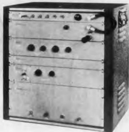
This unit features an electronic pulse delay that can be set to zero or is continuously variable from .030 microseconds to 500 microseconds in five ranges. Pulse width is continuously variable from .02 to 12.5 microseconds in four ranges.
