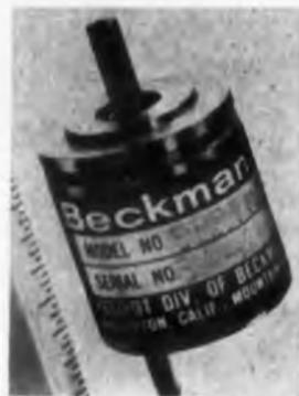
Designated model 8 SM 461, this size 8 servomotor is 0.84-in. long and weighs 1.1 oz. The unit is for 115-v sources. It has a rotor inertia of 0.18 gm-cm<sup>2</sup> and a stall torque of about 0.22 oz-in., providing acceleration at stall of 86,500 radians per sec<sup>2</sup>. Ambient temperature range is -55 to +130 C; maximum operating temperature is 200 C.
