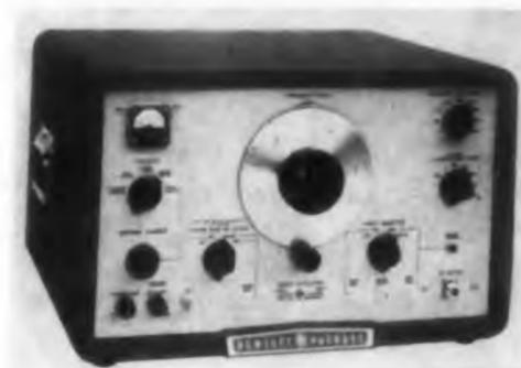
The Model 628A sweep oscillator provides cw and swept rf frequencies from 1 to 2 kmc. The device has independent, direct-reading frequency, sweep-rate and sweep-range controls. The oscillator can be used with an oscilloscope or on mechanical recorders.
