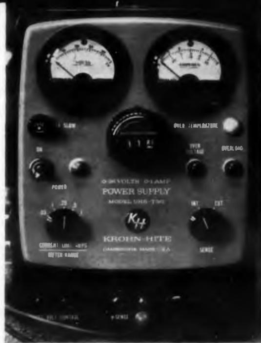
**Bench-model supply** has digital voltage dial, accurate to 50 mv. The dial is also featured on rack-mounted units.
