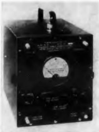
Model NF-157 rf power density meter directly reads power densities from 0.1 to 2000 mw over a continuous frequency range of 200 to 10,000 mc. The unit uses small batteries as a power source and any of three constant-gain probes. Power is measured by a thermistor element in a temperature-compensated dc bridge. The unit weighs 10 lb. Suggested applications include personnel safety indication in strong rf fields, near-field intensity measurement and detection of hot spots and leakage near antennas.
