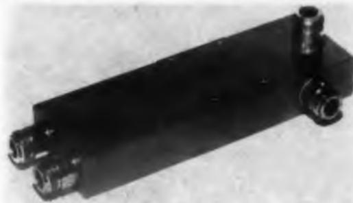
This S-band circulator has a typical size of  $3/4 \times 2-1/2 \times 7$  in. and weighs less than 2 lb. Characteristics are: 20 db isolation, less than 0.5 db insertion loss, and input vswr less than 1.2 over a 2 mc bandwidth. The circulators can be adapted for use with parametric amplifiers as input-output couplers, or in low-power applications of up to 1 w, avg.
