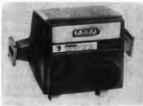
Type 101 broadband, direct-reading attenuators come in nine models covering the frequency range of 3.95 to 40 kmc. Attenuation range is 60 db and maximum vswr is 1.15. The units are rotary-vane type. The value of attenuation is determined by the angular position of a resistive film with respect to the waveguide.
