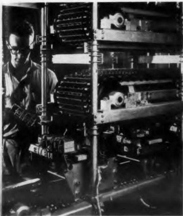
**Electromechanical memory** of letter sorter. Each "comb" is punched according to destination of a particular letter and travels along endless belt. Letter travels in a box on another belt in synchronism with the memory belt. Teeth on combs signal the box to open and to deposit letter into its proper destination bin. Two of the six encoding mechanisms controlled by the operators are visible at the bottom of the photo.
