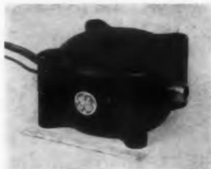
This bowl-magnet, designed for voltage-tunable magnetrons, is a compact, light-weight unit that the firm can apply on a custom basis to any of its S-, L- or X-band vtm's. For example, the Type Z-5337 vtm, with a range of 2,900 to 3,100 mc, weighs 1.5 lb, has a diameter of about 3 in. and has a height of less than 1 in.
