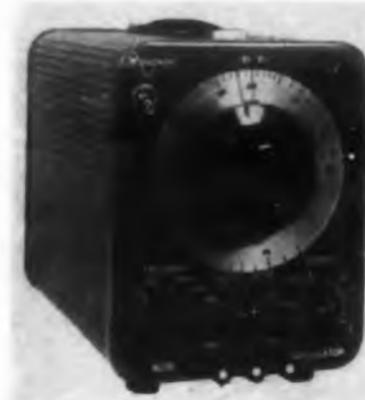
Model 401-B oscillator, a source of audio and ultrasonic sine waves, operates with a distortion of less than 0.1% at full output of 20 v, open-circuit. Frequency range is 9 cps to 120 kc, covered in four decade bands. Accuracy is  $\pm 2\%$ . Output amplitude is controlled by a five-position decade attenuator plus a continuous control; any voltage above 100 mv can be selected. Output amplitude is independent of frequency within  $\pm 0.5$  db. The unit measures 8 x 6 x 10.5 in. and weighs 12 lb.
