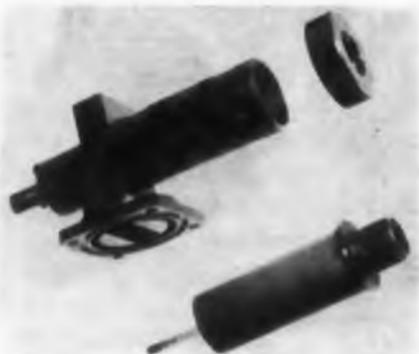
Warranted for 2,000 hr min life, type L-2017 noise source provides an excess noise ratio of 18.5  $\pm$  0.5 db over the frequency range of 8,790 to 9,190 mc. Similar tubes are available for other frequencies. The tubes are particularly useful in providing continuous radar system performance monitoring because the excess noise ratio is unaffected by changes in ambient temperature or operating current over a wide range of values.
