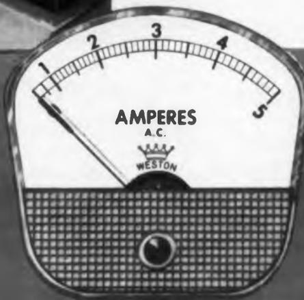
New Model 1724 AC instrument with moving iron mechanism has a 2.25" long scale. Supplied as: voltmeters, ammeters, milliammeters. Model 1721 (2.5" scale) and Model 1741 (4.9" scale) are supplied as: DC voltmeters, ammeters, milli- and microammeters. Rectifier-type AC Model 1722 (2.5" scale) is supplied as: Voltmeters (1,000 ohms/volt), milli- and microammeters.
