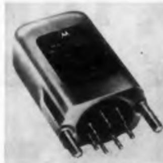
The F5A magnetic modulators have a standard frequency range of 60 cps to 10 kc but can operate as high as 100 kc with low-impedance units. The dual-channel type F5A113 has a signal winding resistance of about 700 ohms. Single-channel type F5A114 is also offered. Originally intended for use as a circuit element in conjunction with amplifiers in servo systems, the units can also be used with thermocouples, strain gages, computing devices, and telemetering equipment.
