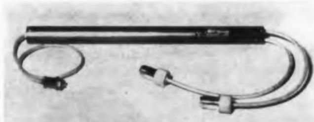
The Type HA-70 traveling wave tube has a noise figure of 7 db max, a 25-db min gain, a 1 mw saturation power output min, and a frequency range of 2,300 to 3,400 mc. It is focused in a 750 gauss solenoid and has a back attenuation of 70 db min. The tube is 22.4 in. long and has a 1-in. diameter. It is warranted for 1,000 hours.
