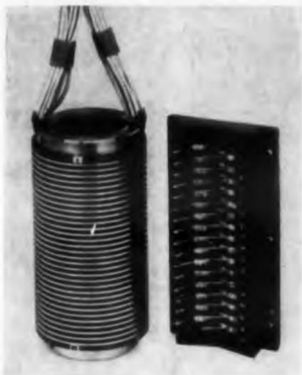
This slip ring brush assembly is manufactured on modular tooling which permits any number of rings from 1 to 32 to be furnished without tooling costs or time delay. The silver graphite brush rides in a rectangular groove on the coin silver ring resulting in reduced noise levels.
