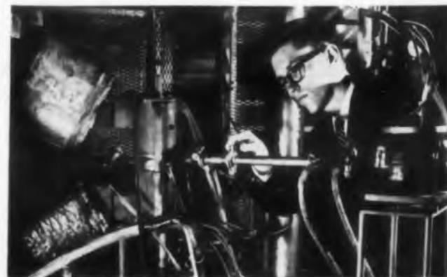
Microfier experiment is conducted at Raytheon's Crossed Field Tube Lab by John Jensen, staff engineer. Electromagnets are at left, and a QK625 M-Type backward wave oscillator delivering 200 w of cw at S-band is at right. The converter, with a 2-in. metal band around it, is located between the pole pieces of the electromagnets.
