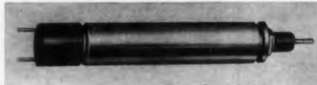
No. 32 solenoid, designed primarily for use in computers and data processing, lifts up to 8 oz intermittent or 6 oz continuous duty and has a life of 20,000,000 cycles. It operates on 6 to 110 v dc with 3 w continuous or 6 w intermittent duty. Enclosure is steel shell; terminals are plug-in or lead types; mounting is 4-28 threaded bushing. The size is 0.5 in. in diameter and 3.5 in. long.
