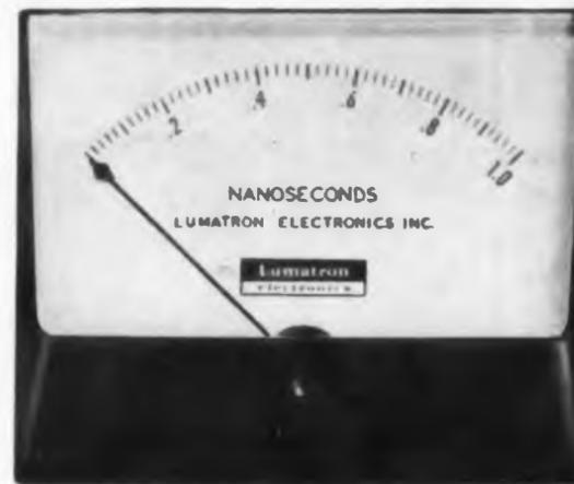
**A** NEW INSTRUMENT measures switching times as short as half a nanosecond. Five times faster and ten times more accurate than earlier instruments that did part of its job, this tester measures rise, fall, turn-on, turn-off, and storage times, one at a time or in any sequence.
