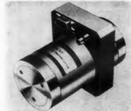
The Model 571 altitude control transducer is economically designed for use in expendable target drones or tactical missile and aircraft applications. The unit employs a trapped-air-pressure design to provide an accurate altitude error signal. It operates to 80,000 ft with a dynamic error band of  $\pm 2\%$ . Functional range is  $\pm 0.5$  psi. The unit has a 2-1/4 in. diam and is 4-1/4 in. long.
