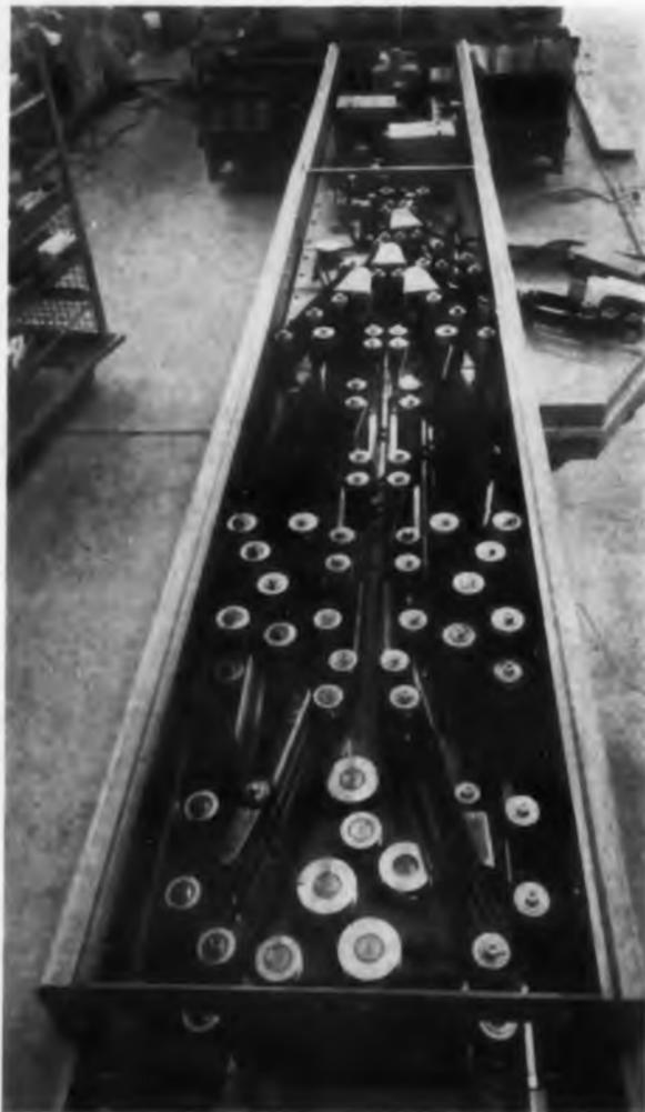
**Rube Goldberg appearance** of facer-canceller belies its 24,000-letter-per-hour capacity. System of photocells controls belt drives moving letters through the machine to cancelling heads in foreground. Metered and unstamped mail is deflected into tray which is shown at the right of machine.
