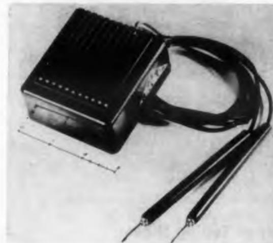
The Circuitester is for production line or lab wiring continuity checks. It is a transistorized buzzer that provides an audible tone when path resistance is less than 0.5 ohms. Path resistance changes between 0.5 and 15 ohms change the pitch of the buzzer substantially; above 15 ohms there is no tone. The device tests for direct wire paths and is not sensitive to paths through inductances or capacitors.
