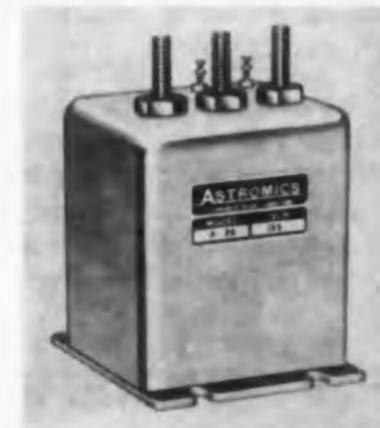
Type A-2A relay is a non-magnetic latching unit that mechanically locks in either the open or closed position, and requires a new command pulse before it can be reactivated. Contacts are plug-in type, assuring contact under extreme conditions and permitting loads up to 20 amp at 26.5 v dc. Energizing current is 0.25 amp at 18 to 32 v dc.
