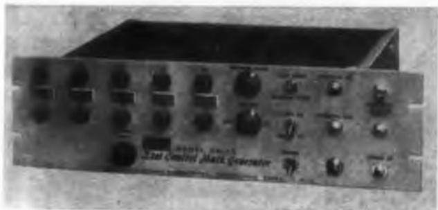
Model CM-10 crystal-controlled marker generator is similar to model CM-6, but is a 10-crystal unit and is rack mounted. Frequency range is 2 to 100 mc. In the higher frequencies, up to the 20th harmonic will be visible, and in the lower frequencies, up to the 10th harmonic will be visible. The outputs of the individual oscillators can be mixed with the output of each completely controlled from maximum output to no output.
