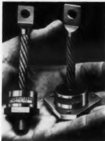
These Quad-Sealed silicon rectifiers are rated from 45 to 150 amp at 50 to 600 v over a temperature range of -20 to +130 C. They can withstand surge currents of 1000 amp peak. They are recommended for industrial power and battery charging applications. Stud mounted, flat base and reverse polarity types are available.
