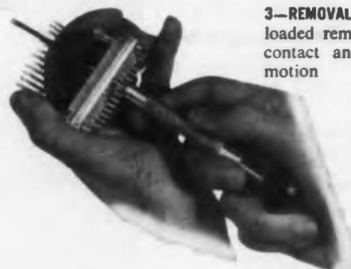
3—REMOVAL . . . Special spring-loaded removal tool removes contact and wire with one motion
