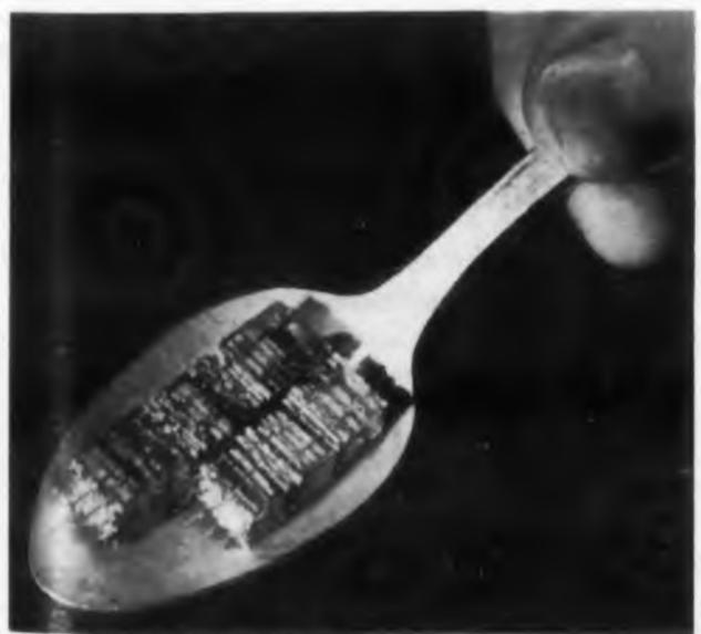
Technician removes micromodule flip-flop from the navigation computer used with the RCA micromodularized inertial-guidance system, upper and lower left. Pencil at lower left points out some of the preamplifier micromodules, which have been mounted on the inner gimbal of the guidance system to cut down on the number of slip-rings required. Size of encapsulated modules is illustrated above. This spoonful is equivalent to six transistor commercial receiver.
