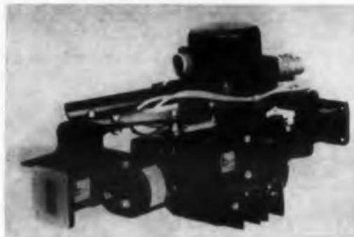
This attenuator is designed to be switched on and off without turning off the transmitter. It can attenuate fixed values from tenths of a decibel to over 20 db. With switch de-activated, power loss is less than 0.6 db. This pressurizable unit is available for most frequency ranges and waveguide sizes.
