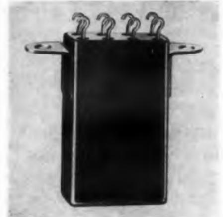
Type JSH relays are spdt and dpdt units with sensitivities of 25 and 40 mw respectively. Non-inductive contact rating is 2 amp at 29 v dc or 1 amp at 115 v ac. The relays can withstand vibration of 15 g from 55 to 2000 cps, 0.09 in. double amplitude from 5 to 55 cps, and shock of 50 g without contact chatter. The units weigh 1.1 oz.
