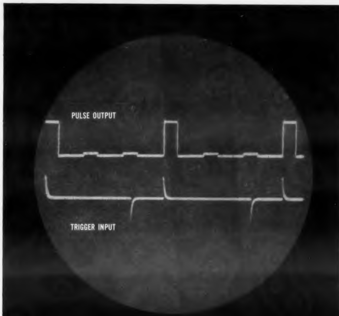
Input and output wave forms for circuit shown below
