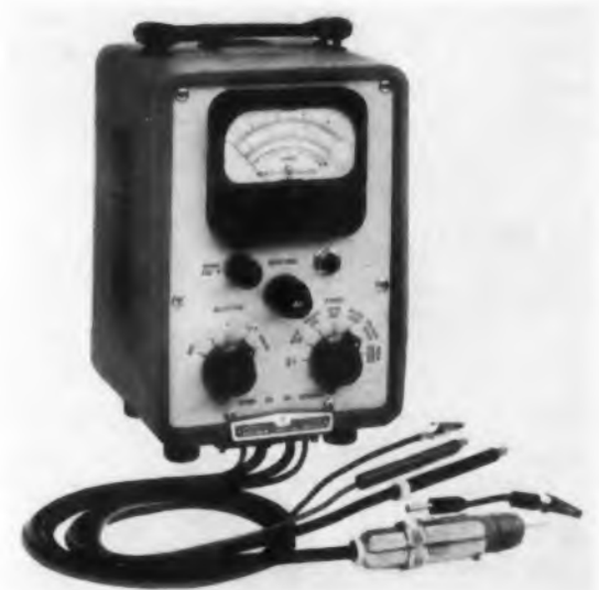
Fig. 12d. Hewlett-Packard. Vacuum Tube Voltmeter 410B provides full-scale readings of dc from 1 to 1000 v and ac from 1 to 300 v from 20 cps to 700 mc with an accuracy of 3 per cent. The 410B reads resistance from 0.2 ohm to 500 meg.
