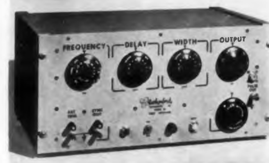
Fig. 2b. Rutherford Electronics. Pulse Generator B7 has repetition rates of 20 cps to 2 mc with variable pulse delay to 10 msec. Pulse width is variable from 50 nsec to 10 msec. Rise and fall times are 15 nsec each.
