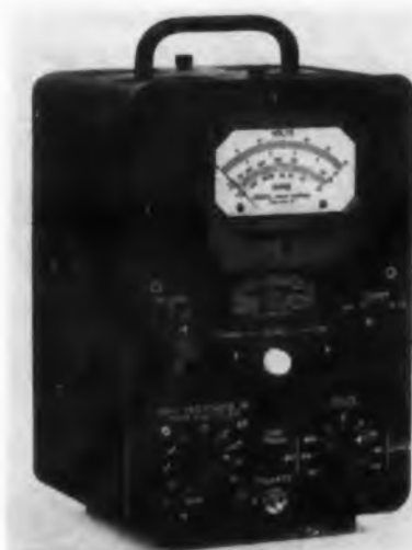
Fig. 19a. General Radio. DC Amplifier and Electrometer 1230-A. Measures resistance from 300 K to 5 \times 10^{14} ohms. Also measures voltage from 30 mv full scale to 10 v dc and currents from 5 \times 10^{-15} amp to 1 ma dc. Also used as sensitive dc amplifier.
