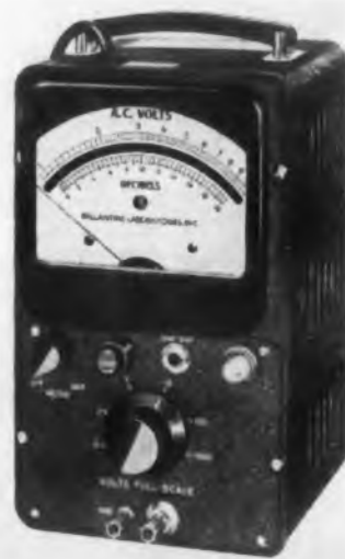
Fig. 9a. Ballantine. Electronic Voltmeter 300D measures sine waves from 10 cps to 250 kc, a somewhat narrower range than the 20 cps to 400 kc of the MVL-2M. The Ballantine has a logarithmic scale which provides a uniform 2 per cent accuracy at any point on the scale.
