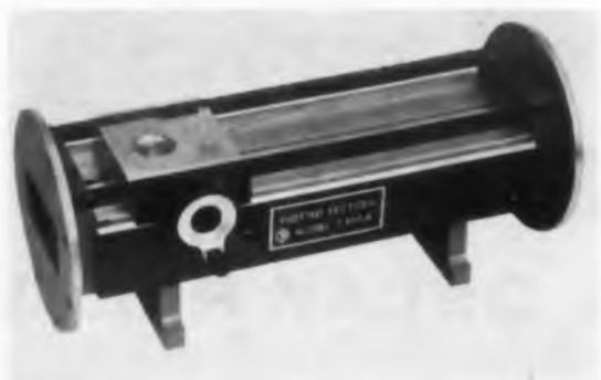
Fig. 18c. FXR. Precision Slotted Section H101A covers 3.95 to 5.85 kmc with vswr of 1.01. Series 101 covers 0.35 to 12.4 kmc.
