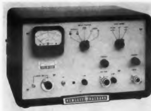
Fig. 16a. Hewlett-Packard Noise Figure Meter 342A is used with a noise source. Frequencies: 30 to 200 mc. Range: 0 to 15 db with indication to infinity. Bandwidth: 1 mc minimum. Russian instrument appears to have facility for front-panel selection of any frequency within its range. Difficult to tell whether Russian unit is automatic. H-P unit can automatically measure and continuously display noise figure and can provide recorder output.
