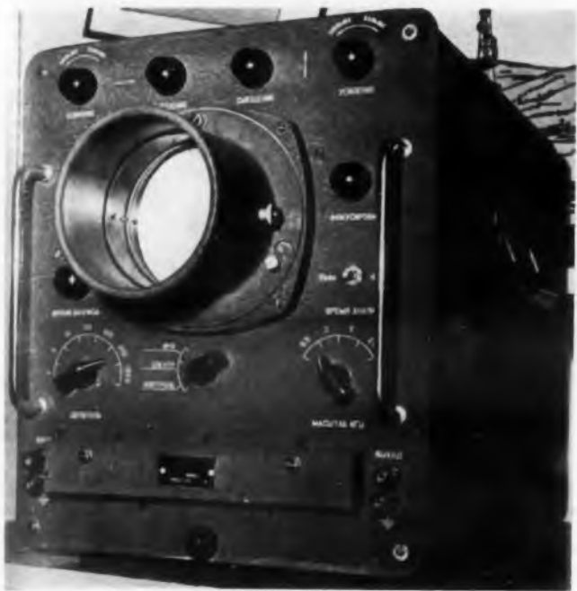
Fig. 6. Spectrum analyzer ASCHX-1 analyzes cw signals from 20 cps to 20 kc.
