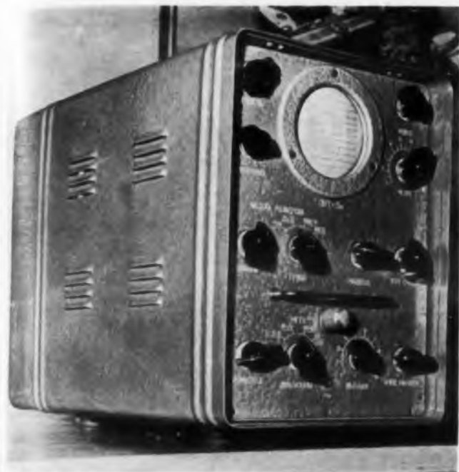
Fig. 1. Pulse generator PNT-3M, principally a serviceman's tool, generates frequency-modulated oscillations from 6 to 232 mc.
