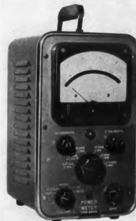
Fig. 14a. FXR. Power Meter B831A, with appropriate temperature-compensated thermistor heads, covers from 10 to 3000 \mu w in six ranges compared with 15 to 5000 \mu w for the MTO-1. The FXR instrument is far more compact than the Russian unit.
