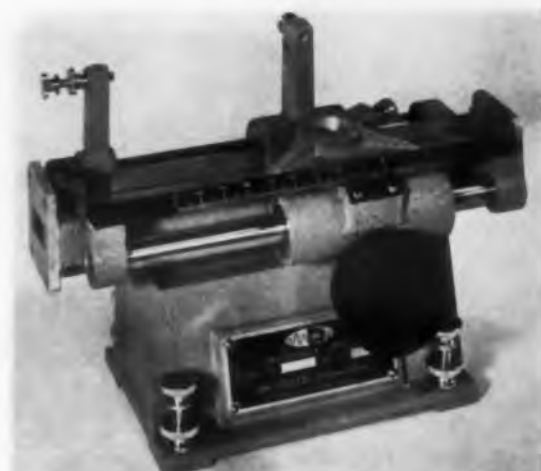
Fig. 18b. Narda Microwave. Waveguide Impedance Meter 220 covers 8.2 to 12.4 kmc with vswr of 1.01. Others available from 2.6 to 18 kmc.
