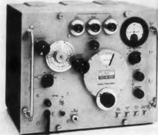
Fig. 6a. Hewlett-Packard UHF Signal Generator 616B covers 1.8 to 4.2 kmc, a slightly wider range than the 3.75 to 5.75 kmc of the Russian unit. The 1 per cent frequency accuracy of the H-P instrument is twice as good as that of the Russian unit.
