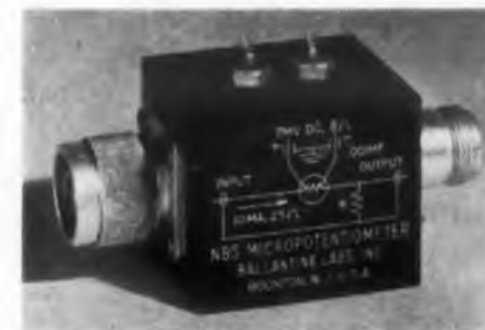
Fig. 11b. Ballantine. Micropotentiometer 440 is basically a low-source-impedance voltage source, useful from dc to almost 1000 mc. It has a uhf thermocouple whose dc output can be read on an external microammeter. Instrument can calibrate sensitive high-frequency voltmeters and, with an auxiliary transfer device, it can calibrate output levels of signal generators.
