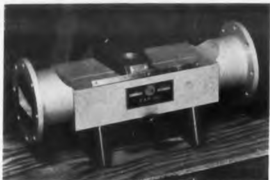
Fig. 18d. Hewlett-Packard. Waveguide Slotted Section S810A covers 2.6 to 3.95 kmc with vswr of 1.01.
