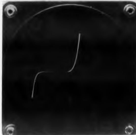
Curve tracer shows the static characteristic curve of the backward diode. On the horizontal scale, each large division equals 0.1 v; on the vertical, each large division equals 1 ma.
