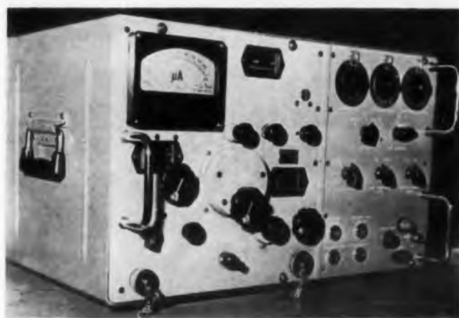
Fig. 3. Signal generator GSS-27 generates frequencies from 2 to 3.8 kmc with a frequency accuracy of 1.5 per
