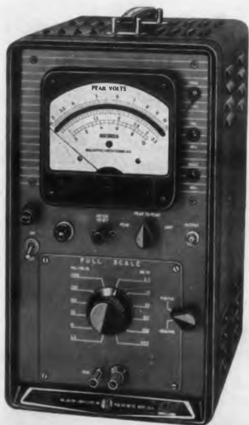
Fig. 13a. Ballantine. Peak Voltmeter 305A gives peak, or peak-to-peak readings of sinusoids from 5 cps to 500 kc and pulses with durations of 0.5 \mu sec to 5 msec. Full scale readings, on logarithmic scales, are from 3.5 to 1000 v.
