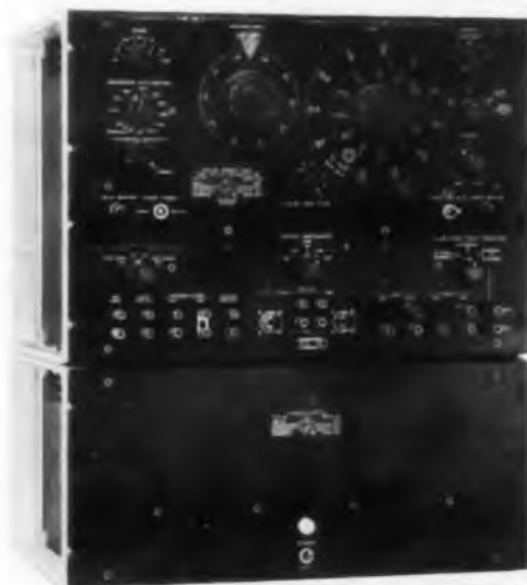
Fig. 1b. General Radio. Pulse, Sweep, and Time Delay Generator 1391-B can provide pulse lengths as long as 1 sec and repetition rates to 250 kc. Its 50-nsec rise time is equal to that of the Russian instrument.
