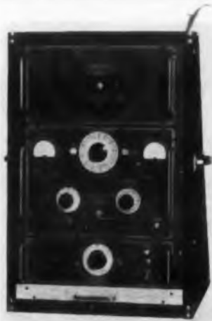
Fig. 3b. Boonton Radio. FM-AM Signal Generator 202-E provides both am and fm coverage for a wider range of frequencies than does the GSS-17. It covers 54 to 216 mc while the latter covers 16 to 128 mc. The 202-E gives from 0 to 50 per cent modulation and provides eight internal-modulation frequencies from 50 cps to 60 kc. Am distortion of less than 5 per cent is the same for both instruments but the Boonton gives less than 2 per cent fm distortion (compared with 3 per cent) over a very wide fm range of 0 to 240 kc (compared with 0 to 75 kc). External am fidelity is 30 cps to 200 kc for the 202-E and 100 cps to 10 kc for the GSS-17 while external fm fidelity is 30 cps to 200 kc for the Boonton and 70 cps to 15 kc for the Russian unit.
