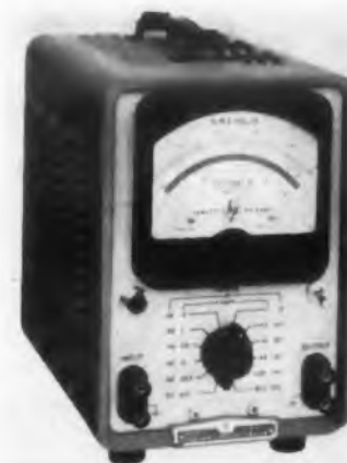
Fig. 10a. Hewlett-Packard. Vacuum Tube Voltmeter 400H covers 1-mv to 300-v full-scale ranges from 10 cps to 4 mc (compared with 30 cps to 10 mc).
