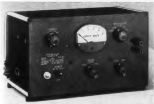
Fig. 15a. General Radio. Random-Noise Generator 1390-B has wider frequency range and considerably higher output: 3 v to 20 kc, 2 v to 500 kc, and 1 v to 5 mc.
