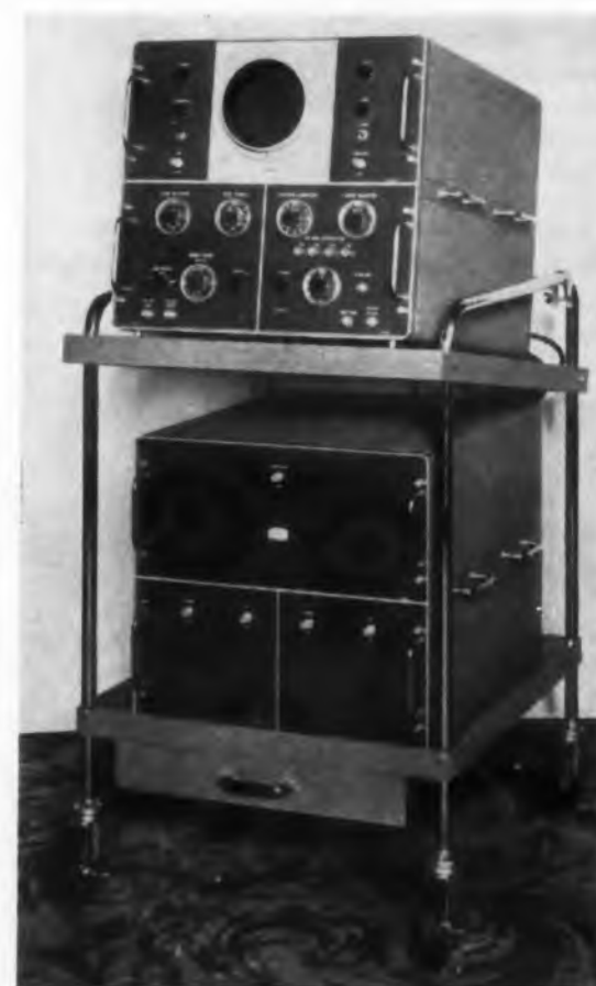
Fig. 20a. Allen B. Du Mont. High-Frequency Oscilloscope 410 provides sweep durations from 0.1 usec to 200 msec, and sensitivity to 20 cm per volt. Fastest sweep speed on Russian instrument is about 10 times faster than that on the 410. Du Mont unit has about 1000 times stated sensitivity of Russian unit. Du Mont scope can be triggered at 250 kc. Both instruments have 4-w input attenuators, the Du Mont at 50 ohms, the Russian at 75 ohms.
