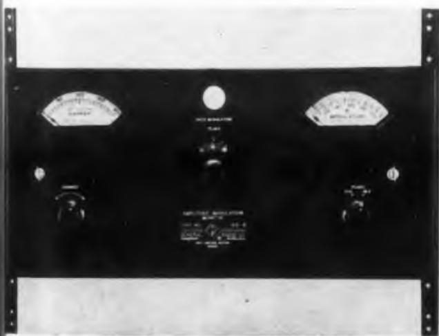
Fig. 7a. General Radio. Amplitude-Modulation Monitor 1931-B measures am per cent modulation from 0 to 110 per cent on positive peaks, to 100 per cent on negative peaks. Works with carriers from 0.5 to 60 mc. Does not have as wide a frequency range as the Russian equipment but per cent modulation range is wider. G-R instrument does not measure frequency deviation. Intermediate frequency of the systems being tested should not exceed 100 mc with maximum bandwidth of 15 mc. Noise source can be mounted on front panel. Though it detracts from appearance, it is convenient when equipment under test is nearby. For other applications, it appears that noise source and cable can be unhooked from front panel.
