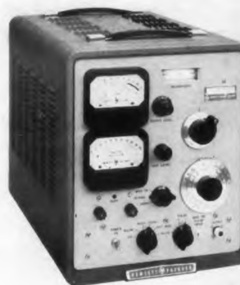
Fig. 5a. Hewlett-Packard. UHF Signal Generator 612A, covering 450 to 1230 mc, overlaps the frequency range of the GSS-15A and the GSS-15B. The H-P 614A covers 800 to 2100 mc and the H-P 608D covers 10 to 480 mc. Maximum power output of the GSS-15A (1 w) and of the GSS-15B (0.5 w) exceed that of the H-P (5 mw).
