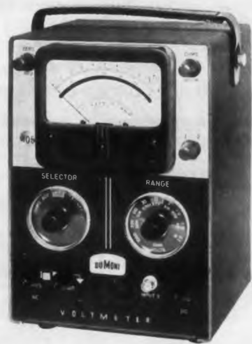
Fig. 12b. Allen B. Du Mont. AC-DC Voltmeter 405 measures dc from 0.1 v to 1000 v full scale, and ac from 0.1 v to 300 v full scale from 50 cps to beyond 700 mc with appropriate probes. Voltages may be measured at either of two switch-selected input terminals. Circuit ground is isolated from chassis so differential voltage measurements can be made. Resistances can be measured from 0.5 ohm to 500 meg.
