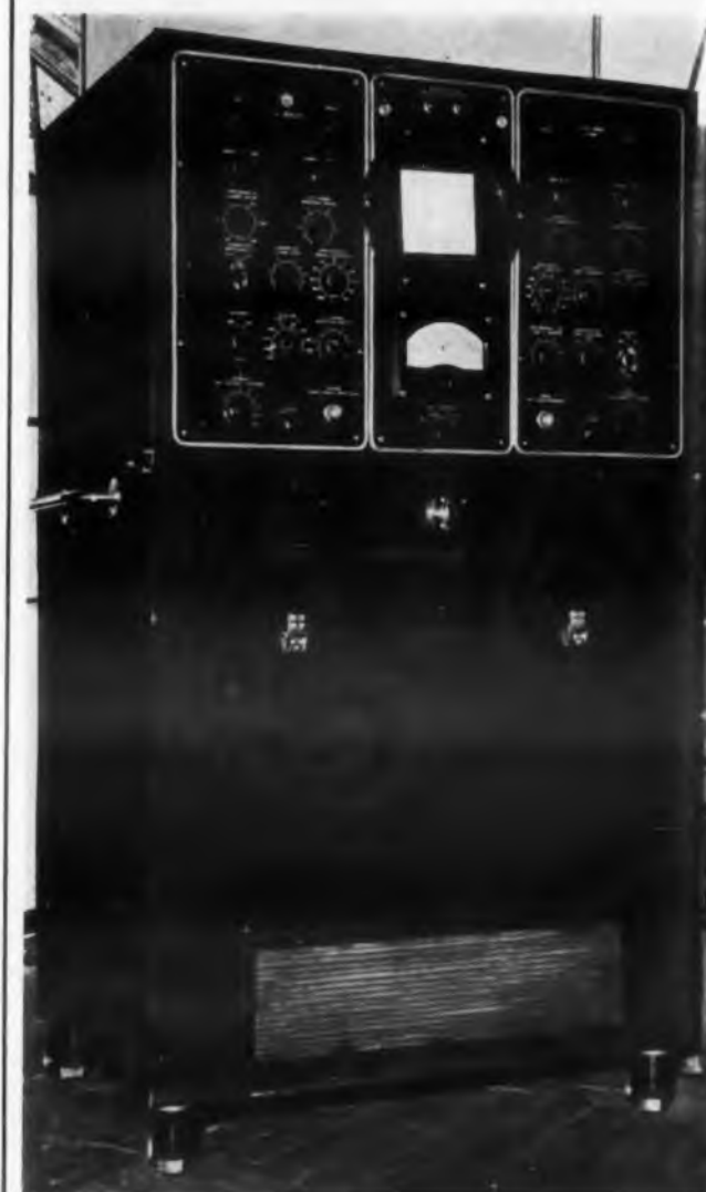
Fig. 5. Dual-beam oscilloscope DESO-1 has a vertical pass band of 30 cps to 60 mc with a minimum sensitivity of 13 mv/mm.
