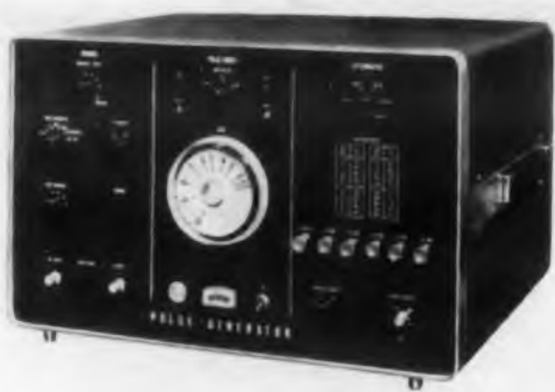
Fig. 1a. Allen B. Du Mont. Pulse Generator 404, with repetition rates from 10 cps to 100 kc, has wider frequency range than the Russian instrument, and its 20-nsec maximum rise time is better than the 50 nsec for the Russian unit. The Russian unit has two channels, the Du Mont only one.
