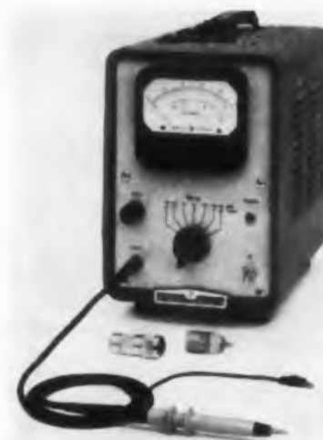
Fig. 11c. Hewlett-Packard. RF Millivoltmeter 411A uses chopper stabilization and a unique feedback system to provide a linear scale calibration from 5 kc to 1 kmc for full-scale voltage ranges from 10 mv to 10 v rms.
