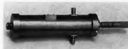
Fig. 11a. Ballantine. A-T Voltmeter 390 uses a continuously adjustable waveguide-below-cutoff piston attenuator to feed a uhf thermocouple whose dc output is read on an auxiliary millivoltmeter. Unknown inputs from 0.5 to 300 v are determined by referring micrometer readings to a calibration chart. Useful from 10 to 1000 mc, the instrument is supplied with an auxiliary millivoltmeter, NBS certification, and calibration curves.
