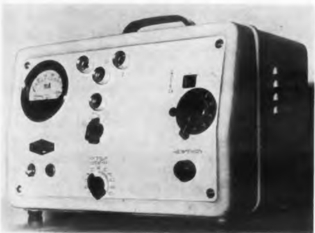
Fig. 7. The Pimel measures the interelectrode capacity of vacuum tubes.
