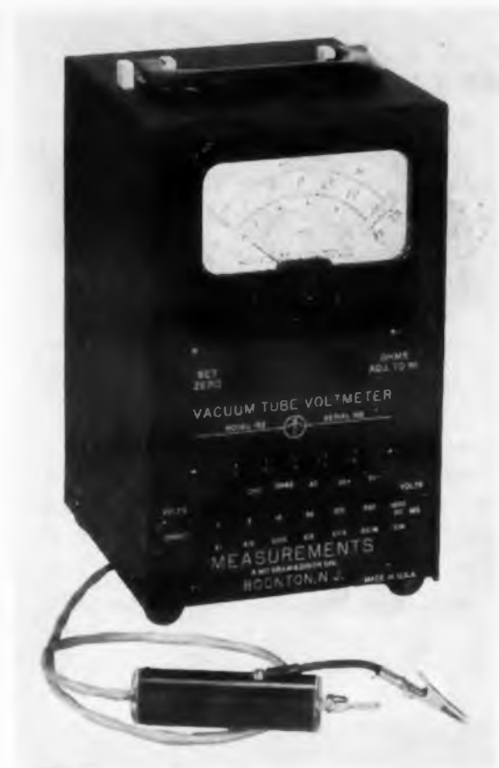
Fig. 12a. Measurements. Vacuum Tube Voltmeter 162 reads ac voltages from 1 v full scale to 300 v in the range from 20 cps to almost 350 mc. It reads dc from 1 v full scale to 1000 v and resistance from 0.2 ohms to 500 meg. On its most sensitive range, instrument can be used as a 0.01- \mu a microammeter.
