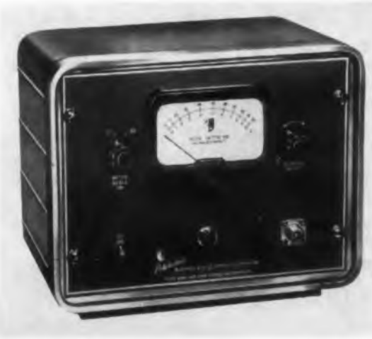
Fig. 16c. Polytechnic Research & Development VHF-UHF Noise Generator 904 covers 30 to 1000 mc with maximum vswr of 1.3. Noise-figure range of 0 to 20 db is narrower than that of Russian unit but noise figures beyond 20 db can be calculated using PRD's instrument. PRD instrument has no restrictions on intermediate frequency or bandwidth.
