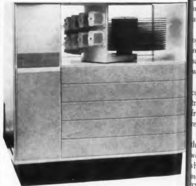
Telex I disk memory has four read-record heads and a head-positioning motor for each disk.
