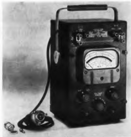
Fig. 12c. General Radio. Vacuum Tube Voltmeter 1800-B covers 0.5 to 500 v full scale for both ac and dc and provides about the same frequency coverage as Russian unit. The G-R instrument does not provide for direct resistance measurements. The 2 per cent accuracy of the 1800-B is better than the 3 per cent which is likely for the Russian instrument.
