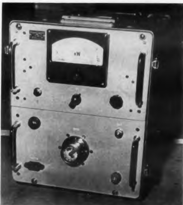
Fig. 4. Power meter IBM-2 measures pulse-power levels from 0.5 to 500 kw over a 30 to 1000-mc range.
