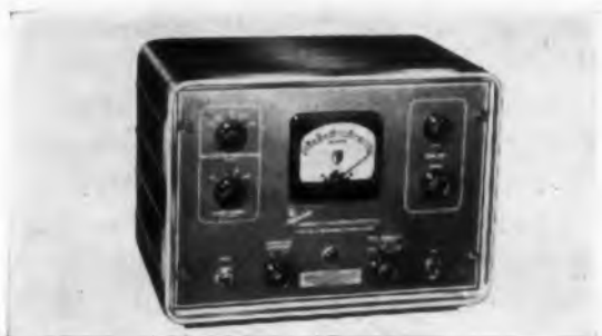
Fig. 14b. Polytechnic Research & Development. Universal Power Bridge 650-A, at maximum sensitivity (100 \mu w) is much less sensitive than the MTO-1, but at minimum sensitivity it can measure higher power levels (100 mw compared with 5 mw). Setting time on the PRD instrument is virtually instantaneous compared with 12 sec for the Russian instrument.
