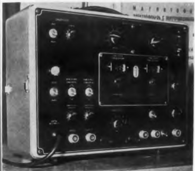
Fig. 2. Pulse generator MGI-1 generates 0.1 to 10- \mu sec wide pulses over a pulse repetition range from 250 cps to 10 kc.
