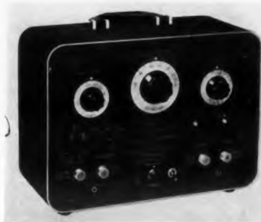
Fig. 2a. Measurements. Standard Pulse Generator 179 has a higher upper frequency limit (60 cps to 100 kc). Its rise and fall times (100 and 150 nsec) are substantially longer than the 6 and 10 nsec times for the Russian unit. Pulse width of the 179 is continuously variable from 0.5 to 60 \mu sec while Russian unit has fixed pulse width of 0.5 \mu sec.
