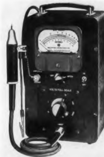
Fig. 10b. Ballantine. Electronic Voltmeter 314 measures 10 mv full scale to 100 v over a 15-cps to 6-mc range. Without the probe, the Ballantine's sensitivity extends to 1 mv full scale. Other Ballantine instruments cover frequencies from 0.01 cps to 6 mc.
