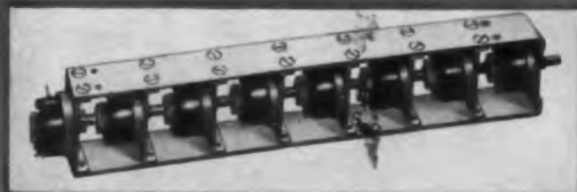
Example of a 360° rotation rheostat with a wire lead tapped winding.
