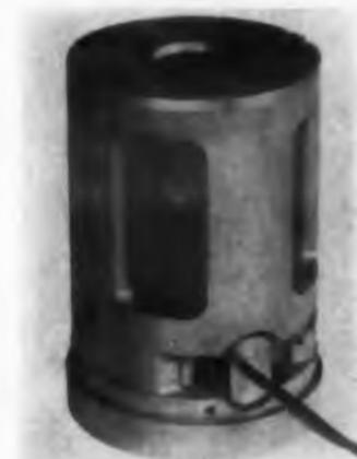
Type PHM pyrotechnic free gyro is for one-time use in short range missiles. Measuring 4.5 x 2.75 in. and weighing about 800 g, the unit stands 100 g shock. It has 2 deg of freedom. Active gyro life is 3 min with an average drift of 1 deg per min.
