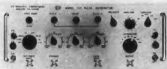
Model 130 pulse generator has a repetition rate of 10 cps to 1 mc, a rise and fall time of less than 10  $\mu$ sec, and two pulse outputs with a relative pulse delay between them of 200  $\mu$ sec to 50 msec. The instrument is suited for fast circuit applications in computer work, transistor testing, and missile applications.
