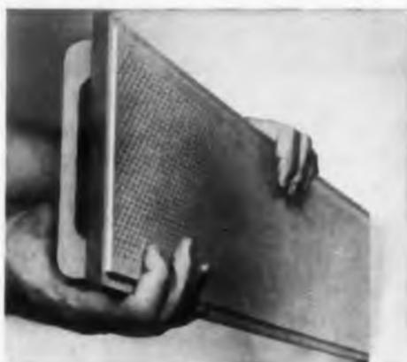
**Melamine Laminates.** Glass cloth or cotton fabric impregnated with melamine formaldehyde resin. Taylor melamine laminates have superior mechanical strength and are especially desirable for their arc-resistant qualities. Good flame and heat resistance, good resistance to the corrosive effects of alkalis and most other common solvents, besides other favorable characteristics. Typical applications include arc barriers, switchboard panels, and circuit-breaker parts in electrical installations.
