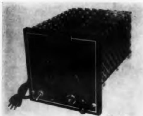
Designed for coupling to an oscilloscope, the Scope-O-Trol accessory unit provides an output of 0 to 300 v dc operating from an input of 115 v at 60 cps. The unit observes on the oscilloscope the regulation, ripple, transient response and other characteristics of dc power supplies by removing the dc component and using the scope to its maximum capacity. Voltage adjustment of the unit is in 75-v steps for coarse adjustment. Ripple is less than 1 mv rms.
