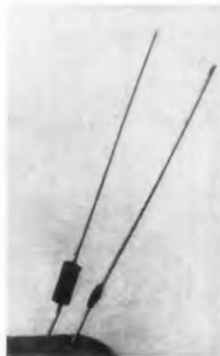
The Ceramin ceramic capacitors measure only 0.25 in. long without leads. Units having a diameter of 0.098 in. are for capacitances of 47 to 560 pf and units with a 0.125-in. diameter, 680 to 1,200 pf. These barium-titanate units are tuned to a tolerance of  $\pm 5\%$  up to 125 C or 10% up to  $\pm 150$  C. They comply with applicable portions of MIL-C-11015A and EIA-SMC-1 specs.
