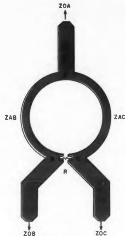
**Fig. 1.** The stripline directional coupler with a 3-db insertion loss shown here is designed about a simple path-length difference.
