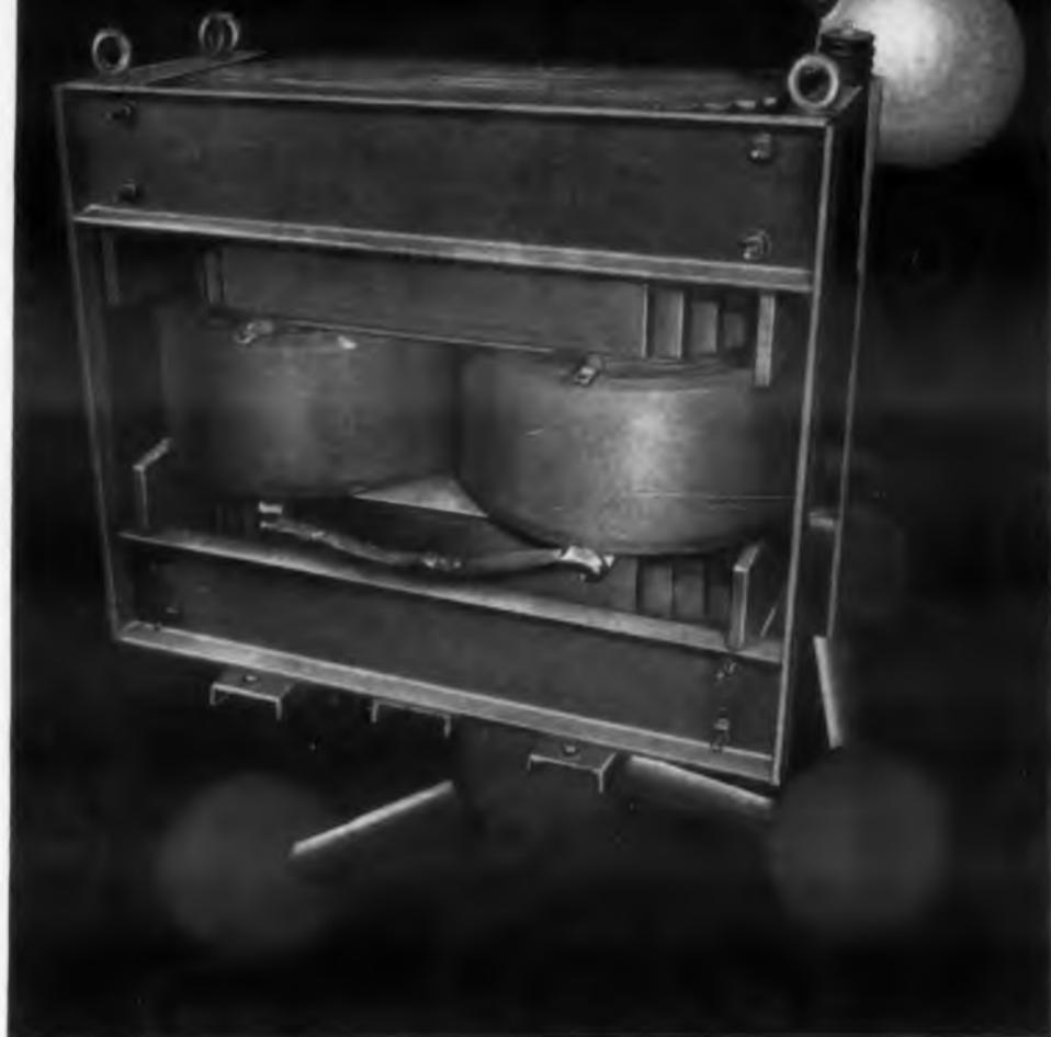
The unit illustrated is the largest transformer manufactured by NWL. It can be made in either air, air-blast or oil-filled versions. The pulse transformer has an output of 10,000 ampere pulses at 1000 volts. The approximate weight is 11,000 lbs. This transformer is typical of the many special units currently being produced by NWL. Pulse transformers can be manufactured up to 200 KV and up to 50,000 KW peak power.
