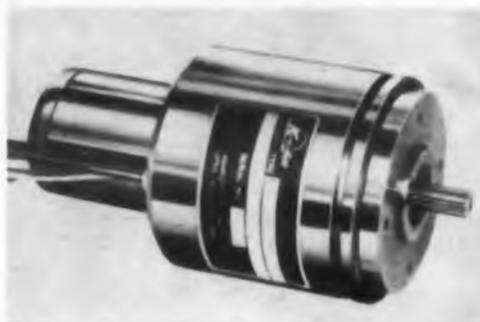
This size 23 precision servo motor-generator is designed for application as a rate servo and to provide damping in very high gain systems. Motor stall torques are available from 5.5 to 9 in.-oz. No-load speed is 9,000 rpm. Generator characteristics include 2.9 v per 1,000 rpm and a linearity of 0.2% to 3,600 rpm. The unit is available with either a plain or pinion shaft.
