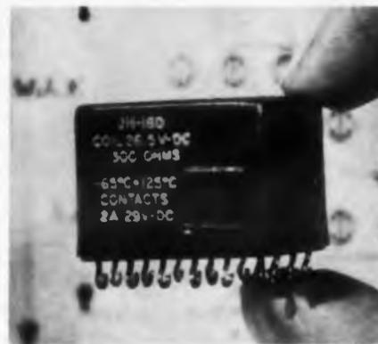
Type JH-18 6 pdt miniature relay has 0.2 in. grid spacing, 2-amp contacts, and occupies less than 1 cu in. of space. It weighs less than 1.8 oz. Standard coils include nominal voltage ratings of 6 to 115 v dc with a power rating of 2.5 w. Dielectric strength is 1,000 v rms at sea level or 750 v rms across open contacts. Insulation resistance is 1000 meg min. The unit stands shock to 50 g and vibration of 28 to 2,000 cps at 20 g or 5 to 28 cps at 0.5-in. double amplitude.
