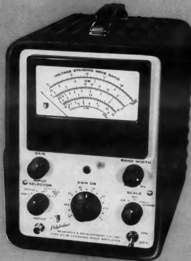
The new portable PRD 277-B Standing Wave Amplifier is designed to meet the present and future needs of microwave test laboratories. Due to its extremely low inherent noise, 0.007  $\mu\text{v}$ , weak signals which once were undetectable by conventional instruments can now be measured. Attenuation in 5 db steps combined with 4 VSWR scales and a large meter permit VSWR measurements to be made with maximum resolution and accuracy.
