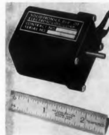
This solid state, subminiature servo drive system has a volume of 1.75 cu in. and delivers a torque of 2 in.-lb from a change of 0.001 v. Actuator arm speed is 270 deg per sec. The device consists of a servo amplifier, a precision gear train and a high-torque servo drive motor.
