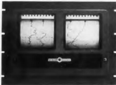
\*Varian offers rack mounted versions too—either singles or twins. The latter is pictured, showing how four channels of recording can be fitted within the 19-inch width of a standard rack.
