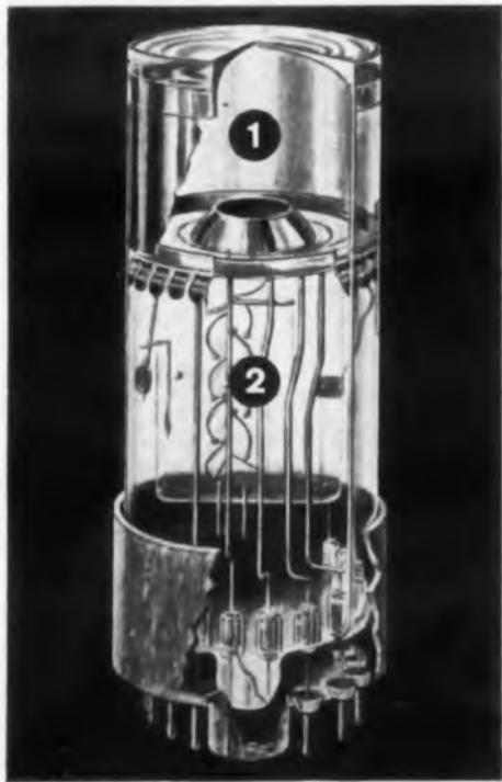
CBS LABORATORIES new line of photomultipliers are specially designed for counting or scanning applications.
