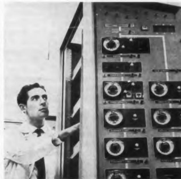
Project Mercury display console is checked over before shipment from Stromberg-Carlson-San Diego, Div. of General Dynamics Corp., to Cape Canaveral. Several control center consoles built under subcontract to Bell Telephone Labs have been delivered to the Cape and Bermuda, where another control station will be located. A Project Mercury flight controller team will monitor data about an astronaut, the capsule and the flight.
