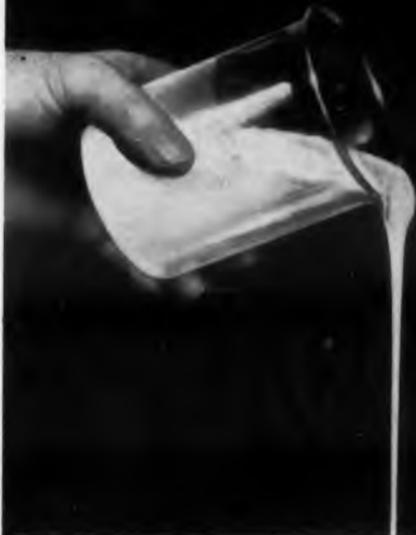
The latest addition to General Electric's RTV family offers lower viscosity than any other available silicone rubber compound — a typical viscosity of 120 poises. Easily pourable, it flows freely in and around intricate contours, making it ideal for protecting electrical and electronic components.
