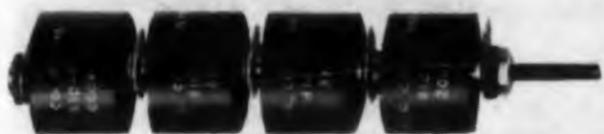
The Series 400 R-Stack wirewound resistors have screw-mounted, bushing-terminated resistance elements. Tolerance is 1% through 0.005%. Units measure 1/2 in. in diameter, 3/4 in. long for 1/2-w resistors and 7/8 in. in diameter, 15/16 in. long for 1-w resistors. Mil specs are met.
