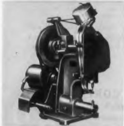
High speed automatic setting of Funnel Flange Eyelets with United Eyeletting Machine Model G.
