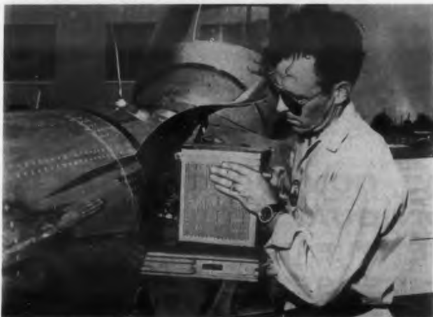
Fig. 1. Grant slides provide access to equipment which must be mounted in "impossible to reach" places on Douglas Interceptor.
