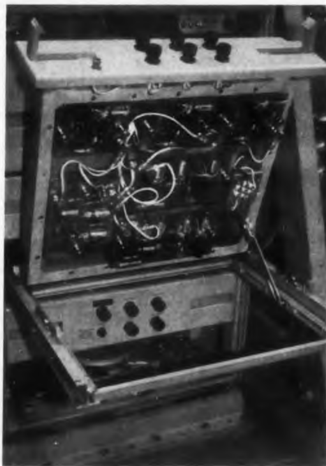
Fig. 3. Chassis slides out to give top access, then tilt up for bottom access.
