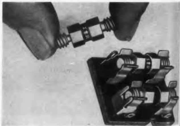
Fig. 7. International Rectifier Corp.'s plug-in rectifier extend plug-in concept to component level.
