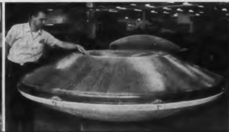
3 92-inch Cassegrain antenna built for U. S. Army Nike-Hercules radar.
