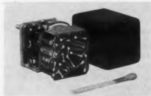
Fig. 23. Lear's expendable module, with flexible PC board, has all input, output, and reference signals conveniently available for maintenance at the header. The 1 cu-in. module is available with several basic configurations.
