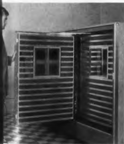
Fig. 7. Pages in the book-shaped layout of large-scale, Control Data Corp. computer can hold 1,000 PC-card modules as well as magnetic-core arrays.
