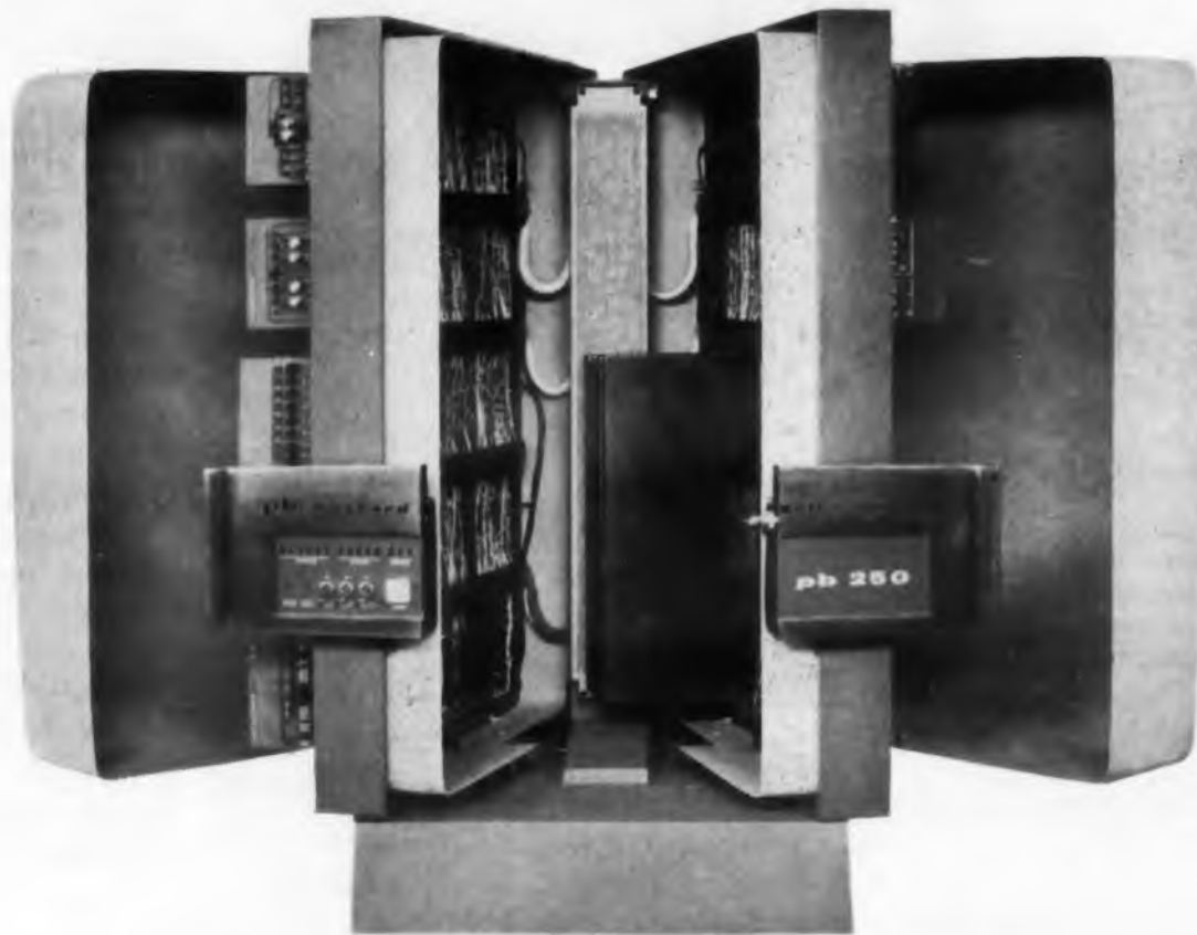
Fig. 5. Computer opens to expose pages of wiring and input cables which travel up spine and branch out to logic modules.
