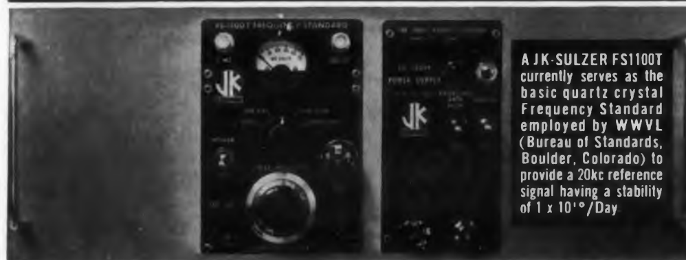
Total Dimensions, Standard and Power Supply: 7 \frac{1}{2} "W x 6"H x 12 \frac{1}{2} "D. Shown mounted in 7" x 19" rack panel.
