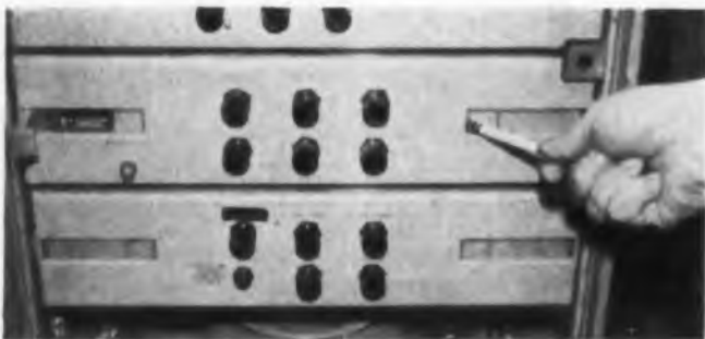
Fig. 2. Push-to-unlatch catches give quick access to drawer-mounted chassis.
