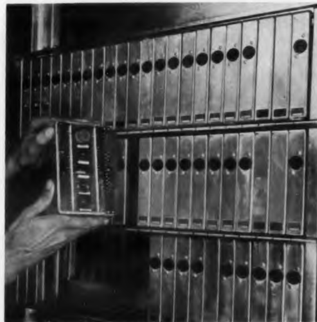
Fig. 9. Only 11 basic modules serve entire numerical control system designed by Hughes Aircraft Co. Unusual modules have components neatly stacked in cordwood fashion and soldered in slots in plastic spacers.
