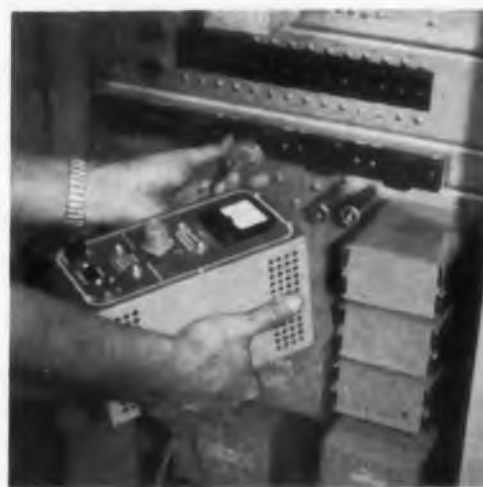
Fig. 11. Convenience outlets (left) on NATO communications receiver allow test equipment and tools to be plugged in right at working area.
