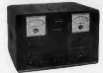
*MODEL 1803 TRANSISTOR PARAMETER TEST SET Measures the small signal "h" parameters and wide range of I_{co} .
