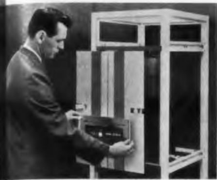
Fig. 4. Book-shaped Packard Bell computer slides out of "book-case" in rack version; sits on cast base in desk-top model.
