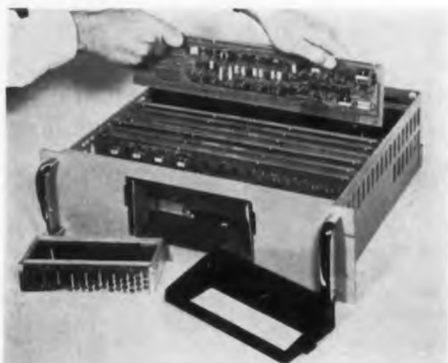
Fig. 17. More than 99 per cent of the components on this Non-Linear Systems digital voltmeter are on plug-in modules. Even the digital readout snaps out for easy lamp replacement.
