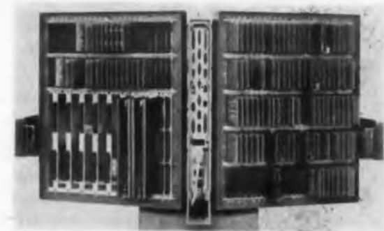
Fig. 6. Back of book exposes connections and plug-in modules of which there are only 13 types.
