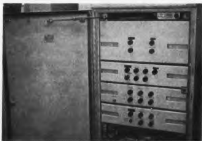
Fig. 1. Swing-out door provides rf shielding and drip-proofing for drawer-mounted chassis in this piece of Lockheed equipment.
