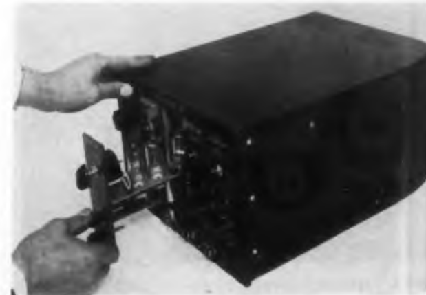
Fig. 19. For higher component densities, AWA isolates functions to specific plug-in blocks.
