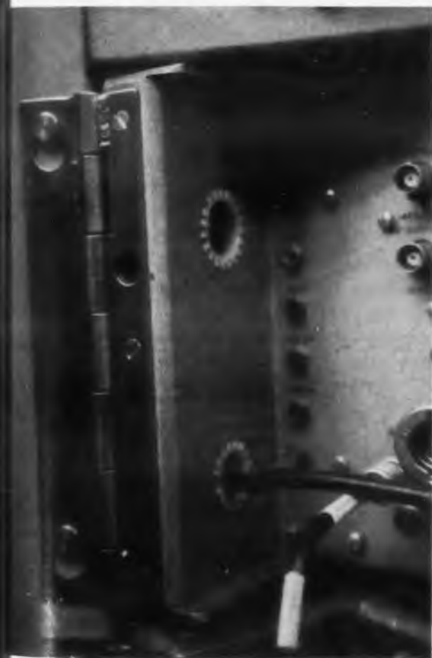
Fig. 14. Performance-monitor panels on BMEWS communications equipment, designed by REL, are mounted on hinges which are secured through special slottings. Panel can be swung out or removed entirely.
