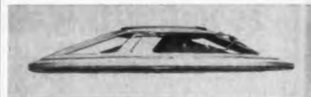
Fig. 1. "Flat" speaker for portable radios has over-all thickness of 3/4 in.
