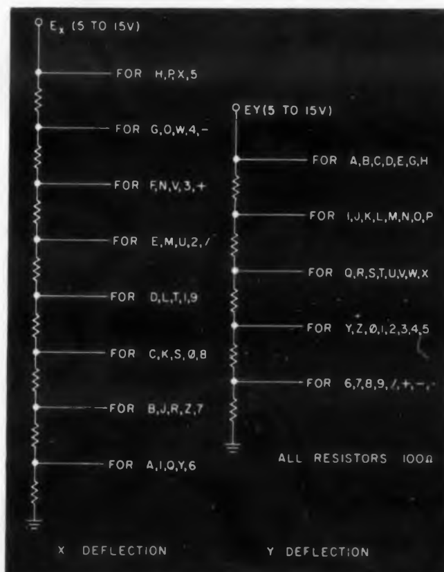
Fig. 1. Crt electron beam is positioned at sub-origin, from which dot pattern is generated, by voltages from two divider networks—one for X-axis coordinate and other for Y-axis coordinate.
