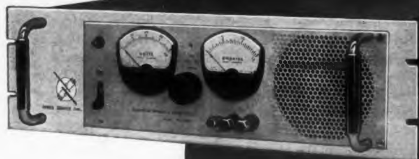
Model PS4315M 0-36 volts DC out at 15 amp maximum
