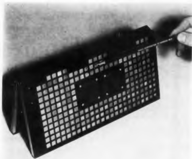
Fig. 38. Mock-up of Micromodule digital differential analyzer designed for use with an inertial guidance system by RCA's Missile Electronics and Controls Div. Corrugated metal sleeves surrounding each module serve as shock isolators and also are used to provide heat transfer to the frame.
