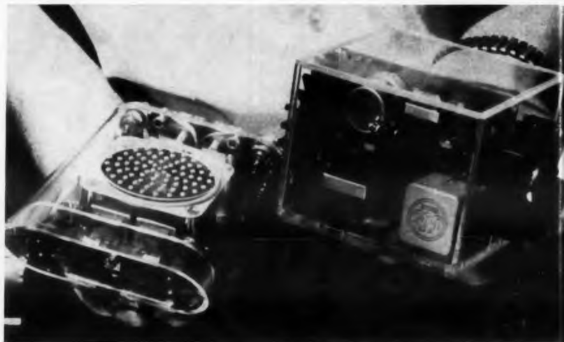
Compact transistorized receiver package that goes in car and oscillator unit which sends out low-frequency signals from road in GM's Electro Lane.
