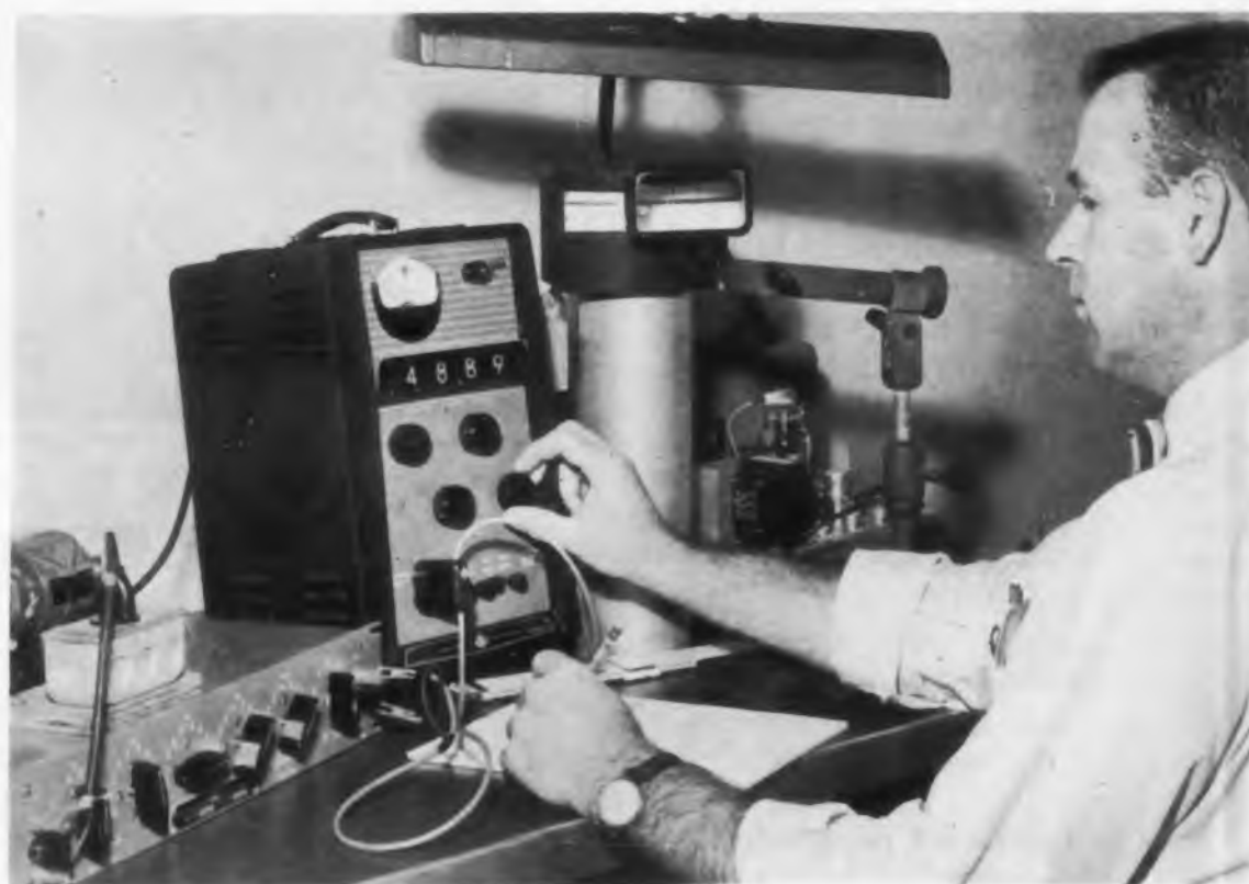
True rms vtvm used to check frequency response of precision dynamometer.
