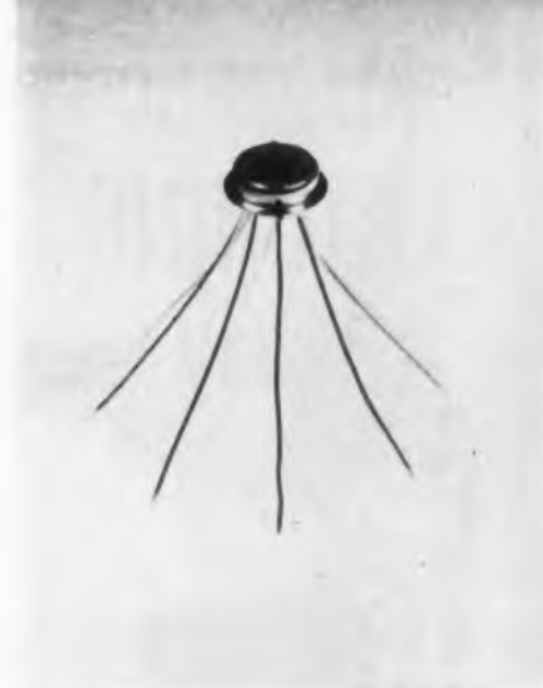
Fig. 27. Sperry-manufactured integrated "Semi-Nets" are encased in TO-5 transistor cans.
