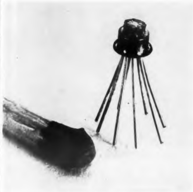
Fig. 25. Silicon Micrologic blocks packaged in miniature transistor cans with eight leads are under development at Fairchild Semiconductor Corp.
