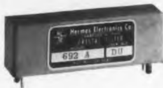
Hermes Crystal Filter, Model 692A, shown half size, occupies only 1.5 cu. ins.
