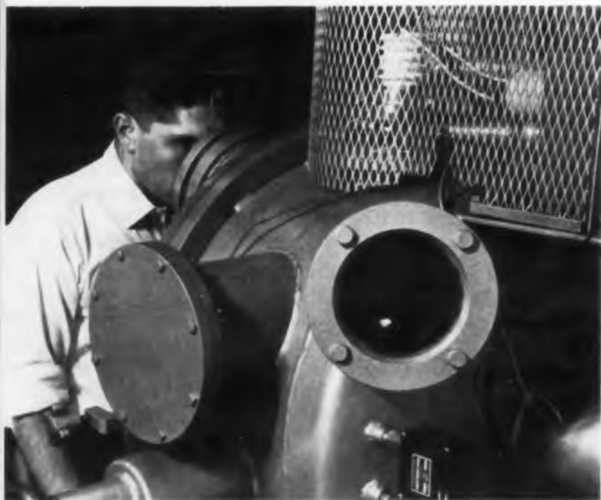
Fig. 30. Electron beam welder developed by NRC Equipment Corp., Newton Highlands, Mass., produces welded joints in vacuum. This machine costs about $17,000.
