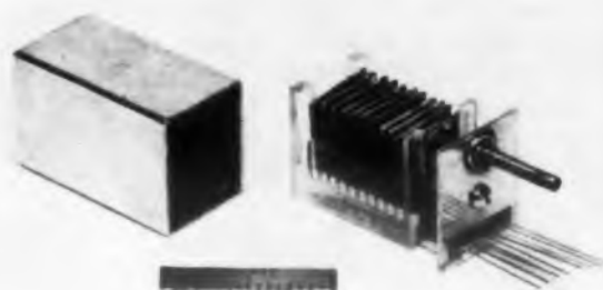
Fig. 35. Wafer interconnection scheme developed by Diamond Ordnance Fuze Laboratories makes use of nickel ribbons from wafers, which are spot-welded to various interconnecting rods. The rods are then rolled down flush with the back of the plastic block and fastened. Wafers are replaced easily by unrolling the rods, right, and clipping the ribbon leads. Blocks are about 1-in. long. Assembled unit shown below.
