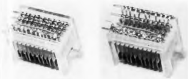
Fig. 35. Wafer interconnection scheme developed by Diamond Ordnance Fuze Laboratories makes use of nickel ribbons from wafers, which are spot-welded to various interconnecting rods. The rods are then rolled down flush with the back of the plastic block and fastened. Wafers are replaced easily by unrolling the rods, right, and clipping the ribbon leads. Blocks are about 1-in. long. Assembled unit shown below.
