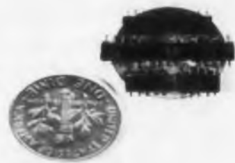
Fig. 23. Seven solid-circuit multivibrators, made by TI, can sit on a dime, with room to spare.
