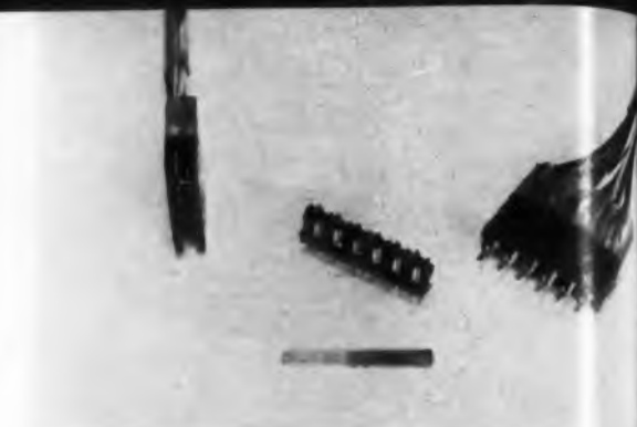
Fig. 43. Various micromin connector configurations are illustrated with these Elco connector units. Potting strengthens joints.
