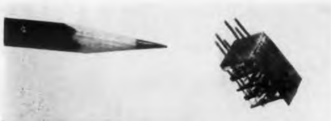
Fig. 36. Two basic interconnections approaches are being explored by IRC for its Mu Circuits. The vertical approach makes use of 3-layer Lamoflex flexible printed wiring to interconnect thin-film circuits deposited on glass wafers. Riser wires along the opposite edge of the package are also used for connections. In the horizontal approach to interconnections, encapsulated circuits are interconnected by means of plated-through holes and solder joints.
