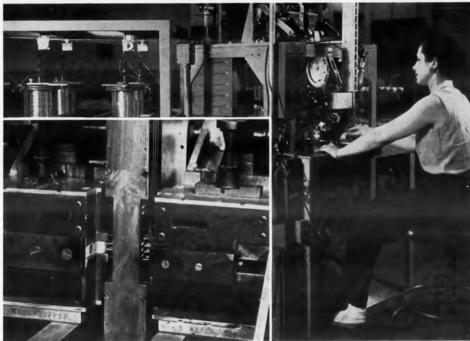
Fig. 12. Electric weld heads, inset, flow solder on heavily pretinned riser wires to make joints to wafer notches in this automated module assembly machine designed by Paktron. Wafers are fed from vertical magazine, in front of operator, and wires from spools at left.
