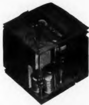
Fig. 2. A model of a welded package showing component arrangement and interconnecting ribbon used to tie components together.
