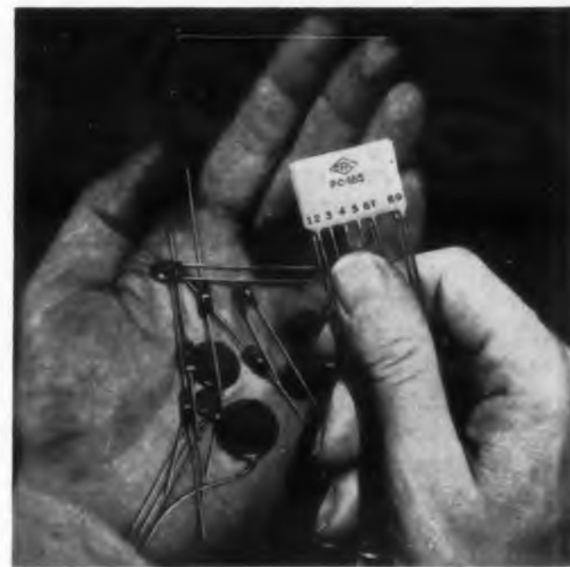
Fig. 7. Centralab, with PECs, was an early supplier of packaged components to replace conventional parts in miniaturization programs.
