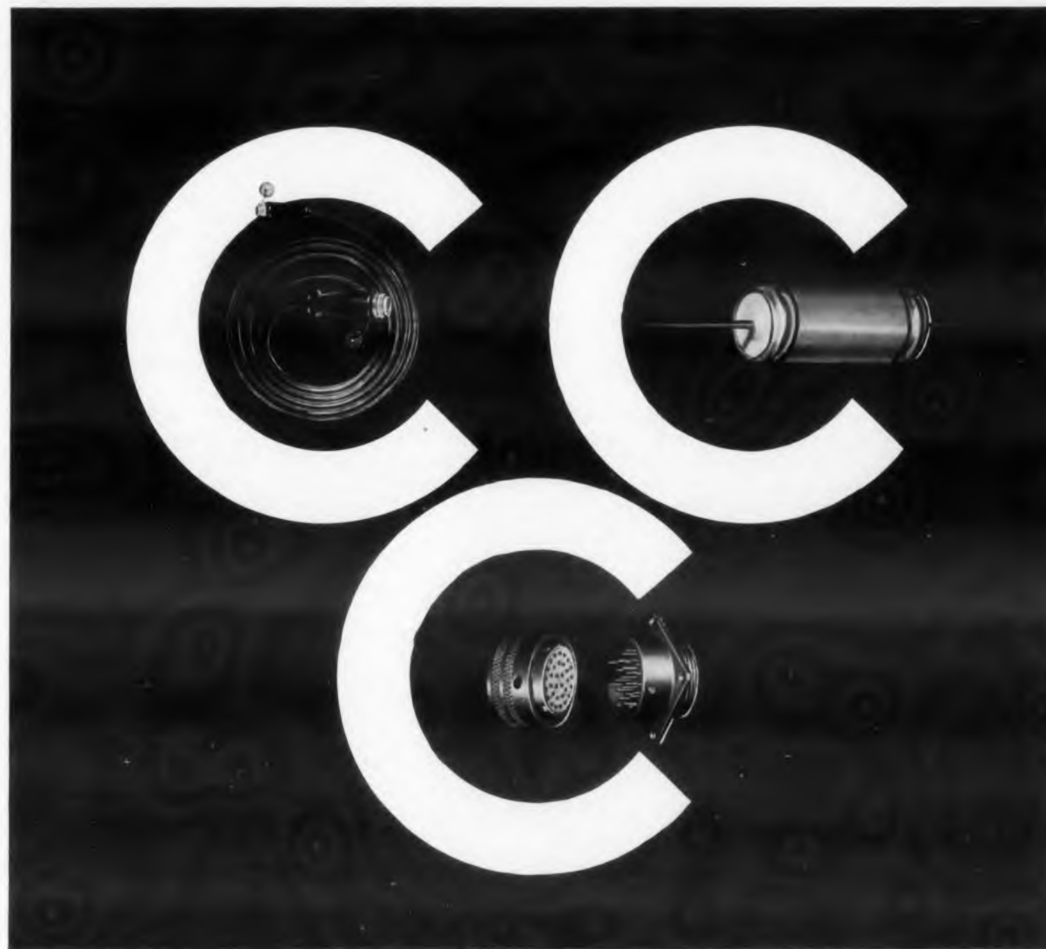
Fig. 5. GE has automated production of welded modules by using standard termination strips. Odd shapes possible with welded approach are illustrated by curved module, upper right.
