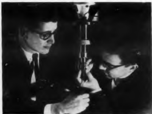
Calcium fluoride optical maser is prepared for experiment by IBM scientists Peter Sorokin (left) and Mirek Stevenson. The maser crystal is at the bottom of the assembly. Above it is a liquid helium-filled dewar flask.
