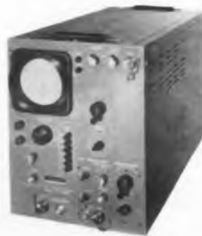
2-Channel Oscilloscope 455 Has 0.4 Nsec Risetime
