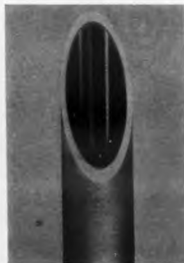
The spectrum-conserving, 2-in. circular waveguide , under development at Bell Laboratories, will create a "private atmosphere" to transmit 10 times the information now carried by microwave link, with no interference possible.
