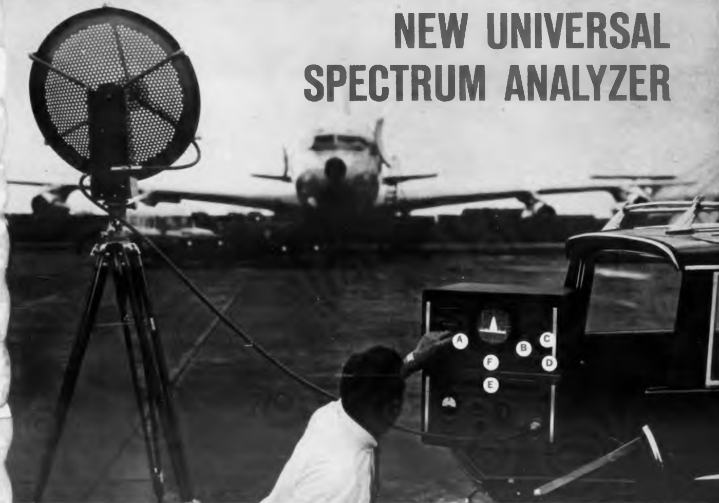
Polarad Model SA-84W being used to make pulse analysis of radar aboard a Pan American Boeing 707, Jet Clipper®
