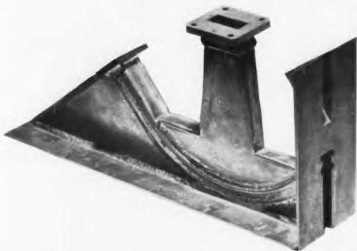
Fig. 6. This large antenna feed could hardly be manufactured to tolerance by any other type of nickel plating method except the zero-stress sulfamate electroforming process.
