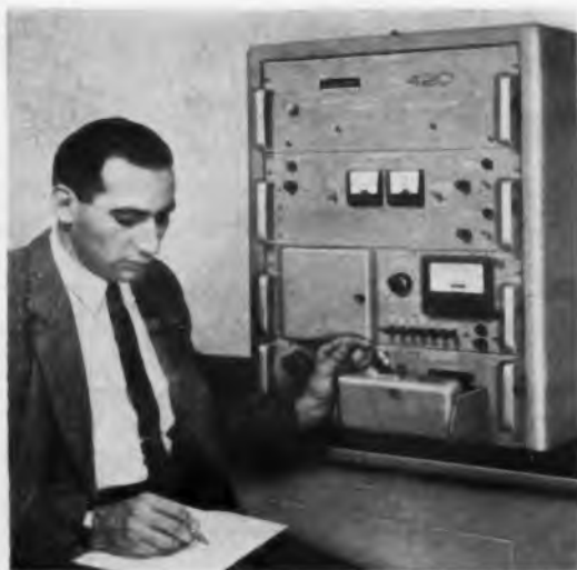
Charles Askanas is shown checking transistor switching speed on Lumatron's Automatic Switching Time Test Set.
