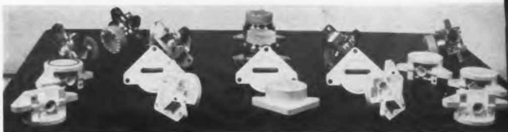
Fig. 7. These examples of C-band antenna parts illustrate the complex shapes that can be accommodated, and the ability to work with quartz parts as easily as metal.
