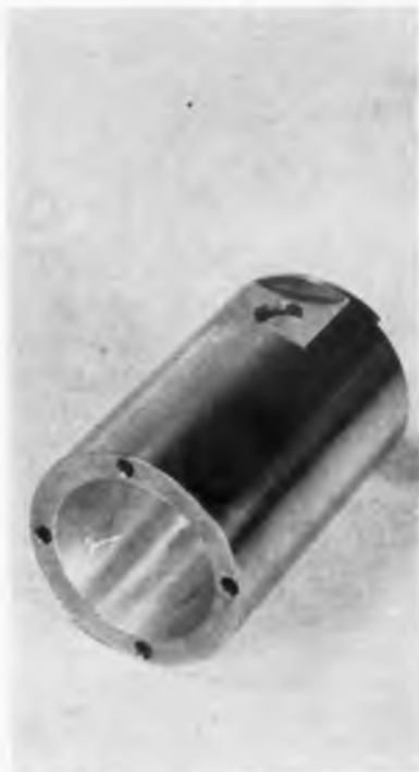
Fig. 1. Microwave tuning cavity produced with reusable mandrel, holds tight ID tolerances.
