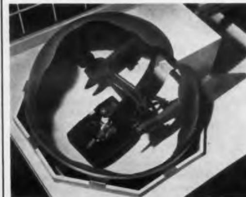
Manned space flight simulator (CVPR-2996) will demonstrate earth orbiting and landing, moon and interplanetary flights, satellite rendezvous missions, lunar landings and launchings.
