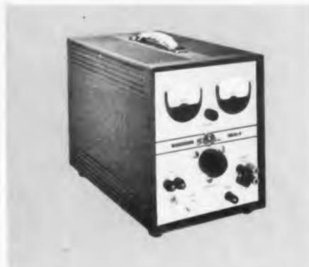
**New portable** fully transistorized d-c power supply. QR36-4AP regulates 0 to 36 vdc output voltage to  $\pm (0.02\% + 1\text{mv})$  against combined line or load variations. Fully metered. Front panel terminals for remote sensing. *Circle 224 on Reader Service Card.*
