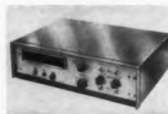
Model 851 is a solid-state, digital frequency-time meter designed for inexpensive application. Basic units are two identical 1-2-4-8 binary-coded decimal counting trains in combination with a pair of input-amplifier channels and a switching unit. Readout may be by Nixie or a lamp system. The set is easily made compatible to control and data systems. Panel height is 5-1/4 in.
