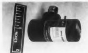
Designed as an acceleration sensing switch, the A9548-01 has a threshold sensitivity of 0.150 g  $\pm 25\%$ . Damping, springs, mass, or material can be varied in the 0.1- to 5-g range. Contacts are rated at 0.1-amp noninductive. The hermetically sealed unit meets requirements of MIL-E-5272C. It may be used as a tilt switch, with threshold at a tilt angle of 8-1/2 deg.
