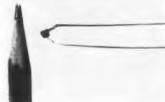
The "Wee Con" series of dipped phenolic-coated, plate ceramic capacitors have rectangular shape and are subminiature in size. They are available in six sizes from 0.150 x 0.150 x 0.100 to 0.600 x 0.500 x 0.150 in. Capacitances range from 10 pf to 0.036  $\mu$ f, working voltage is 200 v dc.
