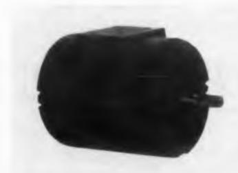
The G frame series of ac motors range from 1/400 to 1 1/4 hp. Windings are induction or hysteresis synchronous, 1- or 3-phase. Motors are self-cooled or totally enclosed, finned or plain. Ambient temperature range is  $-55$  to  $125$  C. Units operate on 60 cps. and are offered with or without mounting base.
