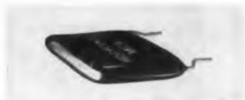
Type MCA epoxy-dipped mylar capacitors are 0.525-in. wide and 0.225-in. thick at 0.01  $\mu$ f. Operating temperature range is  $-55$  to  $100$  C, or to  $125$  C with 50% voltage derating. Capacitance change is 1.5% at  $85$  C. Power factor is less than 1% at 1 kc and  $25$  C. Values range from 0.01 to 0.33  $\mu$ f.
