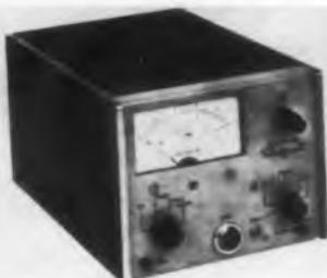
Model 431A power meter has a drift stability of less than 2  $\mu$ w per deg C over a range of 1  $\mu$ w to 10 mw. One zero adjustment is needed for all seven ranges. The meter face is also calibrated in dbm with 5 db between ranges.
