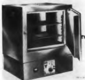
Made for accelerated aging tests, these gravity convection ovens provide temperatures to 650 F. A saturable power reactor control system gives stepless, switchless and infinitely proportional wattage for straight-line, repeatable temperatures throughout the range. There are 4 standard sizes, up to 37 x 20 x 25 in. internal dimensions.
