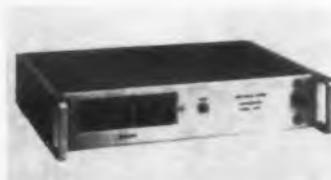
Model 5275A time interval counter provides digital measurements of time intervals over a range of 10 nsec to 0.1 sec. Counted frequency is 100 mc and resolution is 10 nsec. The unit has remote reset and four-line BCD electrical output.
