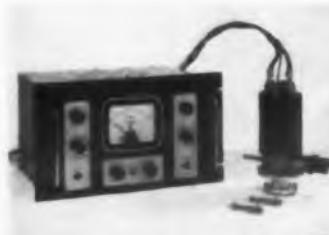
A mass spectrometer amplifier, model 51A will discriminate currents as low as  $10^{-16}$  amp quickly and reliably. Response time is 100 msec to 5 sec. A vibrating capacitor modulator reduces warm-up time. Voltage sensitivity is controlled over four decades with 10 steps per decade. Zero drift is  $\pm 100$   $\mu$ v over a 12-hr period.
