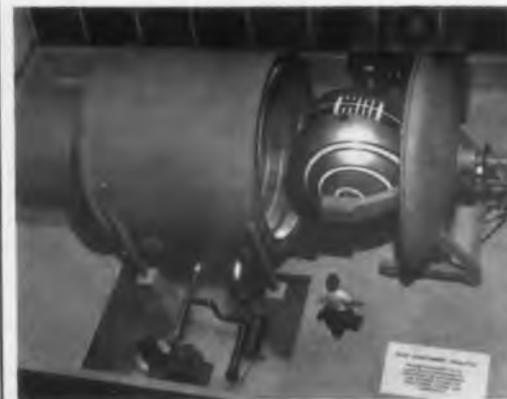
Space environment simulator (CVPR-2997), as depicted in scale model, will test payloads nearly 8 ft in diam by spinning and rotating them to duplicate their positions relative to the sun.
