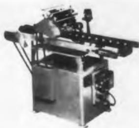
Model RG is a conveyor type machine for printing cylindrical pieces such as capacitors, tubes, etc., at a printing rate of 3,600 units per hr. Model B3-2F is a hand-operated machine for printing serial numbers in a minimum of space.
