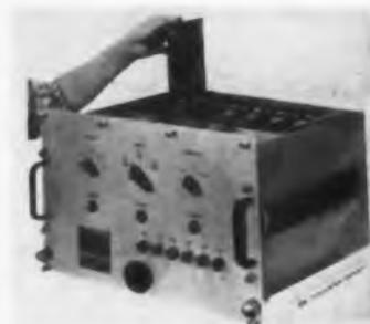
Developed for use in automatic checkout applications, the model M7 multimeter is a solid-state, analog-to-digital converter. Frequency measurements from 1 cps to 100 kc, to an accuracy of 0.01%  $\pm 1$  count, can be made in 0.1 sec. Periods from 0.001 to 0.1 sec can be measured to an accuracy of 0.01%. Voltage and resistance ranges extend to 1 kv ac or dc and 1 meg. The requirements of MIL-E-16400 are met.
