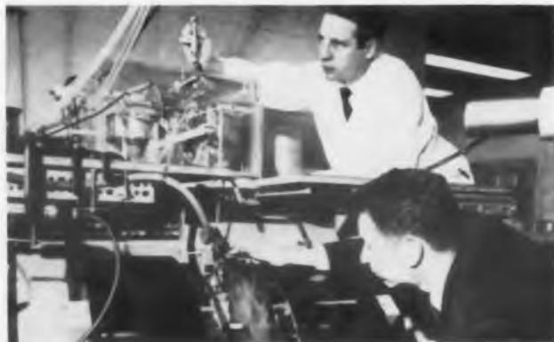
**Antiferromagnetic isolator** is tested at 140 kmc with carcinotron signal source. Isolator, in liquid nitrogen Dewar between poles of the large electromagnet at bottom of photo, is adjusted by Dr. Gerald S. Heller, leader of the Resonance Physics Group at Lincoln Laboratory. At top, John J. Stickler monitors carcinotron output. The tube is said to average 20 mw of power within a 7 per cent tuning band.
