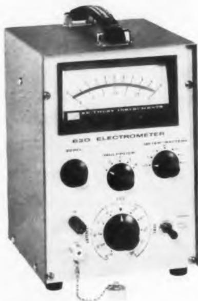
**MODEL 620** Battery-Operated Electrometer offers 31 ranges.
