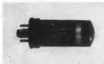
A mercury-wetted contact relay, series V51 is designed to give over a billion reliable operations with complete freedom from contact bounce. Operate time is 3 msec min; release time is about 3 to 3-1/2 msec. Contact and armature assemblies are hermetically sealed in a glass capsule with a hydrogen atmosphere. Switching speed is 100 operations per sec. The relay will switch 250-v-a loads with a maximum of 5 amp, 500 v. Diameter is 1.105 in., height 3.196-in., weight is 4 oz.
