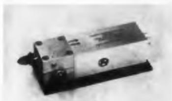
Model CP49 combines a variable reluctance pressure transducer and a dc-energized carrier-demodulator in a single package. Ranges are 5 to 10,000 psi, gage, differential, or absolute. Overpressure is 700 psid or 200% of range; zero shift with line pressure is less than 1% full scale. With an output of 0 to 5 v dc, the unit is regulated against input voltage changes from 25 to 30 v dc. Linearity is within 1/2%, hysteresis within 1/2%. Ambient temperature is  $-65$  to  $250$  F.
