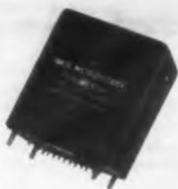
Type 33-5947 analog multiplier-divider is applicable to any type of analog process control in military or industrial instrumentation. It accepts 3 dc analog input voltages and forms a proportional output. The unit may also be connected to square, find geometric means, extract square roots and solve quadratic equations. The solid-state device has a frequency response of 50 cps. Accuracies are  $\pm 0.5\%$  as a multiplier and  $\pm 1\%$  as a divider.
