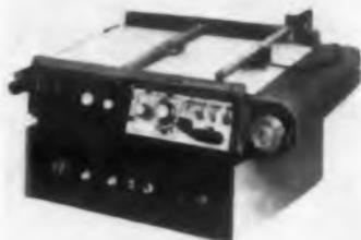
Any time delay encountered in a process control or experimental situation may be reproduced by the model 2D-5 transport delay simulator. It consists of a controller, a standard X-Y recorder, and an optical line follower. Delay time may be varied in steps from 2 to 32 min, or continuously from 4 sec to 7 min. Slopes up to 80 deg can be tracked to within 0.05 in. at speeds through 15 in. per min. An alarm circuit detects errors up to 0.1 in.
