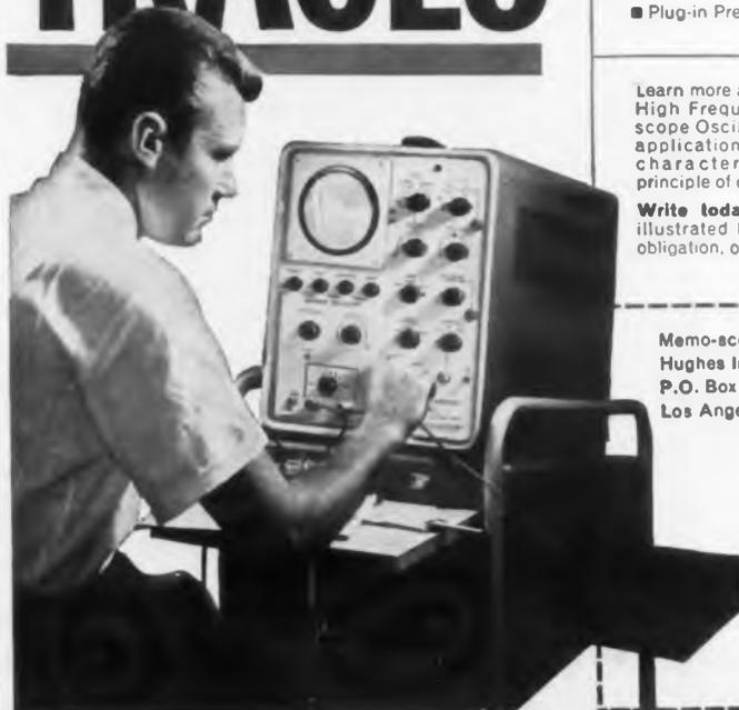
The all-new Hughes High Frequency Memo-scope® Oscilloscope saves you time and money in transient analysis. With its 10 mc bandpass and one million inches per second writing speed, it can store fleeting phenomena for an indefinite period of time. It displays these non-recurring transients for thorough study until intentionally erased. In this way, you can eliminate expensive "hit or miss" methods of transient analysis.
