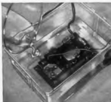
LTV-602 is easily applied, flows freely in-and-around complicated parts. Having a low viscosity in the uncured state, 800-1500 centipoise, LTV is ideal for potting and embedding of electronic assemblies. Unlike "gel-like" potting materials, LTV-602 cures to a flexible solid. Oven cure is overnight, or from 6 to 8 hours at  $75$  to  $80^{\circ}\text{C}$ .
