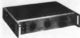
Model 457A ac to dc converter has a conversion accuracy of  $\pm 0.3\% \pm 2$  mv from 50 cps to 50 kc. When used with the firm's model 405 BR CR digital voltmeters it provides ac voltage measurements with three-digit resolution and an over-all accuracy of  $0.5\% \pm 1$  count,  $\pm 0.002$  v. Attenuation ratios are 1 to 1, 10 to 1, 100 to 1, and 1,000 to 1 with highest rated input of 300 v rms.
