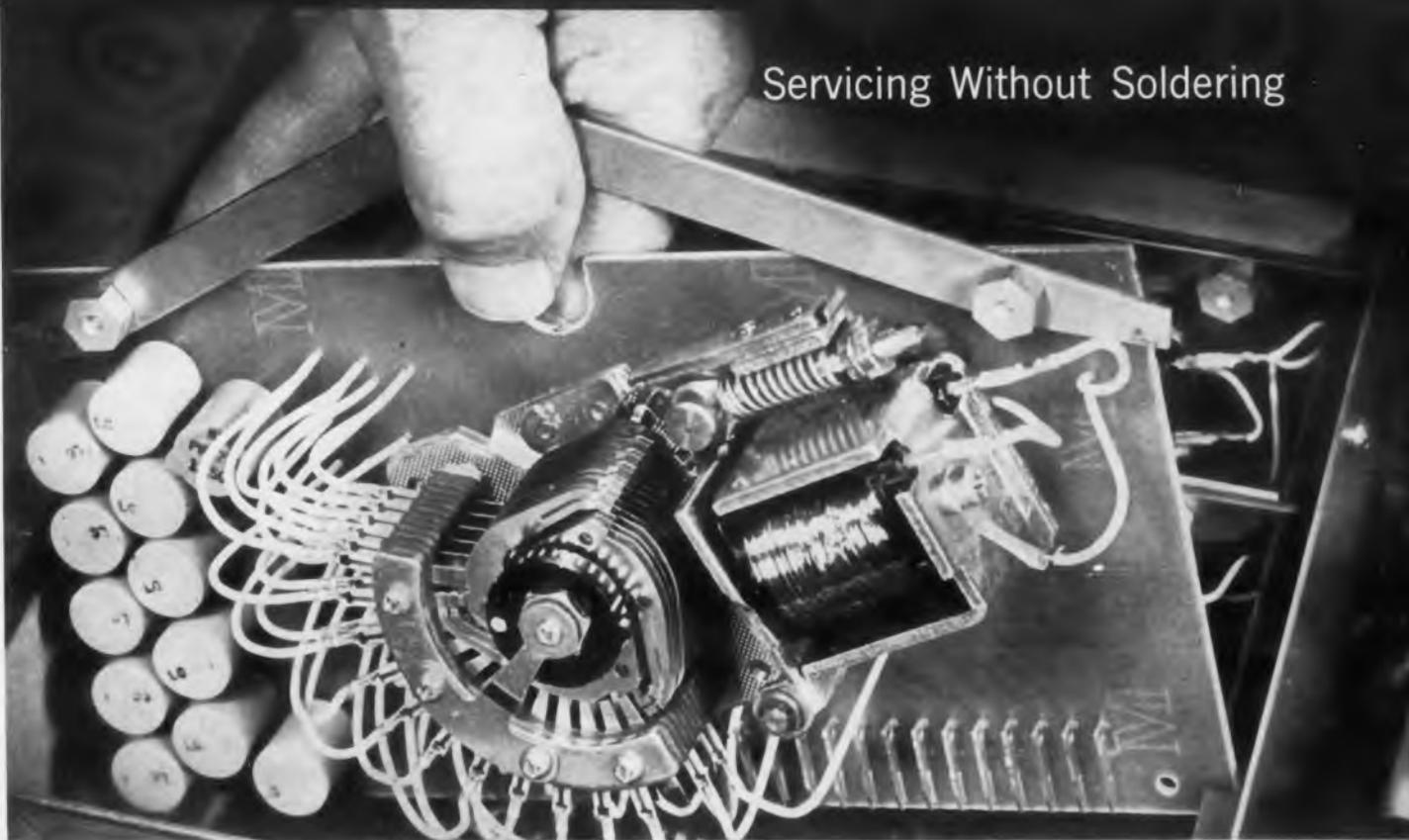
The new NLS 481A digital voltmeter features both plug-in stepping switches and a snap-out readout that virtually eliminate use of a solder gun or other tools in servicing. Note the "finger-control" leverage bars for easy switch removal.
