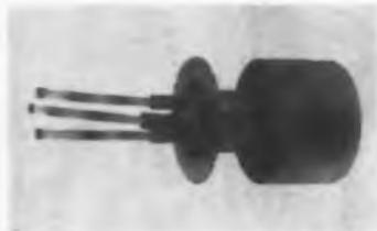
A forced-air cooled triode, type 7900 has a specially processed platinum grid for lower drive power requirements. It is designed for power amplifier use up to 220 mc, and is particularly suitable for TV applications. Class B power output, at 220 mc in an approved cavity, is 5.6 kw. Plate dissipation rating is 4 kw.
