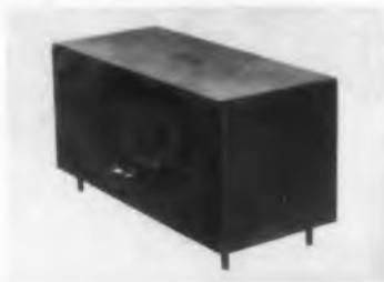
The DL-1000 series of lumped constant delay lines achieve delay-to-rise time ratios as high as 175 to 1. They are available in delays to 500  $\mu$ sec with impedances ranging from 100 to 1,000 ohms. Operating ambient temperature range is from  $-55$  to  $+125$  C.
