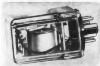
Class 88CP is a clapper-type relay with 8- or 11-pin octal plug and transparent plastic enclosure. Contacts are silver alloy, spdt, dpdt, or 3pdt, rated at 10 amp. Actuation may be 6, 12, 24, or 115 v ac or dc current. Over-all dimensions are 1-3/4 x 1-3/8 x 2-1/16 in. above socket.
