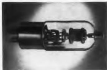
A half-wave, high-vacuum rectifier tube, the 3B24WA has a shock rating of 450 g. The JAN tube has filament voltage of 2.5 v at 3.0 amp ac. Peak plate current is 300 ma; piv is 20 kv. It is designed to operate in installations subject to shock, vibration, and filament fatigue.
