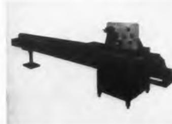
Model 150AB is a semiautomatic marking machine for color-banding and imprinting axial-lead components. It can simultaneously color-band up to six colors, print variable data, or both color-band and print at rates up to 7,000 units per hour. Axial-lead components up to 1/2-in. in diameter and 2-in. long can be handled.
