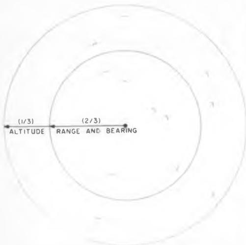
**Possible altitude** display system now being developed for the FAA uses the inner two-thirds of a ppi as a conventional range azimuth display. The outer third of the tube face is calibrated in altitude, so that an altitude pip for each aircraft appears on the same azimuth as the range-and-bearing pip. Aircraft at higher altitudes are shown toward the outside of the altitude sector.
