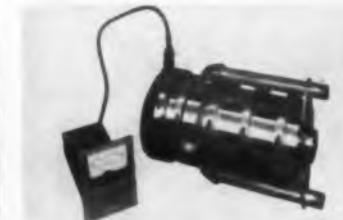
Designed for use with water brakes and other auxiliary-driven, power-absorbing devices, the series PT torquemeter has no rotating or moving parts. The pickup is installed in the same manner as an adaptor flange, and is available in sizes from 200 to 20,000 in. per lb. The rotating shaft of the unit under test passes through the center of the pickup without contact.
