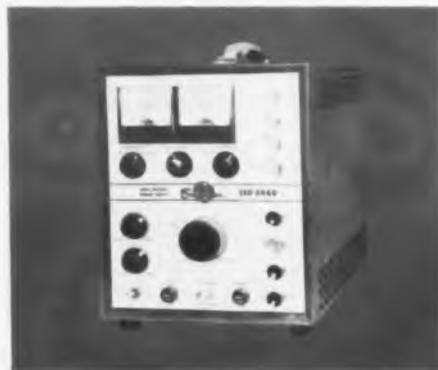
**New portable high-voltage supply** Model 230-6P has unusually versatile controls, unusually complete protective features for a unit of its size. Rated: 0-30,000 vdc, at 0-6 ma. Reversible polarity. "Coarse" and "Fine" front-panel voltage adjustments. *Circle 225 on Reader Service Card.*
