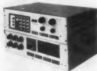
The model F decimal converter changes potentiometer input resistances to decimal output. It is compatible with any equipment having maximum output resistance of 5 K. Decimal readings are obtained in a single scan from a resistance bridge. An error detector prevents readout if the converter balances incorrectly or if the input changes during balancing.
