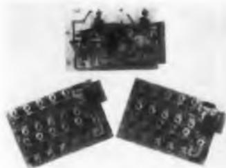
This quarter-square law multiplier can operate in four quadrants, and employs silicon junction diodes in the squaring networks. The multiplier has a static accuracy of 0.025% and extremely high dynamic response. Amplitude error is 0.5%; phase shift is 0.1 deg at 100 cps. Computing networks are mounted on printed-circuit, plug-in cards. All calibrations are made at the factory; no field adjustment is required.
