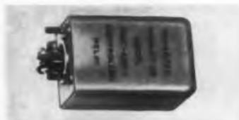
The RMC-400-1 is a magnetic amplifier controlled relay designed for bias protection in airborne radar systems. Specifications are: power required, 102 v, 380 to 420 cps; control power, 105 v dc, 7 ma max; relay pull-in voltage, 95 v max; relay drop-out voltage, 85 v min.
