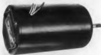
Designed to drive an axial-vane blower, the DE-30-1 induction motor can be used up to 30,000-ft altitude, and in temperatures up to 150 C. Thermal overload protection eliminates smoke hazard. The motor is rated at 1-1/4 hp, 7,500 rpm, with full-load torque of 0.875 lb ft. Full-load current is 4.4 amp; voltage is 200 v, 400 cps, 3 phase. The motor meets military specifications. Weight is 10 lb 2.5 oz.
