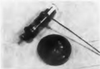
Model VCJ463 is available in fixed capacitance values from 2.0 to 12.0 pf. Operating temperature range is from -55 to 200 C. Capacitance tolerance is 3% at 25 C. Adjustment provides any temperature coefficient between -500 ppm and +500 ppm per C.
