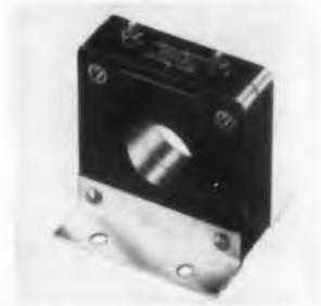
These current transformers are made in a wide number of ranges, at lower cost than previous models. They can be used with wattmeters as well as ammeters. Case is high-impact, abrasive-resistant plastic. They operate at a frequency of 25 to 800 cps. The model 605 is available in 100:5 through 400:5 ratios in 5 types; model 607 is supplied in 6 types with ratios from 500:5 through 1,500:5.
