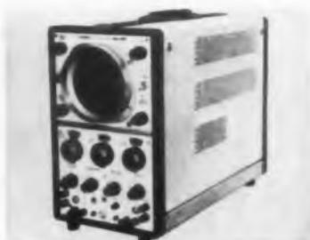
Types 1120 Portable and 1120-R Rack-Mountable permit the simultaneous display of two vertical signals against time, against each other, or versus a third variable fed externally to the X-axis. These main-frame indicators have 64 contacts to mate with plug-in circuits. Both are designed for safe off-ground operation up to 500 v dc.
