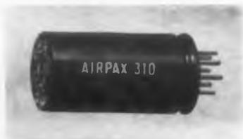
The series 310 chopper is unaffected by extremes of temperature over a  $-65$  to  $125$  C range. Driving voltage is 6.3 v rms, 400 cps. Dwell time is  $147 \pm 18$  deg; phase angle is  $65 \pm 15$  deg. Noise is less than  $200 \mu\text{v}$  average. Contacts are spdt, break before make.
