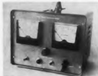
Designed for testing printed circuit boards and cable assemblies, this circuit resistance meter has a range of 0 to 200 milliohms. A safety circuit protects meters from overload damage. The solid-state device is permanently calibrated, and may be operated from 115/230 v, 50/125 cps, or from 30 v dc power supply. It measures 8 x 10 x 8 in. and weighs 11 lb.
