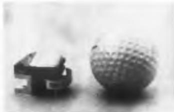
Up to 10 separate switching functions can be remotely controlled with this 1-oz vibrating reed relay. They are available in 30- to 3,000-ohm coil resistances. Driving voltages vary from 1-1/2 to 15 v ac. Reed contacts will pass up to 5 ma. Reed frequencies to within  $\pm 0.05\%$  are available.
