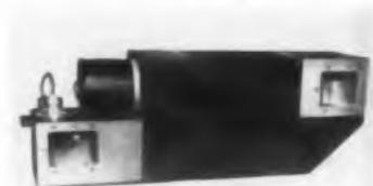
This cooling unit contains an aluminum, plate-fin, counterflow, air-to-air heat exchanger, two axial-flow fans and a temperature control system. Rated cooling capacity is 1.3 kw. Over-all dimensions are 35.9 x 11.9 x 6.5 in.
