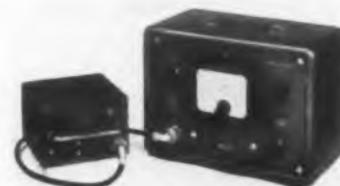
Model 33C is a vibrating capacitor electrometer designed for industrial applications and routine laboratory measurement. Current measurements can be made down to  $10^{-15}$  amp. The separate converter unit, connected with an 8-ft cable, is suited for use with ionization chambers. A built-in 90-v polarizing supply is provided. Voltage is measured in 5 ranges from 10 mv to 1 v; resistance, to  $10^{14}$  ohms. Zero stability is  $\pm 100 \mu\text{v}$  for a 12-hr period.
