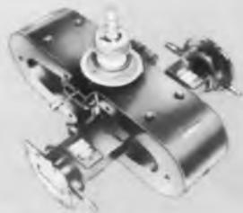
**Two QKS 622 pulsed type Amplitrons\*** in parallel operation produce 6 megawatts of power output over the 2,900 to 3,100 Mc range at efficiencies of 75% to 80% and duty cycles as high as .005. The QKS 783 is a similar Amplitron that covers the 2,700 to 2,900 Mc range. *Circle 203 on Reader Service Card.*
