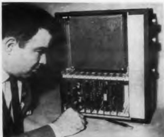
Random-access memory unit developed by Westinghouse Electric Corp. operates at 0.6- $\mu$ sec cycle time with an access time of 0.20  $\mu$ sec.
