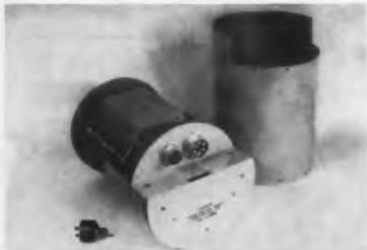
Vibration and acoustic analyzer, developed by Army in cooperation with Gulton Industries, operates at a frequency of 2,000 cps. Power requirement is approximately 75 ma.
