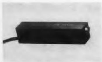
A sealed, all-plastic multi-turn potentiometer, the model 3010 has high-humidity resistance. It can be potted without danger of leakage. Resistances are 10 to 100 K; power rating is 1.0 w at 70 C. Operating temperature is 175 C max and temperature coefficient is 70 ppm max. The 0.1-oz unit measures 1-1/4 x 1/4 x 5/16 in.
