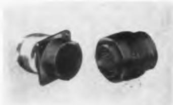
The KPT and KSP styles of miniature MS-type plugs were designed to MIL-C-26482 and SCL-6019. A molded polychloroprene, two-shore insulator holds crimped contacts in positive alignment and maintains a continuous seal from front to back.
