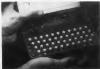
A portable, real-time manual entry code generator, the MG-100 produces perfectly formed Morse characters. Transmission speeds from 6 to 42 words per min may be selected. The 43-character keyboard activates a magnetic-core memory. Rechargeable nickel-cadmium batteries permit 5 hr of continuous operation. Other outputs, such as binary-coded decimal, can be provided.
