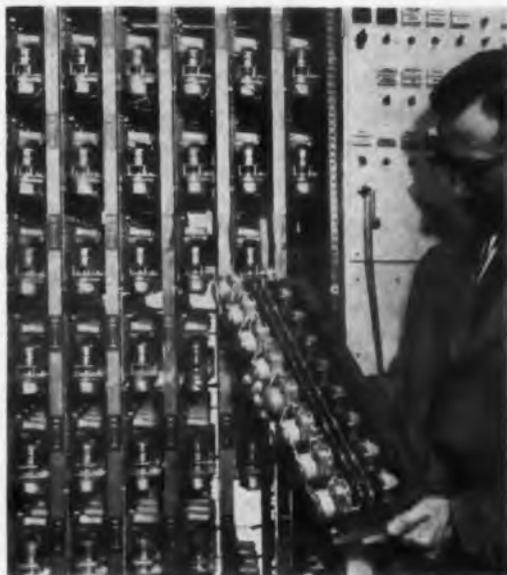
**Mark I perceptron**, now moved to Cornell University, first full-scale learning machine used for pattern recognition, is prototype for smaller versions in many organizations. Mark II now in design at Cornell Aeronautical Laboratory will be special-purpose digital computer programed for threshold logic. Elements shown are transistor-driven relay circuit that operates as association units.
