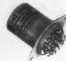
This 6p2t subminiature relay weighs 2.6 oz. It is actuated by a rotary motor which develops high torque-to-size ratio. The motor is self-contained and does not depend on the housing to complete the magnetic circuit. Contact rating of this 1-in. diam relay is 2 amp at 26 v dc or 115 v ac. It is designed and manufactured in accord with MIL-R-5757D.
