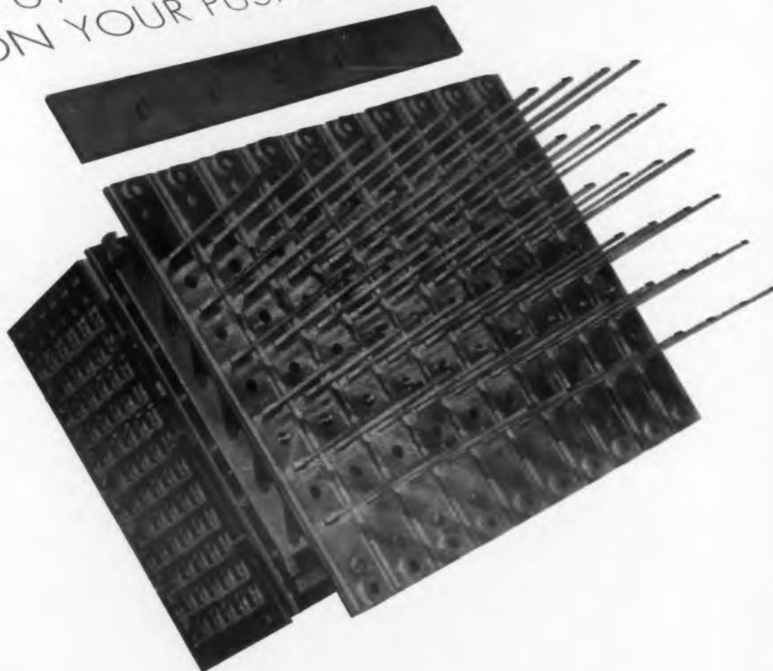
**OAK TYPE 131 PUSHBUTTON SWITCHES** will help you make the most of limited panel space. Only  $\frac{3}{8}$ -in. thick, these switches can be mounted on  $\frac{1}{8}$ -in. centers; a stack of 10 separate gangs of switches requires only  $6\frac{13}{16}$ -in. of panel space. Use Type 131 switches for handling low-power switching in computers, office equipment, communications devices, automatic coin-operated machines and many other military or commercial applications.
