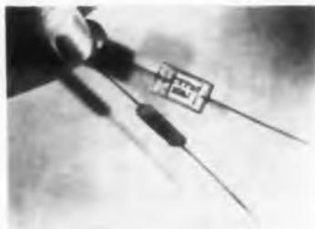
The CYF-20 extends the capacitance range of fusion-sealed glass capacitors to 5,100 pf. The moisture-resistant unit meets or exceeds military performance requirements. Used in high-reliability systems, the capacitors withstand high levels of radiation. Temperature coefficient is  $140 \pm 25$  ppm per deg C over the operating range of  $-55$  to  $125$  C.
