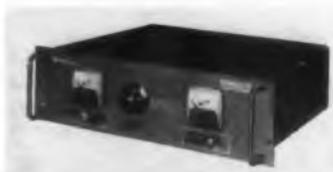
Output of this voltage-regulated dc power supply is continuously variable from 0 to 36 v, at 0 to 10 amp. Load regulation is 0.1% or 3 mv, no load to full load; line regulation is 0.1% for 105 to 125 v ac. Stability is 0.1% or 6 mv over 8 hours. Ripple is less than 1 mv rms. Temperature coefficient is less than 0.05% per deg C.
