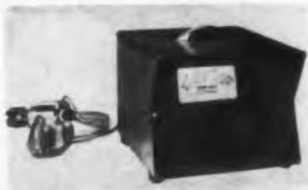
This cold-cathode vacuum gage provides continuous pressure measurement in the  $10^{-1}$  to  $10^{-6}$  mm Hg range of dry air. Tube design provides for disposal of contaminated anode or cathode. Except for seals, the gage tube is made entirely of metal. The anode is of ring design for concentrated ion-beam discharge.
