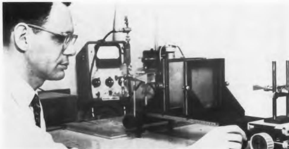
**Interferometer** for measurements at 2 mm. Transmitting horn is at left, receiving horn at right. Dr. Peter E. Tannenwald, assistant leader of the Resonance Physics Group, conducts experiment.
