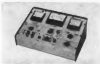
Model T-340 transistor tester is for npn and pnp transistors. It measures the four basic parameters necessary to check a transistor's performance. The  $I_{CO}$  range is 0 to 500  $\mu$ a;  $I_{EO}$  range is 0 to 5 ma;  $I_{CBO}$  range is 0 to 50 ma. Beta ranges cover eight different collector current levels,  $I_C$  set levels are up to 500 ma and  $V_C$  ranges are 0 to 10 v and 0 to 100 v. Results are read directly from a meter.
