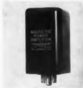
Designed to drive instrument-type two-phase servo motors, these amplifiers control the current to both phases, reducing standby power. Input is dc, polarity-reversible; output is ac, phase-reversible. Input may be as low as 75  $\mu$ a for maximum output.
