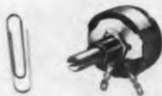
Model R potentiometer can be applied to circuits with frequencies as high as 10 mc with a minimum of distortion. It has a rotational life of 100,000 cycles and is operable from -55 to 125 C. Capacitance is 8 pf. Ratings are 2 and 3 w, 100 ohms to 5 meg.
