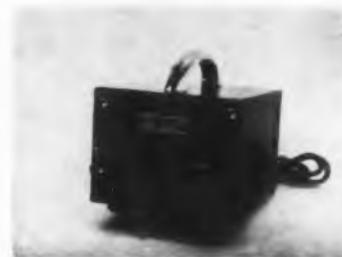
This solid-state power supply, designed for use with thermo-electric cooling units, changes 115 v, 60 or 400 cps, to 1-1/2 v dc. Ripple content is less than 10%. The 4-1/2-lb unit measures 3 x 4 x 5 in. It is available with adjustment and meter.
