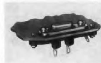
The complete series of spacesaver transistors is accommodated by this socket. Narrow width permits utilization of the space saved by the mating transistor. It is designed to fasten beneath the chassis, and provides direct mounting of the transistor with its mica insulator to the chassis. The transistor is thus provided with maximum heat dissipation by conduction.
