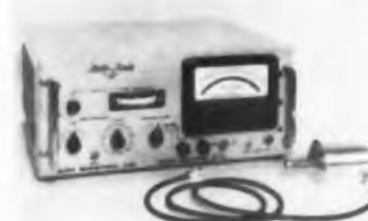
Known as the Auto Node this random noise generator and measuring device has automatic measurement over the range of 5 to 2,000 mc. Accuracy is  $\pm 0.2$  db at 0 to 6 db and  $\pm 1.0$  db at 13 to 15 db with measurement accuracy to  $\pm 0.2$  db over-all. Maximum vswr is 1.1 with a maximum change of 0.002 during operation.
