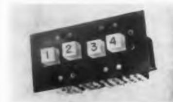
A four-station switch for military aircraft, model WC1730 has an interlock or anti-defeat function whereby one button is always down. Actuating any other button causes the depressed button to return to normal position. The dpdt switch is rated at 5 amp, 125/250 v ac; 5 amp resistive, 30 v dc; and 2.5 amp inductive at 30 v dc. Over-all length is 3-3/4 in. The 9-oz unit has illuminated push-buttons, available in 6 colors. It is designed to meet military requirements.
