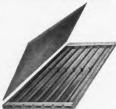
Radar Window of G-E TEXTOLITE 11546 protects exposed feedhorns (A) while permitting transmission of radio frequency energy. Hot air continually blown through window cells prevents ice formation during sub-zero arctic weather.
