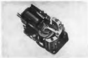
The type 40 rotary stepping switch has 10 points per wiper cycle. It provides up to 30 contacts per cycle and is available with from 1 to 5 bank levels of 10 contacts each. Stepping is by external impulse or self-interruption. Coil voltage is 6 to 110 v dc. The switch will operate up to 65 steps per sec.
