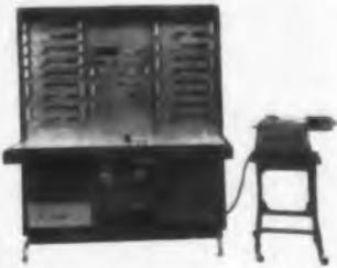
Developed for reliability programs, this semiconductor test system provides repetitive data from lots of transistors or diodes. Fifty or more units may be tested for leakage currents, break-down voltages, saturation voltages, dc gain, reach-through and small signal "h" parameters. Data is recorded on a matrix chart and punched cards. Test accuracy is  $\pm 1\%$ ; repeatability is 0.2%. Power capability is 0 to 1 kv, 0 to 3 amp. The system is self-testing.
