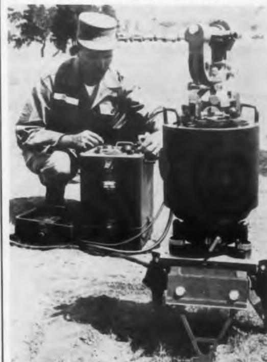
Pinpoint artillery firing accuracy and improved battlefield mobility are possible with ABLE (Autonetics Base Line Equipment), the Army's new portable, gyroscope direction finder. Basically a precision gyrocompass, ABLE determines true north to less than 30 sec of arc in less than 20 min operating time. Under old surveying methods, artillery base lines sometimes took hours or days to establish. ABLE is in production at Autonetics Div., North American Aviation, Inc.
