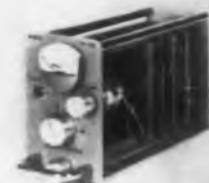
The FR-500 series modular frequency-to-dc converter provides three simultaneous outputs: 0 to 5 v dc; amplified pulse; direct reading indicator on front panel. Input frequency range is from 5 to 3,200 cps in 6 overlapping steps. Output is not affected by an input variation of from 5 mv to 100 v rms.
