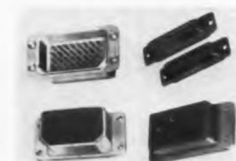
Rack/panel plugs are now offered with crimp snap-in contacts. Affected types are DPX, DPA, DPD, and D subminiature plugs, together with the environmental types such as DAD and DED. The gold-plated, copper contacts are rated at 5 amp. Coaxial inserts are also available. Monobloc insulation is diallyl phthalate. Accessories such as floating mounts and a variety of junction shells are available.
