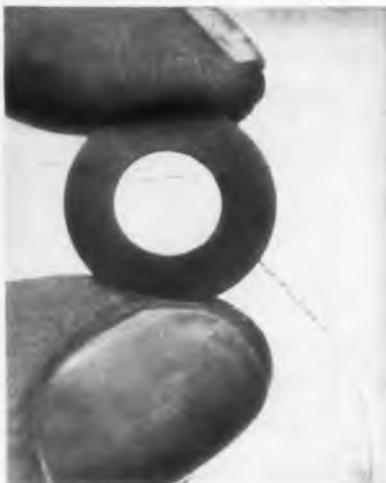
In the Remington Rand Univac physics laboratory, 5 mil. diameter holes are ultrasonically drilled in ferrite cores, then threaded with fine wire in the examination of domain structure. Such experiments prove that a series of alternate-polarity pulses of diminishing amplitude result in concentric rings of alternately directed magnetization. Much smaller cores (80 mil. o.d.) were then studied by means of residual magnetization curves for flux distribution under various modes of partial switching.
