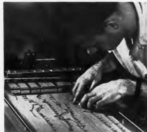
**Control unit** for speech synthesizer at Stromberg-Carlson controls five functions useful in speech synthesis: three formants, intensity, and pitch. Carriage moves along pattern of tracks to control equipment that switches oscillators on and off.
