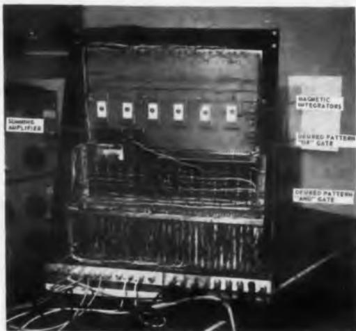
**Learning machine** of perceptron-type built at Aero-nutronic solved problems in Boolean logic equivalent to pattern recognition problems. Machine was test vehicle for biax-type magnetic integrators wanted by Navy for perceptron program at Cornell Aeronautical Laboratory. Larger version of learner under construction at Aero-nutronic will also use magnetic integrators. If performance is satisfactory, still larger version, capable of useful work, will probably be built.
