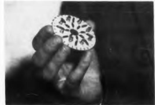
**Tunnel-diode module** for developmental computer memory handles 64 bits in 3-in. diam. Complete read-write cycle was performed in 40  $\mu$ sec with same circuit in different configuration—an 8 x 8 array on 9-in. circuit board. Module is for a word-organized memory designed at Plessey Co., Ltd., Hants, England, that uses voltage-mode selection. Circular arrangement was chosen to reduce delays caused by leads, which slowed read time in array format to 10  $\mu$ sec.
