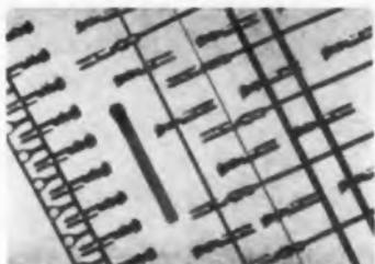
A crimp-type contact, the Varilok will accept all wire sizes from 18 gage to 30 gage. It is said to offer easier and faster production, and positive locking of contacts when inserted into connector castings. Contacts are available loose, for hand crimping, and in reel form for power crimping. Hand and power tools, an insertion tool, and a checking gage are available.
