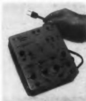
This tape transport programmer automatically controls digital tape machines to run in forward and reverse. Run times and stop times are adjustable from 2.5 msec to 1 sec. Outputs are capable of driving the actuator control circuits of the tape machine. The unit is contained in a case measuring 4 x 7 x 8 in.
