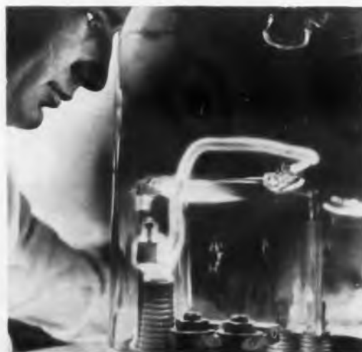
Electron bombardment of a Photopot's crystal surface is performed in tests at Giannini's laboratories. Modifications of the properties of the photoelectric potentiometer under bombardment are studied.
