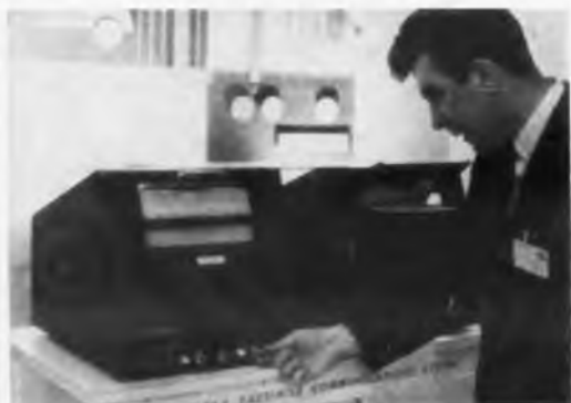
Line drawings or diagrams can be sent over private telephone lines (schedule 2) using this Dictaphone Data-fax system. Light from fluorescent lamps is reflected from the drawing through a 0.01-in. sq. aperture, which is mechanically scanned. The light strikes a photomultiplier tube, and the tube's output modulates a carrier. A helix printer at the receiving end marks electrostatic paper in synchronism with the scanning aperture. A seven-tone gray scale is provided. George Theofanis, service representative, adjusts receiver-printer.
