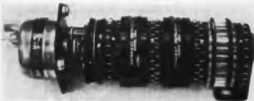
Rings of reed contacts surround solenoid-driven permanent magnet in high-speed rotary switch. The cover has been removed from the deck at the right to expose the glass-enclosed reed contacts.
