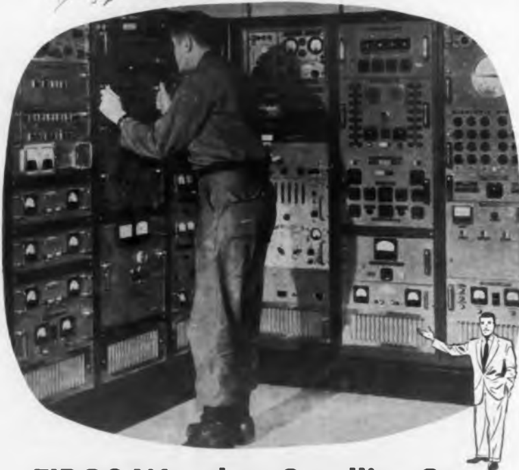
Fort Monmouth Laboratory Control Panel used for the tracking of NASA's TIROS Weather Satellite. Note McLean rack-mounted cooling equipment at the base of each rack. Operator at left checks the TV picture being transmitted. Recording camera is located directly above eyepiece.
