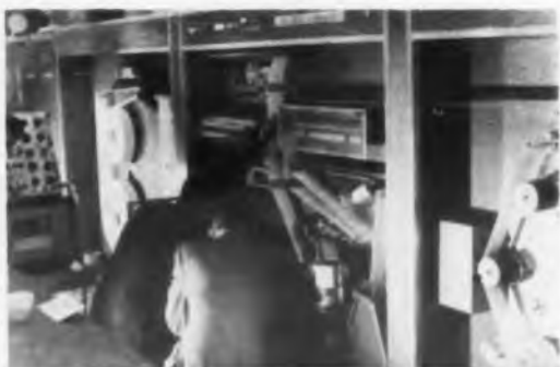
Last-minute adjustments are made on A. B. Dick Co.'s Videograph electrostatic address-label printer, which uses digital-pulse code input.
