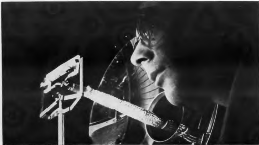
Photo-induced Hall effect in an organic semiconductor is studied with flash tube apparatus at Armour Research Foundation. So far, 10 \mu sec-single pulses focused on anthracene crystals to generate carriers have not resulted in measurable effects. Researchers are trying to detect these by noting the effects of magnetic fields on Hall currents. Armour's W. D. Brennan, shown here, reports apparatus is being modified.
