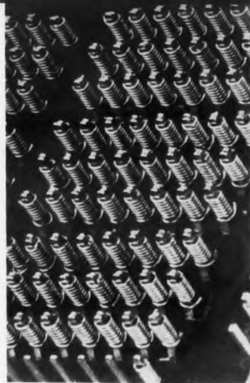
Fig. 5. A series of wire-wrap terminals illustrating the technique.
