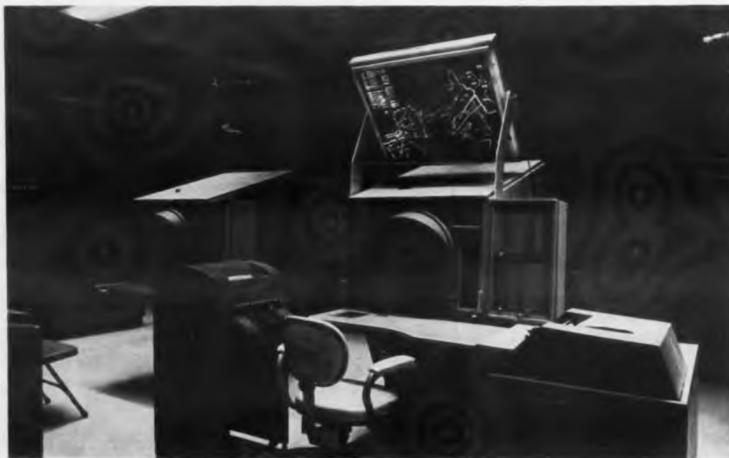
Control team station and equipment for Satin experiment, in which high-altitude air traffic over the New York-Boston area will be controlled by integrating facilities of the present FAA air-traffic network and the SAGE air-defense system.
