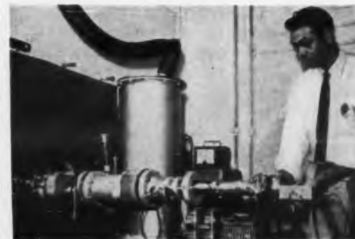
Two megavolts accelerate micron-size particles in test and calibration unit for micrometeorite detectors, set up by Dr. Joseph F. Friichtenicht, above, of Space Technology Laboratories. A Van der Graaf generator, used in the acceleration process, is behind the dark lead shielding at left.
