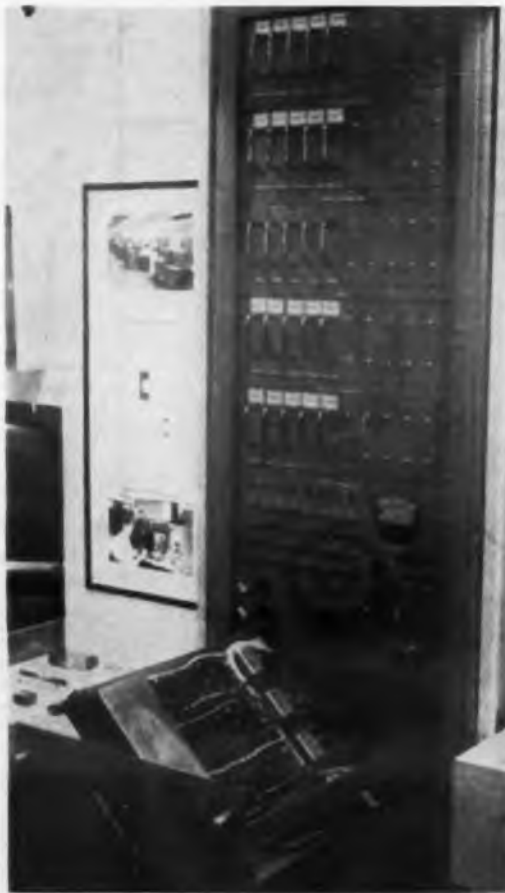
Single-sideband diversity receiver operates at 2 to 30 mc over any of 10 pretuned channels. Unit is being delivered to the Air Force for Operation Quick Fix—a modernization of global communication system. Hughes Aircraft system is designed to operate in quadruple diversity mode.
