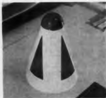
Log-periodic antenna formed on nose cone has a frequency range of from 2,200 to 9,800 mc. Maximum directive gain is about 6 db each way—E plane 50 deg, H plane 80 deg. The antenna, designed by Martin Co., may be single or dual phase with linear or circular polarization.
