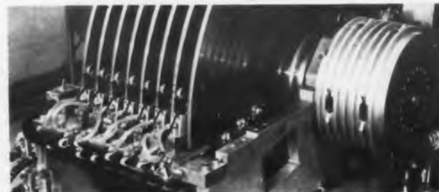
Bryant 4000 file can have from one to 20 disks. Positioning arms, shown with three heads, can have as many as six.
