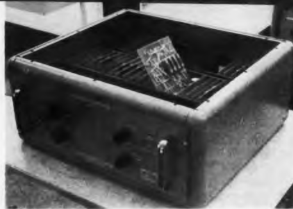
Digital data transceiver designed for modem applications is capable of serial transmission of binary data at rates up to 4,800 bits per sec over high-quality lines, and rates up to 2,400 bits per sec over regular switched telephone voice facilities. The Hughes Aircraft Co. modem codes into four orthogonal phases. It weighs 75 lb and measures 7 by 19 by 18 in.
