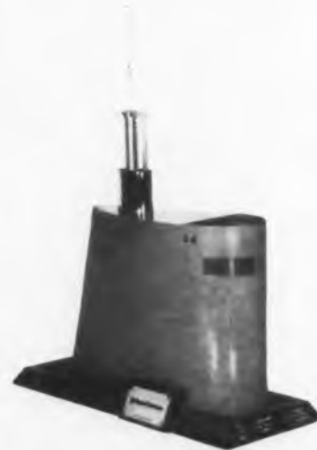
Wide-frequency-range antenna for submarine use employs helix for tuning from 2 to 32 mc. Designed by Hoffman Electronics Corp., the antenna is capable of handling up to 5 kw. Whip is shown partially retracted; entire assembly can be retracted into conning tower in 40 sec.
