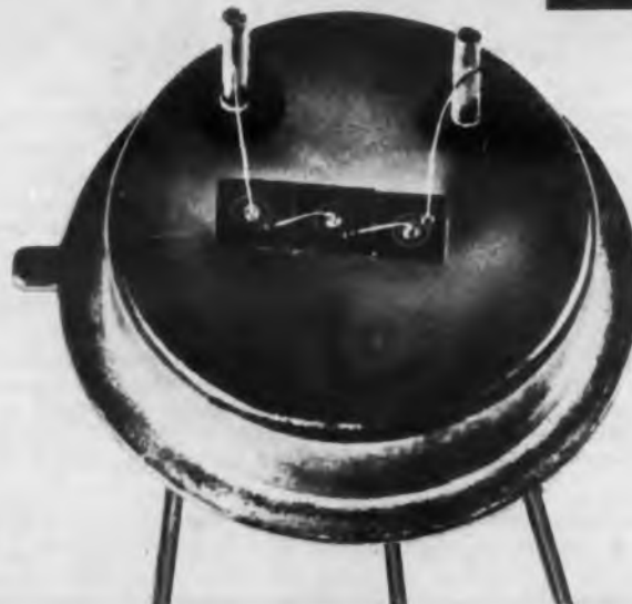
FSP-60 Triple Darlington High Gain Low Noise Amplifier TO-5 size header 3 - 2N1613 Planar Transistors h_{FE} typical = 100,000
