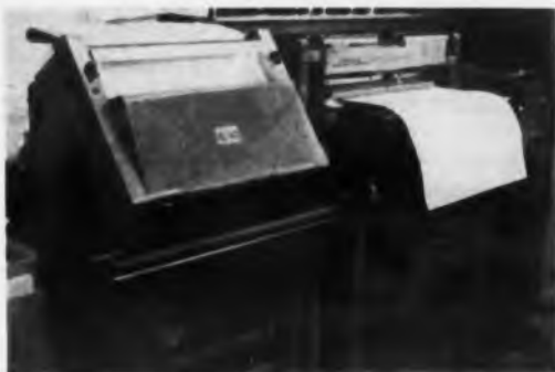
High-speed facsimile scanning and recording system operates at 190 sq in. of copy per min, with 96-line resolution. Aldea system uses 24-kc channel.
