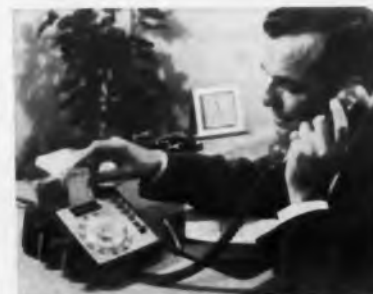
It was perfecting the card dialer which permits, through insertion of a punched card into a slot, automatic dialing of frequently used numbers.
