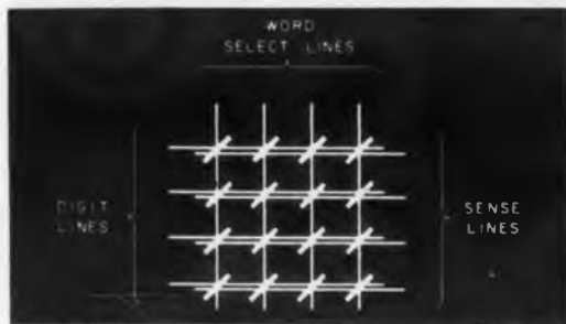
Fig. 1. A word-organized selection system with four words of four bits each.
