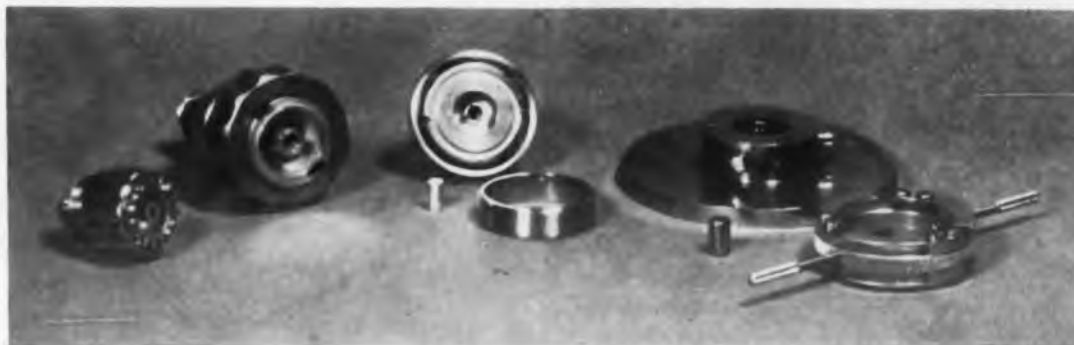
Standard, high-precision connector may well be selected from the ones in this photo. From left to right: General Radio 900, Rohde & Schwarz Dezifix, Marconi H-1 and NBS-modified Woods connector.
