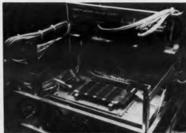
Computer memory (top) consists of glass plates carrying small, rectangular magnetic-film elements and sandwiched between flexible printed-circuit sheets. Film thickness is 1,200 Å, giving strong signal from small spots. Complete 256 13-bit word memory, mounted on stiffening boards, is shown in lower photo. Provision is made for eventual four-fold increase in memory capacity.
