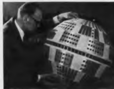
It was preparing an experiment in world-wide communications using "active" satellites powered by the solar battery, a Bell Laboratories invention.
