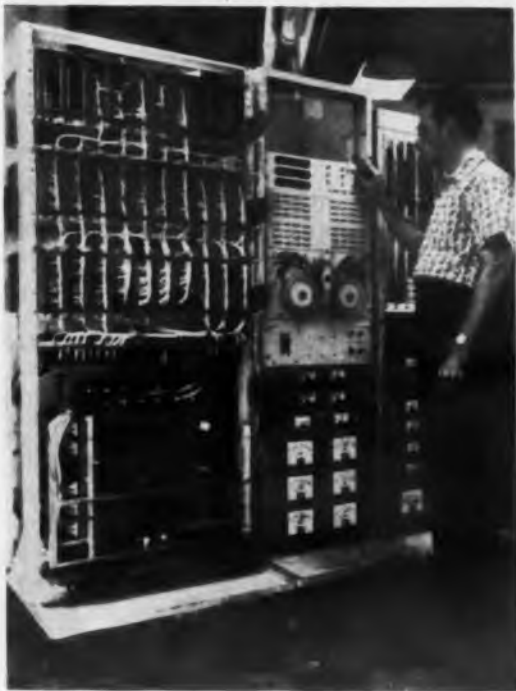
FX-1 computer , said to be 10 times faster than any general-purpose digital computer now in use is adjusted by John Laynor, staff member of Lincoln Laboratory's digital computer group. The computer was built to test feasibility of high-speed operation with conventional components and fabrication techniques.
