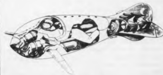
Shielded version of chariot operates at 12 knots underwater. Upper cylinder in nose houses navigation aids. Operator's compartment is flooded.
