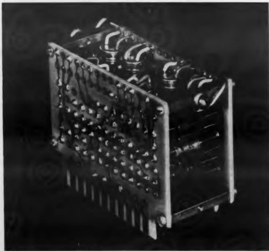
Plug-in unit for FX-1. Computer uses 325 such units of 12 standardized basic types. Approximately 3,000 special high-speed transistors are included in the computer. These are Philco L-5447 germanium MADT's similar to the company's 2N769 transistor.
