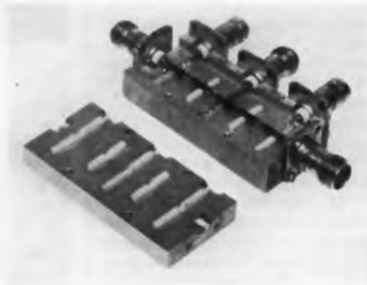
Fig. 3. Single-pole, double-throw diode switch. Device can also be used as a power divider. Each leg contains two diodes and construction shown is typical of the switches described here. The switch permits pulse repetition rates of up to 30 kc in moderate-power circuits.
