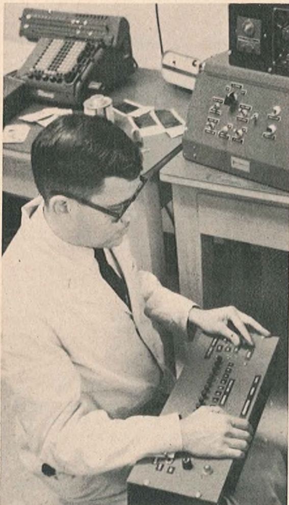
The author, Gordon Silverman, checks the performance of his relay electronic dash-processing system. The relay memory stages use fewer components than their semiconductor equivalents and do not introduce signal distortion.
