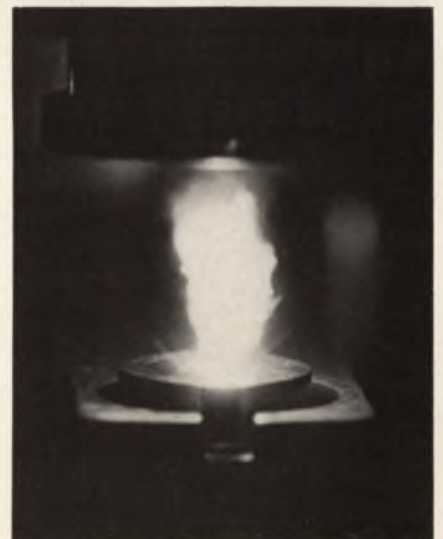
Ruby laser cutting a diamond die for wire-drawing operation at Western Electric Co. substitutes a two-minute job for a two-day task.
