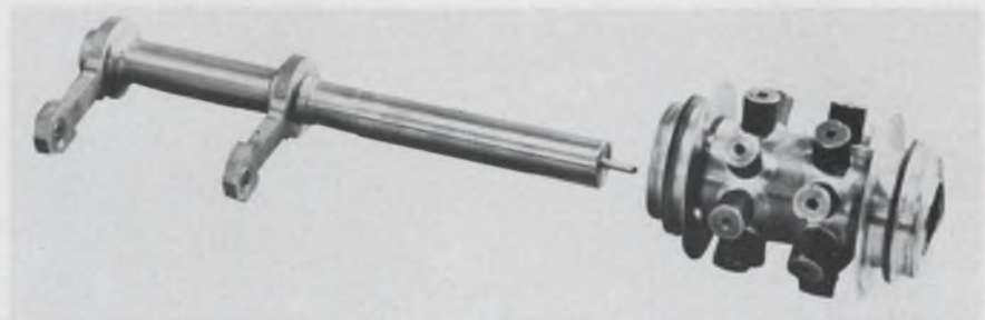
1. Heat pipe (left) and thermionic converter (right) team up to convert thermal energy directly to electricity.
