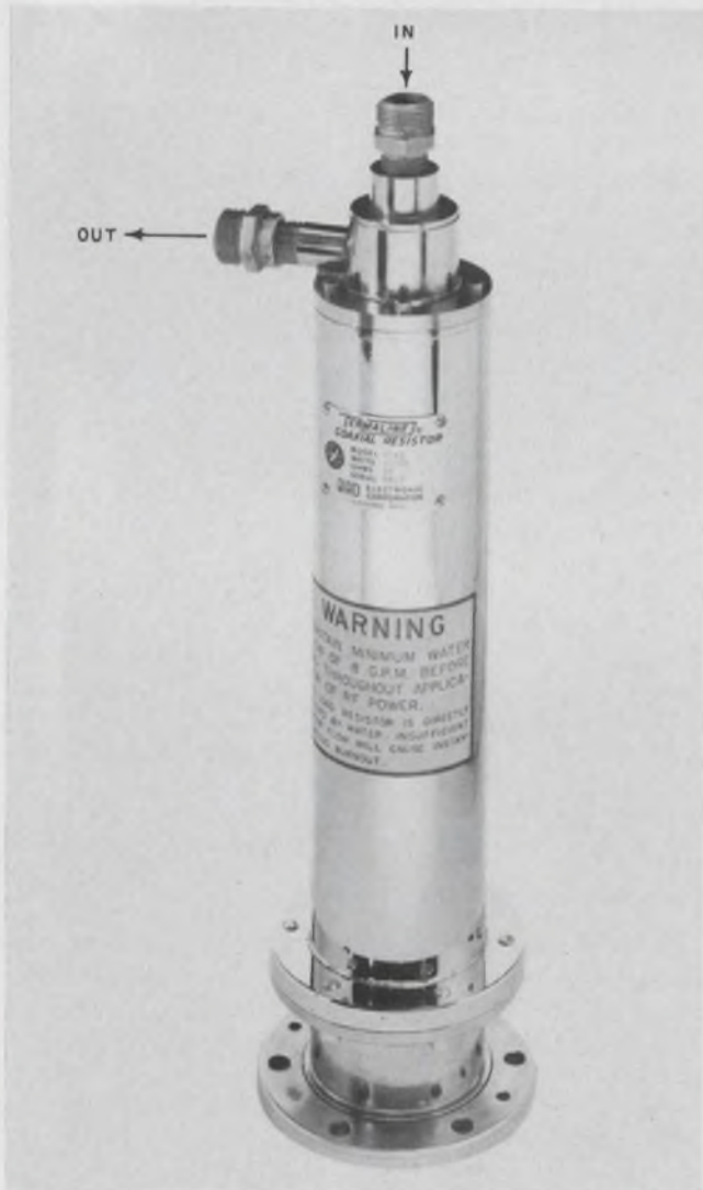
4. The power resistor inside this dummy load (a film deposited on ceramic substrate) is cooled directly with water at a rate of about 8 gallons per minute. This termination (Bird TERMALINE® Model 8762) is rated 50 kW.
