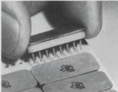
Figure 4. New plug-in flat packages for TI integrated circuits are easily handled and inserted into industrial-type PC boards.
