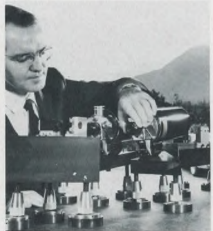
Optical telescope, being adjusted by Dr. George Clark of Electro-Optical Systems, is used in experiments to measure the effect of atmospheric attenuation on laser beams. A pulsed neodymium laser output is beamed at mountain in background and signal attenuation is measured.
