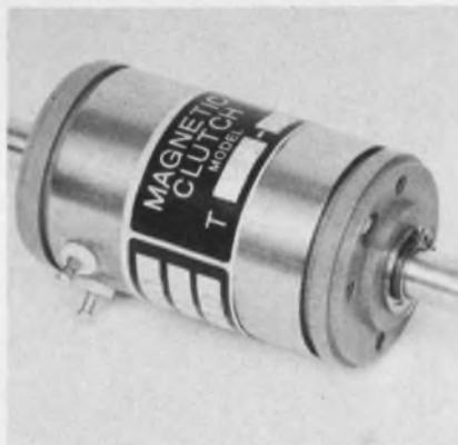
A magnetic particle clutch, Series T-570, features extremely low output inertia and high power gain for compatibility with modern servo systems. Torque-to-inertia ratio is  $7.61 \times 10^6$  rad/sec<sup>2</sup>.
