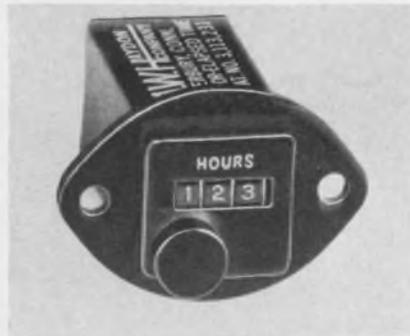
Instantaneous zero reset is a feature of the micro-miniature elapsed time indicators, Models LM19202 and LM19203. Readout is 99.9 and 999 hours respectively. Units are hermetically sealed and meet applicable requirements of MIL-M-7793C. Timing tolerance is  $\pm$  one digit at 400 Hz. Operating voltage is 115 VAC at 400Hz.
