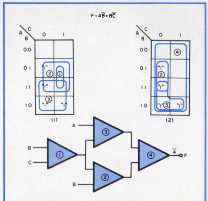
Fig. 7. Each NAND block corresponds to one of the loops generated on the map by the inhibiting process.
