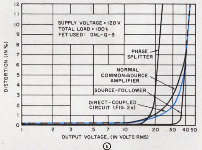
source-follower is especially useful whenever an extremely high input impedance or a low output impedance is desired. It should not, however, be applied in all cases. To cite a few, it should never work into a load smaller than 100 k $\Omega$ , or be used with a generator resistance higher than the input resistance before feedback (10 M $\Omega$  in Fig. 1a).
