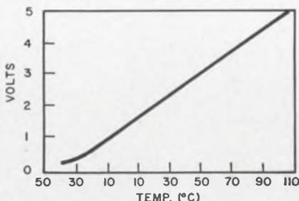
The transducer's output is sufficient for telemetry purposes to the extent that no preamplification is required.
