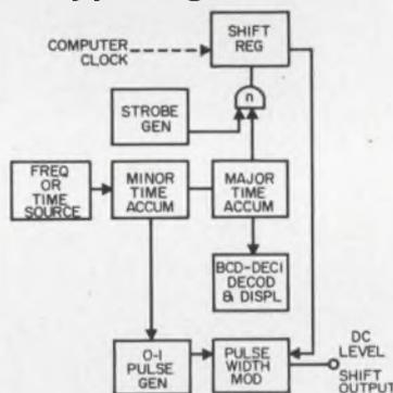
Here's a digital clock-time code generator using integrated circuit logic. It can provide BCD outputs of time and date in either parallel or serial form, or in any combination.
