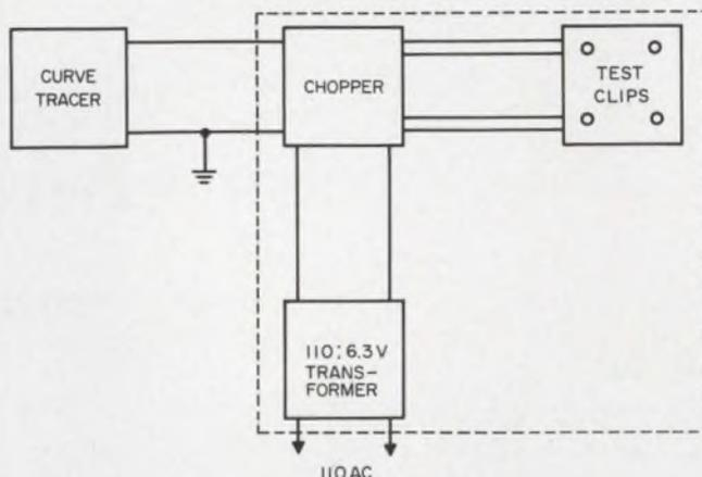
Diodes are quickly and simply matched when this test jig is used in conjunction with a curve-tracer. The chopper is employed for viewing the low-voltage portions of the  $E/I$  curves. For higher level portions, a reed relay should be substituted for the chopper.
