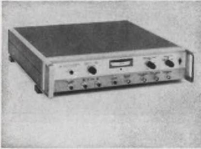
Model 8708A signal-generator synchronizer uses phase-lock techniques to give test signals stable within 2 parts in  $10^7$  over 10 minutes. Automatic synchronization is achieved within the range of the 606B (50 kHz to 65 MHz) or 608F (10 MHz to 455 MHz sig gens.
