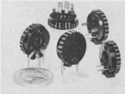
Trimmer needs in printed-circuit test, measurement and communications equipment are met by a new miniature closed-construction potentiometer. It features a rotational life in excess of 25,000 cycles and is 0.696" in diameter and 0.250" deep (including knob). Designated the Model 9, its range is 100Ω to 10 MΩ (1/5 W) in the linear version and 200Ω to 1 MΩ (1/10 W) with a non-linear taper. 20% tolerance is standard; 10% optional.
