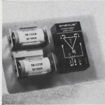
Designed for services requiring low power consumption, Model 2LV-1 operational amplifier features a 4 mW standby power drain at  $\pm 2.5$  V. The all-silicon unit can be operated from batteries, and offers a dc open loop gain of 10,000 with an output capability of  $\pm 1.5$  V at  $\pm 1.5$  mA. The 2.02 x 1.14 x 0.62-in. device operates from  $-25^\circ$  to  $+85^\circ$  C.
