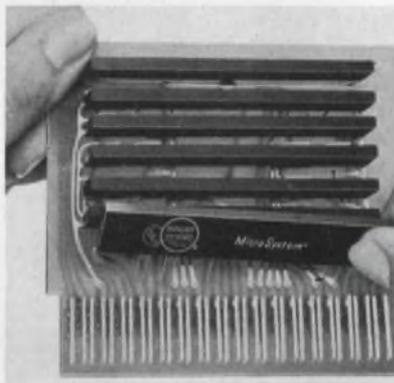
A wide range of standard and special purpose logic cards using integrated circuits includes a free running Multivibrator.
