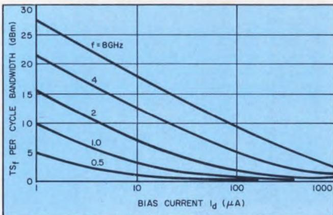
10. The frequency-dependent sensitivity factor,  $TS$  increases with increasing bias current. It also depends on the cut-off frequency,  $f$ .
