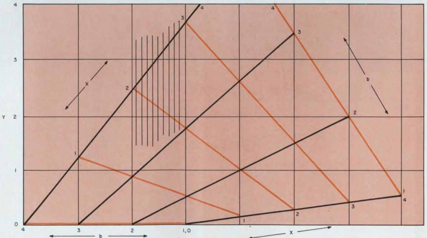
6. Joining of  $X = 0, X = 2, X = 3,$  and  $X = 4$  points on overlay. Interpolation is the next step.
