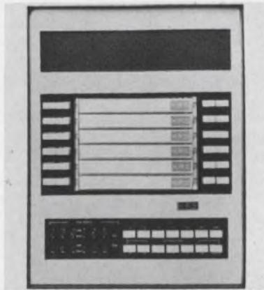
Twelve data channels are provided by the KRS Data-Stack DR-2 recorder. Different versions offer front panel/remote control, or remote control alone, of: random access, cartridge serial/parallel control, cartridge group sequencing, and cue tones. This basic system building block records dc to 100 kHz.
