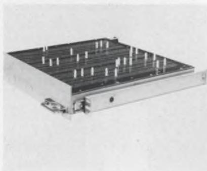
Chassis-mounted multi-switch and program boards with mechanical pull-out and lock-in features are equipped with lever handles that are designed for positive latching of the drawer in the rack. It can make or break multiple pin connectors mounted at the rear of the chassis. Pin friction of up to 400 pounds is easily overcome.
