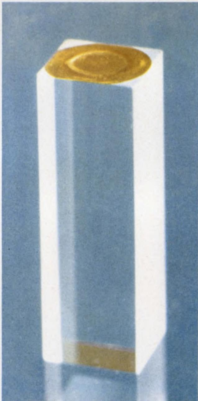
**Multiple thin films** deposited on single-crystal sapphire rod function as efficient acoustic transducers at microwave frequencies. (paper 37.1)
