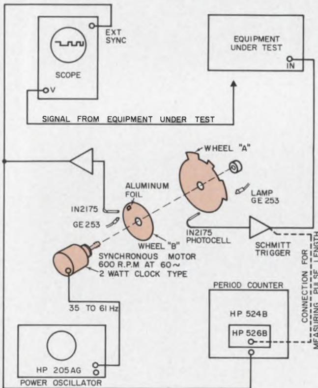
Teletype signals are generated by this variable-speed photochopping system. Wheels A and B produce the various facsimile and timing pulses. The system is also capable of viewing teletype signals.
