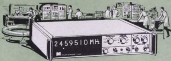
Reliability, accuracy and compactness because Monsanto designs this counter-timer with 90% integrated circuits. Seven of its sixteen printed circuit boards are interchangeable for easy maintenance. **\$1,975.00**
