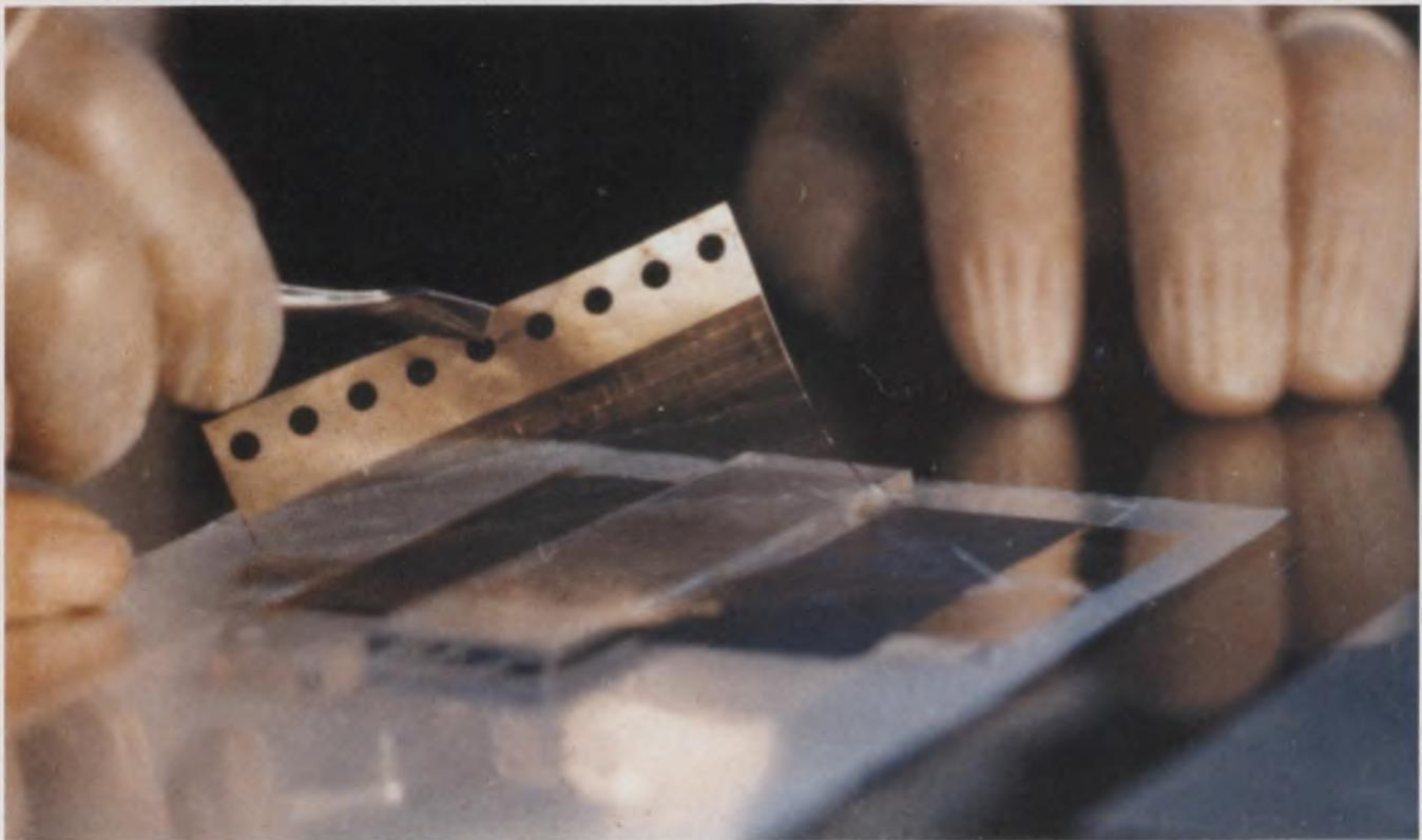
**Thin-film polycrystalline solar cells** are now under development at RCA Laboratories. (paper 77.2)
