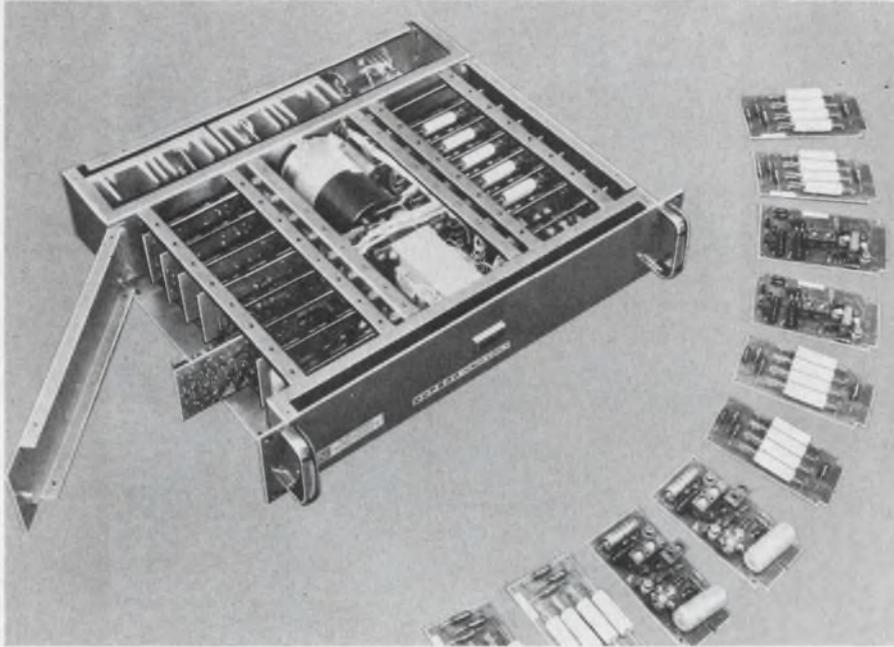
Current and voltage are fully programable with easily interchangeable modular circuits.
