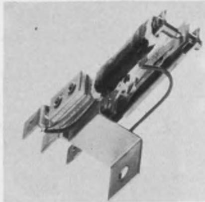
A thermal switch, Series 4300 is being offered. The Series 4300 switch is a snap-acting, heavy duty bimetal actuated unit. Contacts are single pole single throw, available either normally open or normally closed. These switch-units are capable of switching up to a 30 A resistive load, or a 1500 watt Tungsten load.
