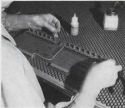
bypassed this problem with EASTMAN 910 Adhesive. A drop of EASTMAN 910 Adhesive is applied to the transistor collar cap to bond it in its slot. Although the bond is strong enough to withstand 1000 G's, the porosity of the surface permits easy rupture and ready transistor replacement.
