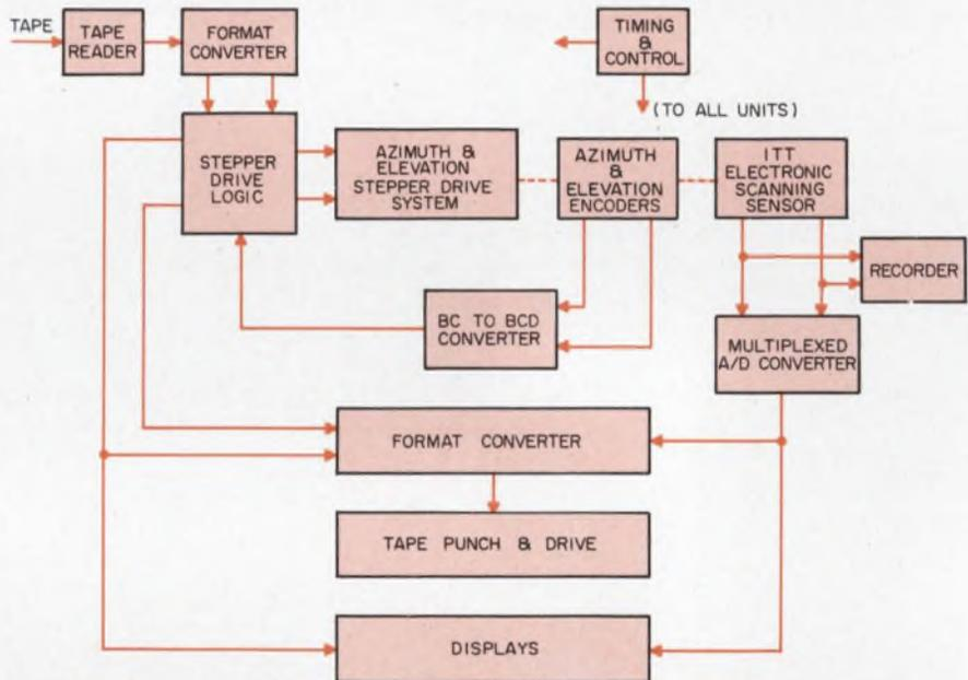
ACME (Antenna Contour Measuring Equipment) system, under development at ITT Federal Laboratories, will be installed at NASA's 85-foot tracking antenna at Rosman, N. C.
