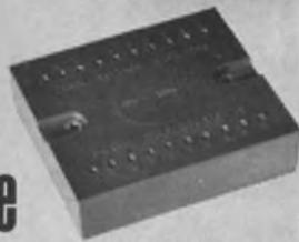
Regulate up to 20,000 volts. Simply connect in parallel with molded packaged power supply (above) or any high voltage unit and obtain automatically both line and load voltage regulation as well as ripple reduction. Nominal current rating is 0.5 to 1 ma. for better than 1% stabilization. Regulation over range of 0 to 5 ma. is 3%. Can be wired in series for high voltage service. Built-in taps provide for selection of twenty regulated voltages. Ideal for photo-multiplier tubes.
