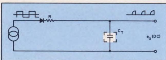
13. Integrator network is formed by resistor R and the transducer in this circuit.
