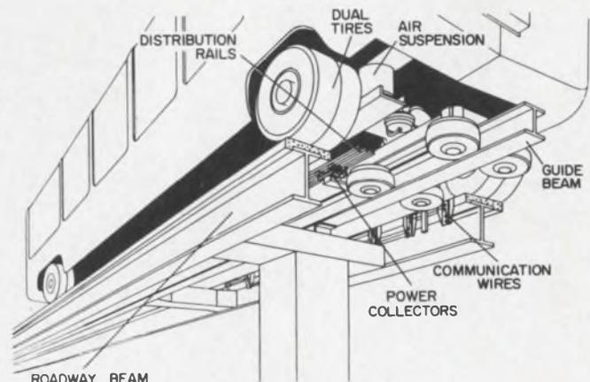
1. The Westinghouse Sky Bus rolls quietly through South Park controlled completely by computers. Its dual rubber tires run on two concrete tracks that are supported by steel "I" beams. Two dc motors propel each car.
