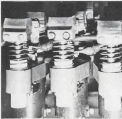
3. Articulated pantograph, or brushes, tap rails for three-phase power. Brushes contact rails from bottom.
