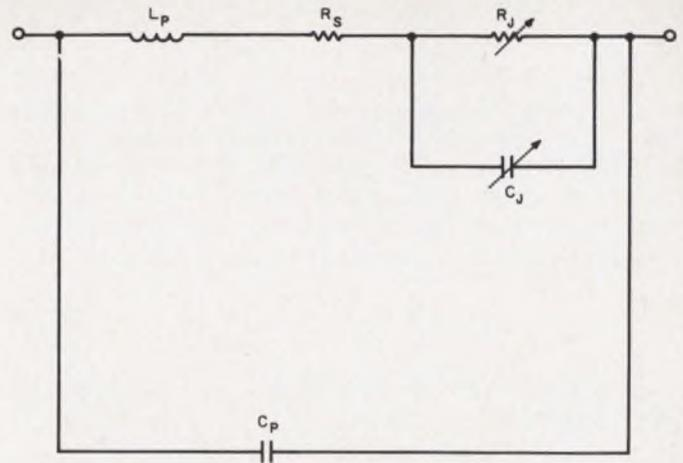
1. Equivalent circuit of hot-carrier diode shows important parameters. Typical values are: 11 ohms series resistance, 0.15 pF package capacitance, and 3 nH package inductance.
