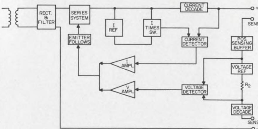
Current and voltage limiting are accomplished through independent regulator channels which provide automatic crossover to either mode for limiting or control. Remote sensing and load are related by these systems.
