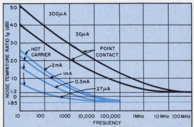
3. The intrinsic noise temperature,  $t_d$ , of hot carrier diodes is less than that of point-contact types. The asymptotic value of  $t_w$  is shot and thermal noises.
