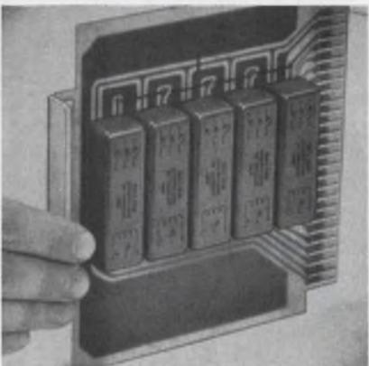
Signals from microvolts to 200 V are switched in under 750  $\mu$ s by a low-to-medium level signal switching sub-system module, the Microscanner. Available in six models (three dpst and three 3pst, two or three circuits/channel), the units accept drives of 6, 12 or 20 Vdc. Uses include data multiplexing and analog data switching.
