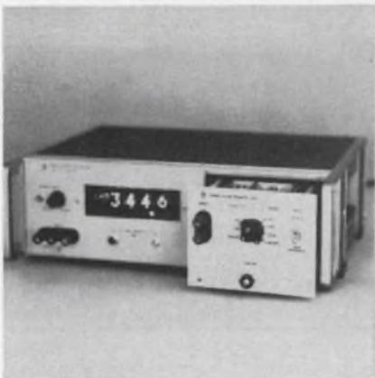
Designed for use with HP's Model 3440A digital voltmeter, model 3446A ac/dc remote plug-in unit makes it possible to remote-control the instrument's voltage range and/or function. The remote unit adds usefulness to the DVM in programed automatic data acquisition or manual test service. DVM remains accurate.
