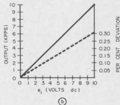
1. **Conventional analog-to-frequency converter (a)** operates with an output of 0-10 Kpps and has linearity of 0.5%. Integrator's reset time ( $T_R$ ) limits linearity of the response, especially at high pulse rates. Curve shows the relationship between input voltage, output pulse rate and deviation from linear response (b). Note error due to  $T_R$ .
