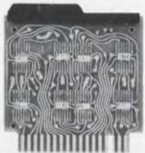
SR-335 SHIFT REGISTER PAC contains 8 prewired integrated circuit shift register stages. Up to 16 custom assembled stages can be supplied to meet customer design requirements.
