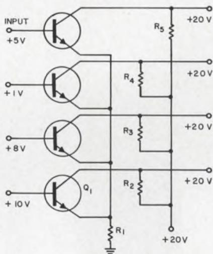
circuit. With the maximum input voltage on the base of  $Q_1$ , the base-emitter junction of  $Q_1$  will be the only one forward biased. Voltages on the emitters of all transistors, except  $Q_1$ , will be more positive than the voltages on their respective bases and they will be cut off. The output voltages of these transistors will be very high compared to that of  $Q_1$ .
