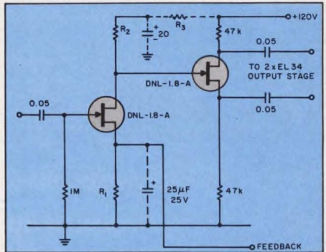
4. Hi-fi power amplifiers may be driven by this direct-coupled FET phase-splitter. High gain and low distortion are provided by the phase-splitter and source-follower FET combination. The dashed components are used for filtering.
