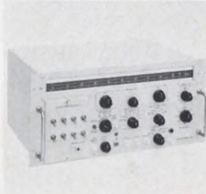
An FM receiver is used in this analyzer designed for use in testing FM circuits. The receiver covers 50-90 MHz, and converters allow RF measurements over 3.7-11.7 GHz. Resolution is 0.5 ns. The model 336 receiver has a companion FM transmitter, model 335.
