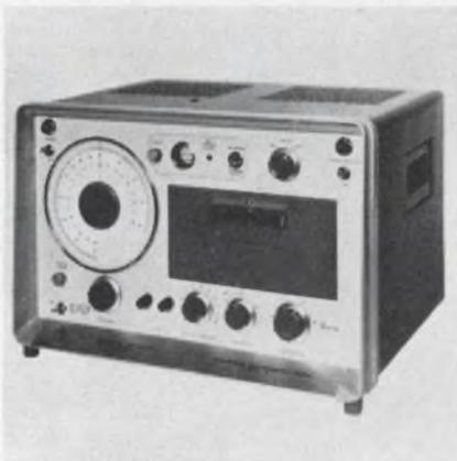
Model SG-88 function generator creates any single-valued waveform. A rotating transparent disc with an opaque representation of the desired waveform is scanned by a narrow light beam. Lenses, mirrors, and a phototransistor convert the light to a signal producing a waveform (0.005-50 Hz at levels from +25 to -25 Vdc).
