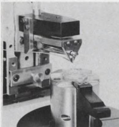
Using ultrasonics, this new model WU-100 wire bonder welds a wide range of power transistors such as TO-3's, TO-66's, stud packs and other large devices. It bonds wire from 5 to 40 mils.
