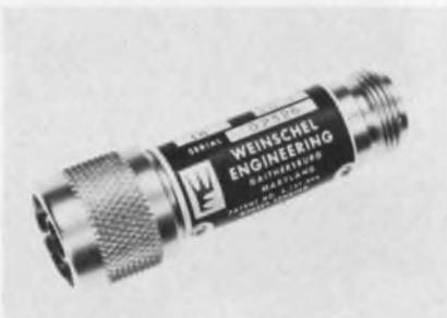
The models 1 and 2 coax attenuators broaden the range of applications for coaxial systems—including use of the 12.4 to 18.0 GHz, band usually reserved for waveguide. Both models applicable where isolation between RF components is needed. The attenuators can also be used in the calibration of directional couplers, antenna characteristics, and in the simulation of path losses.
