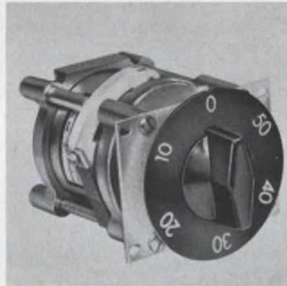
Each module of the ATV-Series turret attenuators occupies  $<$  a 3-in. cube space. Designed for the dc to 1.2GHz frequency range, the units provide from 0-50 dB attenuation. Accuracy is  $\pm 0.5$  dB. Maximum feed thru is 0.1 dB at 1.2 GHz. All contacts are coin silver. Carbon disc resistors are used.
