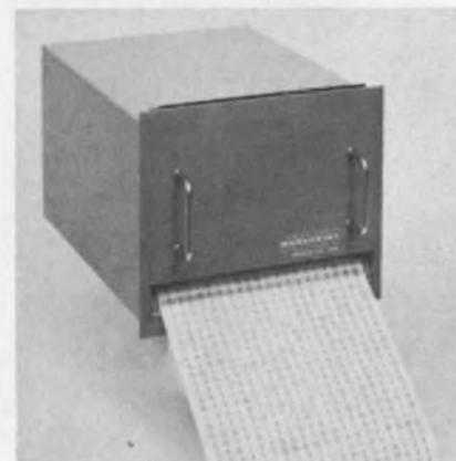
Tape printed data in binary form is presented by the Modu-printer series. According to size, they have capacities for 9, 14, or 20 bits. Each bit needs 6 ms minimum to reach 1 or 0. The installed modules may be moved to either position without decoding from binary sources. Maximum line printing rate is six per second.
