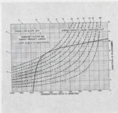
Alnico 9, a new permanent magnet material, has an energy product of typically 10.0 M.G.O. and a coercive force of 1580 H Oersteds, as shown on graph. Its straight line magnetic axis and high coercive force permits use in short sections such as flat squares, rectangles, discs and rings as well as cylinders, solid or cored, and blocks.
