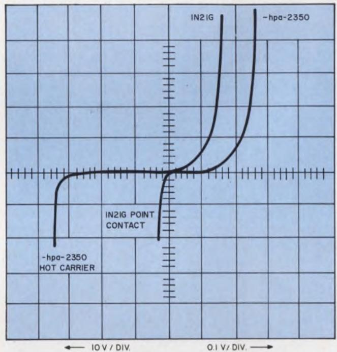
2. Voltage vs current profiles of a hot-carrier diode and a point-contact diode show the higher reverse breakdown voltage of the hot-carrier type.
