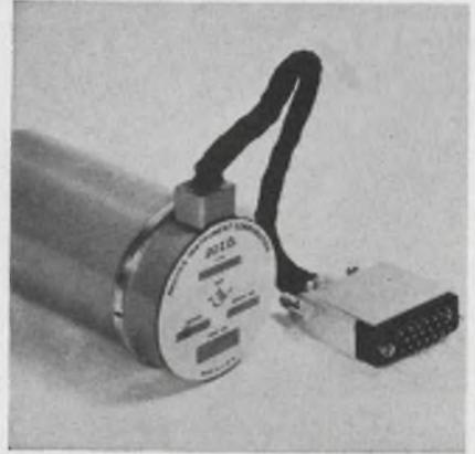
Containing a D'Arsonval torquer, the 20IG type C40D permanent magnet torquer rate integrating gyro is said to eliminate magnetic restraints, hysteresis, saturation non-linearities and power drain from a reference field. The 0.1% torquer linearity holds for 300,000 degree/hours torquer rate and the company guarantees 5000 hours as the dynamic wearout wheel bearing life.
