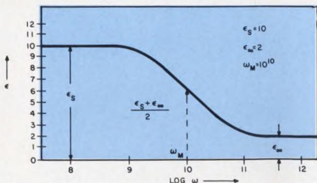
1. Dielectric constant decreases with increasing electric-field frequencies of about  $10^{10}$  Hz and higher. This is shown for a low-density material.
