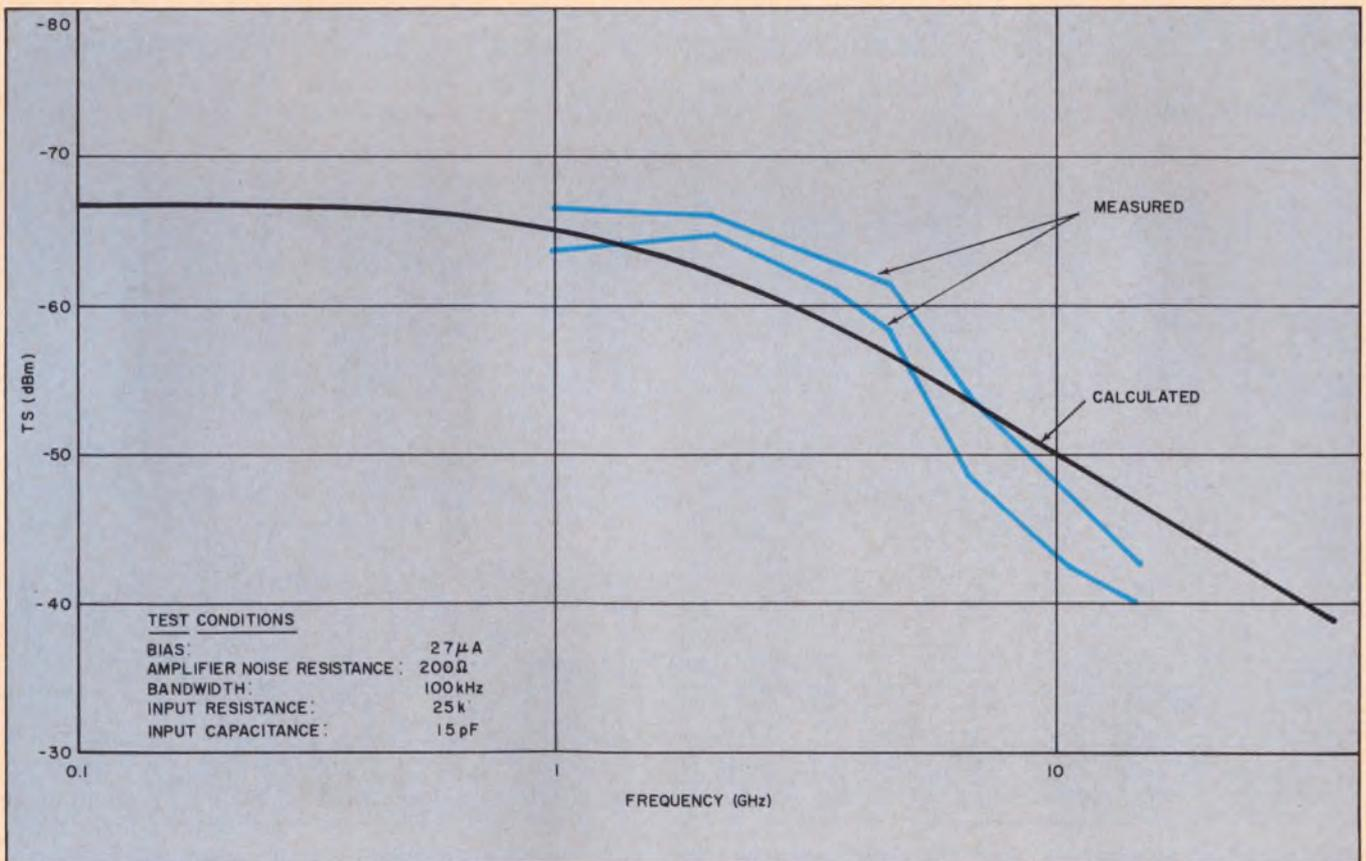
12. A comparison of measured and calculated sensitivity values for hot-carrier diodes indicates a close correlation.
