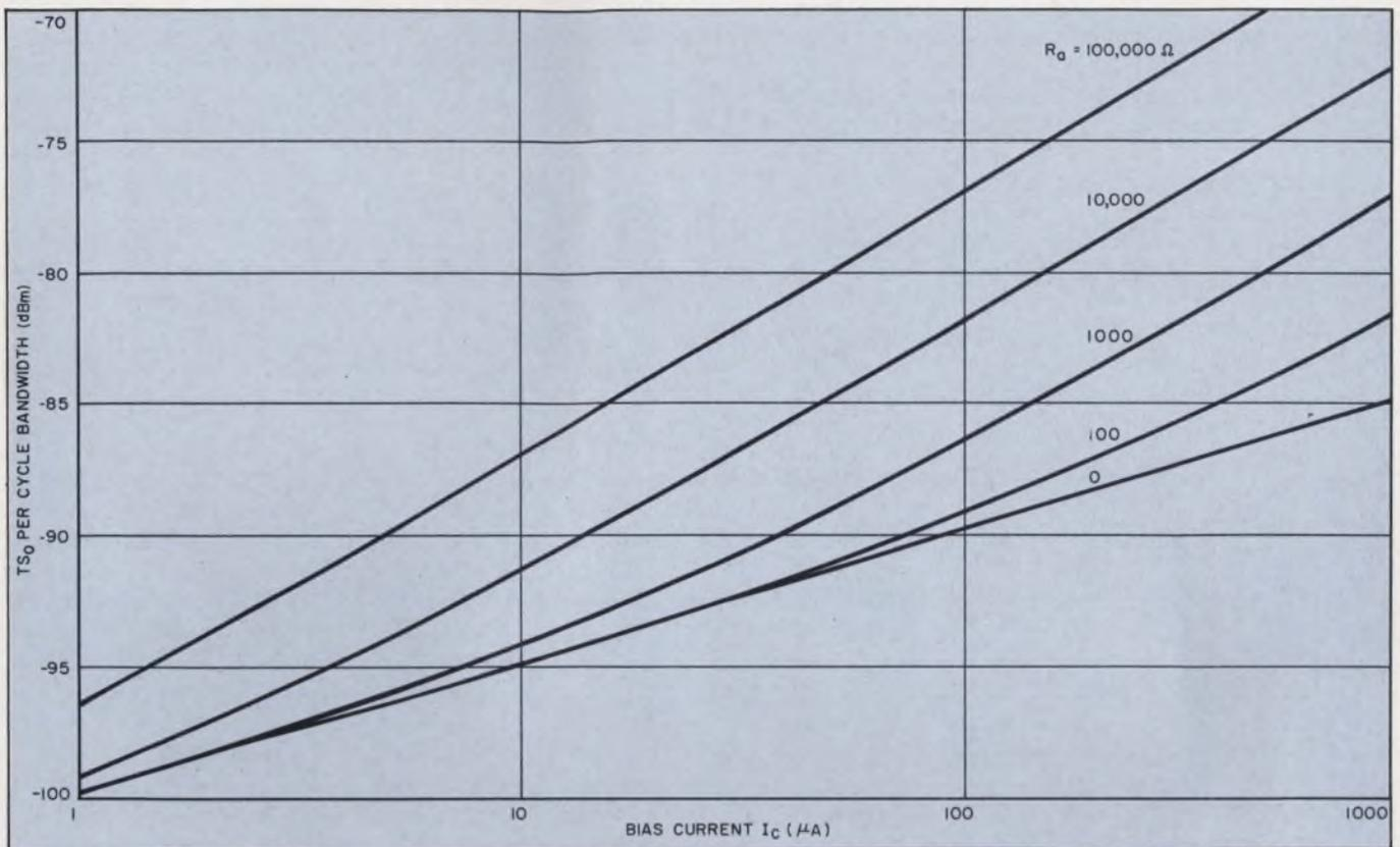
8. The dc tangential sensitivity,  $TS_o$ , decreases with increasing bias current and with increasing  $R_a$ .  $R_a$  is the
