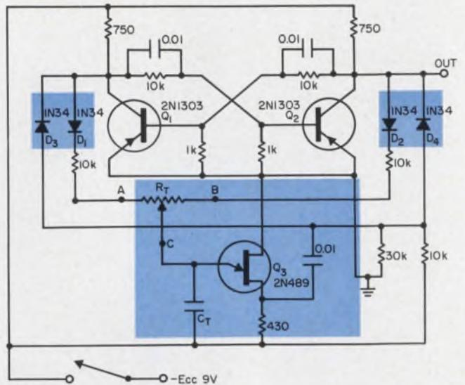
UJT, steering diodes and potentiometer add to versatility of bistable multivibrator.  $Q_3$ ,  $D_1 - D_2$  and  $R_T$  enable symmetry, pulse width and repetition rate to be independently controlled.
