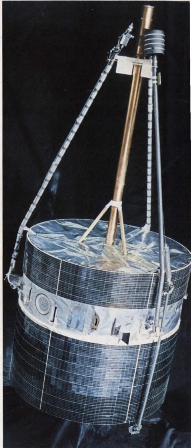
Pioneer VI space vehicle was launched on Dec. 16, 1965 to provide data on interplanetary environments. Its electronic equipment is powered by 10,368 individual solar cells. (paper 67.2)
