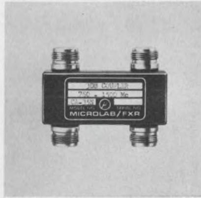
A 25 dB directivity over a full octave frequency range, with a  $\pm 1$  dB coupling deviation are featured in Series CA hybrid couplers. Mainline vswr is 1.15. Six units cover the 200 to 4000 MHz range in overlapping octave bandwidths, with either N or TNC connectors. The 4-port devices offer both ends of the auxiliary line.
