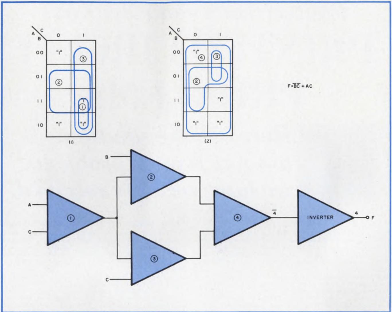
9. Inverter is needed at the output when '0' blocks are generated by the map-factoring method. This is because
