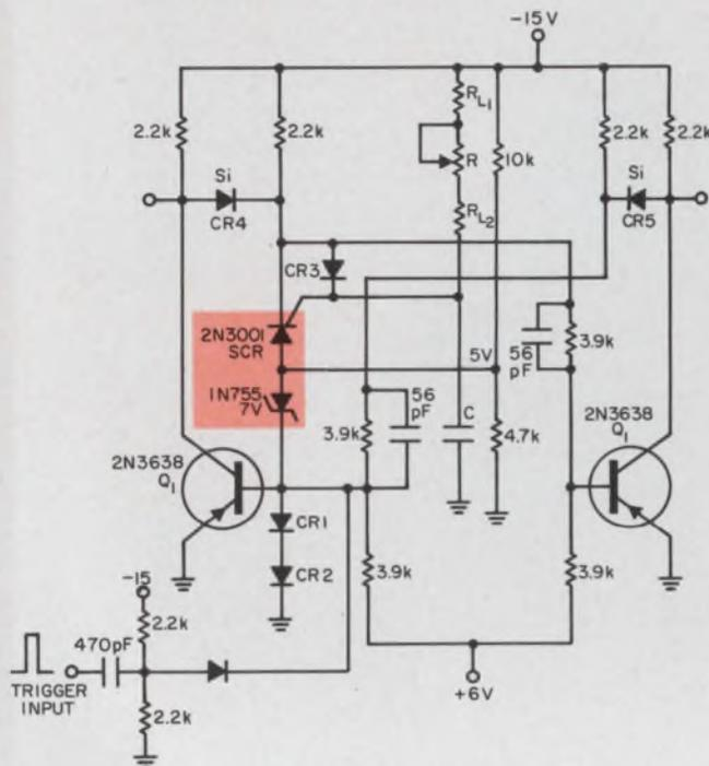
This modified one-shot multivibrator uses an SCR-zener combination for longer time delays and squarer outputs. In effect, these components isolate the timing elements from the switching network.
