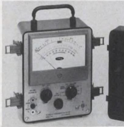
Diodes, rectifiers, transistors, and FETs are checked by model 259 in- or out-of-circuit. It measures both transistors and diodes, in-circuit, for reverse leakage down to 500 ohms of loading. It also measures FETs for leakage and transconductance, and both low and high power transistors for Beta ( $h_{fe}$ ) within a 1 to 100 range.
