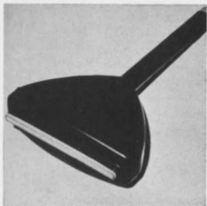
Three new CRTs are offered. The KC237P (pictured) is a line-scan type featuring a flat fiber optic faceplate; it is used to display separate line-scan for film readout. The KC2287P is a fiber optic tube with 3-in. diameter, designed for radar application to convert circle to line scan. The K2619P is a 5-1/4-in. faceplate, single beam type unit for computer readout.
