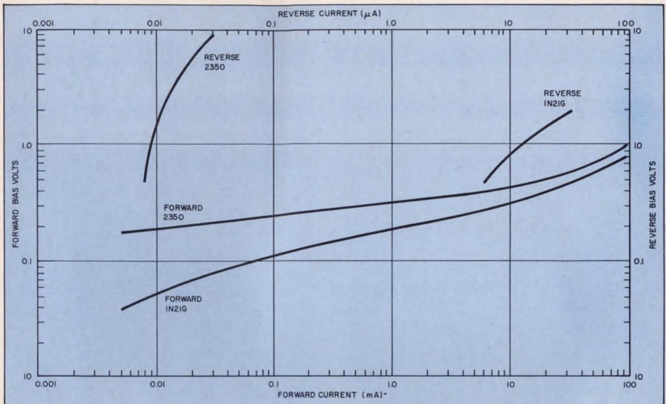
5. The value of  $\bar{x}$  is the slope of the log-log plot of the V-I characteristics, shown here. For hot-carrier diodes  $\bar{x}$  is much larger and remains constant over a larger range of
