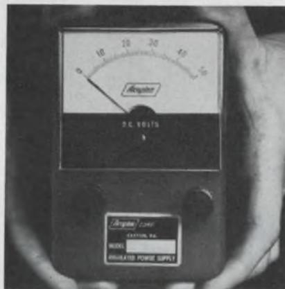
The Pow-A-Meter is an adjustable power supply with an integral voltmeter. The supply can be plugged into a breadboard, instrument or other equipment, eliminating the need for external power supplies, voltmeters and leads. Four models are available with nominal output voltages from 6 to 50 V and current out from 200 to 500 mA.
