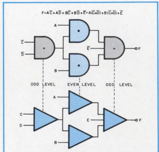
4. By rearranging the function equation, complemented variables can often be located at odd logic levels.
