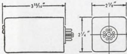
Select Type CCO-23MD for an ultra stable time base. Compact plug-in unit incorporates a high Q glass sealed crystal and full proportional temperature control. Solid state oscillator and oven circuitry assure long term reliability.
