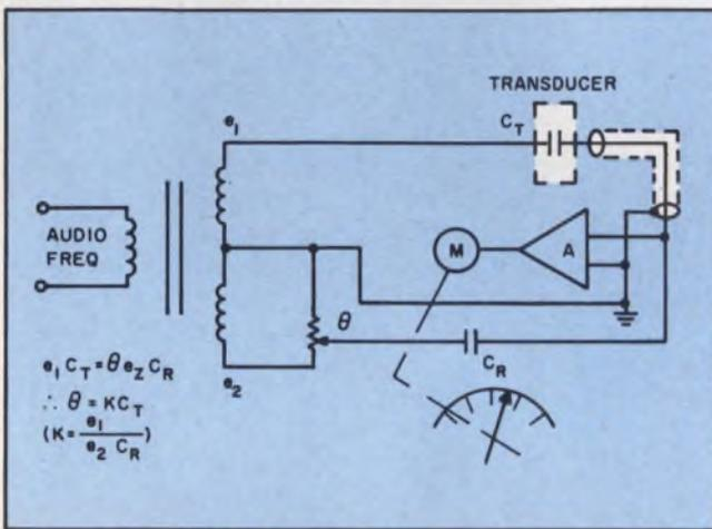
9. Self-balancing servo type of bridge circuit provides a continuous measurement of capacitance. The capacitance value is indicated by a motor-driven potentiometer.
