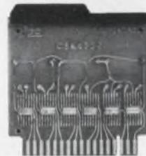
PN-335 NON-INVERTING POWER AMPLIFIER PAC contains 6 three-input AND gates. Each gate contains two inverting amplifiers in series which provide the non-inverted output. Electrically common outputs and built in short circuit protection are standard features.
