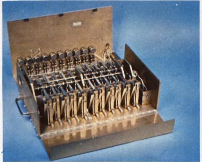
**Single-shot transient analyzer** permits easy analysis of complex transient waveforms. The analyzer was developed by General Dynamics/Convair for use in electromagnetic compatibility measurements. (paper 65.2)
