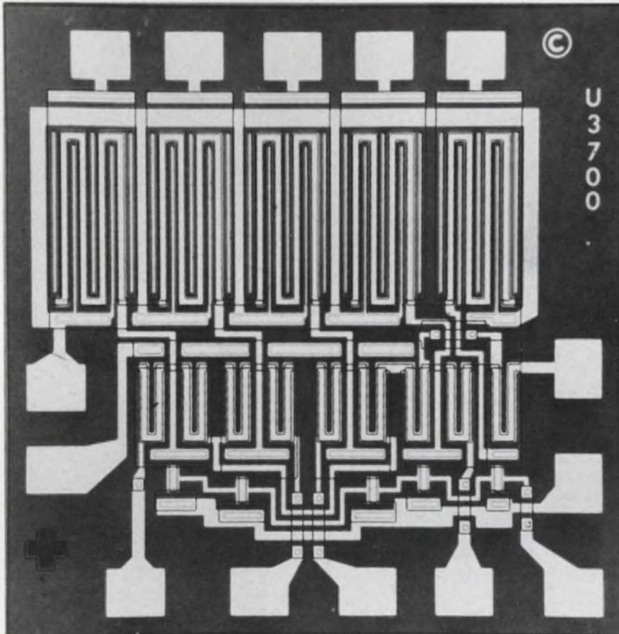
Multi-channel IC commutator has low on-resistance.
