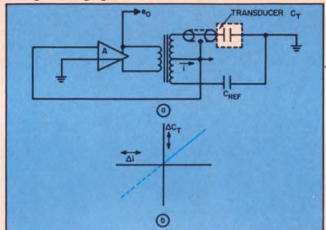
7. Basic RF oscillator circuit has a disadvantage in that it responds to the capacitance of the lead connecting the transducer to the measuring circuit.
