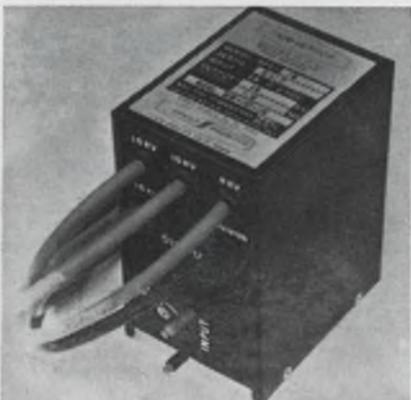
Model SFU High Voltage Converter outputs are from 6 to 20 kVdc tapped in 2 kV steps, up to four common-ground taps.
