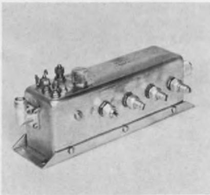
Model VM-2250/100-10, uses the newest snap-action diodes for s-band telemetry multiplying.
