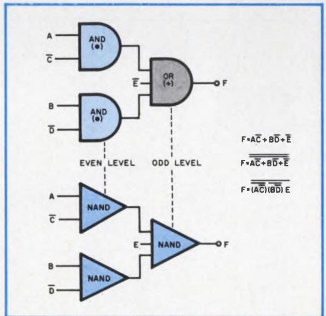
2. AND/OR TO NAND transformation results in the complementing of all variables that are present at odd levels. Variables at even levels are not.
