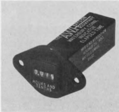
Two microminiature elapsed time indicators for operation on 28VDC, include model K19703 with a four digit counter providing a maximum of 9999 hours; K19702 has a four digit indicator for hours and tenths. Maximum readout is 999.9.
