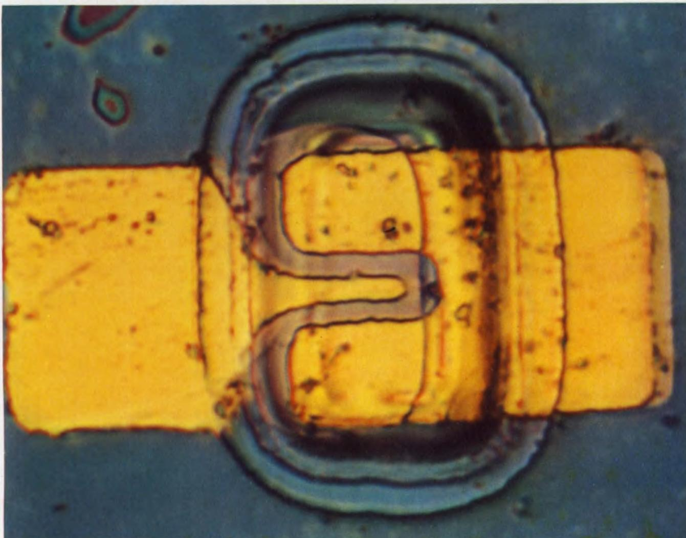
**Schottky barrier diode** will serve as a balanced mixer in the phased array radar being developed by Texas Instruments. The diode is formed in epitaxial packets in high-
