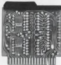
LD-335 NEGATIVE LOGIC LEVEL DRIVER PAC contains 8 two-input AND gates, followed by level shifters. Standard  $\mu$ -PAC signals (+6 V and 0 V) are converted to negative logic levels (0 V to -25 V at 60 ma per circuit).
