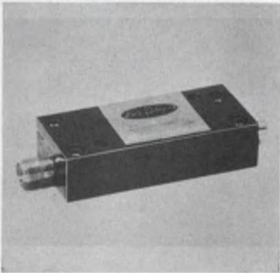
A series of three video detectors measures under 0.75 cu in., meet Class 4 environmental requirements of MIL-E-5400 and MIL-T-5422. All three units can be operated with self- or external-bias. A typical unit, model TV 11 has a -53 dB sensitivity over the full RF bandwidth from 2-4 GHz with video bandwidth exceeding 17 MHz.
