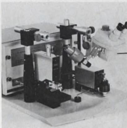
A multi-purpose microcircuit bonding system welds, brazes, parallel-gap soldering and thin-film diffusion bonding.
