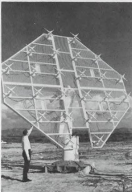
High-gain telemetry monopulse array antenna with 40-dB null depths is destined for use in the Apollo tracking program. Built by Cubic Corp., the antenna has a vswr of less than 1.2 to 1 and a gain in excess of 22 dB in the 215-MHz-to-265-MHz range.
