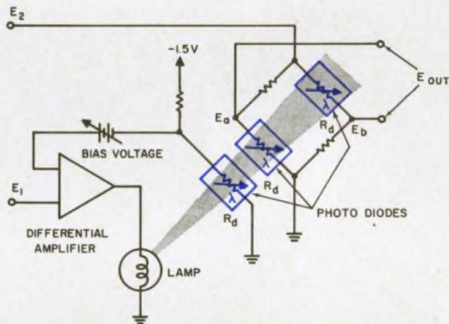
If  $E_1$  is held constant, then an increase in  $E_2$  causes an increase in  $E_{out}$  and a decrease in  $E_2$  causes a decrease in  $E_{out}$ . Thus the voltage,  $E_{out}$ , is a linear function of the light source and the voltage applied to the bridge; or  $E_{out}$  is proportional to  $E_1$  times  $E_2$ .
