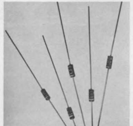
**MW hot-carrier diode**
