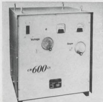
A new rectifier type power supply features continuously adjustable voltage and slope. With a 100% duty-cycle rating of 600 amps (750 at 60% duty-cycle), it has an 85% or better efficiency rating, and a 0.9 or better power factor. Rectifiers are surge-rated at 8000 amps.
