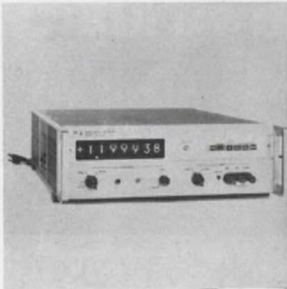
A 1 ppm resolution is featured in the Model H04-3460A Digital Voltmeter. An integrating-potentiometric unit, it measures 100 mV within 0.005% of reading. Accuracy is retained for at least 90 days. Designed for automatic operation in digital data acquisition systems, the unit's four ranges, up to  $\pm 1000$  V, can be selected.
