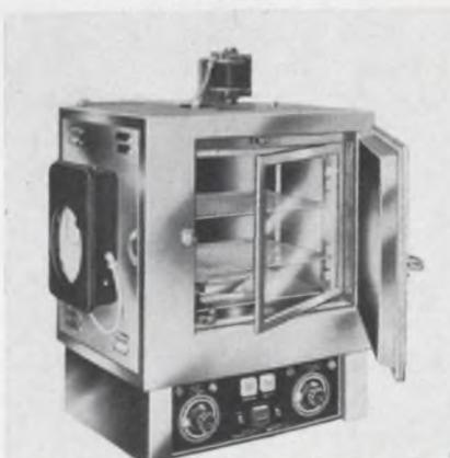
An air-cooled combination temperature/humidity cabinet is capable of meeting MIL-202C, method 106B and other stringent single steady state test requirements.
