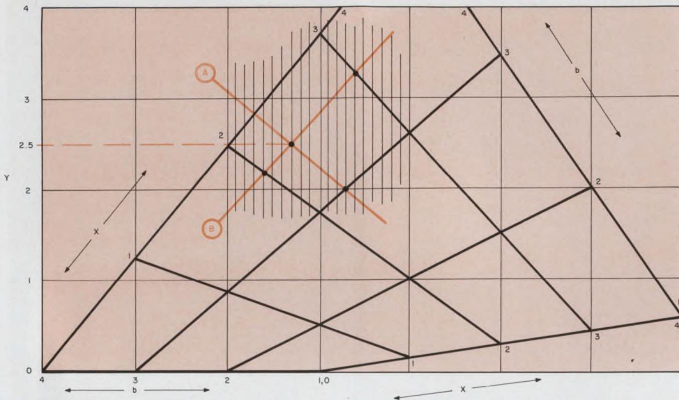
7. Interpolation for points where  $X = 2.3$ . By observing the intersection of the lines A and B relative to the graph's
