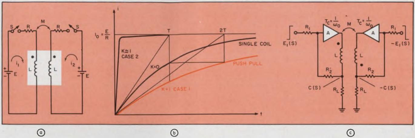
5. Push-pull circuits are sometimes preferred to single-ended deflection stages (a) because they offer constant load, less stringent power supply needs and ease of display referencing. Bandwidth and current rise time with
