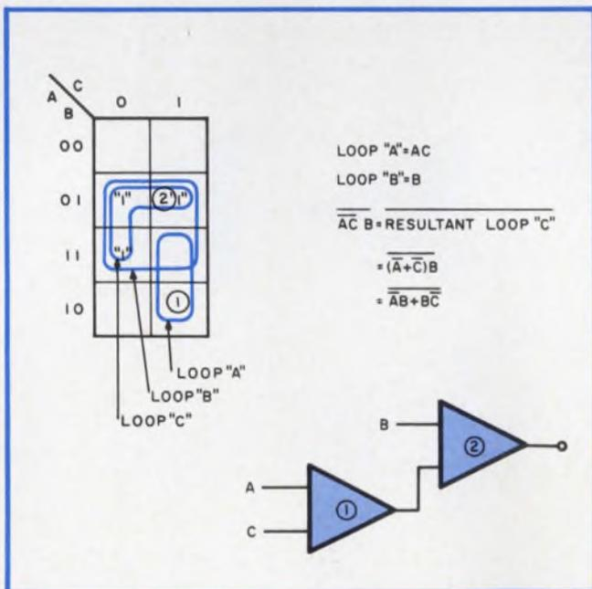
6. Either all "0" or all "1" blocks of the map must be generated when using the map-factoring method.
