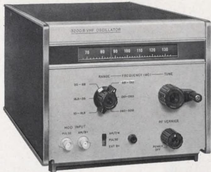
The VHF Oscillator Model 3200B is designed for general purpose laboratory use including receiver and amplifier testing, driving bridges, slotted lines, antenna and filter networks, and as a local oscillator for heterodyne detector systems in the frequency range from 10 to 500 mc.
