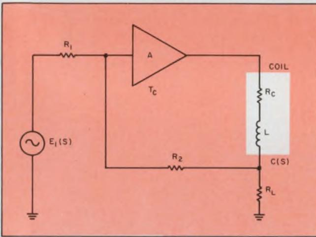
4. Greater coil inductances exhibit large resistances. For larger yokes, the resistor's influence on the transfer function must now be considered. Here  $R_c$  denotes the coil resistance, which modifies the gain and feedback values, according to its comparison with the load.
