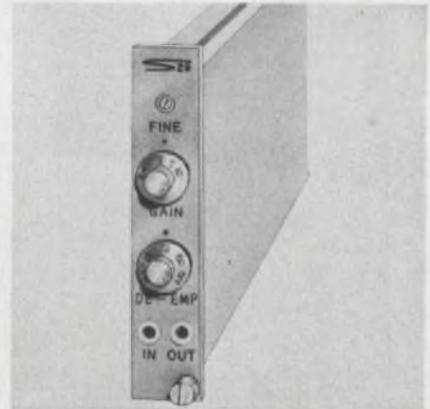
Features of the Model S-29 telemetry amplifier include a switchable de-emphasis circuit and a frequency response of 300 Hz to 2 MHz at a gain of 5 or less. In addition, dual inputs provide a low impedance for summing the outputs of the manufacturer's line of VCOs containing built-in mixing resistors. Output voltage is 20 V and current is 100 mA.
