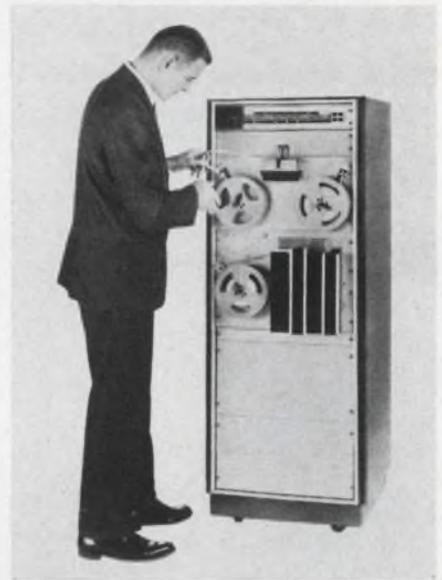
Speed of 1200 words per minute is offered by the System 311, which can operate over standard telephone lines.
