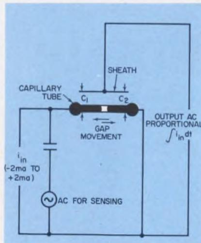
$C_1$  and  $C_2$  are differentially proportional to the position of the electrolytic gap, thus proportional to the time integral of the input amplitude.
