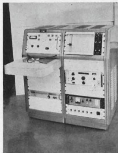
Wide-range filter test set was developed by Sylvania Electronic Systems for use in high-volume filter production (paper 28.1).
