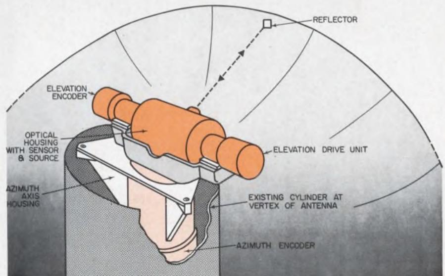
**Photoelectric sensor and source, mounted on a platform at the vertex of the antenna, directs a laser beam at one of 1100 reflectors. The system is designed to detect surface deflections by measuring the angular coordinates of the targets with an accuracy of  $\pm 5$  seconds of arc.**
