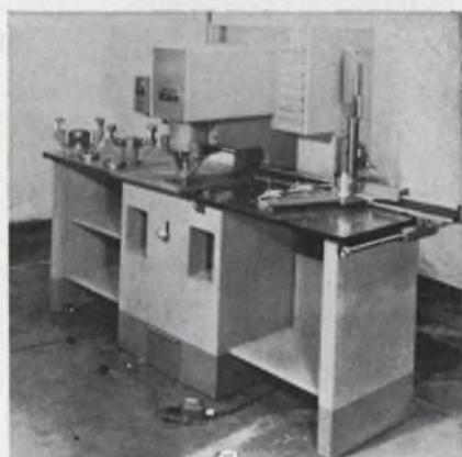
A 30 ton capacity sheet metal fabricator punches 1-in. diameter holes in 1/4-in. material or 3-1/2-in. holes in 10 gauge material.
