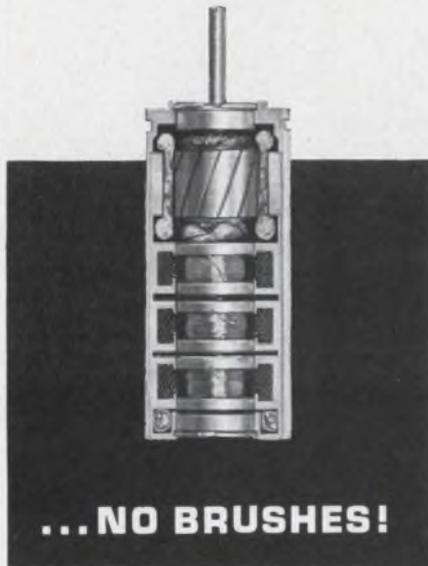
Rotary transformers couple power into rotors without contact, eliminating the number-one cause of early synchro failure. Without brushes, synchro life depends on bearing life alone—normally at least 5 or 6 times average brush life.
