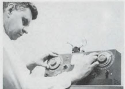
1. T. A. Benham operates a Heath Impedance Bridge that he fitted with Braille-readout dials.
