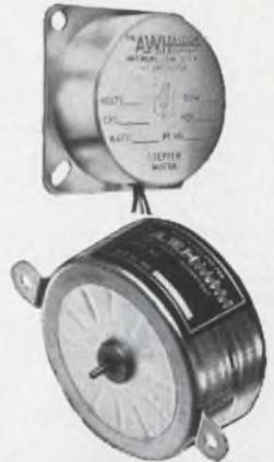
These steppers respond in discrete shaft angle increments to pulsed inputs. Some of their uses are driving counters, positioning synchros, pots, or rotary devices; driving cams, actuators, drums, or charts. They can be used for integrating timing, data transfer, count or position memory, and for digital/analog conversion.
