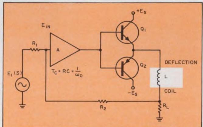
1. In a single-ended deflection system the yoke is connected to the output of an emitter-follower stage. A voltage-drop sample of coil current is then fed back to the preamplifier. Observe that the preamp is the limiting factor on over-all bandwidth.
