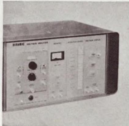
The Diramic Ubiquitous spectrum analyzer covers all frequencies simultaneously in real time within an analysis band up to 10 kHz. The standard model has a 48-dB dynamic range and 60 dB and 72 dB options are available. An internal memory can be used to capture transients and replace tape loops and storage scopes.
