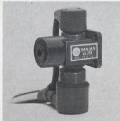
A reflex klystron oscillator designed as a pump tube for parametric amplifiers and masers, the VA-294 delivers a minimum of 100 mW into a matched load over the entire tuning range. Tubes are available to any specified frequency between 26.5 and 40 GHz, and offer a 1 GHz mechanical tuning range. They may be cooled by conduction, forced air or liquid immersion.
