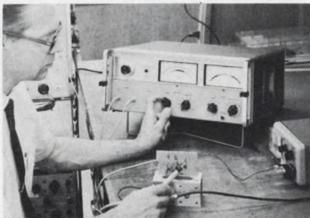
2. Hewlett-Packard vector voltmeter is used to provide voltage and relative phase measurements at a glance.
