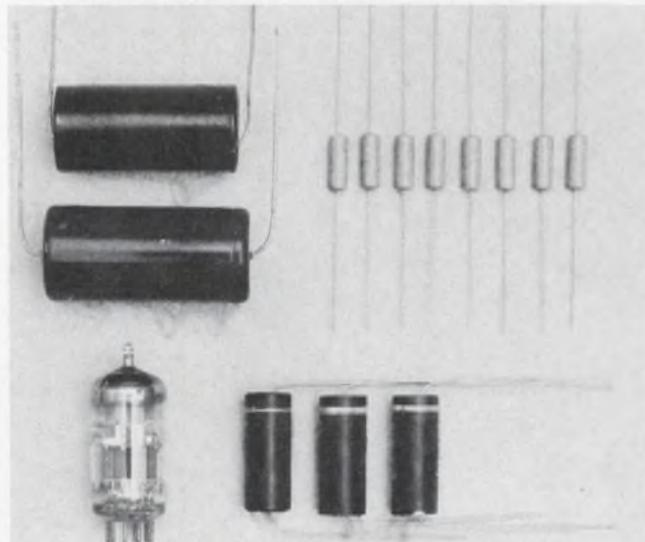
**Reap another benefET!** In addition to the superior performance FETs offer in audio equipment, they require (top) less in the way of associated components and size than bipolar (middle) and tube (bottom) counterparts.
