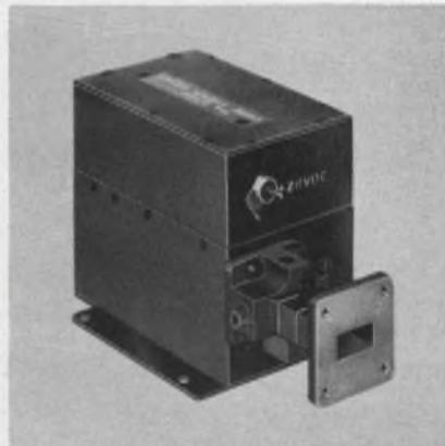
Short-term stability of  $\pm 5 \times 10^{-9}$  100 ms and  $-30$  dB spurious response are featured in the MA-8730. The solid-state, crystal controlled local oscillator operates in the 14-16 GHz frequency range. Minimum power output is 4 mW with low input power drain on a single 28-V supply. The 1.5 lb unit has data link applications.
