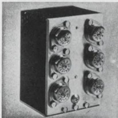
The Voltrac is an over-or-under voltage protector capable of protecting circuitry by shutting down a power source delivering up to 100 Amperes. It may be specified to operate at any differential voltage from supply nominal, and can be wired to track the output of an adjustable supply while still providing protection. An integral contactor is included.
