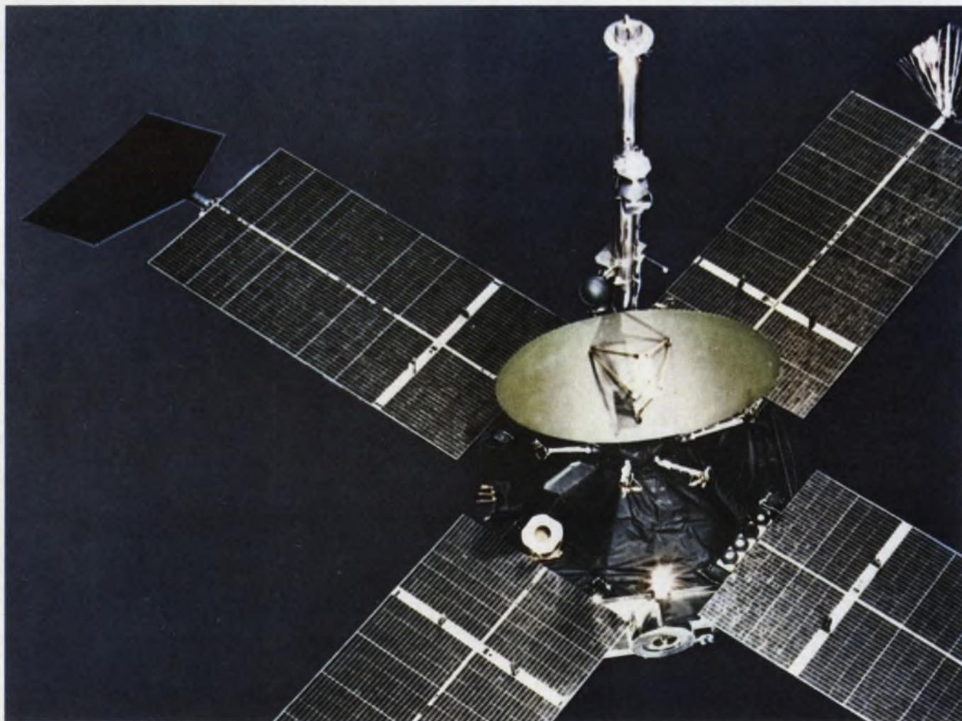
**Mariner IV** completed its flight to the vicinity of Mars on July 14, 1965 and sent back photographs and other measurements of the "red" planet. Its 10-watt telemetry
