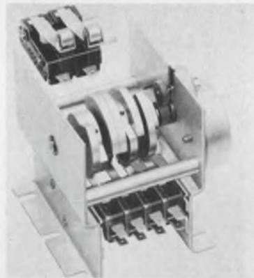
Over-all cycle times from 6 seconds to 25 hours are available with the L42401 and L42402 series of repeat cycle timers. Up to eight SPDT switches are available to control either 15 or 25 A loads at 115 VAC, 60 Hz. Synchronous motor drive is furnished for either 6, 12, 24, 115 or 230 VAC, 50 or 60 Hz operation.
