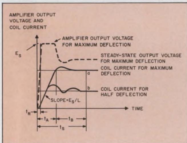
6. Overdriven stages aren't faster! The plot of output vs time for various overdrive conditions shows that settling time  $t_s$  remains fairly constant. Since overdriving does not speed up the settling time, it is not a recommended operating mode. Moreover, greater power is called for.
