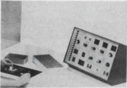
A high-speed go/no-go diode and transistor tester has 10-second program changing.
