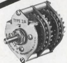
**Type 2A:** An instrument control switch of the highest quality possible with a reasonable price. This switch is a must for all applications where the rating and requirements are high. Rating 5 amp carrying. Size  $1\frac{3}{4}$ " by  $2\frac{1}{4}$ ". Available in all combinations with up to 26 decks and 2 to 26 positions. Has adjustable stop. Solenoid operated if required.
