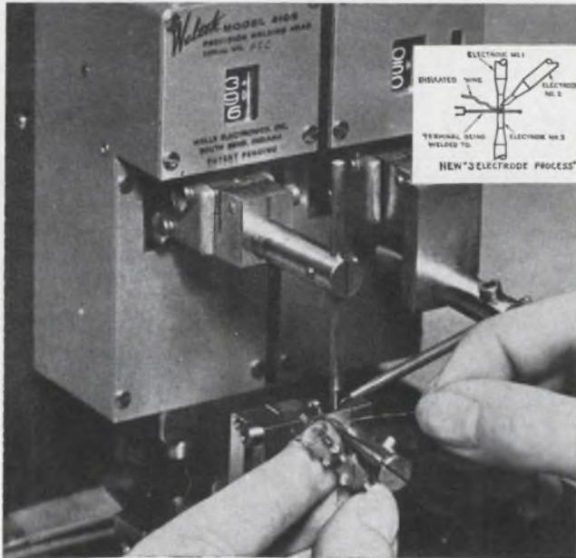
Get rid of costly wire stripping operations... ask about our new AC-10/410-E system. It welds through insulated wire (up to .010" dia.) in less than 1/3 second. Send samples.
