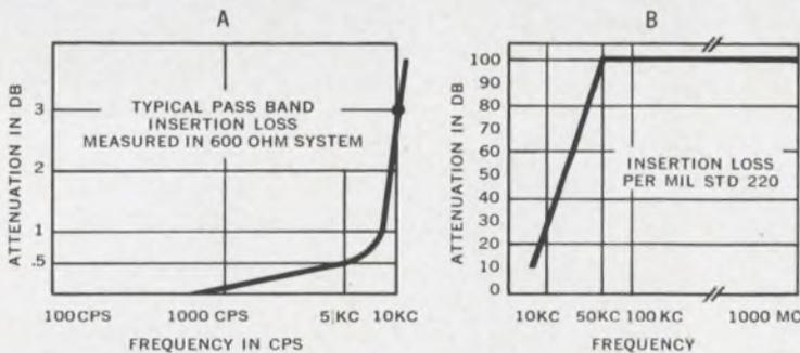
Graphs A and B show typical characteristics of Potter signal line filters. These filters are used on systems which must meet Defense Communications Agency criteria and provide maximum attenuation above the pass band with less than ½ db attenuation in the pass band. ■ Write for further information on these and other Potter filters.
