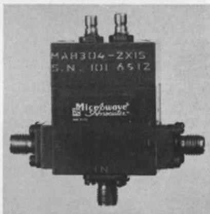
Capable of operating at any 500 MHz band in the 7-12 GHz frequency range, the MA-8304 S is a low power spdt switch. It weighs 2.5 oz and has a switching time under 10 ns. Power handling capabilities are 25 W peak and 2 W average. Insertion loss is 1 dB and isolation is 20 dB. Uses include antenna lobing, system calibration and pulse shaping.
