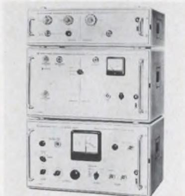
Test assembly type LFM determines group delay and phase distortion of transmission systems. The group-delay measuring section has  $\pm 1000$  ns,  $\pm 300$  ns,  $\pm 100$  ns,  $\pm 30$  ns,  $\pm 10$  ns ranges, all  $\pm 2\%$ . The group-delay test set video modulator covers a range of 100 kHz to 10 MHz. The RF modulator covers 25 to 250 MHz.
