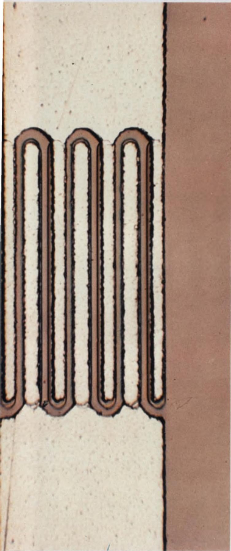
**PIN switching diode** was developed by Texas Instruments for use in IC microwave phased array radar. Over 12,000 such diodes will be required in a system now under development by the company. (paper 45.1)
