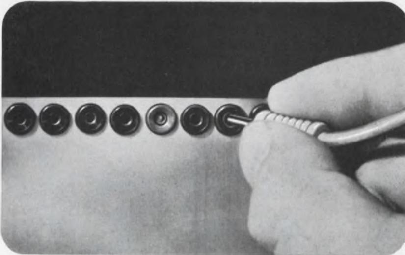
Now Ucinite offers you press-in test jacks for high-density, low-weight applications. Using nylon insulators available in 11 colors, these new test jacks have stamped or screw-machined closed-entry, beryllium-copper contacts that meet the performance requirements of MS-16108. They are available in a variety of terminal styles, and finishes. For complete details write for Bulletin 7072.
