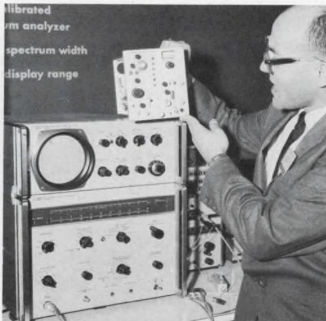
Significant size difference between a plug-in and a conventional spectrum analyzer is demonstrated by the author.
