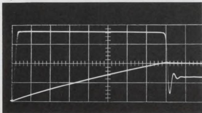
7. Step-up display performance: Coil voltage and coil current data taken from a single-ended deflection amplifier show good agreement with calculated values. For  $E_s = 18$  volts,  $L = 25 \mu\text{h}$ ,  $R_T = 0.5$  ohms and  $T_c = 50$  ns, the system exhibited a settling time of  $17.0 \mu\text{s}$ . One vertical centimeter represents 5 units (volts and amps) and each horizontal centimeter  $2 \mu\text{s}$ . Voltage is displayed as a step function and current as a ramp.
