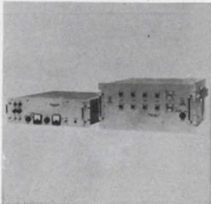
Five bands cover 1.0-18.0 MHz in the Model 135 Multiband amplifier. Output power is 18 W to 12.4 MHz, 8 W beyond. Small signal gain is 35 dB per band. Type "n" RF connections and waveguide are provided.
