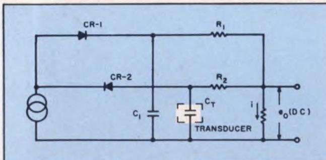
12. Dc output voltage that is a linear function of transducer capacitance is produced by this rectifier-type circuit. Either one or both of the capacitors may be a transducer.
