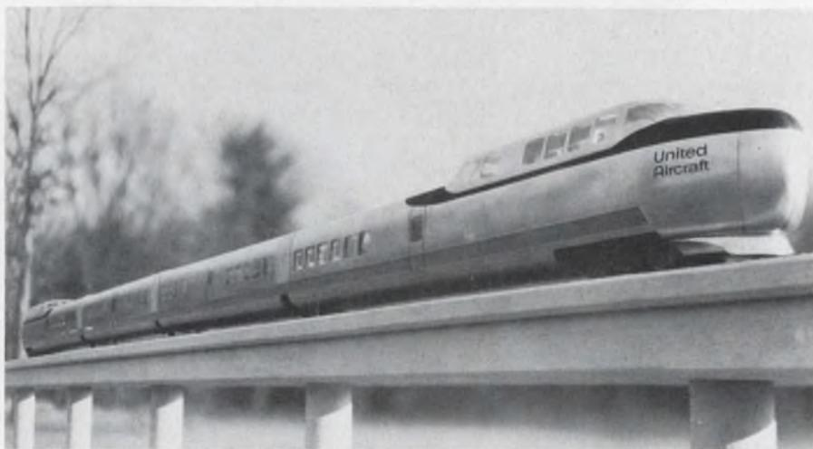
**Gas-turbine engines** will power this high-speed train designed by United Aircraft. Two such trains will be used in a demonstration project between Boston and Providence as part of the Commerce Dept.'s Northeast Corridor Demonstration program.
