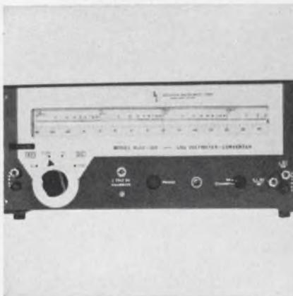
The model HLFC-120 frequency converter provides a dc output voltage directly proportional to the logarithm of the input frequency. Input can vary from 0.5 V to 100 V with high harmonics and not affect accuracy. Output is 100 mV at 350 ohms. Plug-in frequency discriminators cover 3 decades, 5 Hz to 20 kHz.
