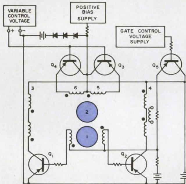
The frequency of the multivibrator is controlled by a full-wave voltage-limiter arrangement of transistors  $Q_3$  and  $Q_4$  and windings 5 and 6.
