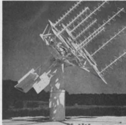
Designed for use aboard instrumentation ships, a line of telemetry antennas is mounted on a heavy duty positioner and is reported to withstand 120 mph winds with icing conditions. The elevation-over-azimuth positioner will operate at a maximum speed of 40°/s under a windload of 75 mph.
