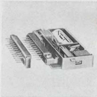
A single-digit count module displays its count visually as it indicates it electrically. These units may be mounted side-by-side to form a multi-digit counter for electrical control functions.
