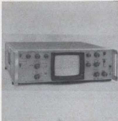
For testing TV waveforms, Model 191A oscilloscope features a 1% vertical accuracy for most measurements, 1% stability for all operations. A new CRT shows low-duty-cycle signals full screen. T/2, T and 2T sine-squared test pulses, used to test transmission facilities, are 62.5 to 250 ns.
