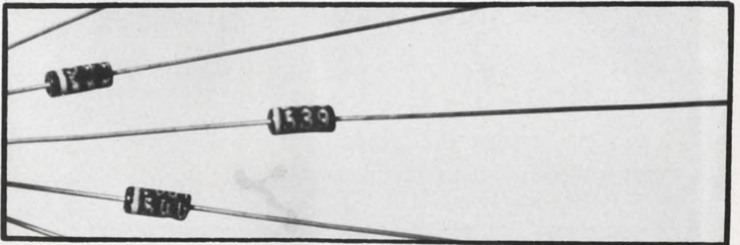
Schottky diode has 6.5db noise figure at 2.5GHz. 266
