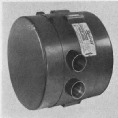
Up to 94 cfm air-flow and 2 psig pressure are featured in the Spiral blower. Three versions are available, including model SL6. This unit, in computer applications, uses two independent air paths to serve separate functions. One, for magnetic tape slack control; the other, for capstan motor cooling. Other models are for document and card handling.
