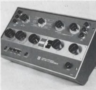
A guarded high-precision potentiometer, known as the K-5 model contains improvements over the earlier K-3. Range and balancing controls are aligned from left to right in order of usage.
