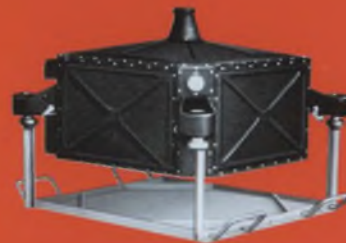
Saturn I guidance computer continuously determined the course to achieve orbit. In six test flights, these computers NASA Saturn I vehicle controlled the direction and thrust of second-stage engines. The computer on four of the flights controlled four of the first-stage engines as well, and also timed engine
