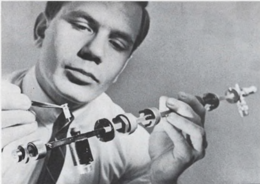
Millimeter-wave Gunn-effect device packaged in standard crystal mount is inserted into waveguide by RCA scientist. Forty milliwatts at 40 GHz is reported from the new epitaxially grown unit.
