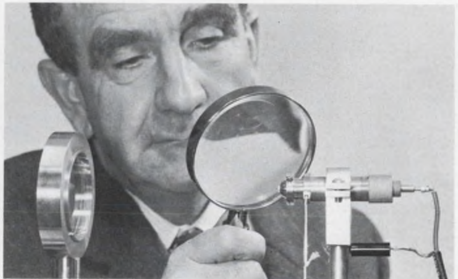
Optical radar transmitter electrodes under examination by the system's inventor, Dr. Heinz Fischer of the Air Force Cambridge Research Laboratories. The system is said to be superior to the laser for short-distance ranging. The lens shown at left focuses the light to increase range.
