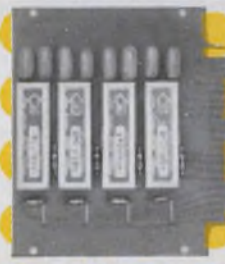
HGSW functional circuit incorporating HGSM steel-enclosed modules and additional components
