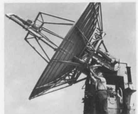
Antenna for the Moon Bounce system is a 16-foot-diameter dish.
