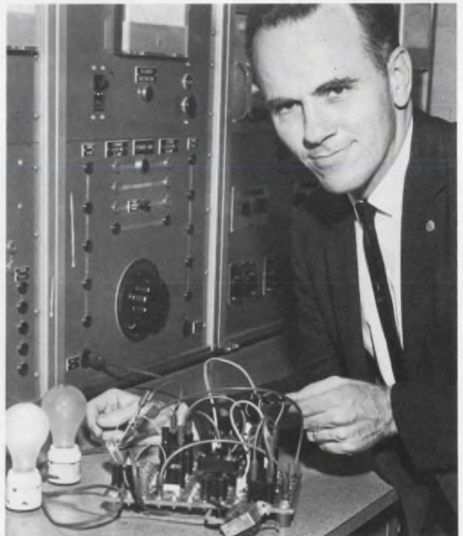
To make one light dimmer Author Howell uses his all-solid-state dual flasher design. It provides balanced control of the intensity of the two lamps.
