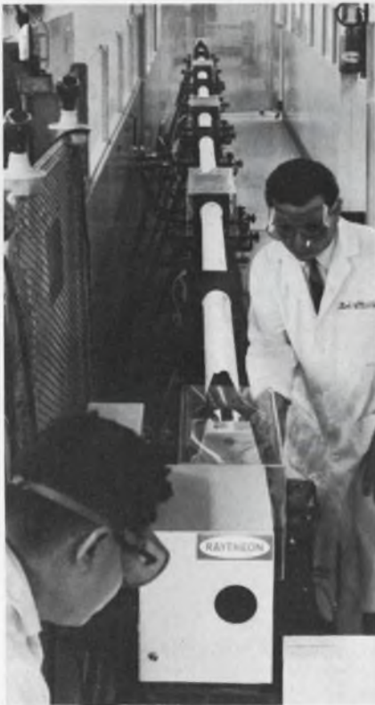
At least 500 watts of cw power is delivered by Raytheon's CO 2 laser.
