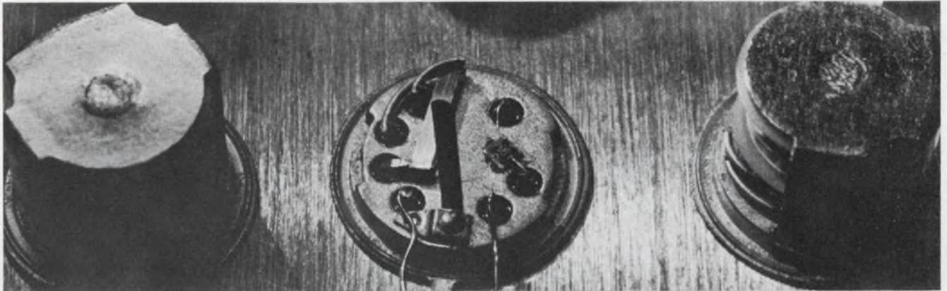
A relay and a FET in a TO-5 can? For operation off low-level micrologic, this spdt relay has its
