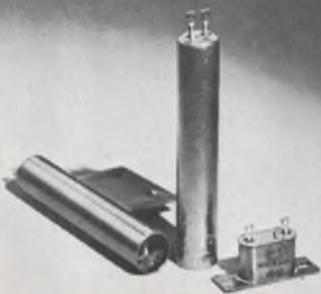
**Cartridge Type:** Series C8 hermetically sealed and still adjustable. Contact rating up to 5 amps. **Crystal Can Size:** Series VE-2 hermetically sealed. Contact rating up to 3 amps. **Features:** Rapid rate of response; minimal differential; operating range,  $-65^{\circ}$  to  $+300^{\circ}\text{F}$ ; vibration to 2000 Hz; shock to 50g.
