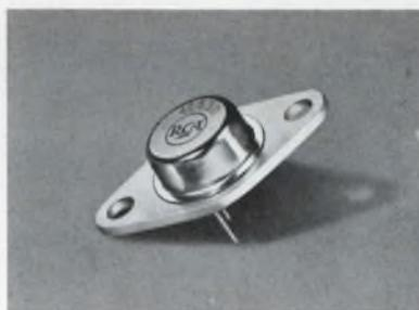
RCA brings you a new generation of control devices! Each of these 6-amp Triacs can provide the same full-wave function as *two* SCRs... with the option of using either positive or negative gate-trigger signals. Hermetically sealed in an all-welded TO-66 package, RCA 40429 and 40430 can simplify your control circuits... reduce costs... add reliability and efficiency.
