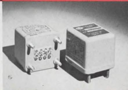
Series 900-064 has been accepted as a standard for many military and aerospace applications where high quality, reliability and cost are requirements. **Features:** hermetically sealed; fixed or adjustable time delays 0.1 to 60 sec.; solid state or relay output; vibration to 2000 Hz; shock, 50g.
