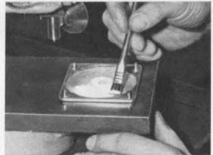
G-E two-part RTV, available in a range of viscosities, seals filament condenser plate in dielectric heater. Also protects against vibration.
