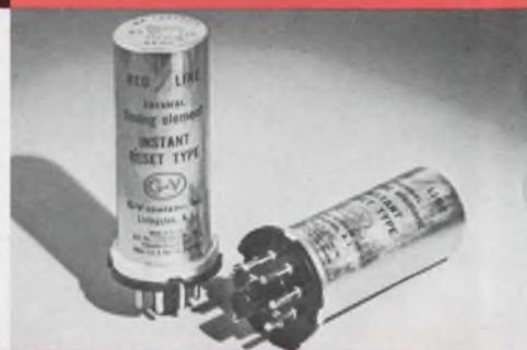
G-V is the largest source and offers the widest variety. Several types are hermetically sealed and still adjustable. All meet requirements of Mil-R-19648. Available in a wide variety including: sub-miniature, miniature, octal and missile types. **Features:** delay time, 0.1 sec. to 3 min.; heater voltages to 230 V; ambient operating temp.,  $-55^{\circ}\text{C}$  to  $+125^{\circ}\text{C}$ ; vibration to 2000 Hz; shock to 50g.
