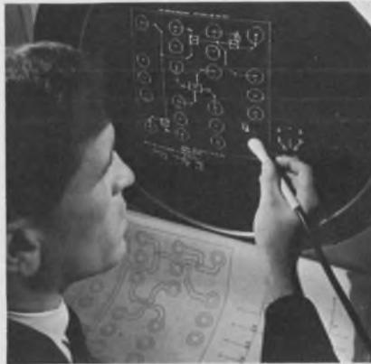
**Computer-aided computer design**—with a computer-controlled graphic display and light-pen. Final hard-copy drawing is used to make mask for actual fabrication.
