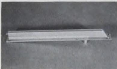
**Solution:** Amecom's Blade Antennas that provide horizontal and vertical polarization; 2% bandwidths tunable over a 15% band, with less than 2.0:1 VSWR.
