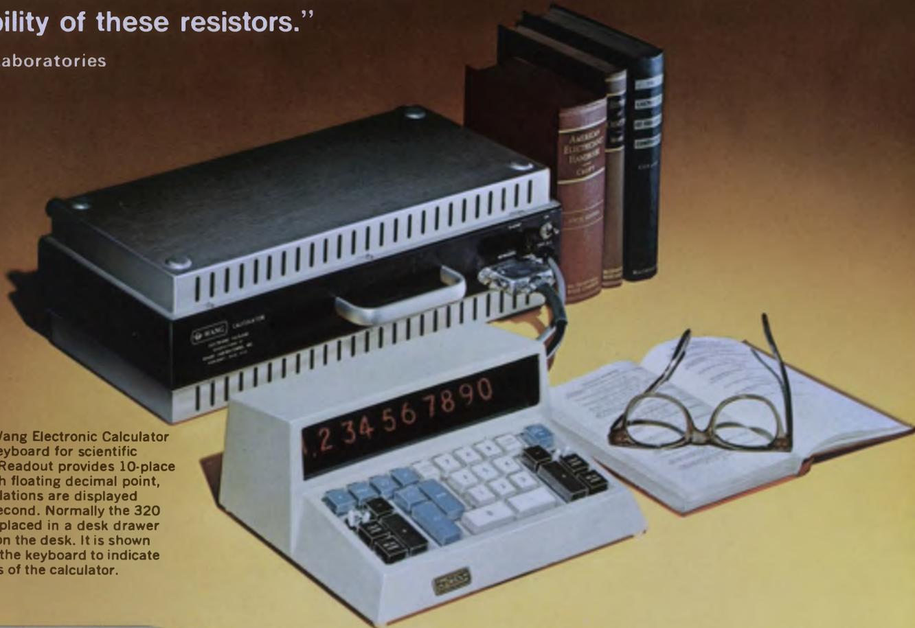
Model 320 Wang Electronic Calculator with 320K keyboard for scientific application. Readout provides 10-place accuracy with floating decimal point, and all calculations are displayed in one millisecond. Normally the 320 calculator is placed in a desk drawer rather than on the desk. It is shown here next to the keyboard to indicate compactness of the calculator.
