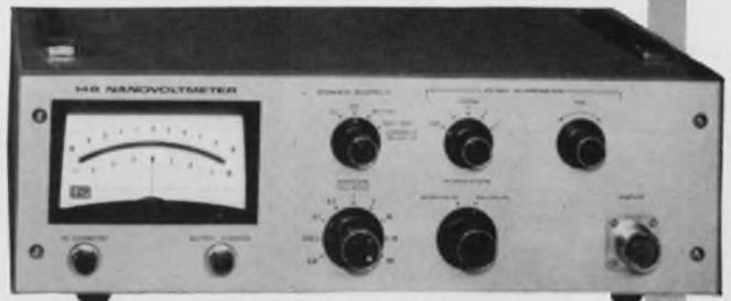
**MODEL 148 NANO-VOLTMETER** — is truly the most sensitive voltmeter ever made. Ideal for Cryogenic, Hall Effect, Thermopile and other similar studies or measurements. It features 10 nanovolt f.s. sensitivity with less than 1 nanovolt noise. And, stability of better than 10 nanovolts per day. Ac input rejection is 3000:1.
