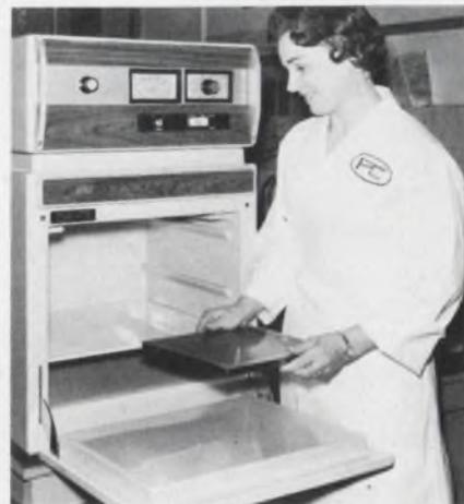
The table-top unit has interlocks on the door and exposure will stop if the door is pulled open.
