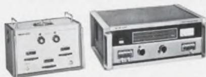
B801B in conjunction with Wayne Kerr SR268 Combined Source and Detector, with single dial tuned system to provide ganged tuning of source and detector from 100kHz-100MHz simultaneously in one operation.
