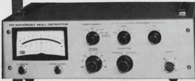
**MODEL 147 NANO-VOLT NULL DETECTOR** — is designed for use with high resolution potentiometers and bridges — L & N 7556, Guildline 9144 or 9120, Biddle 605001, and others. Lets you resolve 0.01 microvolt with a 300 ohm source. Keeps zero shift to less than  $10^{-10}$  volt per ohm. Drift is within 25 nanovolts per day. Ac input rejection is 5000:1.
