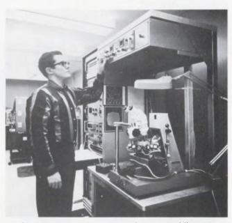
6. The automatic probe-test equipment rapidly and accurately determines which circuits on a slice are good and which are defective. The data are fed to a probe processing program.
