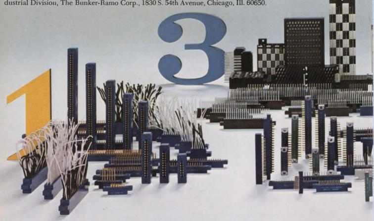
BIFURCATED BELLOWS CONTACTS For smooth, positive mating action—that's easy on your PC board surface—pick Amphenol's 225 Series. Bifurcation provides 2 points of contact, even on irregular surfaces. Bellows action exerts positive pressure, even under extreme vibration. Gives you thousands of insertions and withdrawals without failure. Nine sizes, ten tail styles, four mounting configurations, two contact platings, and solder, taper pin or Crimp Poke-Home® terminations. Exceeds MIL-C-21097B.
