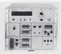
Left: Static tape reader by Hickok provides 540 contacts for each program step on the tape. Above: Digital data logger by Solartron has a capacity of 1000 channels. It responds to a signal of 2.5 microvolts.
