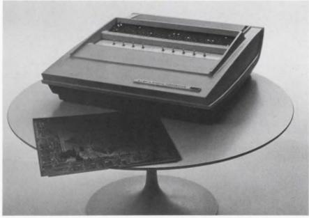
MSI arrives in the Data General Nova computer, which features four accumulators—two used as index registers, in a \$6050 basic machine with 1024 16-bit words of storage. Read-only memory modules are also offered by Data General, to users who provide a paper tape of a debugged program.
