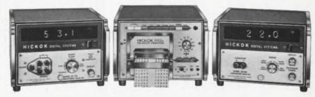
Printer will print the output from two independent DMS 3200 Digital Measuring Systems.
