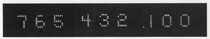
Solid-state indicators display an array of bright red dots in numeral form. The thin,
