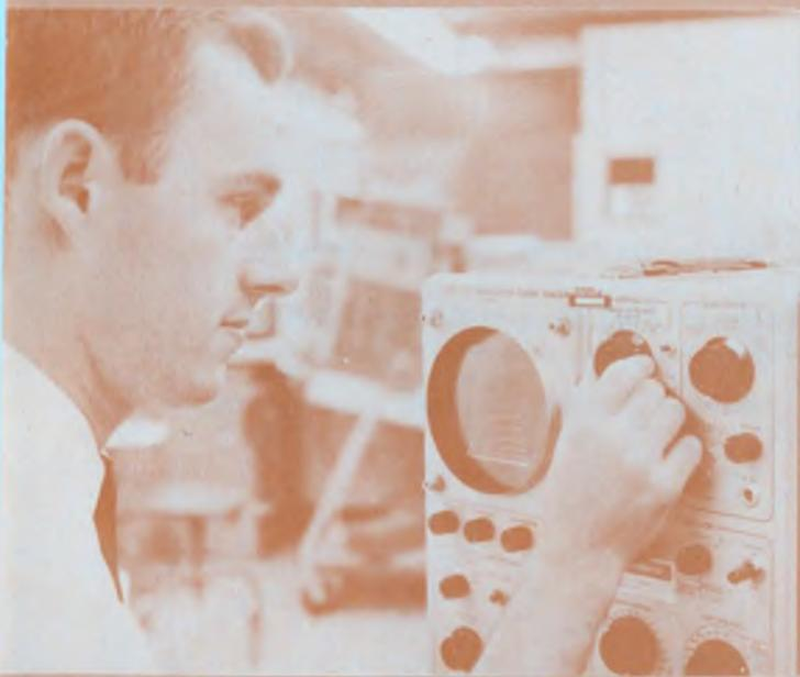
Author Carlson views the family of drain-current vs drain-voltage curves for an MOS unit under test.
