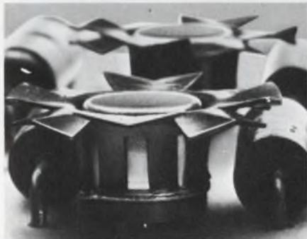
TO5's and TO18's in high density packages can be cooled off with efficient push-on Fan Tops that cost only pennies. T-shaped, need no board room, let other components snugly close. Spring fingers accommodate wide case diameter variations. Models for RO97's, RO97A and D-style plastic devices also.
