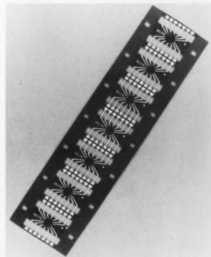
**Silicon IC chips are attached to lead frames that are part of a plastic film strip in GE's new miniMod package. The chips are then encapsulated in a protective epoxy.**
