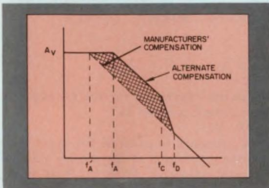
2. Bode plots of both compensation techniques are compared by graphical superposition to illustrate the increased gain for the extended frequency domain. Note the addition of another pole and zero to the Bode plot.
