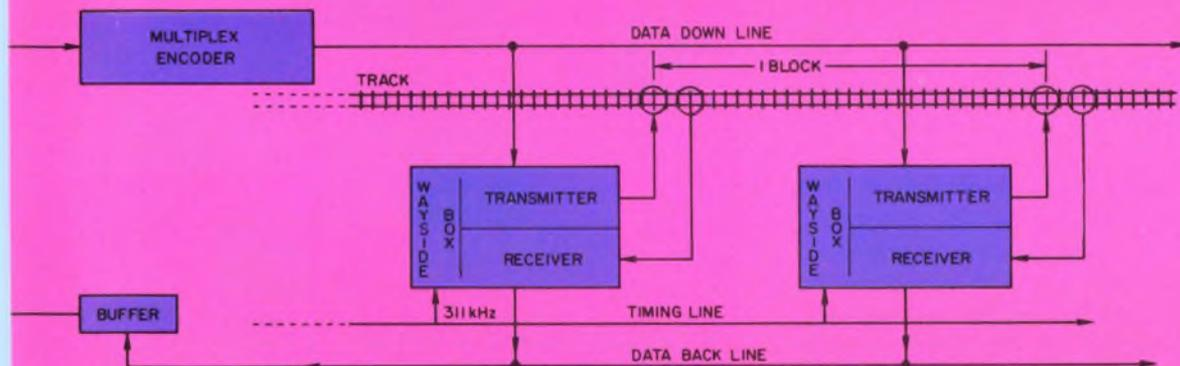
1. Speed commands on the Bay Area Rapid Transit system will be sent to up to 30 wayside boxes simultaneously on a single line with this multiplexed communication system. The comparison of data received with data transmitted in the fail-safe, bit-by-bit comparator yields vehicle location information as well.
