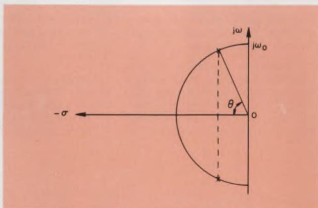
1. The poles of the filter can be arbitrarily placed anywhere in the  $s$ -plane in order to achieve the desired value of damping. The angle  $\Theta$  is given as  $\cos^{-1} \zeta$ , where  $\zeta$  is determined by the relative values of the passive components chosen for the particular active filter.
