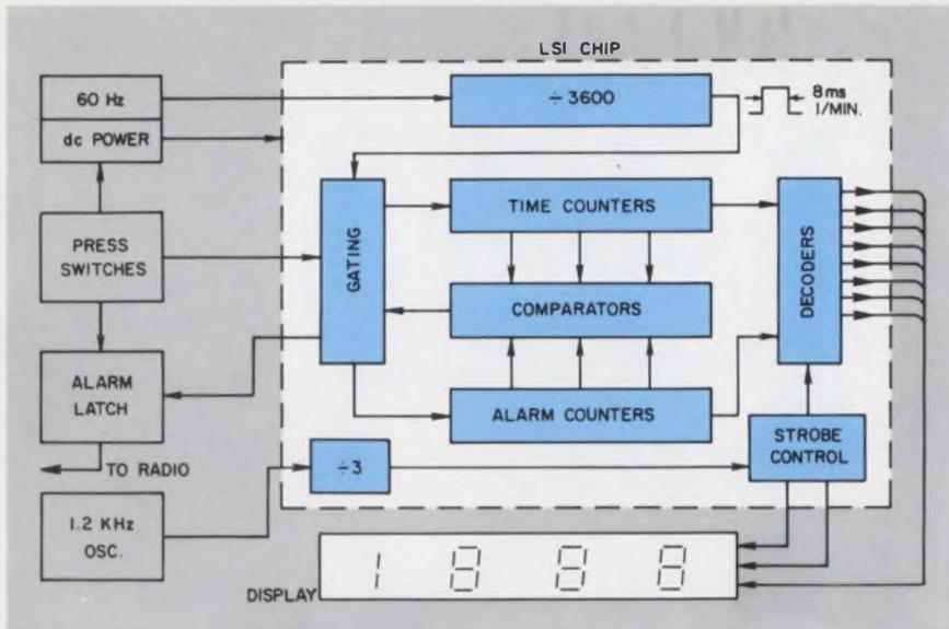
The LSI chip in the clock radio contains timekeeping and alarm circuits that drive the digital readouts. The timing system is controlled by the 60-Hz line. Either the time or alarm-time setting is displayed on command. The cost of the chip is high but will come down in volume production.
