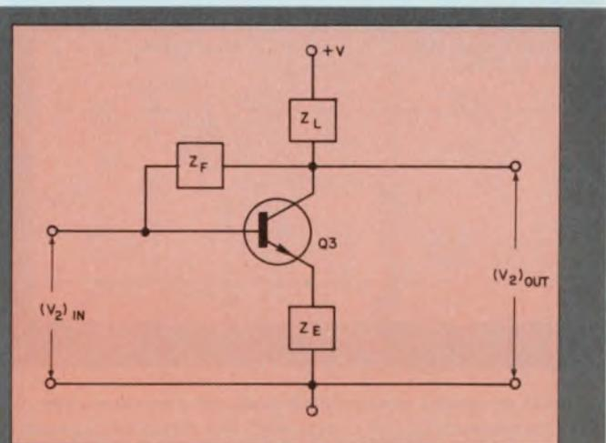
4. The device's second stage is redrawn (a) for analytical simplicity. Internal as well as compensation (external) feedback elements are recognized. The second
