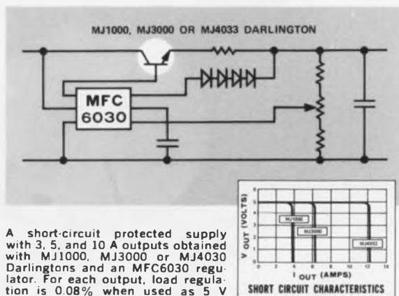
A short-circuit protected supply with 3, 5, and 10 A outputs obtained with MJ1000, MJ3000 or MJ4030 Darlington and an MFC6030 regulator. For each output, load regulation is 0.08% when used as 5 V regulator. Short-circuit characteristics indicate limiting performance with each Darlington. MFC6030 Functional Circuit has 38 V maximum input voltage, 200 mW maximum load current and 3 V minimum voltage differential.
