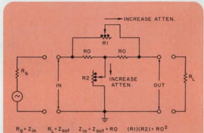
$$R_G = Z_{in} \quad R_L = Z_{out} \quad Z_{in} = Z_{out} = RO \quad (R1)(R2) = RO^2$$
