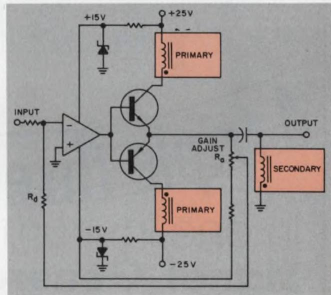
2. The transformer doubles the power and efficiency of the output stage by coupling the power developed in the collector circuits into the load. The output can now provide  $\pm 10$  V at currents up to  $\pm 200$  mA. This circuit can also be used as an oscillator-driver by employing the feedback scheme illustrated in Fig. 1.
