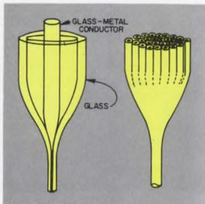
Fiber electron optics begin as glass-coated wires (left) that are stacked and drawn into multifiber bundles (right). A new glass-metal conductor makes possible these large-area high-resolution arrays.
