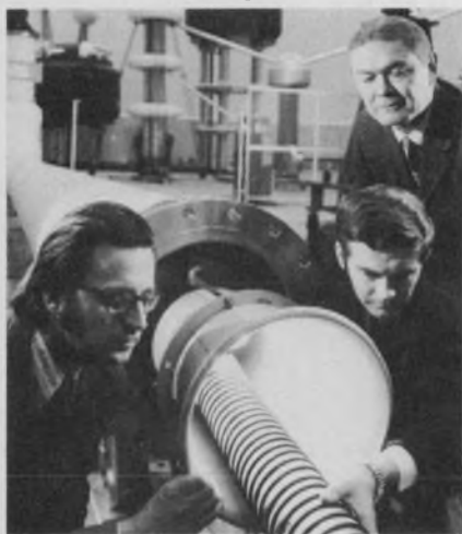
Cryogenically cooled ( -320^{\circ}\text{F} ) aluminum power cable withstood 435,000 V at GE's R&D Center.
