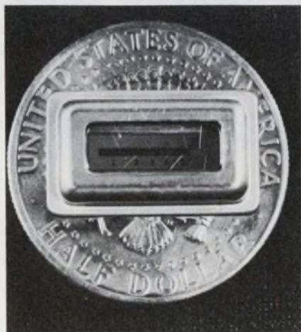
Ten-element spectral array will analyze earth resources from small aircraft flying at 5000 feet.
