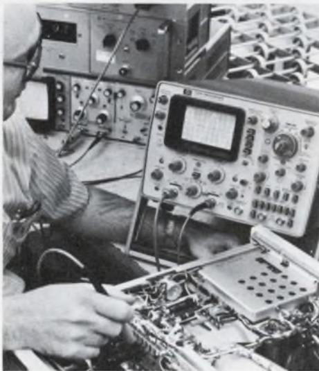
The 1703A variable persistence scope makes it easy to check slowly moving waveforms, such as in medical equipment.
