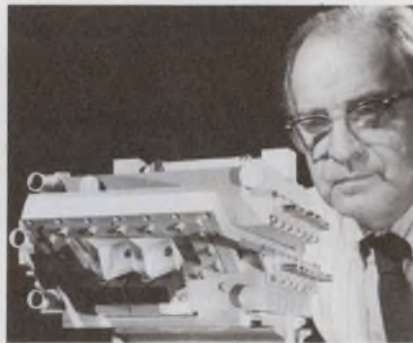
GE's new Big Mini glass laser, built for moderate-power operation (up to several hundred watts, average) is the preamp for a bigger laser.
