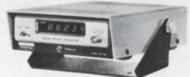
For counting capability into the high frequency region at modest cost, check out the Heath/Schlumberger 80 MHz frequency counters:
