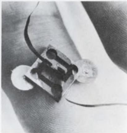
As positive or negative strain is applied across the strain axis of the gage, the capacitor plates either expand apart or contract together. Although the plates are initially in a state of mild compression, they can still compress further together due to the crushability of the Mica.
