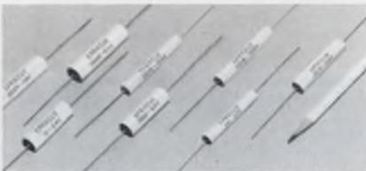
**TYPE 430P METFILM® 'E' CAPACITORS.** High-Voltage metallized polyester-film capacitors designed for voltage multiplier circuits used in electrostatic copiers, TV power supplies, etc. Working voltages from 4,000 to 15,000 V. Capacitance is stable with time, temperature, voltage. Write for Engineering Bulletin 2445.1 or;
