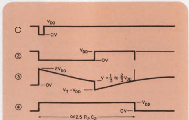
2. Waveforms show the output pulse triggered by a ZERO at the set input.
