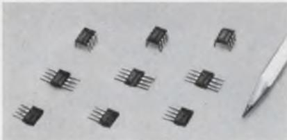
**HALL EFFECT SWITCH ICs.** Actuated magnetically, not mechanically or optically. Hall generator trigger circuit and signal amplification circuit on single silicon chip. Reliable (no moving parts). Easy interfacing with DTL/TTL/MOS logic. High speed. Low cost. Write for Engineering Bulletin 27,402A or;
