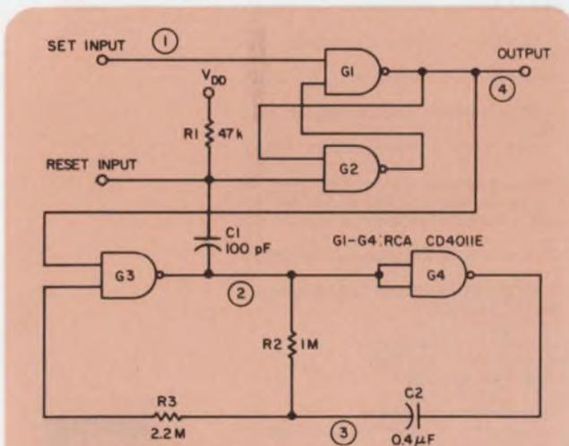
1. CMOS gates  $G_1$  and  $G_2$  act as a flip-flop that governs the period of oscillator  $G_3$  and  $G_4$ .
