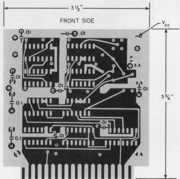
2. You don't always need the ground plane, as in this high-speed counter layout. The capacitors provide low frequency bypassing. Signal lines are short, and no transmission lines are used.
