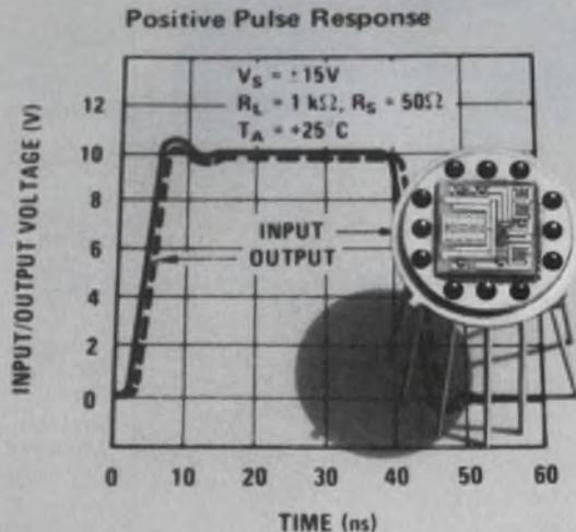
The Halex Model HX 0033 Voltage Follower is a high impedance, unity gain buffer used for ultra high-speed interface requirements. Slew rates are typically 1500 V/usec. Pin-for-pin replacement, \$30. each, in 100-piece lots, off-the-shelf delivery.
