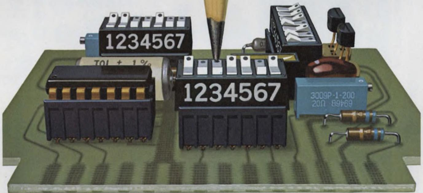
Our DIP switch, in fact. A brand-new device that lets you program your IC's right on their boards. Without the labor costs, nuisance and excessive space required by jumper wires or bracket-mounted toggle switches.
