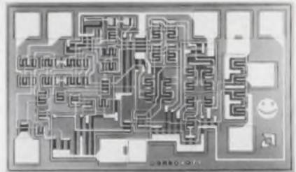
. . . if you were the world's fastest comparator. That's what Jim Giles, Director of Linear Engineering, felt when he designed the Advanced Micro Devices Am685. The device has a 7.5-ns maximum prop delay (measured with a 100-mV step and 5-mV overdrive).
