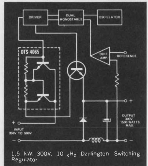
in circuit design where dc drive conditions may have created awkward problems when using SCR's.
