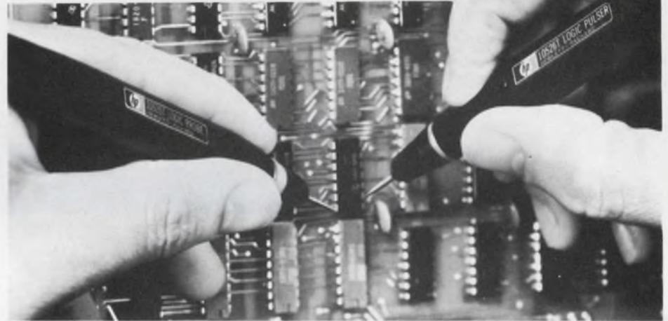
Together the pulser and probe form an IC logic stimulus-response test set that's only the size of two pens.
