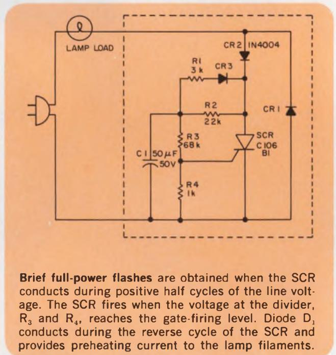
Brief full-power flashes are obtained when the SCR conducts during positive half cycles of the line voltage. The SCR fires when the voltage at the divider,  $R_3$  and  $R_4$ , reaches the gate-firing level. Diode  $D_1$  conducts during the reverse cycle of the SCR and provides preheating current to the lamp filaments.
