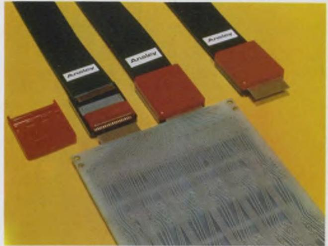
This flat cable, zero-insertion-force connector from Analely clamps spring-loaded contacts to the PC board.
