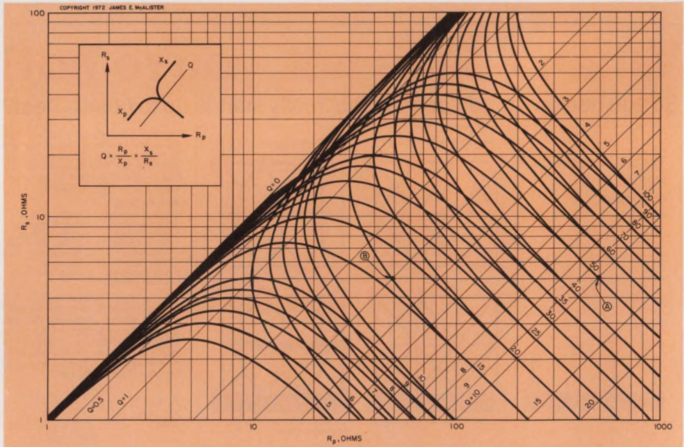
1. Two-element series or parallel networks are represented along with their over-all circuit  $Q$ . The family of curves represents a general series-parallel transfor-
