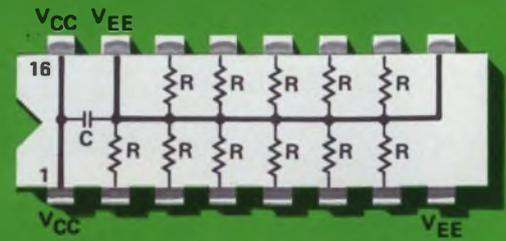
**SERIES 898-42 -5.2 VOLT TERMINATORS** contain twelve resistors for pull-down to the -5.2 volt bus. Each unit contains a 0.01  $\mu$ F decoupling capacitor to bypass the -5.2 volt bus. Price (1,000-4,999) \$1.25
