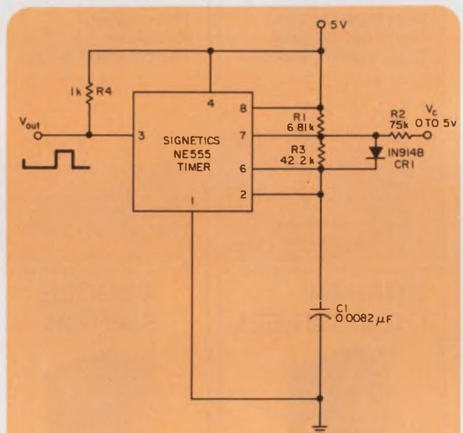
Duty cycle range of astable circuit is increased by the use of diode  $CR_1$ , because the charge and discharge time constants of  $C_1$  become independent. Charging current depends on  $R_1$ ,  $R_2$ ,  $V_c$  and the 5-V supply, but the discharge rate depends only on  $R_3$ .
