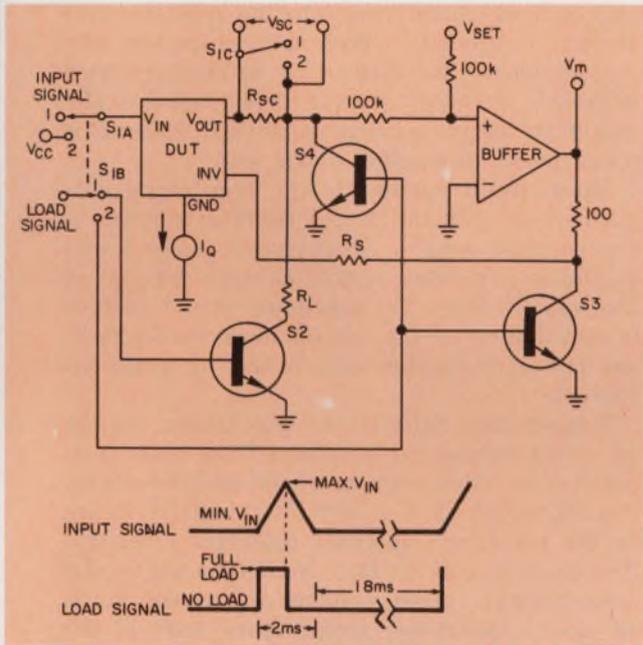
2. To avoid heating the IC chip, line and load regulation are measured semiautomatically with a low-duty-cycle input voltage. Load is varied from zero to full.
