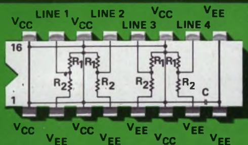
**SERIES 898-43 THEVENIN EQUIVALENT TERMINATORS** contain four Thevenin equivalent terminator sections. Each terminator section consists of two resistors connected as a divider from the ground bus to the  $-5.2$  volt bus providing a Thevenin equivalent voltage of  $-2.0$  volts. Each unit contains a  $0.01 \mu\text{F}$  decoupling capacitor to bypass the  $-5.2$  volt bus. Series 898-43 units are available with Thevenin equivalent impedances of 50, 75, and 100 ohms.
