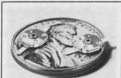
**Thin-Trim®** variable capacitors are designed to replace fixed tuning techniques. Applications include crystal oscillators, CATV amplifiers, communication and test equipment. Series 9410 has high Q's with five capacitance ranges from 1.0 - 4.5 pf to 10.0 - 50.0 pf. Johanson Manufacturing Corporation, Boonton, N. J. (201) 334-2676
