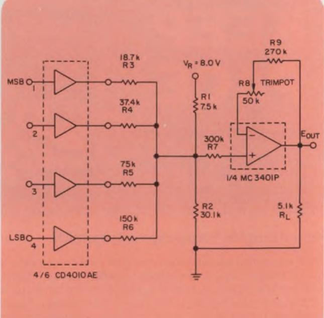
2. Practical four-bit converter is designed on the basis of Eqs. 3 to 5. Normalized values have been scaled by  $10^4$ . Potentiometer  $R_8$  is used to compensate for offset and to obtain maximum accuracy. The calibration point is 0111, with an output of 5.4 V.
