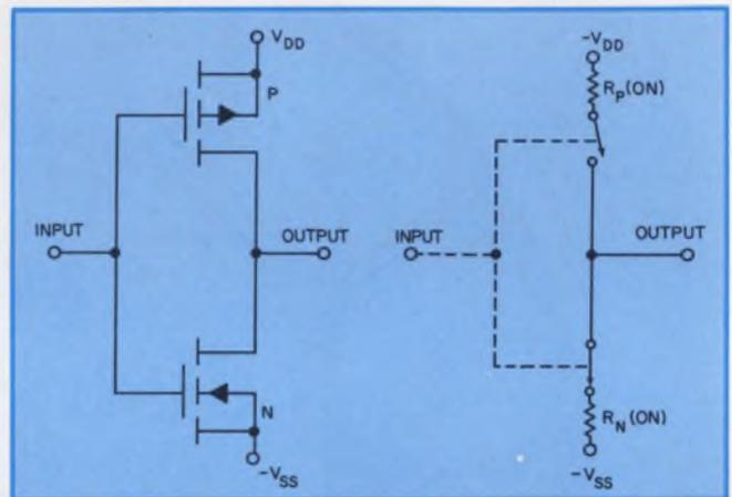
1. The basic CMOS circuit element is composed of a CMOS inverter (left) with its equivalent circuit (right). In SCL devices output signals are driven off the chip with just such an inverter for higher sinking currents. Output impedance—the ON-channel resistance—is typically  $500 \Omega$  for either a HIGH or LOW output.
