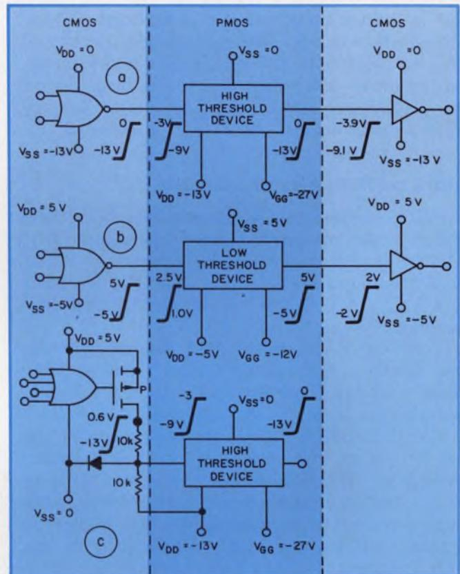
3. The CMOS-PMOS interface can be accomplished by a direct connection, since typical output swings go from  $V_{SS}$  to  $V_{DD}$  (a and b). When interfacing positive-logic, positive-supply CMOS with negative-logic, negative-supply PMOS, the configuration in c can be used.
