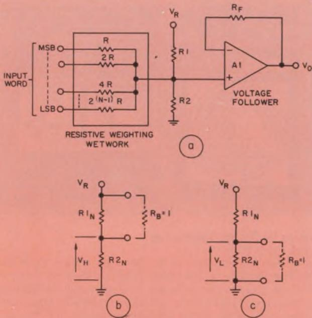
1. Resistive divider, interposed between binary weighting network, allows d/a conversion with outputs that lie between two specified limits (a). The circuit model for calculation of  $R_1$  and  $R_2$  places the binary network across  $R_1$  at maximum output (b) and across  $R_2$  at minimum output (c).
