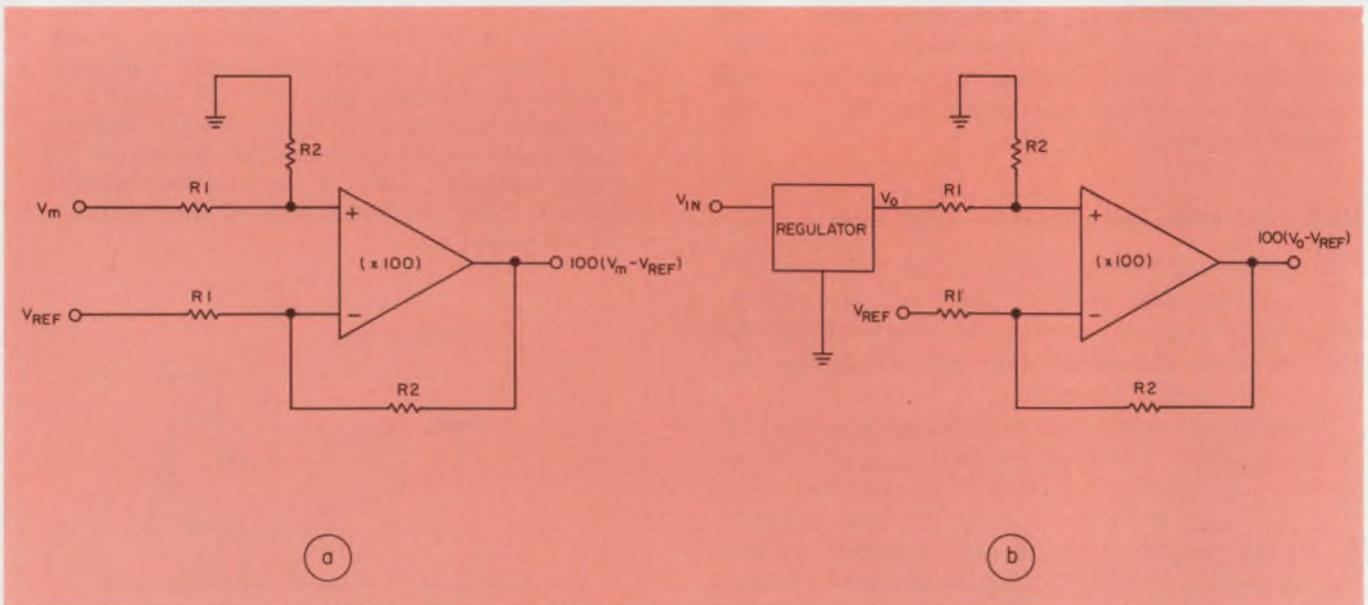
4. Changes in  $V_m$  are small compared with the nominal value of  $V_m$ , making it difficult to determine regulation accurately. Resolution is considerably improved (above) with a difference amplifier. A similar circuit
