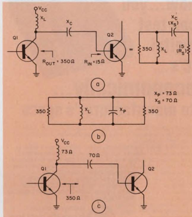
3. A series-to-parallel conversion solves the interstage coupling problem (a) for  $X_L$  and  $X_c$ . The inductive reactance is made equal to the equivalent parallel capacitor reactance of  $X_c$ . No additional transformations are required to determine the value for  $X_L$ .
