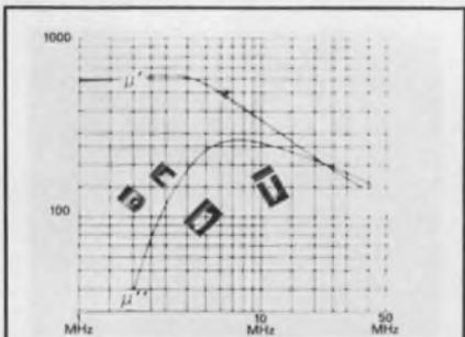
**20 MHz ferrite components** are possible with new "hot-pressed" ferrite manufacturing technique. Extremely low losses and exceptional high frequency performance are combined in these new materials for digital and analog recording heads and inductors. National Micronetics, Inc., Route 28, West Hurley, N.Y. 12491. 914-338-0333.
