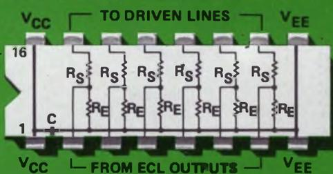
**SERIES 898-44 SERIES LINE TERMINATORS** contain six series terminator sections. Each section is designed for terminating a line at the driven end with a series resistor value equal to the line impedance minus the 7 ohm output impedance for 10,000 series ECL. The second resistor in each section is a pull-down resistor to the  $-5.2$  volt bus. Each unit contains a  $0.01 \mu\text{F}$  decoupling capacitor to bypass the  $-5.2$  volt bus.
