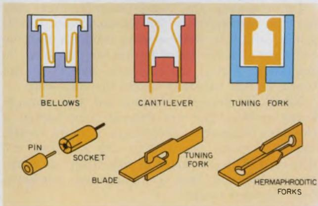
1. There are six basic contact styles. For the one-piece connector, there are the bellows, cantilever and tuning fork. For the two-piece connector, there are the pin-and-socket, blade-and-tuning-fork and hermaphroditic.
