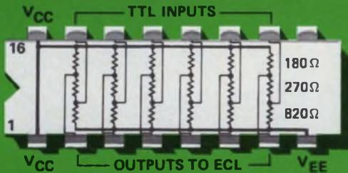
**SERIES 898-45 TTL TO ECL TRANSLATOR** contains six identical three-resistor sections for direct translation from TTL to ECL, both operating between a +5 volt supply and ground. Price (1,000-4,999) \$1.25
