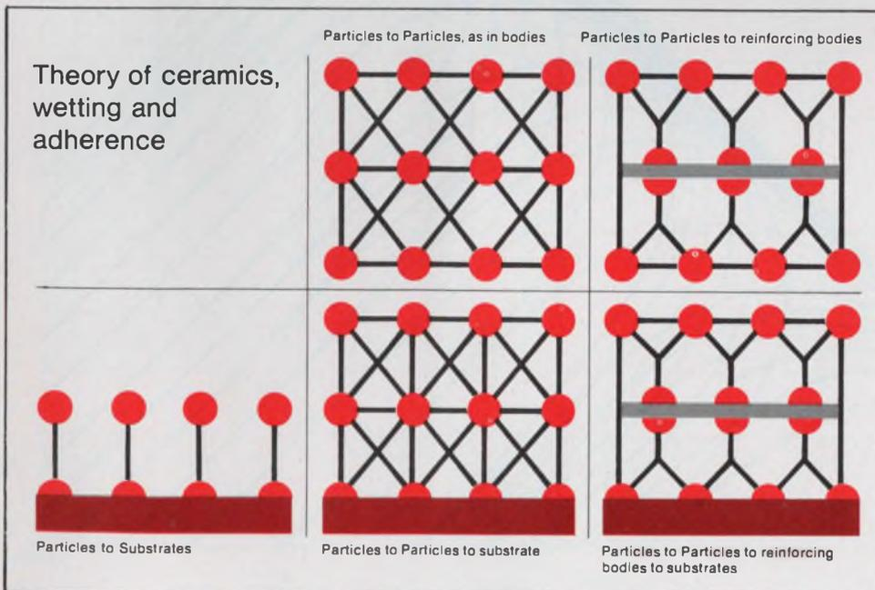
SermeTel bonding product systems have the answer to difficult applications. Can be custom mixed to offer electrical properties ranging from non-conductors to high conductors and bonding for temperatures from  $-375^\circ\text{F}$  to  $6000^\circ\text{F}$ .
