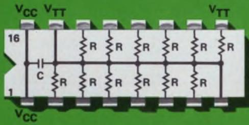
**SERIES 898-41 -2.0 VOLT TERMINATORS** contain eleven resistors for ECL line termination to a -2.0 volt bus. Each unit includes a 0.01  $\mu$ F decoupling capacitor to bypass the -2.0 volt bus. Standard R values of 50, 75, and 100 ohms are available and are designated 898-41-R50, 898-41-R75, and 898-41-R100. Price (1,000-4,999) \$1.25
