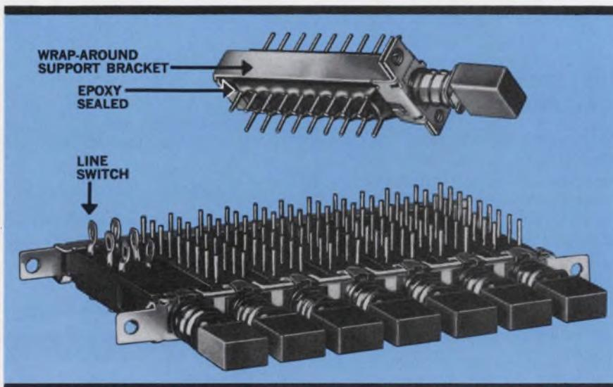
Centralab push button switches\* are available as single modules (wrap-around support bracket optional) or as ganged assemblies. They are rated .45 Amp at 115 VAC or 1 Amp at 28 VAC. Other options include epoxy seal and modular size line switches.
