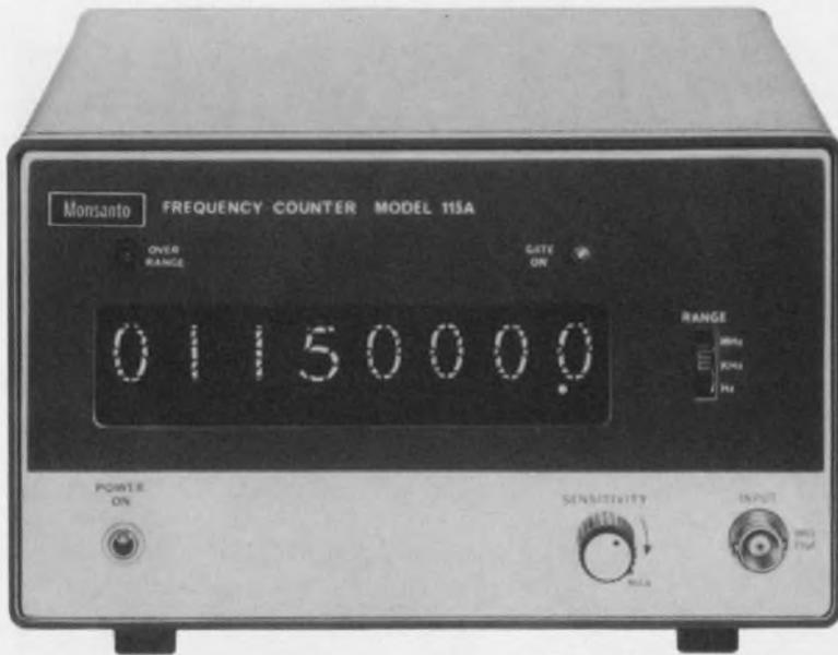
In addition to Monsanto's standard high quality craftsmanship, this great counter has these specific features: standard 6-digit display with 8-digit option — frequency range from 5Hz to 150MHz — sensitivity of 25mV to 80MHz, 50mV to 150MHz — crystal controlled clock — 3 basic time bases — non-blinking display with memory — state of the art circuits including LSI, MOS and MECL 10000 — optional BCD output — optional I.F. subtraction.
