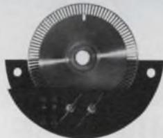
The Decitrak® naked encoder is specially designed for OEM applications . . . a stripped-down, low-cost incremental encoder easily integrated into systems designs. One part of the unit is a coded disc easily mounted to your shaft; the other is an LED light source/photocell assembly ready for installation into your equipment. An economical, flexible solution to your systems design problems! Contact us today for a low, low quote and your **free** copy of our new applications brochure.
