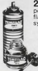
**2. TEMPILAQ<sup>®</sup>:** materials of calibrated melting points suspended in an inert, volatile non-flammable vehicle. Available in over 100 systematically spaced temperature ratings from 100° to 2500°F. Tempilaq<sup>®</sup> indicates its temperature rating by liquefying within  $\pm 1\%$  of its rating. Available in bottles or spray cans.
