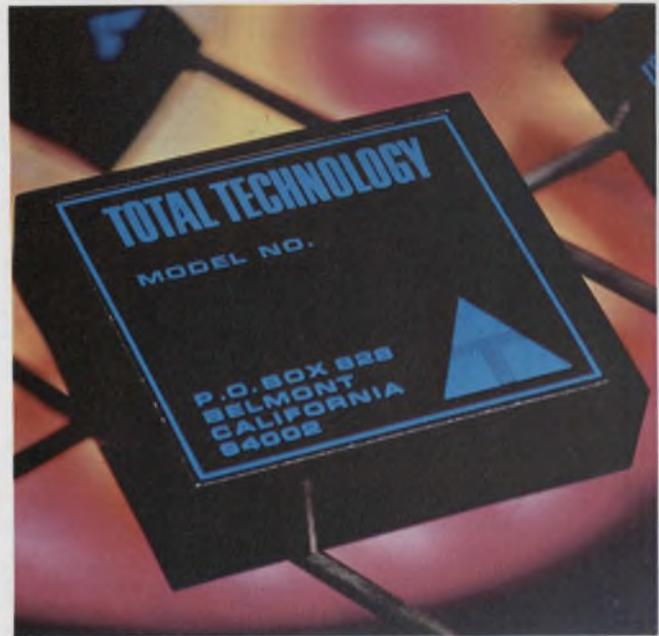
Modules made by Total Technology include function generators, noise generators, voltage controlled amplifiers, antilog amps, bandpass filters, multipliers, and summing amplifiers.
